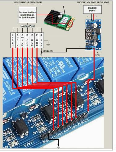
10. Output board signal input wiring.
