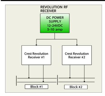
4. The basic Revolution setup with only train control and no sound or accessories.
