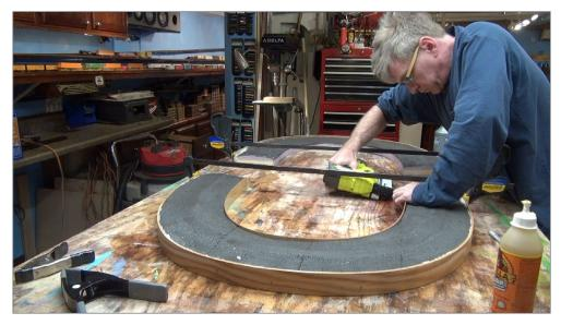
11. Within 5 minutes of attaching the wood sides, I used bar clamps to draw the layout back into the correct shape as the plywood wants to spread the U shape open. The bar clamps prevent this and hold everything to shape as the glue cures over 20 to 30 minutes. Once the glue sets up, you can remove the clamps and the layout will hold its shape.
