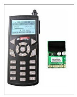
The Revolution is a wireless radio system operating in the 2.4 GHz frequency range between the handheld unit and its receiver(s). The only wires are what's needed to connect the receiver to its power (can be batteries in G scale), any control relays, and a speaker for sound.
