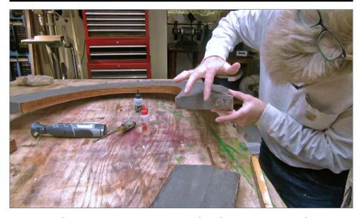
13. I used 5-minute 2-part epoxy to glue the magnets into their routed circles. I placed a piece of paper between the modules as they were connected, ensuring precise alignment as the magnets find each other, "snap," and mate up. The paper prevents the modules and or the magnets from permanently attaching to each other while the glue cures and sets up. I did this same process with all eight magnets holding the layout together. Watch and follow this process in the video portion of this column
