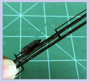
17. Brake/center sill assembly so far. Here is how the assembly looks at this point with the clevis and brake lever fit together, and the center sill parts held in place. My fingers are holding it all together for this photo.
