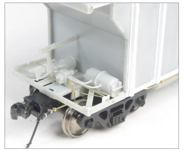
Plano Model Products makes a beautiful etched metal set for rebuilding the end cages of PS 4427 cubic foot covered hoppers. Some of the pieces in the set are not useable for these cars but the ladder posts, stirrups, cut lever brackets, rope pull loops, and crossover platforms work great.
