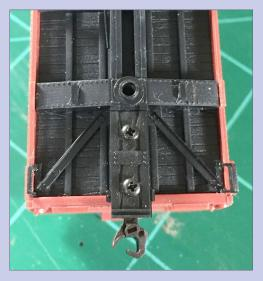
33. Proto:HO couplers fit great, too. If you use the Accurail **Proto:HO scale couplers** (that is my preference), they have a cover that reflects the prototype draft gear. The lid is not needed when installing these on the 36-foot box car kits. These couplers also have less play between coupled faces and reflect the prototype with a closer coupling than other couplers. The Accurail **Proto:HO couplers have** worked well on my freight cars.
