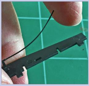
**15.** Careful to not snap off the brake rod. As I said before, the brake rod casting is made from a flexible material; just don't bend it too far!
