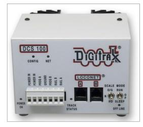
2. Track connections on Digitrax DCS100. The "main" track connects to RAIL A and RAIL B (right side of the grey connector). The "programming" track connects to PROG A and PROG B (in the center of the same connector). *Bruce Petrarca photo*
