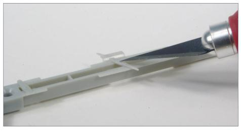
11. Remove this brake rigging from the center sill.
