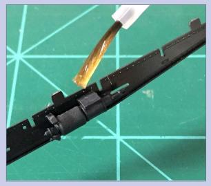
12. Apply cement to brake cylinder. A touch of styrene cement holds the cylinder in place. Cement also can be applied to the back side of the center sill casting.
