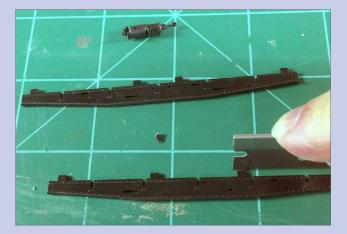
**5. Cut off sprue nubs with sharp blade.** My favorite cutting tool is a fresh single-edge razor blade although an X-Acto knife with a fresh blade will work as well. I start each project with a new blade for clean cuts.
