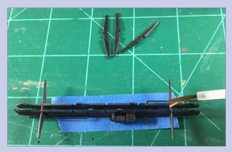
21. Cement two cross bearers in place. A touch of styrene cement fixes the two cross bearers in place.
