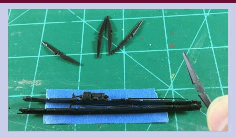
19. Get the five cross bearer castings. Don't worry, we will correct the odd center sill parts spacing shortly. The tape keeps the center sill sides standing up and not falling over – which is mainly what we need to make final assembly easier.
