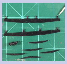
4. Roughly trim parts from the sprue. Use the flush nippers to remove the parts from the sprue by cutting through the sprue back a bit from where the part joins the sprue. I am pointing with the toothpick at the excess sprue nub to be removed with the sharp blade.
