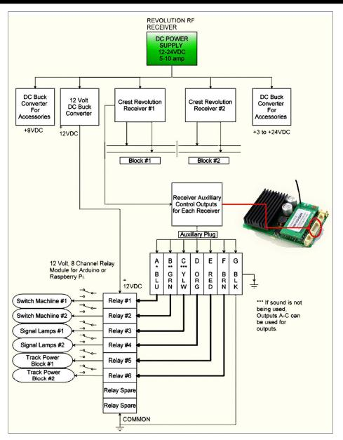
7. Adding accessories to the receiver involves not only extra wiring, but providing a power supply for the accessories you are powering.
