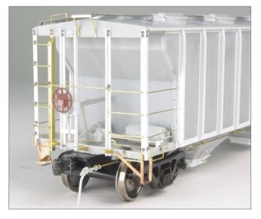
26. Completed end of car with roof walk supports and brake wheel.
