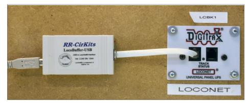
4. Computer Interface LocoBuffer-USB for Digitrax command stations. This was a prior installation at our club (pcmrc.org). The LocoBuffer-USB has since been moved behind the fascia panel and connected to one of the rear jacks on the UP5 panel. *Bruce Petrarca photo*
