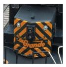
New DRGW late delivery nose with protruding gyralight
