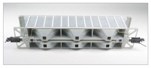
16. New train line made from .015" brass wire follows the outside of the car.
