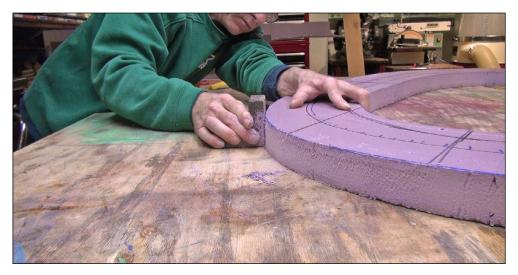
7. To start the N scale layout, I drew the layout's dimensions on a sheet of two-inch pink foam. The track radius is about 14 inches and the layout's overall size is 3'x4'4". It could be expanded by adding more modules, as you will see.
