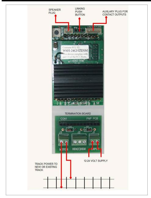
5. Receiver showing electrical hookup points to both the receiver and termination board.
