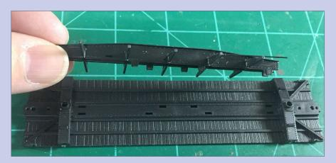
**24. Check underframe assembly fit.** Now we can check the installation on the car bottom casting. The center sill casting tabs are keyed to slots on the car bottom casting.
