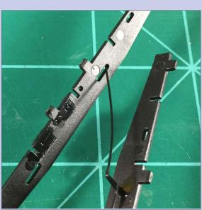
16. Thread brake rod through other sill. Now thread the other brake rod end through the center sill that has the brake culinder on it. The long brake lever goes through the other wide slot and inserted into the clevis on the brake cylinder. Remember we started out by testfitting it [9, 10].
