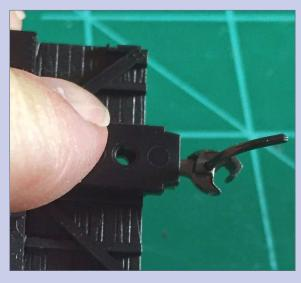
**30. Attach the coupler box to the car bottom.** The assembly slides into place on the car body bottom. Install the screw provided in the kit to finish it up.
