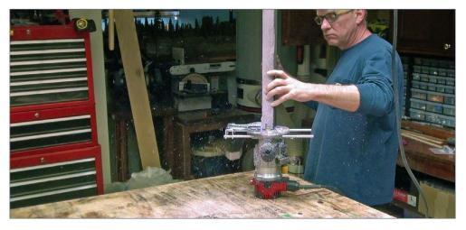
9. To create a solid surface to mount the magnets, I set my router to a depth of <sup>3</sup>/<sub>4</sub>" and used a <sup>3</sup>/<sub>4</sub>" straight router bit. I then guided the ends of the layout along the router fence to cut a straight groove into the ends of the foam sections.
