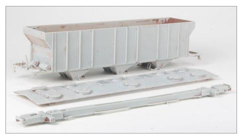
29. Athearn car disassembled and paint stripped using 99% isopropyl alcohol.
