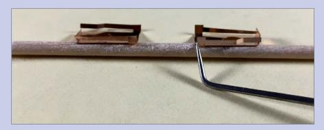
**28. Coupler spring modifications.** I've heard of modelers having difficulty installing #58 Kadee couplers on these models. They say the #58 flat coupler spring does not fit. I trim parts of the spring: here is a comparison of a trimmed spring on the left and a spring straight from a new package of Kadee #58 couplers on the right. Note the difference in height front and back. Use flush-cutting nippers and carefully file any rough remains away. Once the spring is modified, it fits fine.
