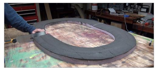
8. I used blue painters masking tape to represent the N-scale track in the middle of the layout, following the flow of the ovalshaped circuit, then carved the track profile and topography with a horse rasp and Stanley Surform planer. I sealed the top of the layout with brown latex house paint and cut the layout into two pieces at the center of the oval, as you see here.
