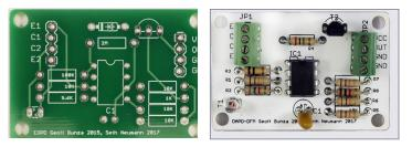
Also new from MRCS is an Enhanced Optical Position Detector
