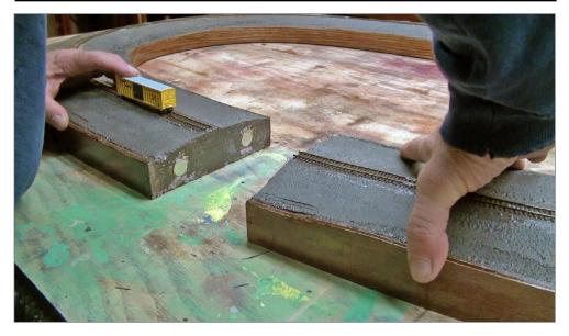
15. When the track was firmly in place, I cut the rails apart at the module connection points on each side of the layout. I then pulled the layout apart, placed an N scale box car on the track and snapped the layout back together. The magnets made a solid connection and the rails lined up perfectly as I rolled the box car across the connection.
