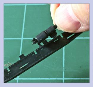
11. Install brake cylinder onto center sill. At this point, we can install the brake cylinder to the proper center sill part. It fits only one way.
