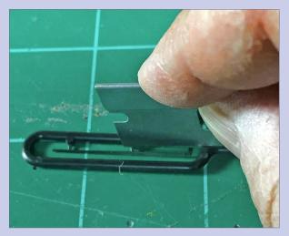
6. Cut "closeclearance" sprues with the sharp blade. The brake levers and rods are a onepiece casting with tight sprue clearances. I use the sharp razor blade to cut the sprue here on these parts.
