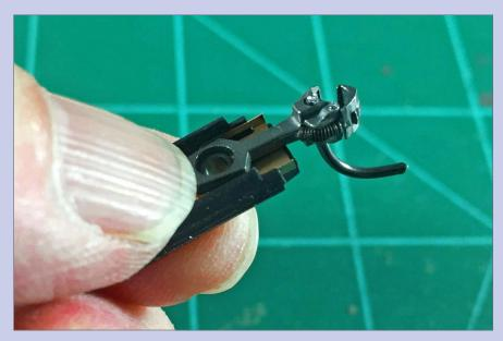
**29. Install the coupler spring in the box.** I install the spring in the lid first and then add the coupler.
