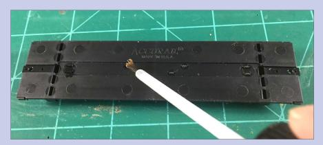
**26. Apply cement from above.** Touch the tabs with some cement from the top side of the car body casting. Allow this to completely dry before installing the car weight.
