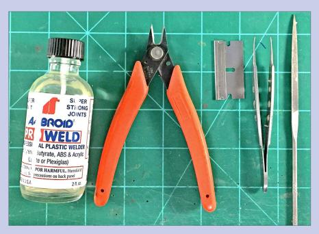
**3. Gather the tools needed for assembly.** Styrene cement is used in a few spot applications. A sharp blade like a fresh single-edged razor blade or an X-Acto knife with a fresh blade is a must for removing larger parts from the sprue. The orange-handled flush side cutter also works to remove the parts from the sprue [4]. Keep a roll of masking or painter's tape handy for the later steps.
