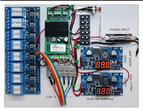
12. My complete unit showing the receiver, the relay board and two auxiliary power supply boards.
