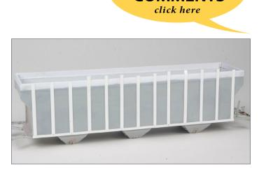
32. Strips of .005" styrene added to hopper sides.
