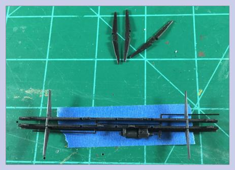
**20. Install two end cross bearers.** Carefully install the two cross bearer castings at the ends of the center sill. Adjust the center sill spacing on the tape so the cross bearers fit into place. The angled part of the cross bearer castings is facing down toward the tape for this installation. The top is flat as it goes against the car floor.
