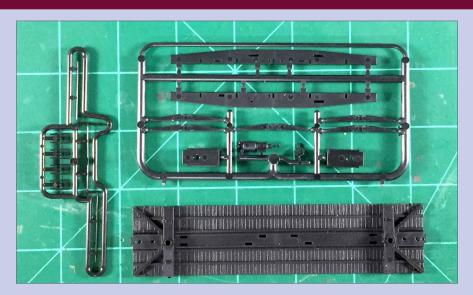
**2. Gather the underframe parts.** The sprue on the left has the brake levers and rods cast in a flexible material. Above the main underframe part is the sprue with the center sills, K brake component, cross bearers, coupler box covers, and the brake wheel.
