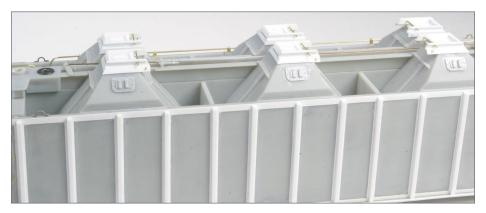
25. Completed hopper outlets and slack adjuster glued in place on center sill.
