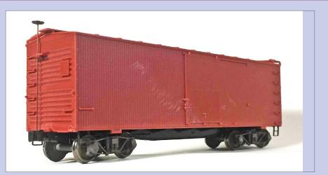
**34. Snap on car shell, add steps and trucks.** With the car shell in place, the double-rung sill steps fit into their locations. The sill steps are cast in engineering plastic and are designed for a press fit. Then screw the trucks onto the car bottom, and the model is ready for painting and decaling! I substituted AC&F arch bar trucks by Tahoe Model Works [resincarworks.com/ tahoe.htm] for the Accurail kit trucks.
