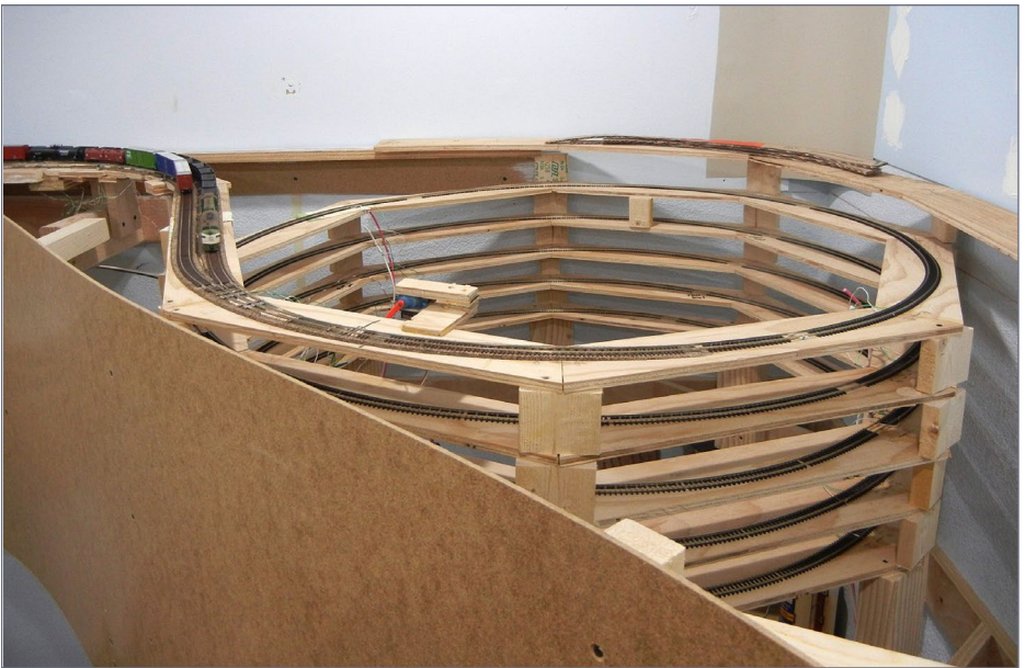
13. The other helix is between Rice and Milligan, in the opposite corner of the room, also an 18" radius and a 2-3/8" climb per loop.
