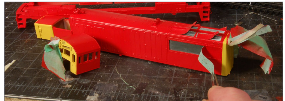
12. Shell and cab masked and ready for a coat of red paint.
