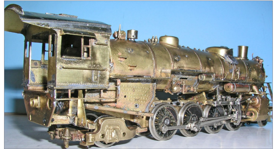
13. More major detail added to the engineer's side.
