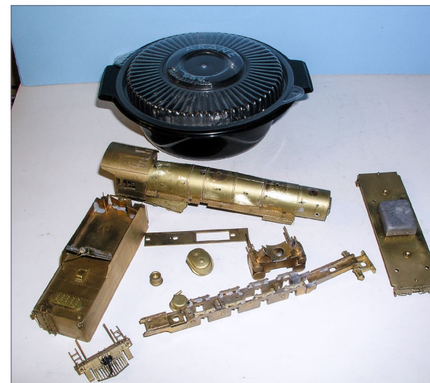
3. The model with some of the unwanted boiler detail unsoldered and removed. I went on to also remove the running boards, cab, boiler backhead, and smokebox front.
