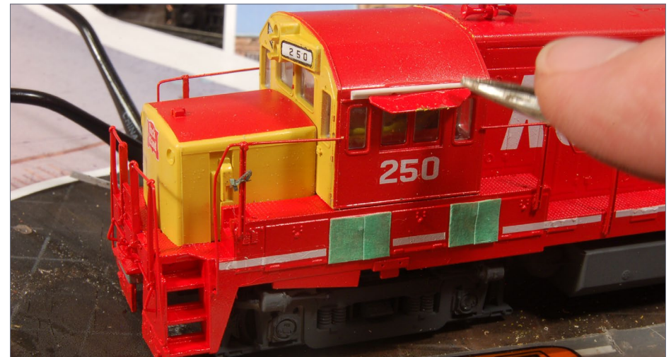
18. Attach the sunshade bracket. Also note the masking of some battery box doors to keep them free from weathering and simulate the freshly-painted look of these doors on the prototype.
