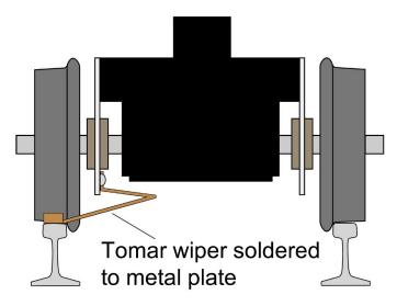
4. I added the Tomar wiper to the blue-box Athearn loco by folding it and soldering it to a truck's metal plate as shown. By adjusting the V-bend angle, I can control how much tension the wiper puts on the rail.
