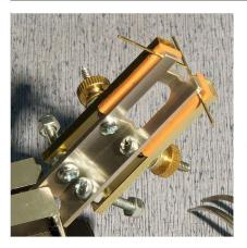
Coffman Engineering has introduced a new website at coffmaneng.com and announced their newest corner clamp, the AC-8-3 Mini Combo Right Clamp. With a jaw length of one inch, the clamp features a vise tab at the end for hands-free operation, high temperature silicone rubber pads to allow the modeler to solder while the pieces are in the clamp, two sets of
