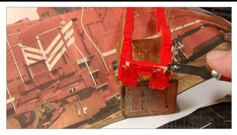
15. Removing incorrect front pilot details using an X-Acto blade.
