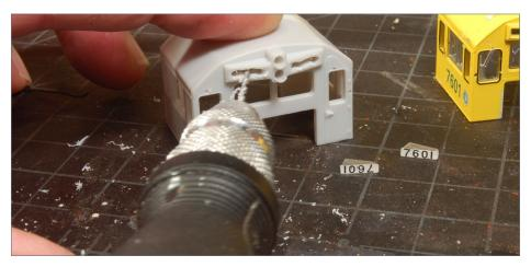
6. I hollowed out the cast number boards on my cab, starting with a drill in my motor tool.
