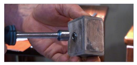
11. While the track glue cured, I built a small wood box from scrap pieces of ¼-inch oak. I then drilled a hole in the box to accept a 2-conductor microphone female jack.
