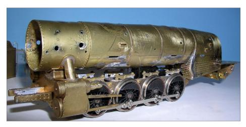
6. The stripped boiler minus all the detail, running boards, cab, boiler backhead, and smokebox front. To start the rebuild, I added firebox front sheet castings.
