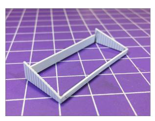
27. As always, don't forget to remove any paint from gluing surfaces. This is especially critical here where the mating surfaces are so tiny. Be certain that the four pieces are flush on the bottom or your porch roof will be slightly off.
