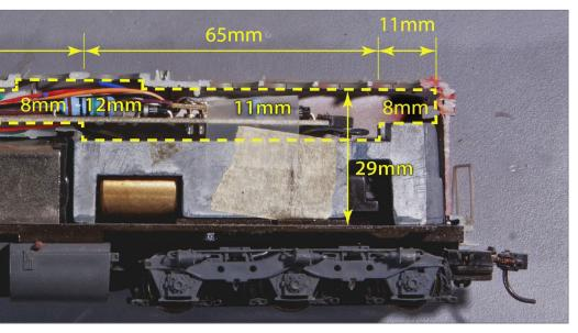
average closer to 6mm above the motor and weights. Older Bachmann diesels have even less space, with the weight taking all but a few millimeters of the space inside the top of the shell.
