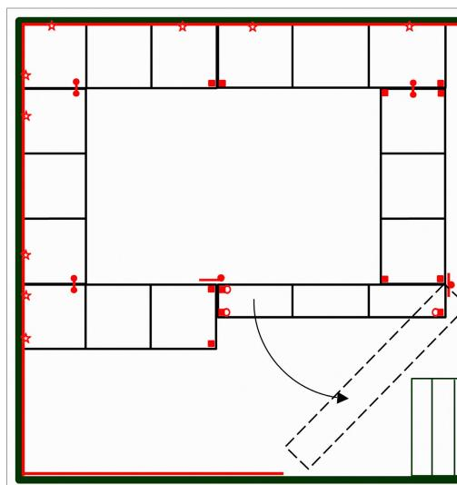
8. Stage 1 benchwork construction: module benchwork in black, supporting structure in red.
