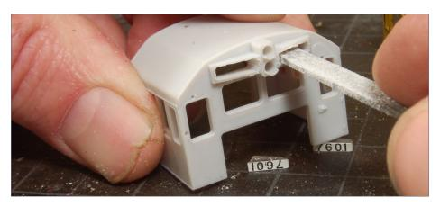
7. I finished opening the cab number boards using a small file, working slowly until the factory number boards fit perfectly.
