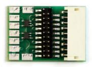
SoundTraxx has introduced a simple device (JST-21PNEM) that adapts any SoundTraxx 21PNEM decoder to an NMRA 9-Pin DCC quick-plug equipped model. The JST-21PNEM can also be used with a SoundTraxx 9-Pin JST Power Harness to create a universal-
