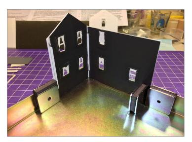
15. Next, I used a very handy magnetic gluing jig to true up the walls to a 90-degree angle and hold them in place while I applied cement to the joint.
