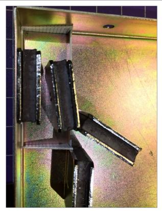
26. You can see I rely pretty heavily on this magnetic gluing jig. No less than four magnets hold everything square in the corner for gluing. Like the main walls of the house, I first glued two pieces together, making two 2-piece assemblies (2 "L"s) before I glued the 2 "L"s together.
