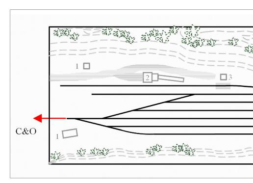
4. Elkhorn yard module, 2 x 6-feet, N scale. Structure key: (1) shed, (2) coal loader, (3) track scale, (4) office, and (5) fuel tank.
