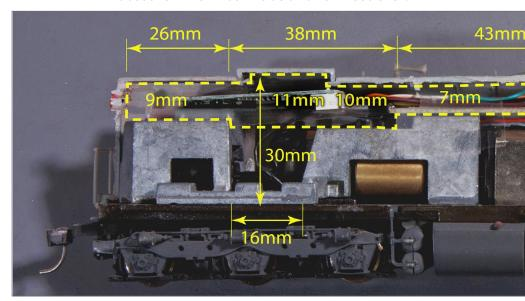
9. To give you an idea of the space typically available inside an HO diesel loco, here is a cross-section of a Proto-2000 SD9. This loco is actually fairly roomy above the motor and weights. Some locos
