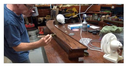
9. I stained the wood to match my layout room and then applied 4 coats of polyurethane, wet sanding between coats for a smooth finish. This will seal the plywood to prevent it from warping or sagging due to humidity.
