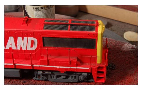
21. The finished grilles after removing the masking.
