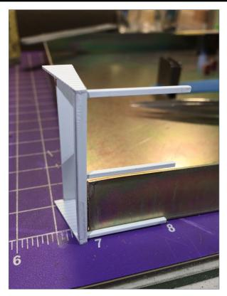
28. I next added the roof support legs to the roof support frame. Be sure not to force the legs at all when you insert them between the roof frame sides. File/sand to fit as needed, or else risk forcing the frame apart. It's also important that the supports be at a right angle to the frame, as shown.
