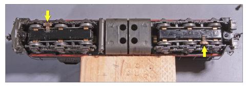
2. Adding Tomar phosphor-bronze railhead sliders (yellow arrows) to this blue-box Athearn loco makes it extremely sure-footed when it comes to electrical pickup. Note the old-style sintered metal wheels are not particularly clean, yet the loco still runs without stalling!
