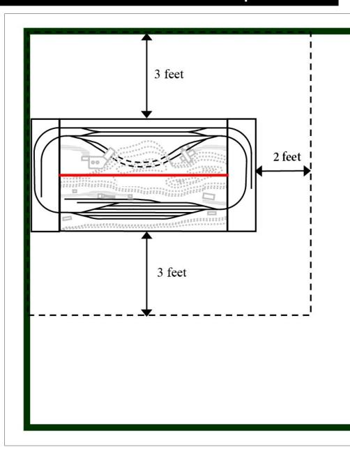
7. Island layout positioned in basement. Required footprint for layout and crew access is about 10 x 10 feet.
