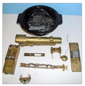
2. The disassembled model after stripping the paint.
