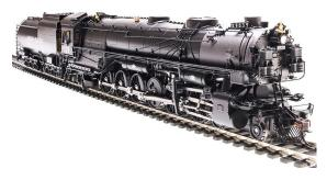
The 4-12-2 was the largest North American steam locomotive built with a rigid wheelbase. In the 1920s Union Pacific used 2-10-2 and 2-8-8-0 locomotives on main line freight trains
