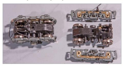
6. Many modern HO diesel trucks have metal plates in the side frames like you see here. The electrical contact point becomes the wheel axle tip through a hole in the metal plate. The reliability of the electrical path depends on how much slop exists between the axle tip and the hole.
