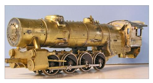
7. Progress so far with the new cab installed domes replaced, and the new smokebox front in place.
