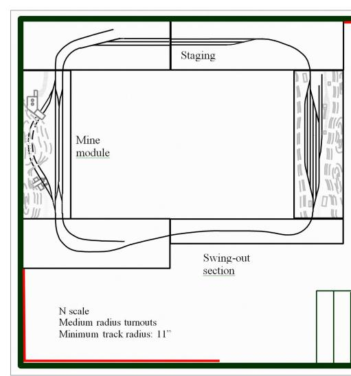
9. Stage 1 module layout and track plan. Overall layout dimensions are 8 x 13-feet. A 6 x 9-foot inside area is available for the operators, accessed via the swing-out section.
