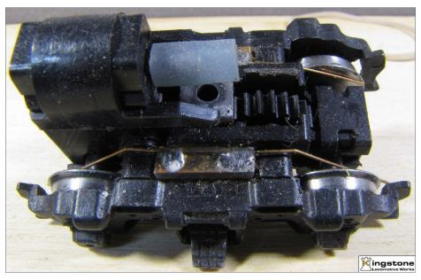
5. Adding wheel wipers to a loco such as those shown here adds an alternate electrical path directly from the wheels and bypasses the sometimes weak wheel-to-axle-to-metal-plate path. Adding a wire from the wiper PC board to the loco motor PC board or decoder also improves reliability by providing a second path for the electrical current. *Photo by Bernd Fanghanel*
