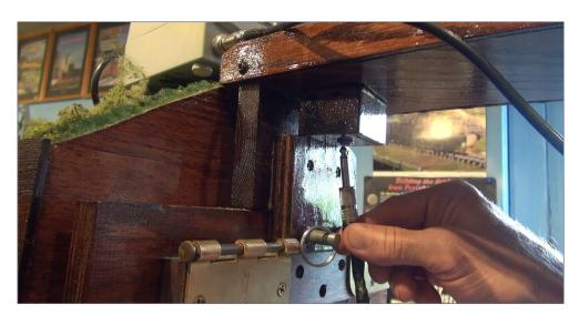
13. The wood box was glued up under the lift-out section. The male microphone jack simply plugs in, providing track power to the section.
