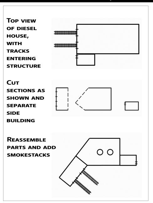
11. Kitbashing steps to convert the Walthers Diesel House to a power plant for use on the mine module.
