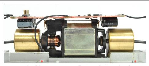
13. Example of how a TCS Keep-Alive® motherboard replacement locates the capacitors in otherwise dead space over the flywheels. This clever trick allows fitting stay-alive into locos more easily. *Photo by Train Control Systems*
