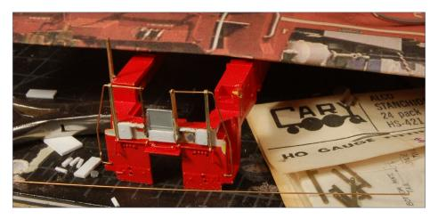
16. New front pilot details match the prototype loco.
