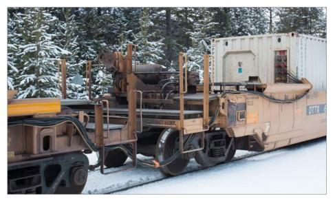
3. Connections between cars and the generator-set container. While the containers are on the train they are powered by the genset. Once they are off, other power sources are used. *Andrew Hall photo*
