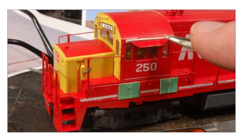
18. Attach the sunshade bracket. Also note the masking of some battery box doors to keep them free from weathering and simulate the freshly-painted look of these doors on the prototype.
