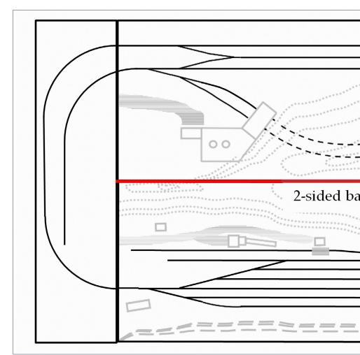
6. Island layout configuration, 4 x 8-foot overall size. The yard and mine modules are placed back to back and two end modules are added.
