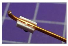
33. I next routed out the back with an .060" drill bit in my Dremel, being careful not to break through the front. A foot/speed pedal really helps here. I bent the wire and clipped it so that most of the curve was gone and it would fit
