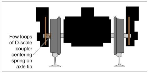
7. To improve power pickup on locos that rely on axle-tip-to-side frame contact, put a few loops of an O-scale coupler centering spring on each axle tip. Don't overdo it, though, or you'll start to create extra drag and limit your loco's pulling power. Just a few loops with minimal pressure guarantee a current path between the wheels and the side frames.
