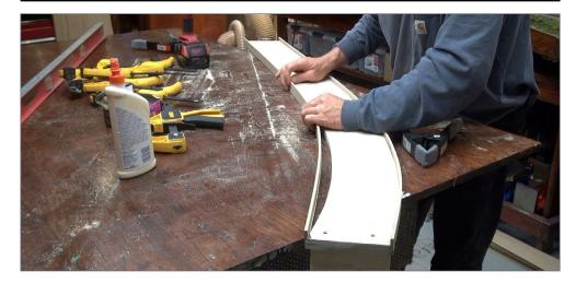
8. Moving back to the workbench, I cut two strips of ¼-inch plywood to form protective walls 3/8-inch-high along both sides of the main. This was glued with wood glue and screwed in place with 3/8-inch metal screws.
