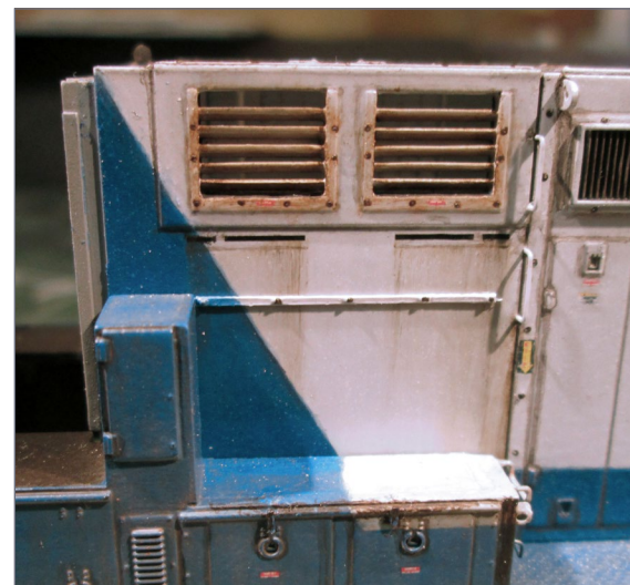
57. Location of the batten-and-bolts strip above the A/C unit (A/C unit temporarily removed).
