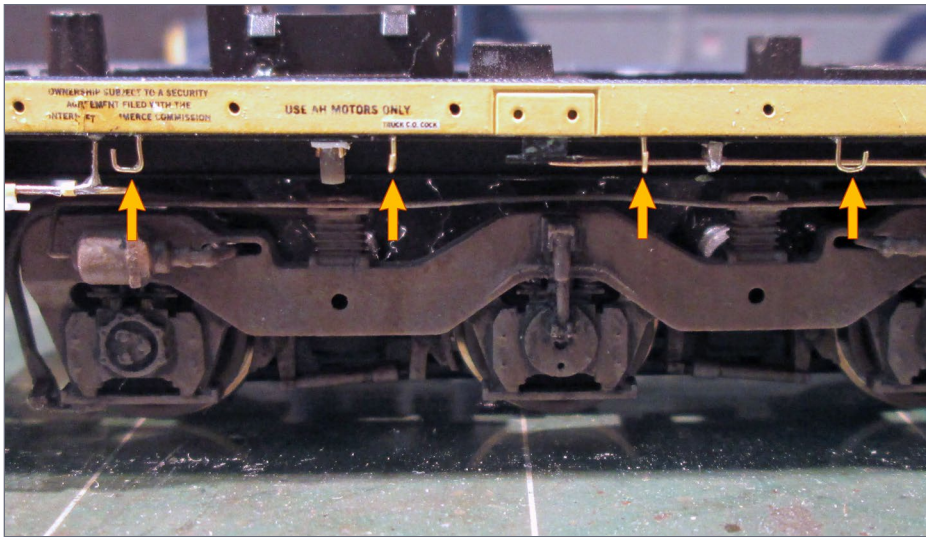
41b. More hangers for chain on the side sill, indicated with arrows.
