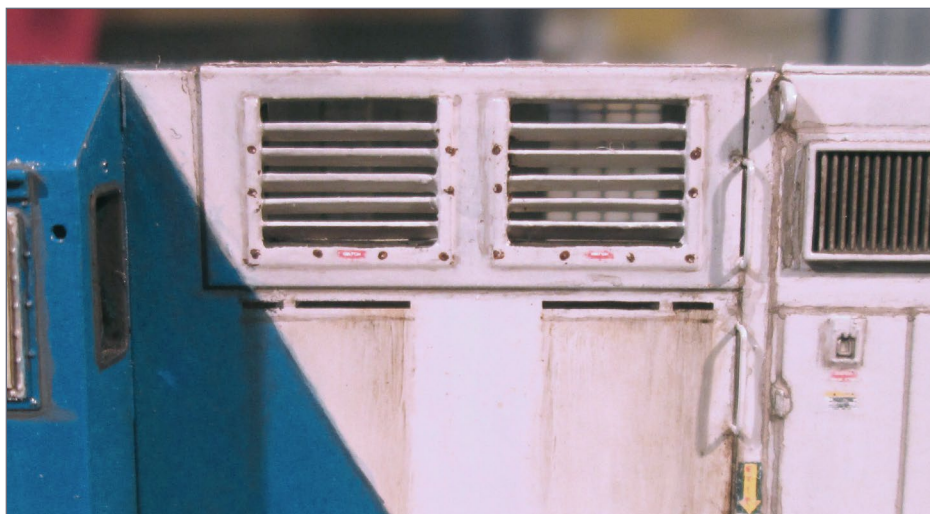
50. Creating apparent hood slits using decals plus some weathering.
