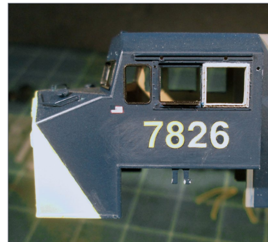
44. Altering the loco cab number from 7799 to 7826.
