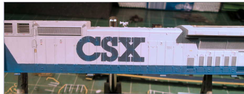
46. Applying a fade coat to the blue on the long hood.
