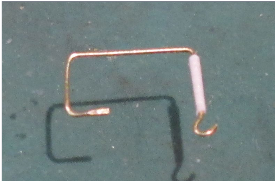
40a. Scratchbuilt hanger for hanging chain from truck side frame.
