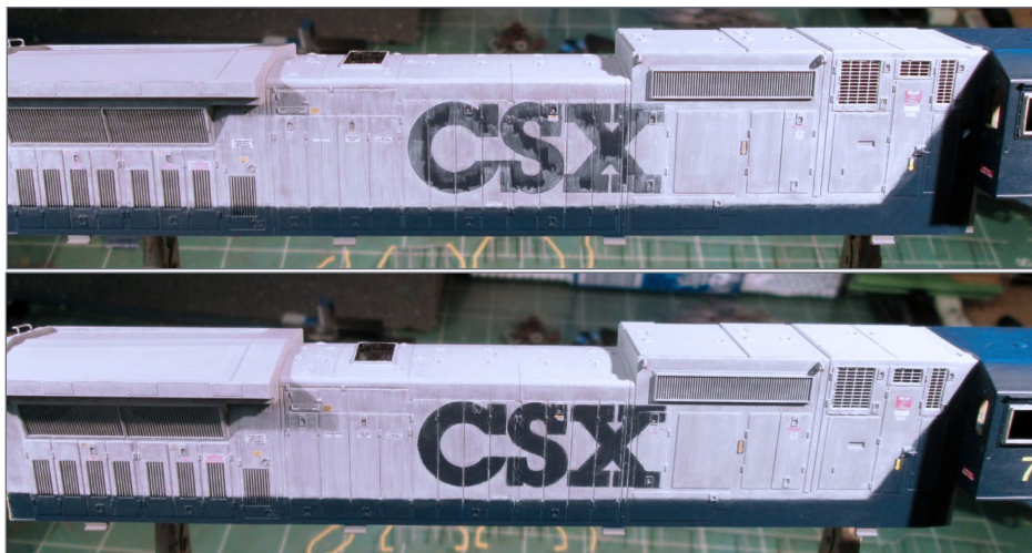
45a, b. Applying a fade coat to the gray on the long hood and subsequent cleanup.
