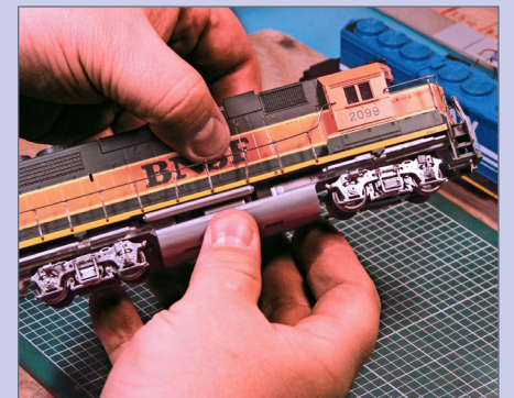
5a, b, c. Removing shell with bottom pins: To remove a shell which has the bottom internal retainers, grip the fuel tank, and gently squeeze and rock the body until it comes off.
