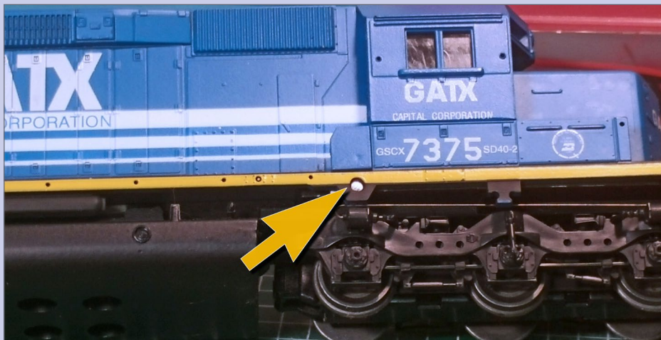
3a, 3b. Finding shell retainer pins: Shell side retainers are used on many Blue Box locos.
