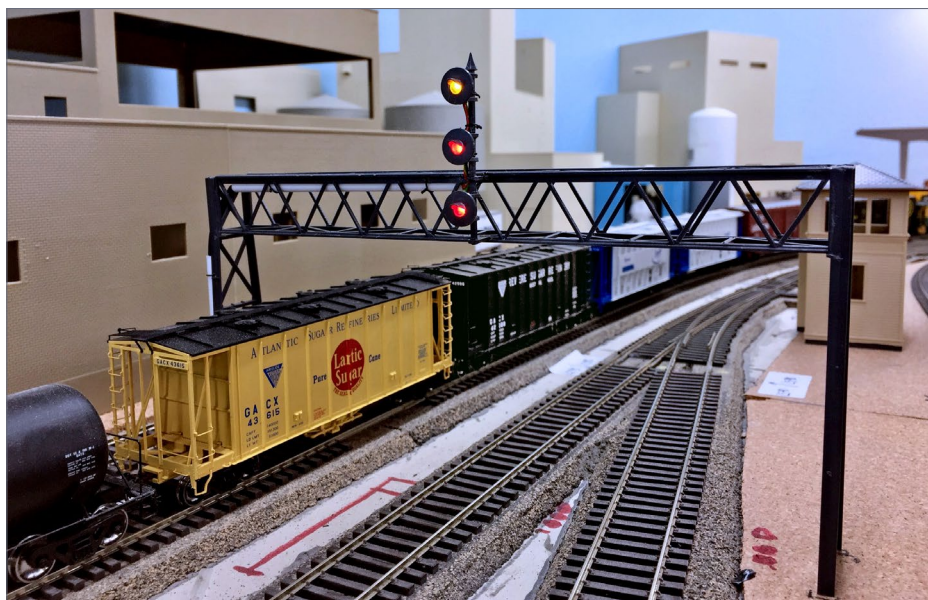
34. A universal-style signal bridge can span two to four tracks.
