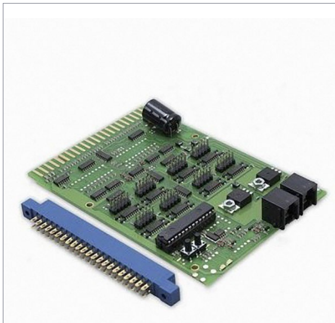
43. The Digitrax SE8C can drive 32 signal heads. It also can drive eight slow-motion switch machines. Each of the signal cable outputs can drive four separate LED signal heads.
