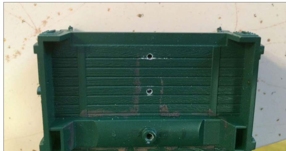
7. The holes go all the way through the car floor. While this isn't desirable per se, I can easily snip off any portion of the mounting screws that protrudes through the floor.
