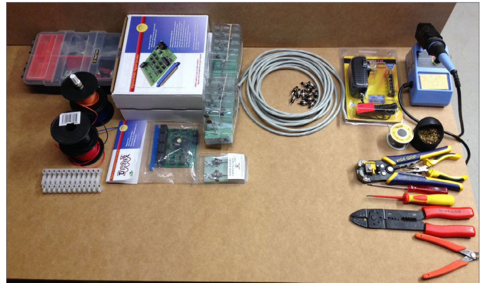
3. Some of the hardware, materials, signal masts, and tools required to install the detection and signaling system on my layout.
