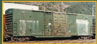
BCOL - 100,000 series, re-built 1990s w/vents, w/team door
