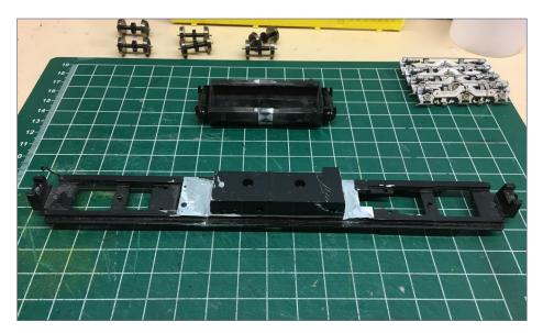
6. I had to mill down the ends of the metal block on the bottom of the chassis so the extended C30-7 fuel tank would fit. This was made easy work thanks to my Dremel motor tool. This also shows the fuel tank before painting, and the trucks after painting.
