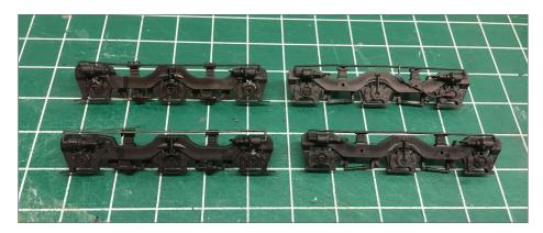
9. The Adirondack side frames after "rebuilding" (on the left), next to the newer GSC side frames. I used parts from the other pair of GSC side frames to update the Adirondack side frames. Now they look very similar, except for the placement of the holes.
