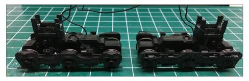
8. Test-fitting the older Adirondack side frame on one of the C40-8 truck assemblies. Again, the older Adirondack truck is on the left, and the newer GSC truck is on the right.
