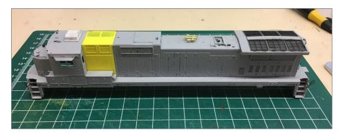
13. Test-fit the parts on the sill to make sure they have been filed down appropriately. The air conditioner is added to the top of the cab and the new five-chime brass air horn is attached to the center of the long hood. I will wait to add the exhaust stack so I don't have to repaint it silver.
