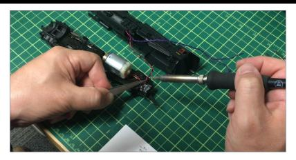
27. He makes a map of the wires, power positive and negative, the light wire feeds and speaker feeds, by drawing a diagram of the existing wires on a piece of paper. Following this chart, George solders the wires through the plug. He then reattaches the boiler to the power assembly.
