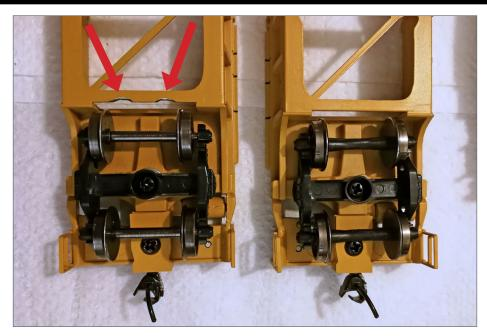
5. Before and after. You can see the notches I milled into the frame.
