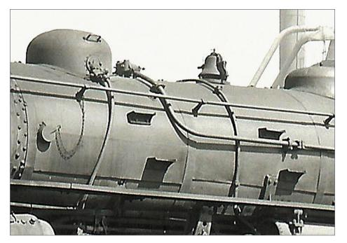
17. Boiler mid-section on the prototype loco.
