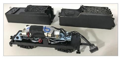
9. Broadway Limited tender chassis with electronics and twin speakers. In the back are the two different tender bodies – see the text for details.
