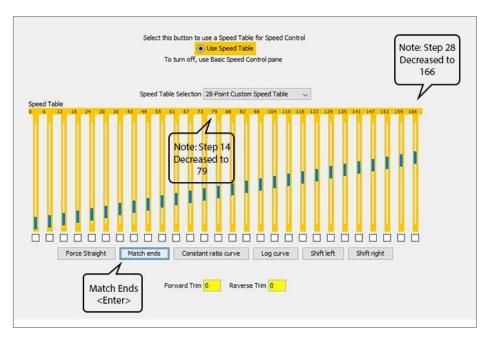
6. Adjusted linear speed curve.
