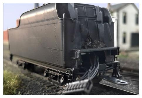
10. I needed to cut a slot in the replacement tender body to allow all the wires to pass through.
