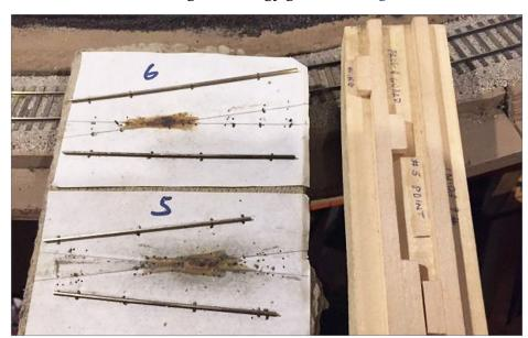
3. Jigs for cutting rail allow all pieces to be cut to the same length and create a "kit" of prefabricated pieces.
