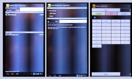
20-22. Engine Driver Setup: server setup, set loco address, change to throttle and run!
