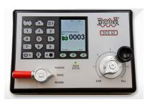
**Digitrax** displayed a wide range of electronic items in their Amherst booth including their DCS 52 Zephyr Express, a 3.0 amp LocoNet command station, booster, and throttle. This latest version features a backlit 3D
