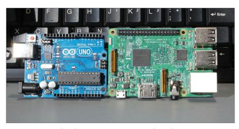
1. Arduino Uno (left) and Raspberry Pi 3B (right).
