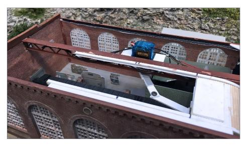
10. The servo, linkage, and door in the closed position.
