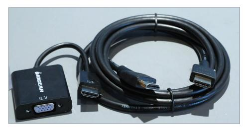
9. VGA to HDMI Adapter & HDMI Cable.
