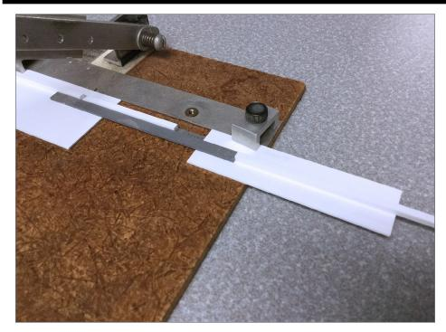
6. Now the stop has been turned end-for-end and is positioned to cut longer pieces of material.
