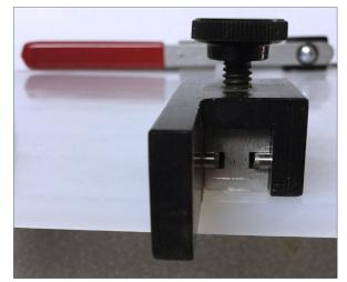
18. This close-up shows the sliding stop pushed beyond the right end of the tool. The two pins on the black sliding stop engage the aluminum H channel which is partially visible below the lock bolt. Turning that lock bolt will lock the sliding stop in place.
