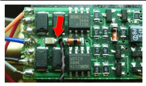
6. NCE D14SR negative (ground) connection location on the decoder circuit board. *Photo by Marcus Ammann*
