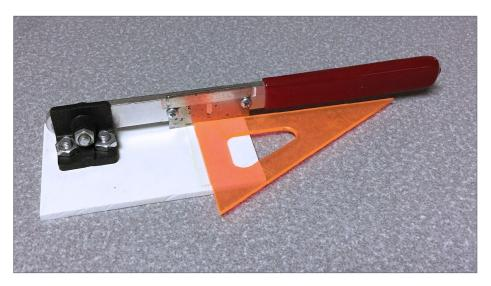
11. This shows how to ensure that the fence is at a right angle to the razor blade.
