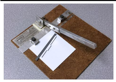
8. The stripwood to be cut is placed on the back side of the fence for the first cut.
