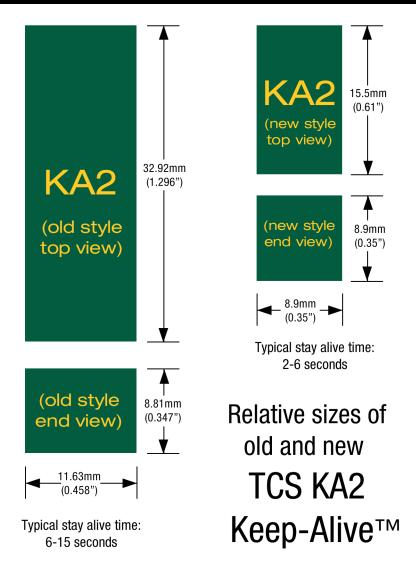
3. Diagram showing the size and stay-alive differences between the old TCS KA2 and the new much smaller KA2. Narrow hood diesels have about 18mm of width inside, which means the new KA2 can go in the shell sideways! Also, the clearance above the motor inside typically is 8-12mm in spots.
