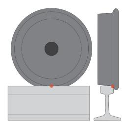
1. The electrical contact between wheels & rail is on the inside rail head and quite small.
