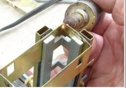
Clamps for soldering and gluing!
