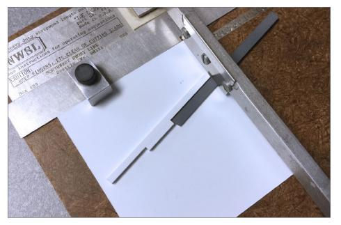
9. It is then reversed and the cut end slid up to the stop for the next cut. The piece can then be turned over and pushed up to the stop for the next cut.
