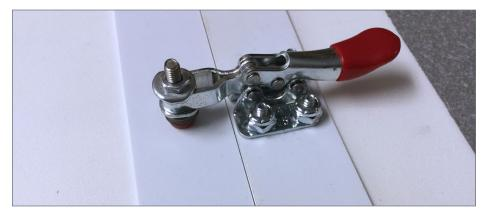
13. A close-up of the hold-down toggle clamp in the clamped position.
