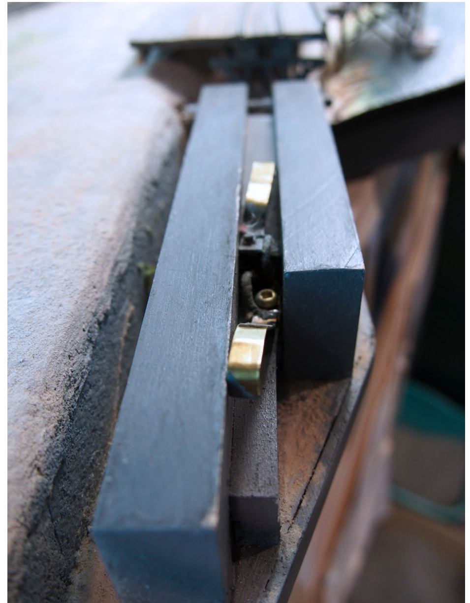
13. Closeup of the docking base with its electrical contacts. Crude, but it works!
