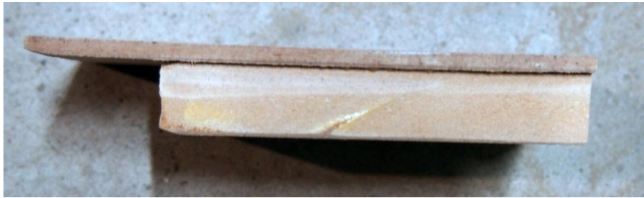
18. The end door construction. A piece of 1/8" hardboard, cut over-sized so it overlaps the sides. This provides a stop for the doors and a handle for opening them.
