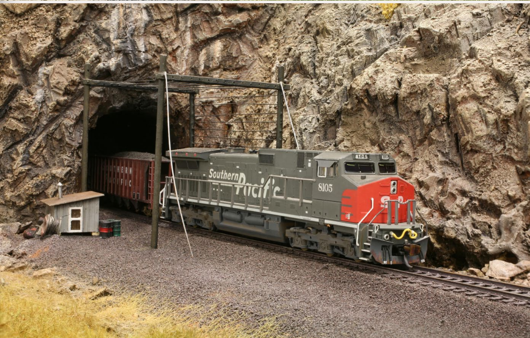
FIGURE 7: This N-scale model scene uses MicroEngineering code 55 track. The finer spikehead detail on this track makes this photograph difficult to tell from an HO model photo. MicroEngineering track has the finest detail of any N-scale track on the market, with Atlas code 55 a close second.
