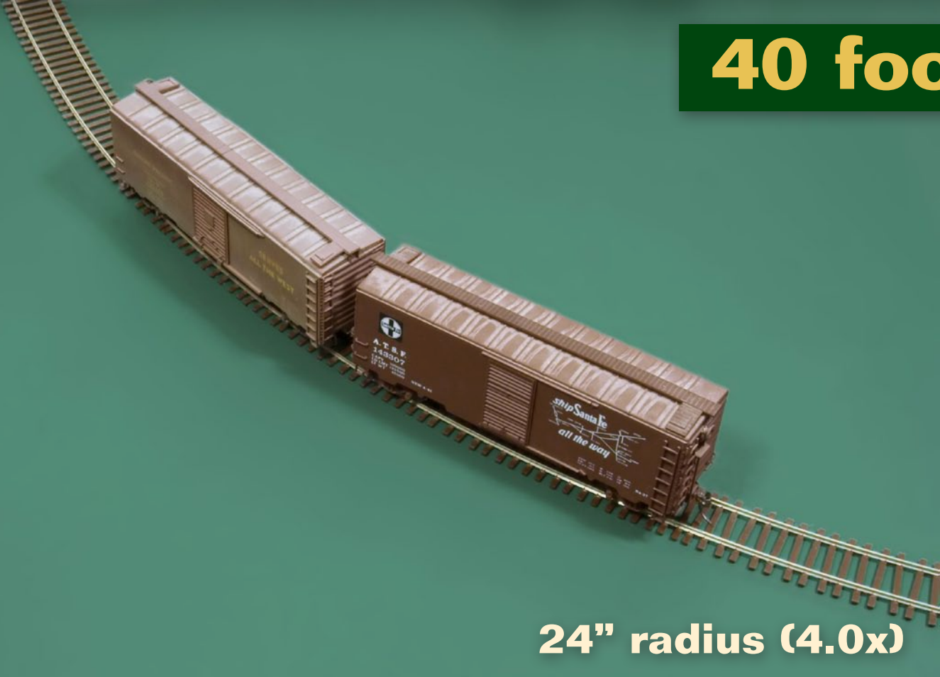
FIGURE 9: Once again as predicted, the cars look realistic at the 4.0x radius curve when viewed from the outside of the curve.
