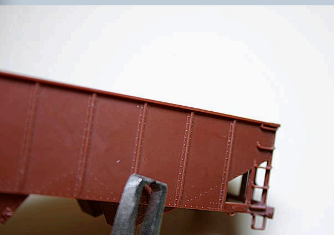
FIGURE 6: Use despruing nippers to carefully cut across the width of each post above taper. Then use the nippers to remove the tapered portion without removing the rivet detail or the flange. Carefully sand the surface smooth.
