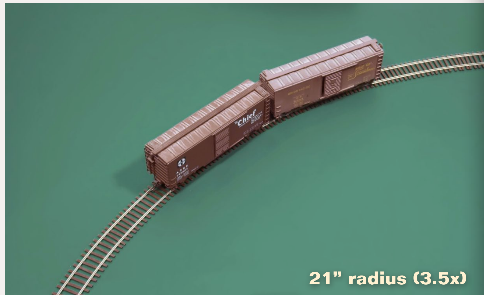
FIGURE 8: As predicted, the cars look reasonably realistic on the 3.5x radius curve when viewed from the inside of the curve.
