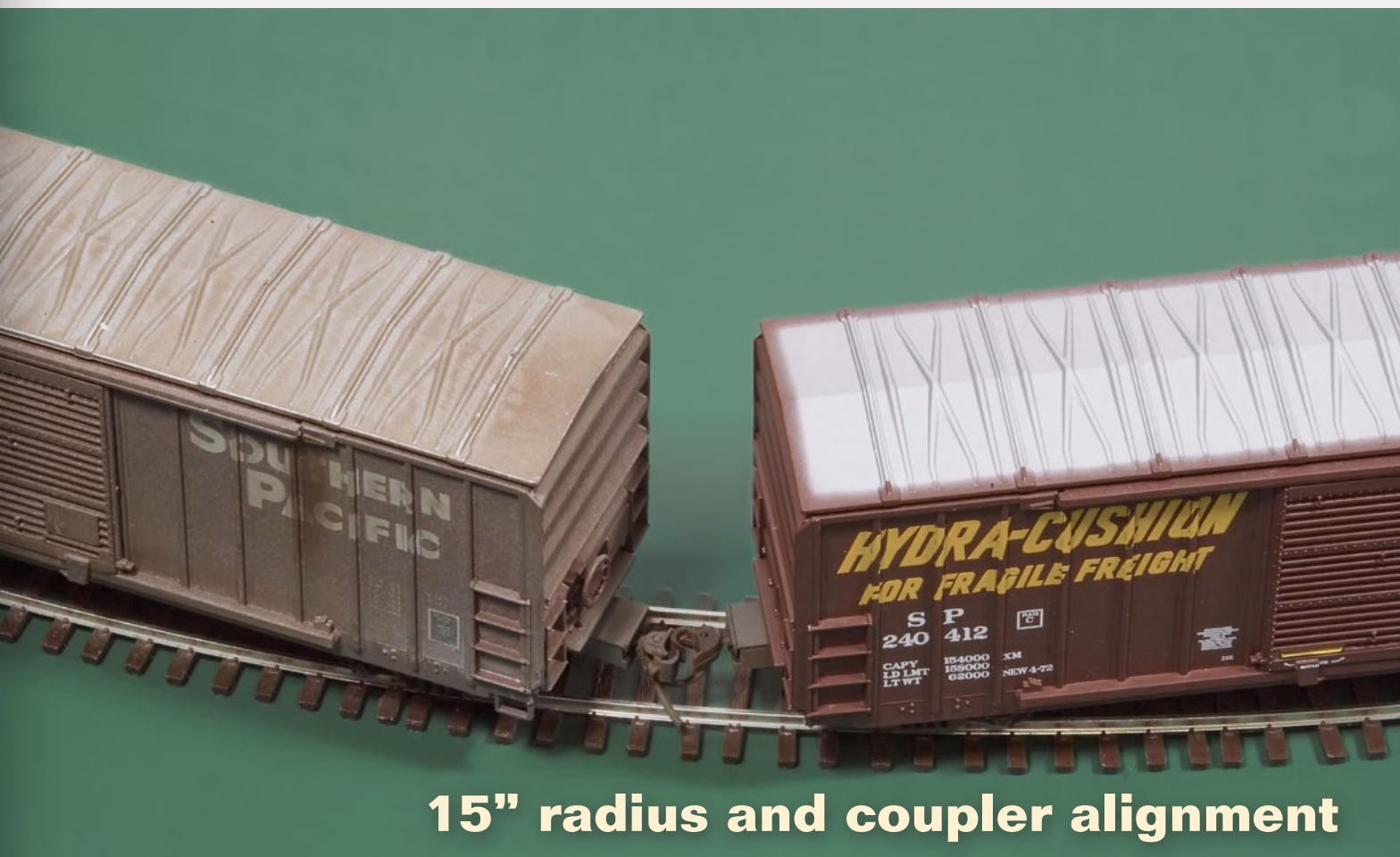
FIGURE 19: On the 2.0x radius curve, the 50 foot car coupler jaws do not align and can only be made to couple with much effort.
