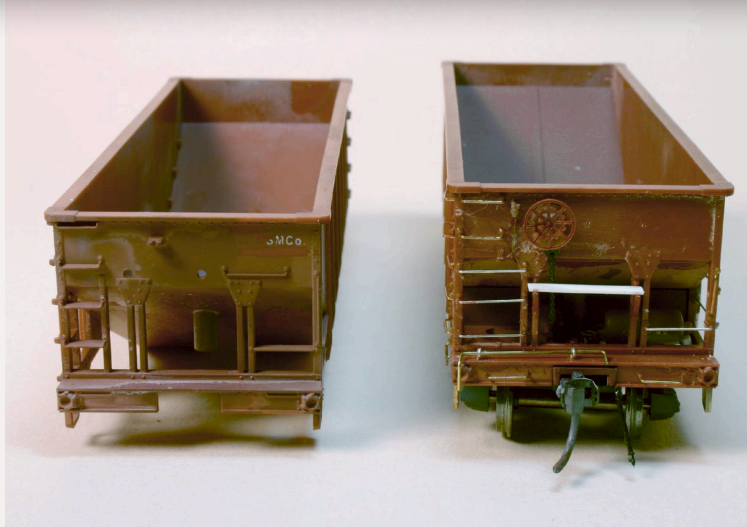
FIGURE 7: The finished model before painting (right) and the stock Bowser end (left). Note the CV car has an additional grab (six, compared with the Bowser models' five) on the right side. There were two long grabs (of different lengths) on the left side. Finally, on the ends, the PRR GLA, and therefore the Bowser model, had shorter grabs, requiring the use of a vertical post between the corner of the car and the vertical support.
