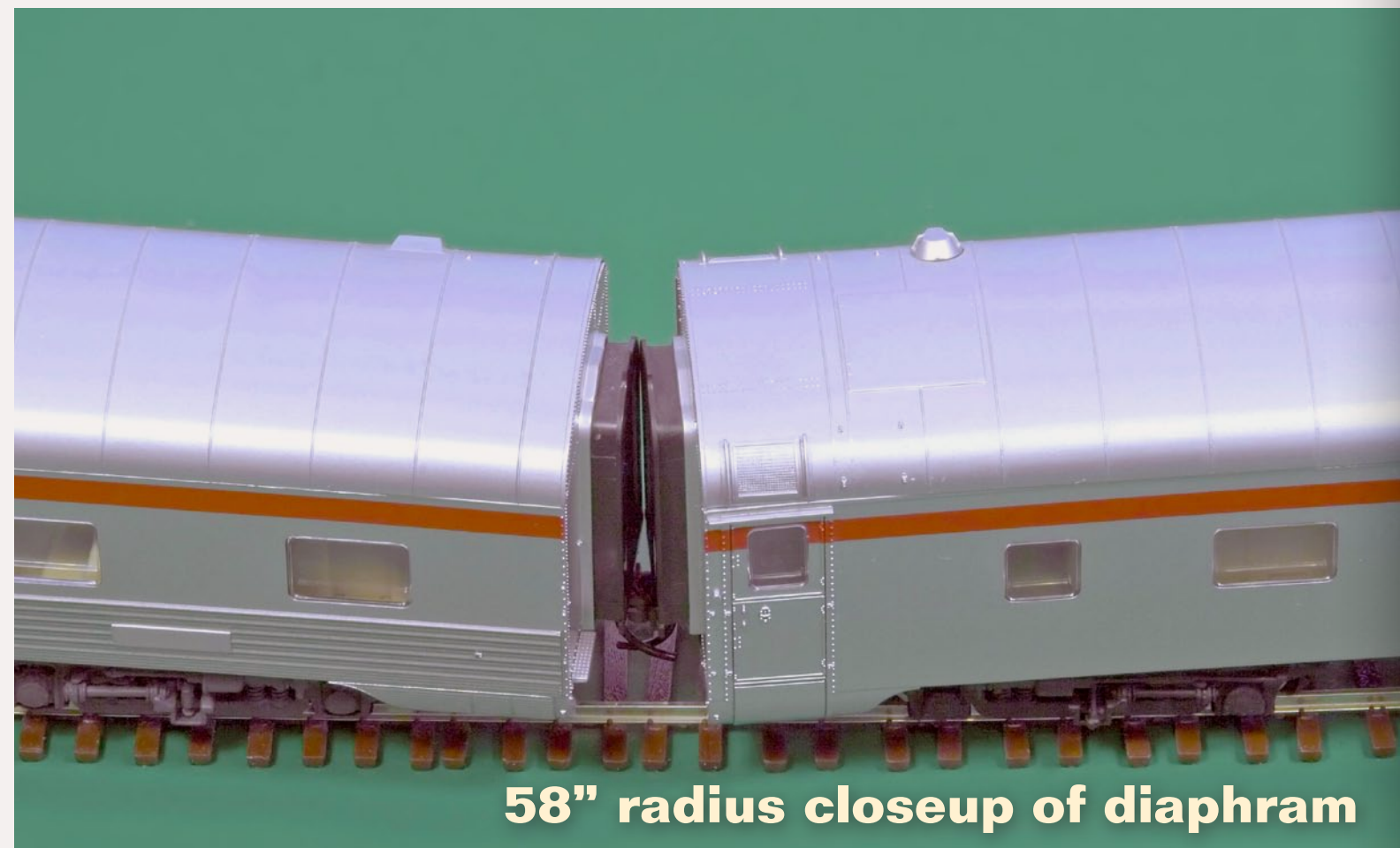
FIGURE 28: The 5.0x curve diaphragm alignment looks far better, but it's still not perfect. Even 58" model curves are much sharper than the prototype.
