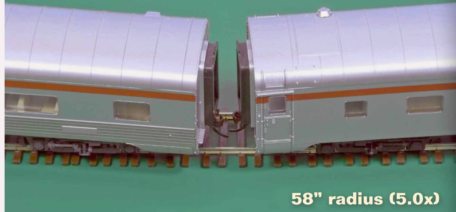
FIGURE 26: Consistent with the 5.0x guidelines, the coupler alignment on a 58" curve essentially matches straight track for these 80 footers.
