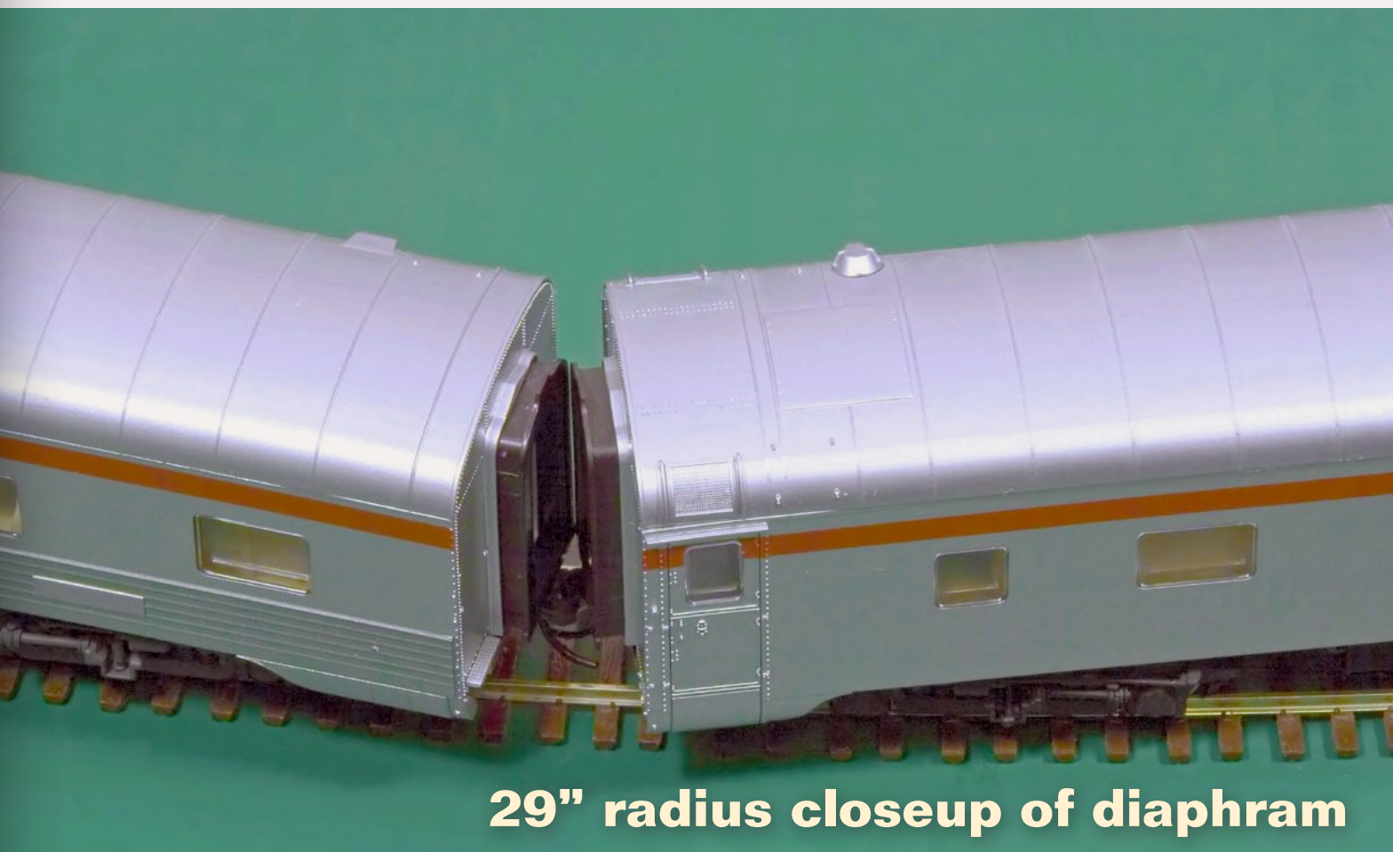
FIGURE 27: With passenger cars, we also need to get the diaphragms to line up. Obviously, it isn't going to happen on the 2.5x curve.
