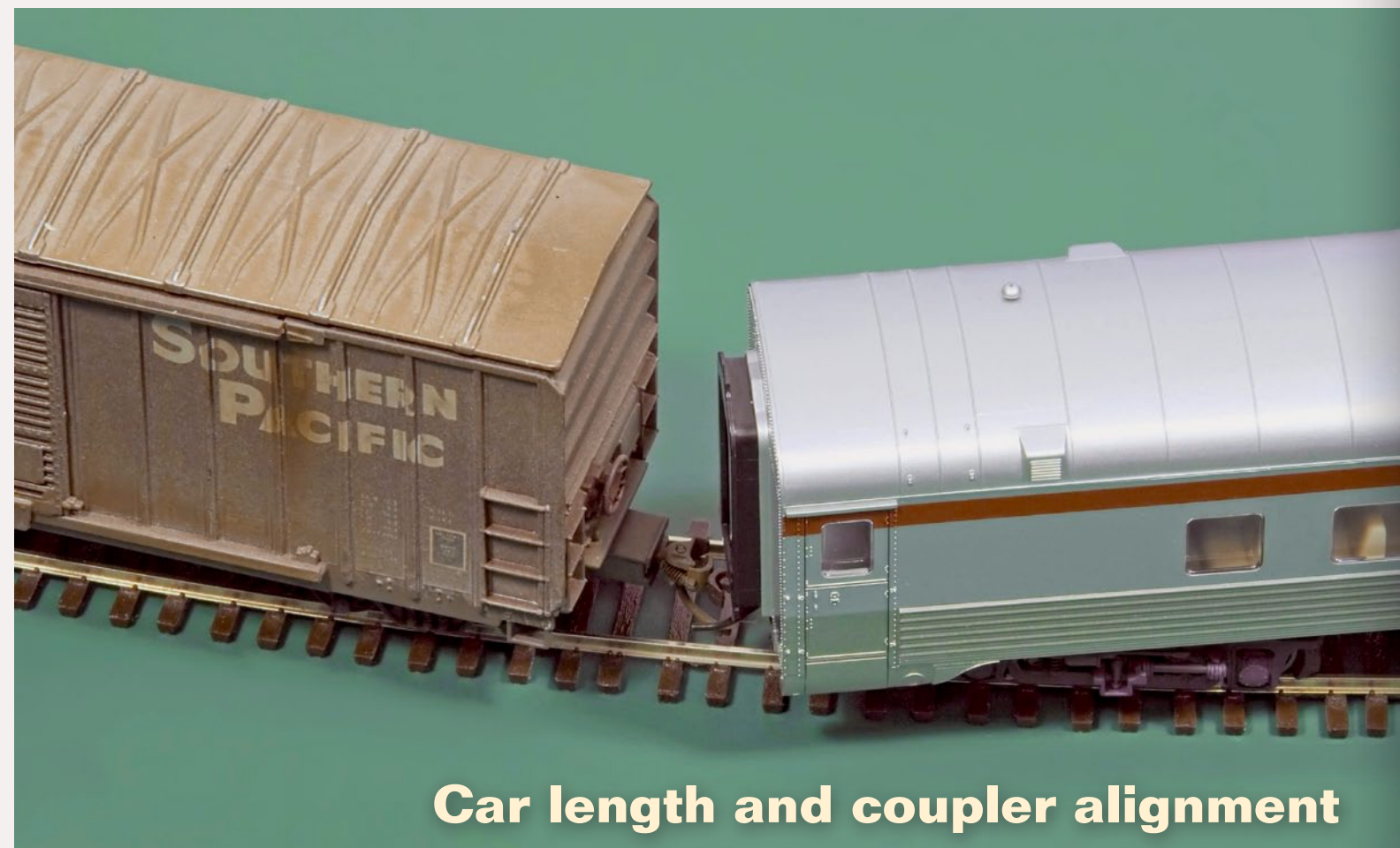
FIGURE 20: The coupler jaws completely miss each other when you mix a 50 foot and an 80 foot car on a 23" radius curve (50 ft = 3.0x, 80 ft = 2.0x).
