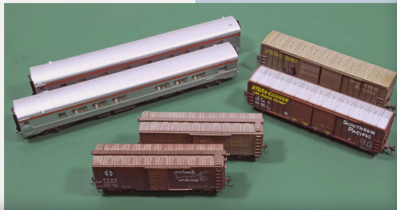
FIGURE 4: We're using these HO cars to do our equipment tests. In the picture going clockwise we have: Walthers 83 foot passenger cars, Athearn 53 foot outside-braced box cars, and Athearn 43 foot box cars. All cars have body-mounted magnetic couplers, although the Walthers passenger cars have special draft gear boxes that allow the couplers to swing up to 50% of the car width.
