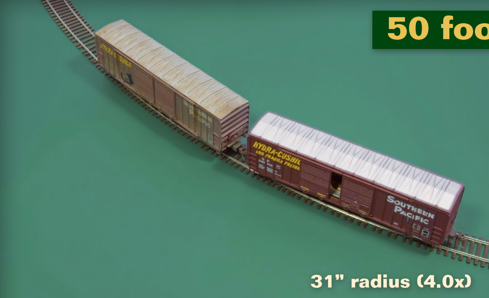
FIGURE 17: As predicted, the 4.0x radius curve looks prototypically realistic when viewed from the outside of the curve.
