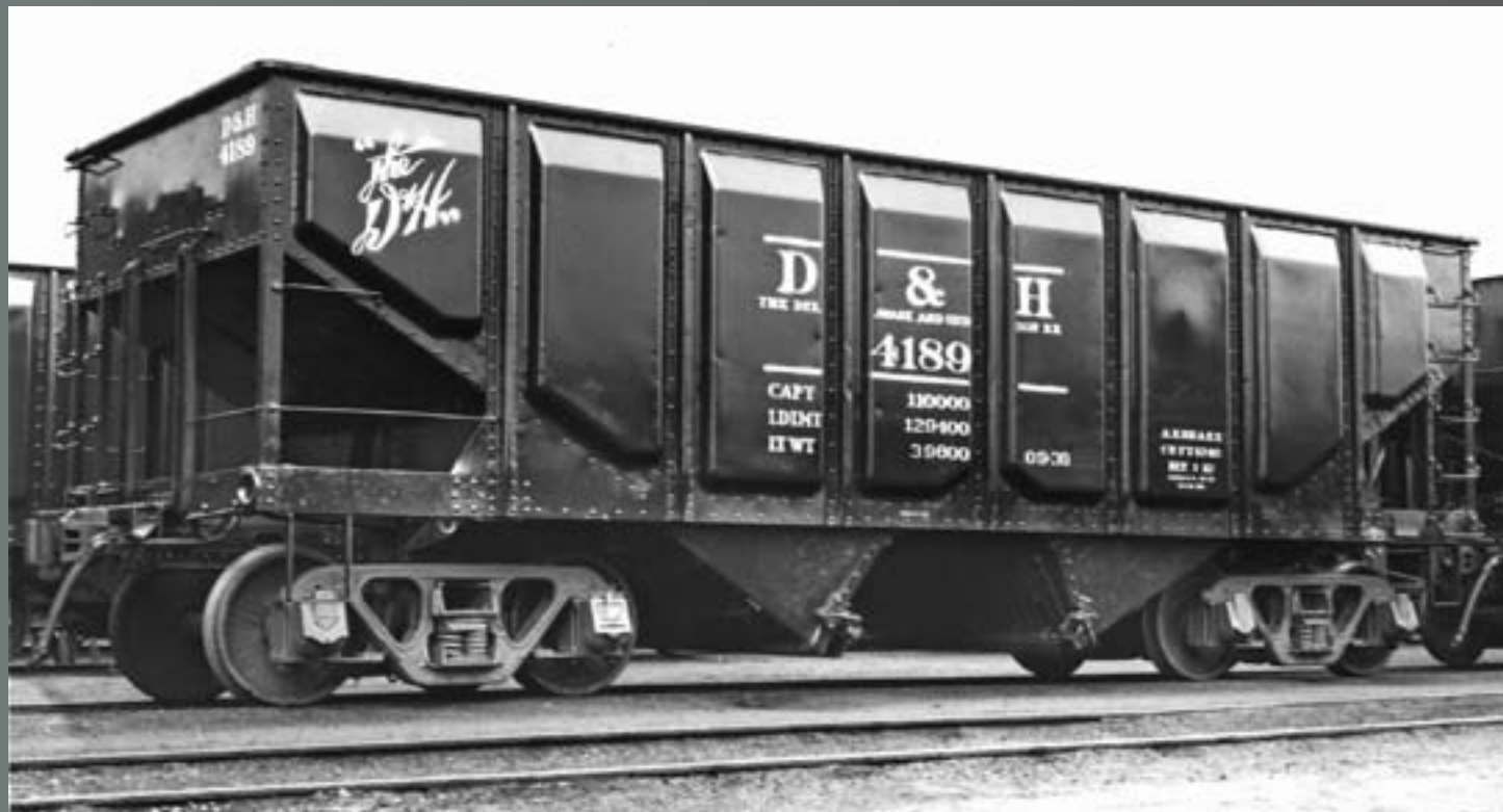
Figure 1: The Delaware & Hudson got a thousand USRA twin hoppers immediately following World War I and numbered them 3201-4200. In the 1930s, more than 300 of them were rebuilt with panel steel sides. Only a month after being rebuilt at the Oneonta, NY shops, D&H 4189 was at Binghamton, NY in September, 1936. Panel sides increased its cubic capacity from 1880 cubic feet to 1940 cubic feet. Note its original USRA Andrews trucks. –Keith Sirman collection
