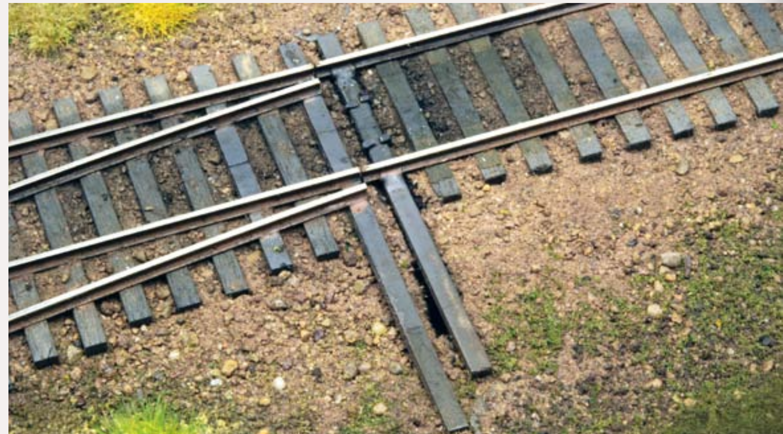
FIGURE 7: Alignment between the bridge rails and the rest of the turnout is critical in a stub switch. The prototype used a cast metal bracket to hold the ends of the rail of the turnout in correct gauge, and cast into this was a stop that would align the moveable rail of the bridge. For our models a different approach is needed, which the author covers in this article.
