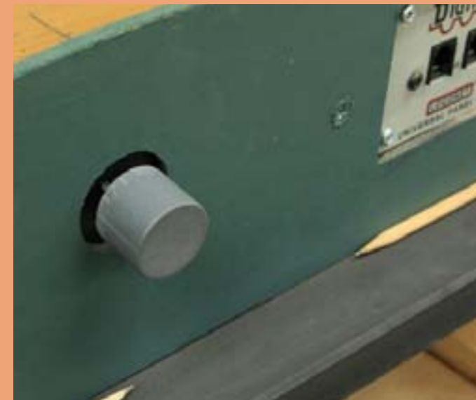
Figure 46: Hole in Fascia for knob.
