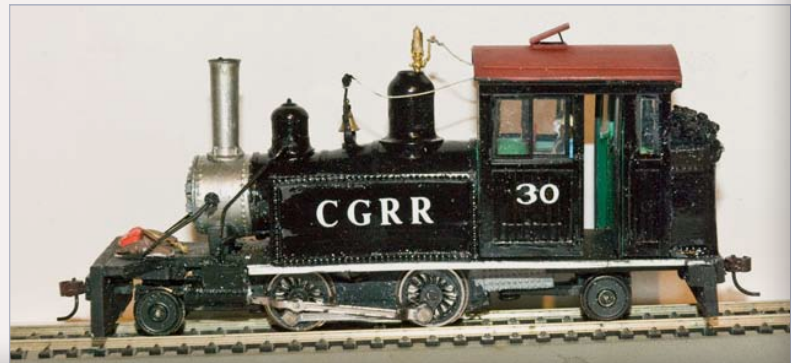
FIGURE 6: This HO On30 loco was converted from a Hornby 2-4-2 with kit and scratchbuilt parts. Photo by Dave Butler.
