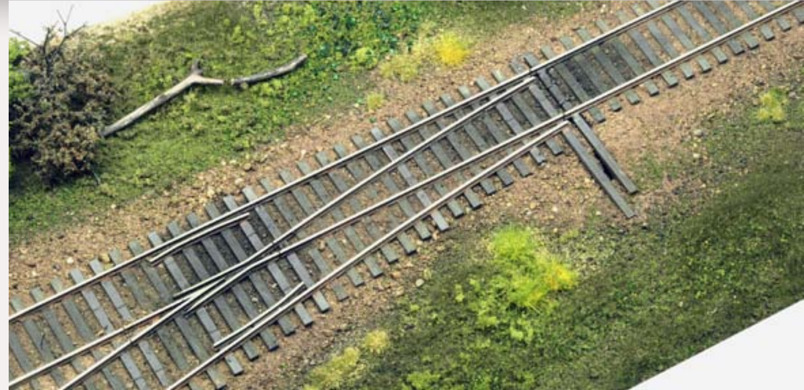
FIGURE 6: The “switch” portion of a stub switch is the same as a modern turnout, missing are the moveable switchpoints, instead a moveable bridge was used.
