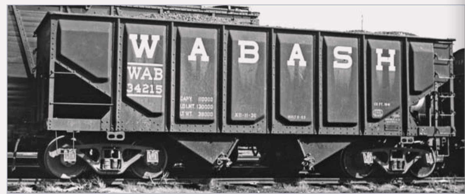
Figure 7: The Wabash received 1000 twin hoppers from the USRA and then purchased additional cars of similar design in the early 1920s. The Wabash was so enthusiastic about replacement panel sides for its twin hopper cars that it not only rebuilt almost all of them as panel side cars in the 1930s but, beginning in 1937, constructed almost 2000 new panel side hoppers in its own Decatur, IL shops. WAB 34215, originally one of 750 31000-31749 series USRA-design cars built in 1923, is shown here at East St. Louis, IL in 1938 after being rebuilt with panel sides at Decatur in November, 1937 and renumbered into the 34000-34499 series. –Joe Collias collection.
