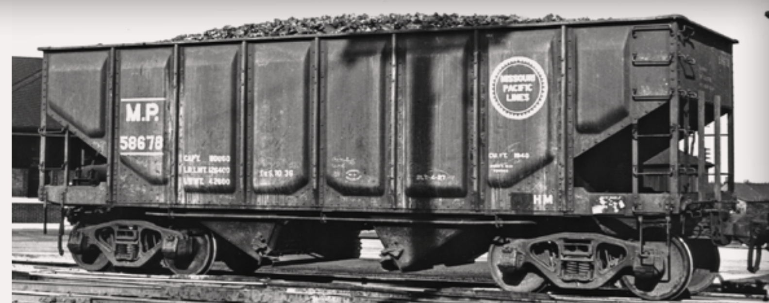
Figure 6: Missouri Pacific MP 58678 was one of 190 cars in the 58000-58749 series built as USRA clones in April, 1927 and rebuilt with panel sides and Commonwealth cast steel hoppers at the DeSoto, MO shops in October, 1936.
