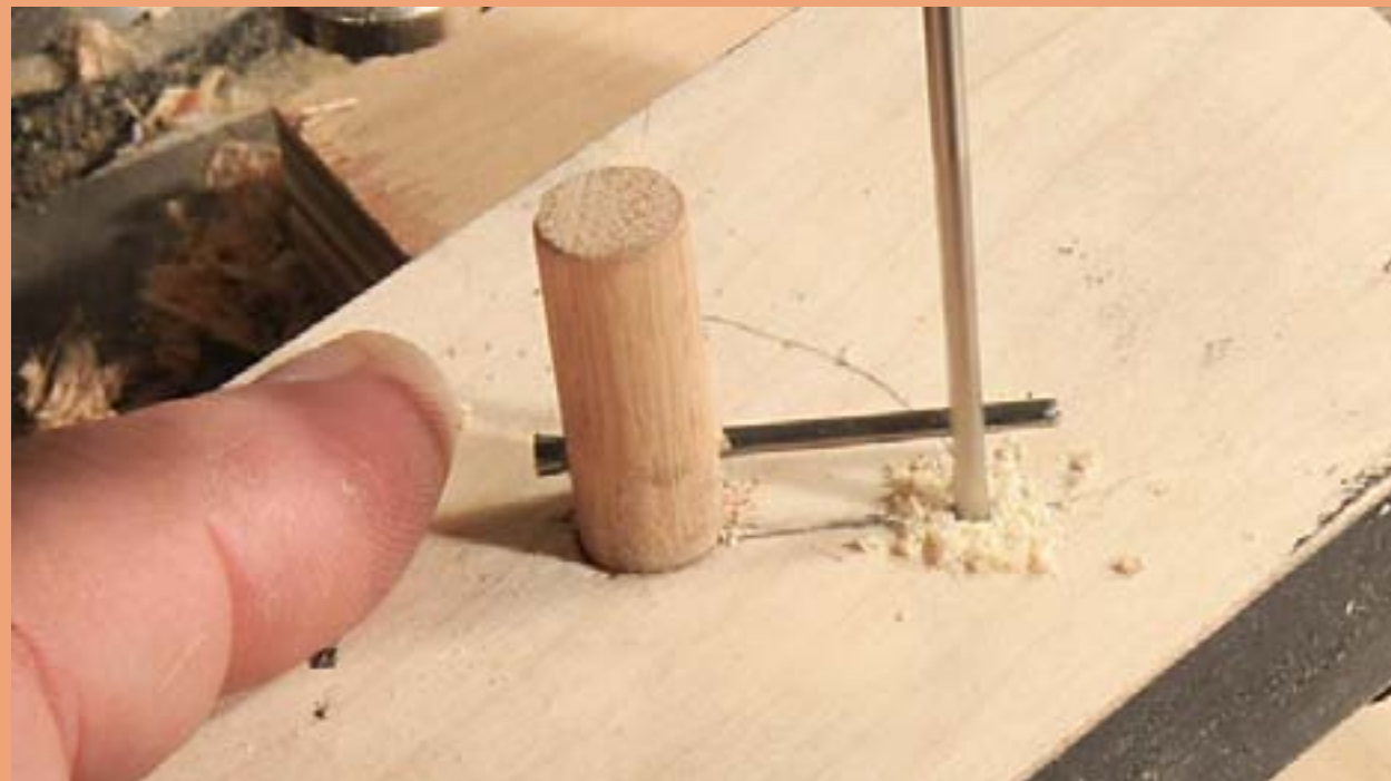
Figure 34: Drilling a travel stop hole.
