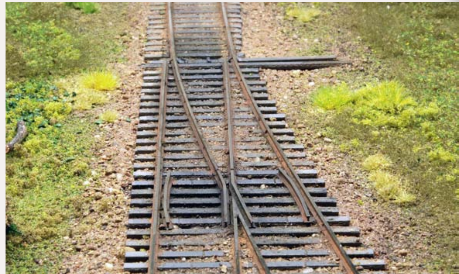
FIGURE 4: To switch routes, the rails of the bridle are slid into position to match the route on the turnout. The curved route has been selected here.
