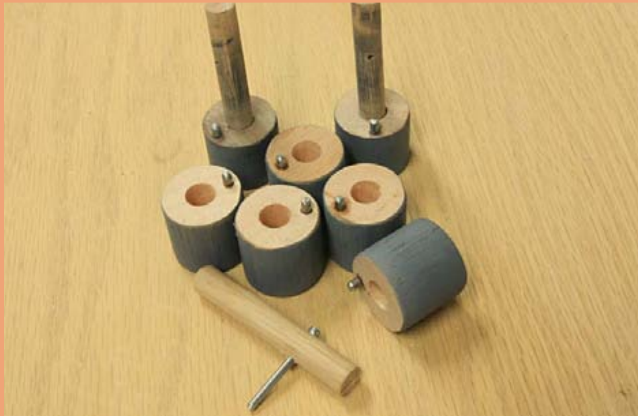
Figure 20: Knobs with locking pins epoxied in place.
