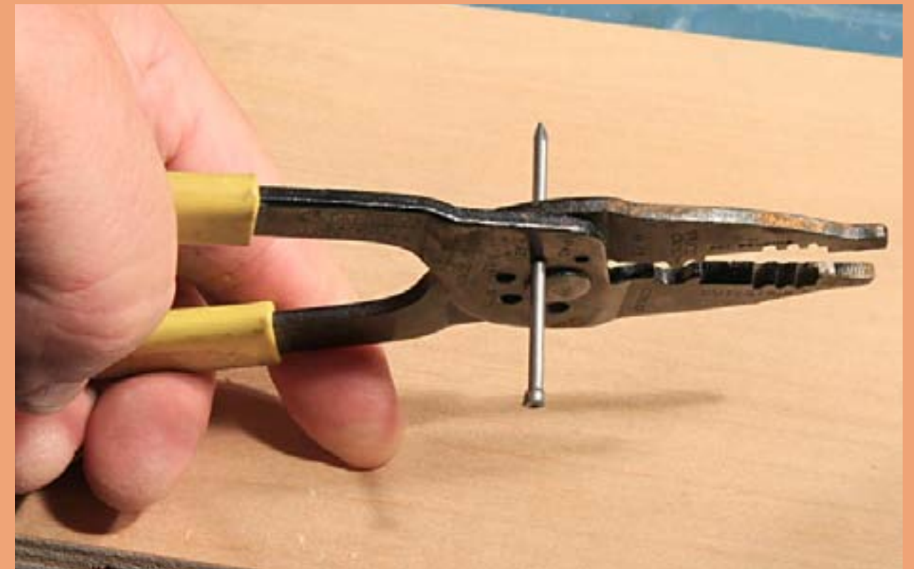
Figure 31: Cutting travel stop pins with wire stripper.
