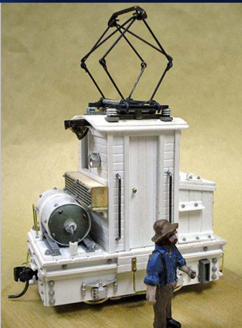
FIGURE 21: No. 1 is nearing the end of its construction. Smaller details: bell, HO headlamps and HO tool box etc. are added. Note the use of brass pins to simulate large rivets and the prolific use of nut-bolt-washer castings. Photo by Junior Yamachi.
