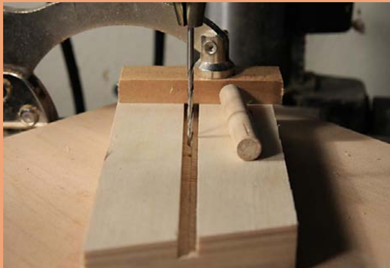
Figure 27: Setting up the travel stop pin hole jig.
