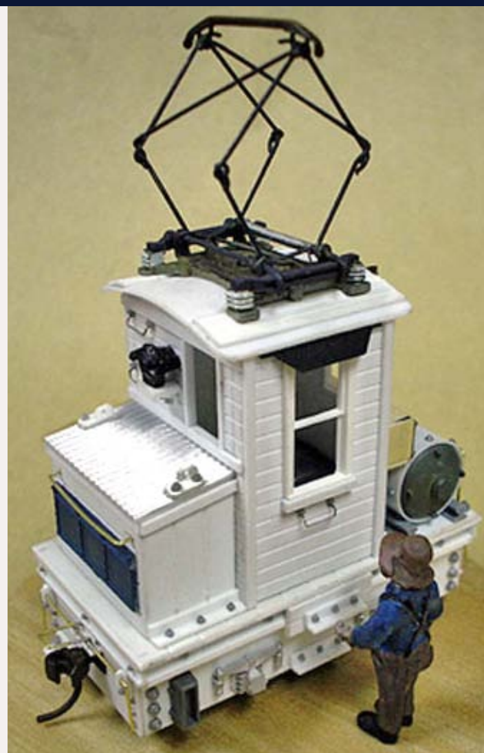
FIGURE 22: The left side and front of No. 1 as it sits ready for painting. The unit was sized to fit the SPUD power unit. Photo by Junior Yamachi.
