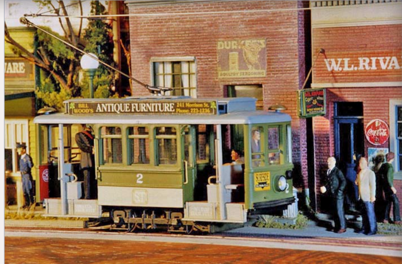
FIGURE 11: Surfeside Traction Co. No. 2 is a kitbashed trolley made from an LGB "Gnomy" toy with a SPUD power truck and a shortened Brill side frame. The background is a 5 inch by 24 inch Surfeside City diorama. Photo by Junior Yamachi.
