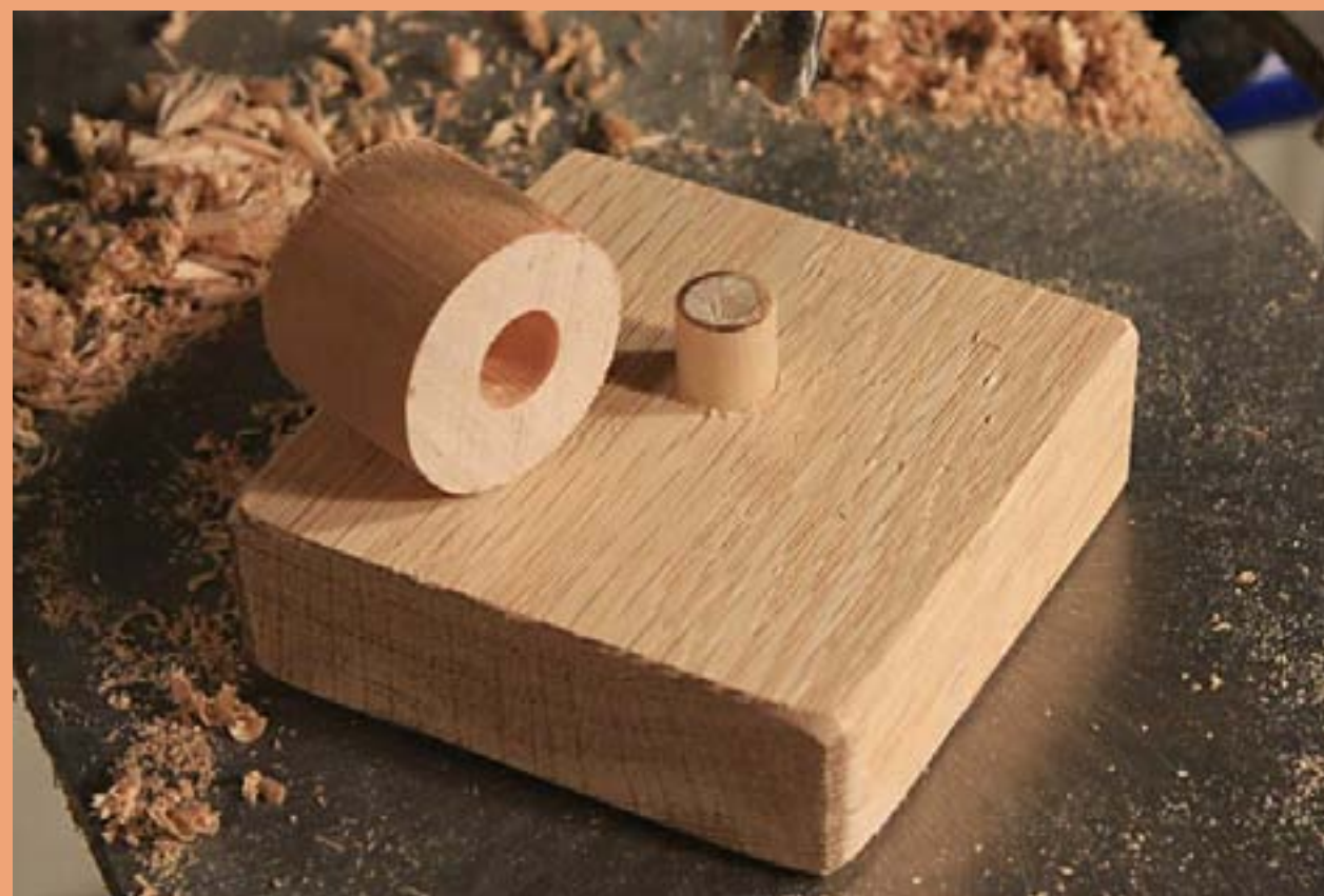
Figure 12: Locking pin jig with shaft installed.
