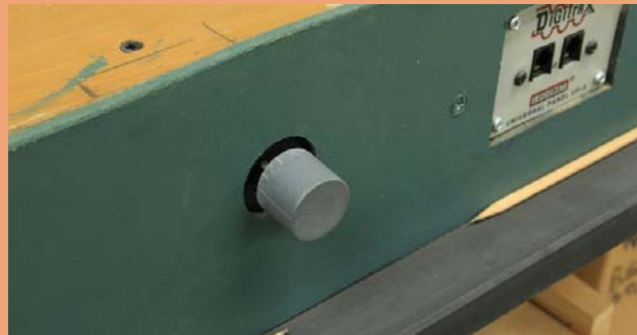
Figure 23: Turnout control installed behind fascia.
