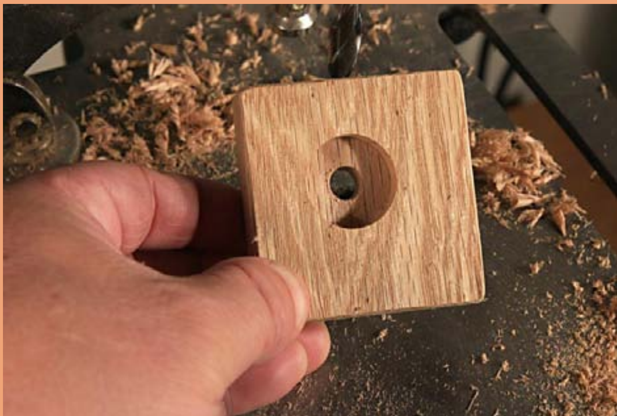
Figure 7: Completed shaft hole jig.
