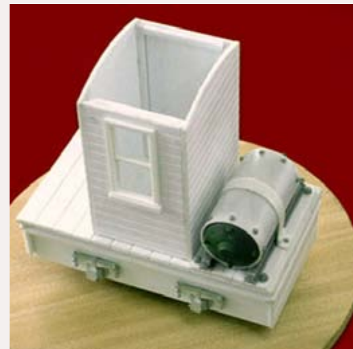
FIGURE 19: No. 1 under construction has a window from an O scale structure, Evergreen V-groove siding, plastic angles and channels and an N scale tank container. Note the styrene axle bearings from a 1:80 scale diesel. Photo by Junior Yamachi.
