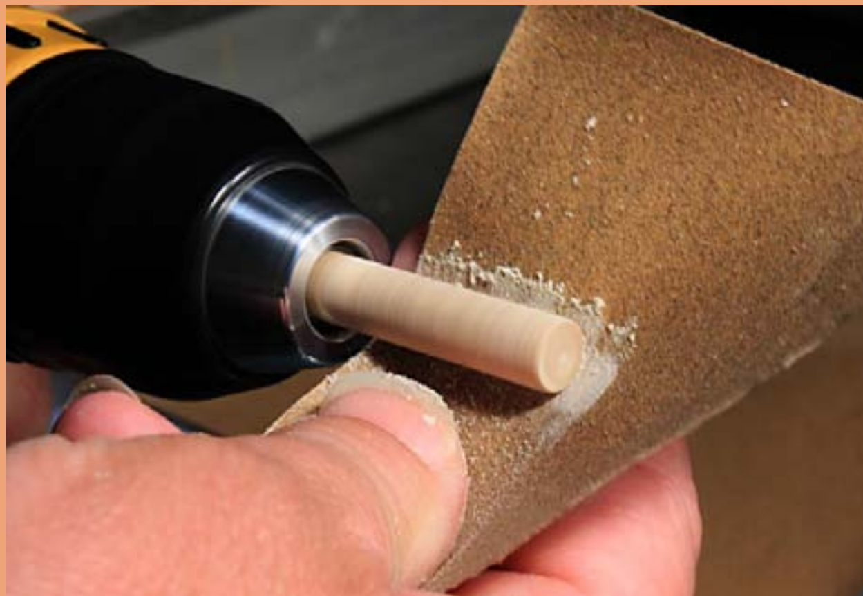
Figure 25: Sanding a shaft using a drill motor.
