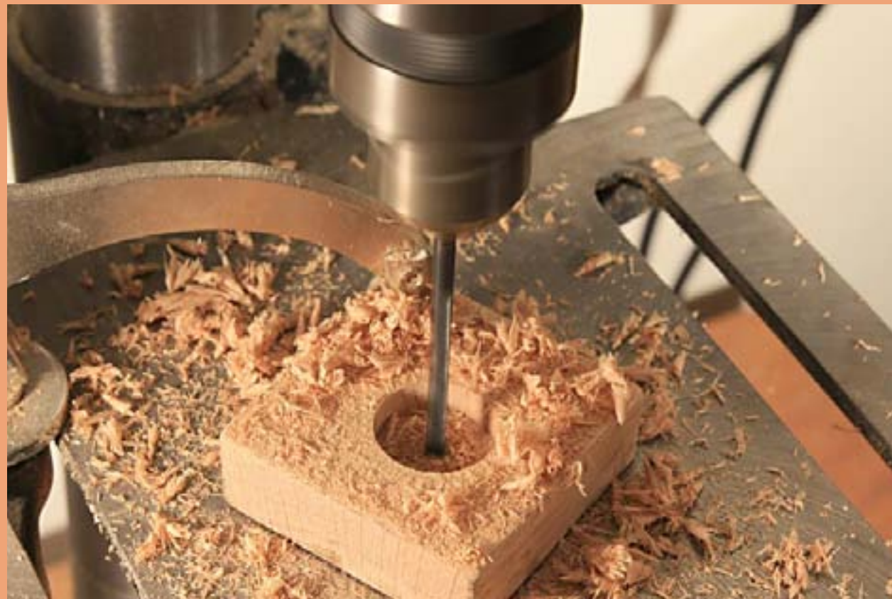
Figure 6: Pilot hole for the shaft.
