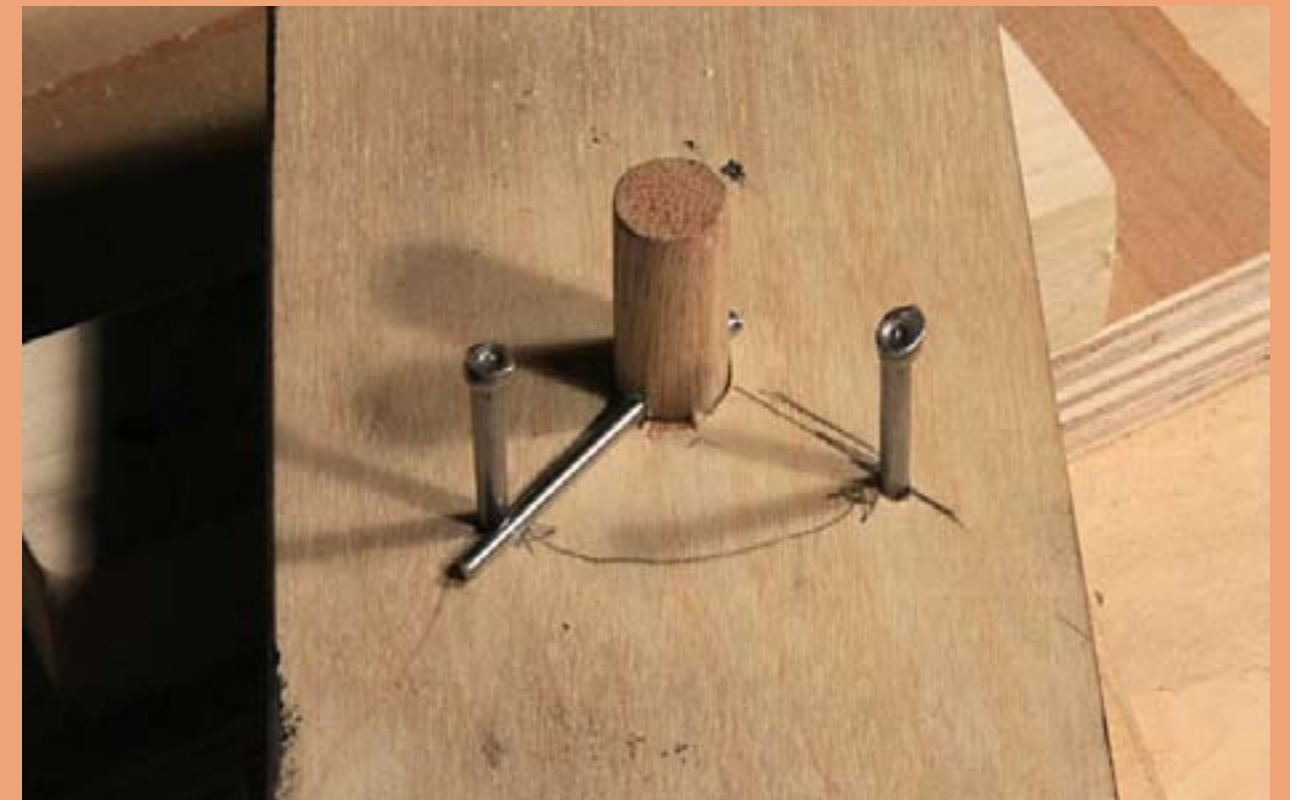
Figure 35: The travel stops installed in the holes.
