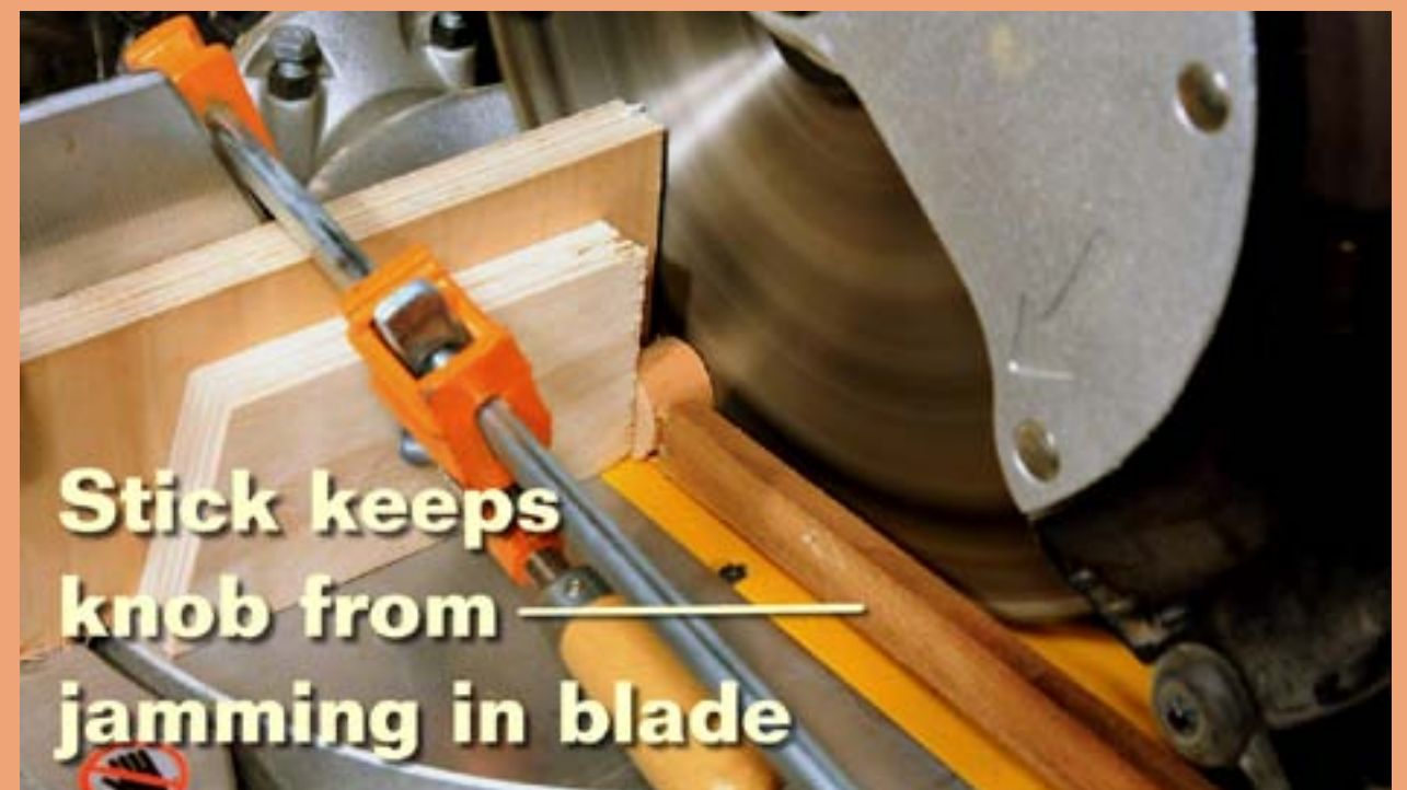
Figure 9: Cutting a knob from a 1" dowel.
