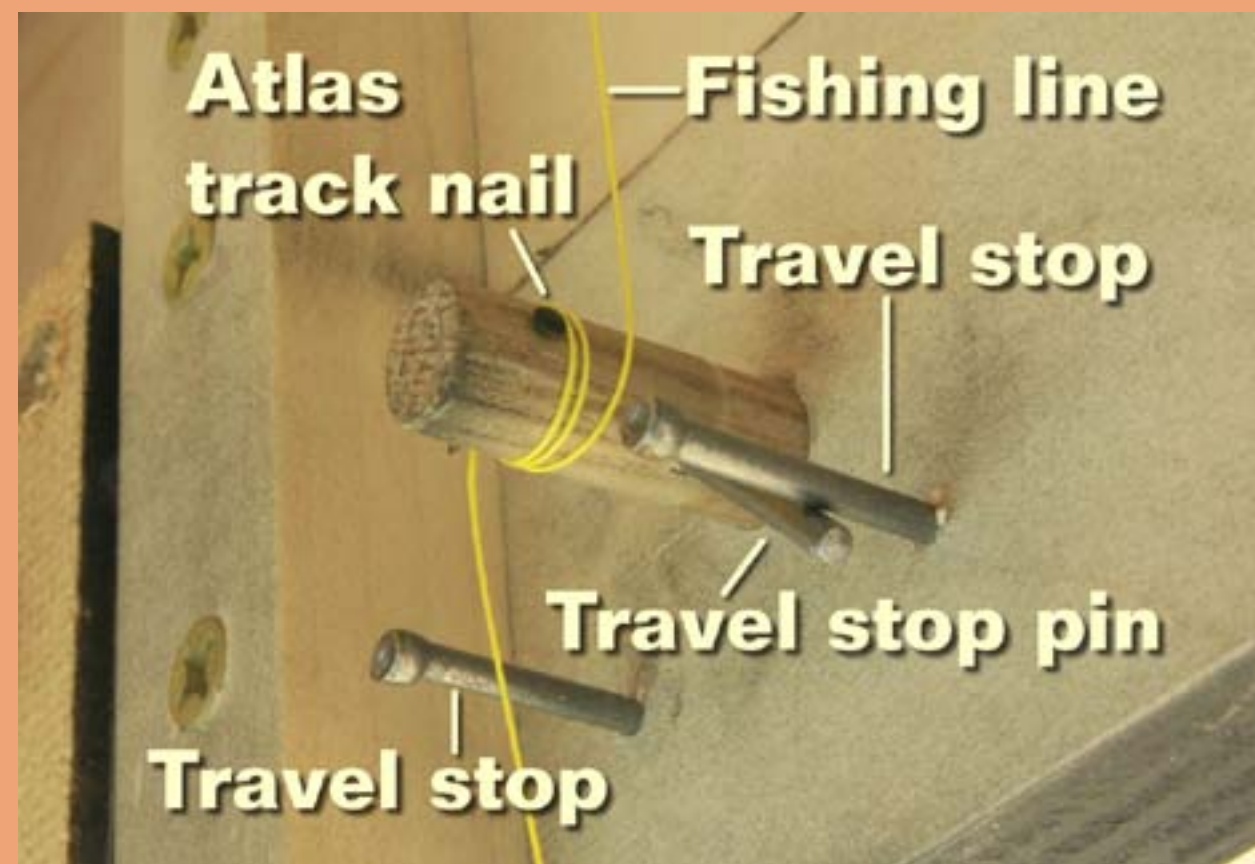
Figure 42: Line wrapped around the shaft.
