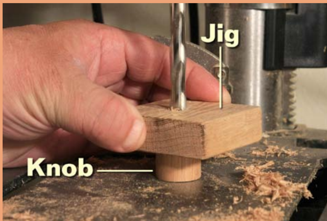
Figure 10: Drilling a shaft hole in a knob using jig.
