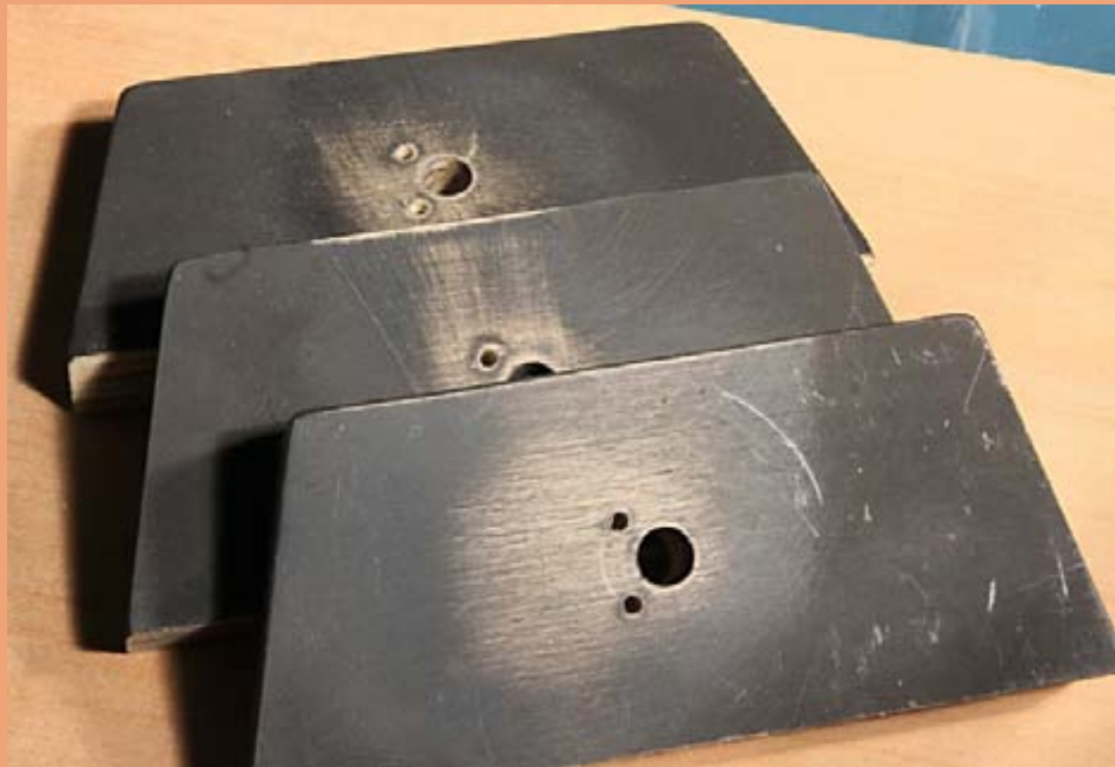
Figure 22: Panels with shaft and locking pin holes.
