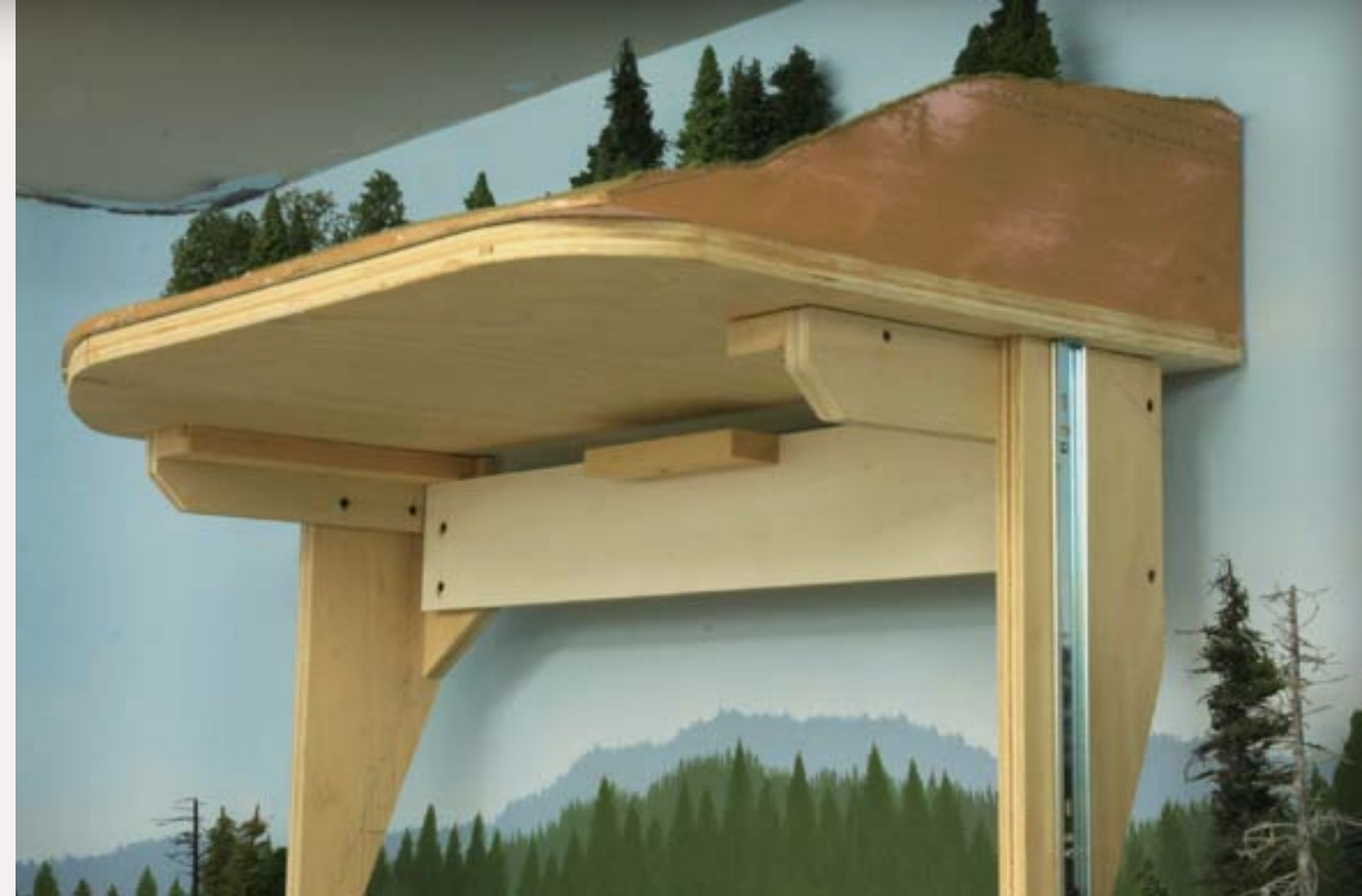
FIGURE 2: The access hatch in its raised position shows the importance of knowing your vertical clearance. There are only a couple of inches between the tree tops and the ceiling.
