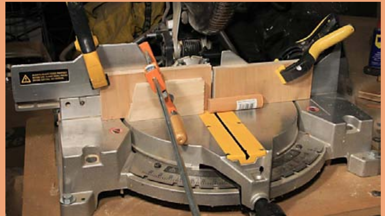
Figure 8: Setting up the chop saw to cut knobs.
