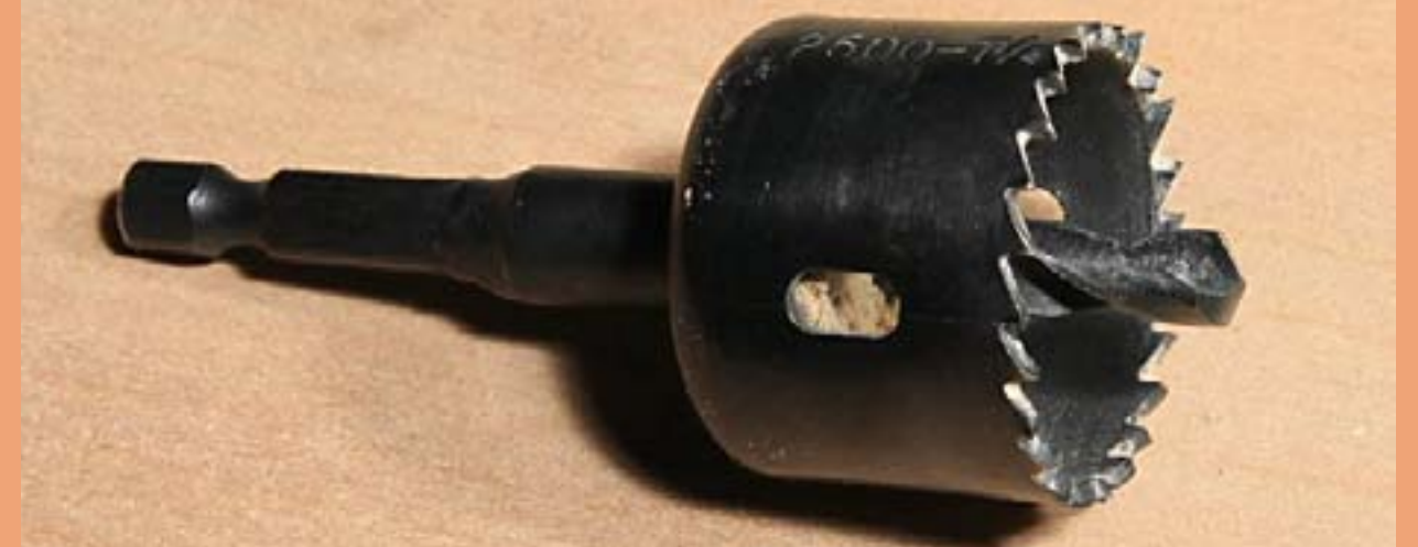
Figure 45: Hole cutter used when cutting knob-holes in fascia for behind the fascia mounting.
