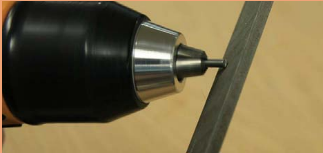
Figure 19: Deburring a locking pin.
