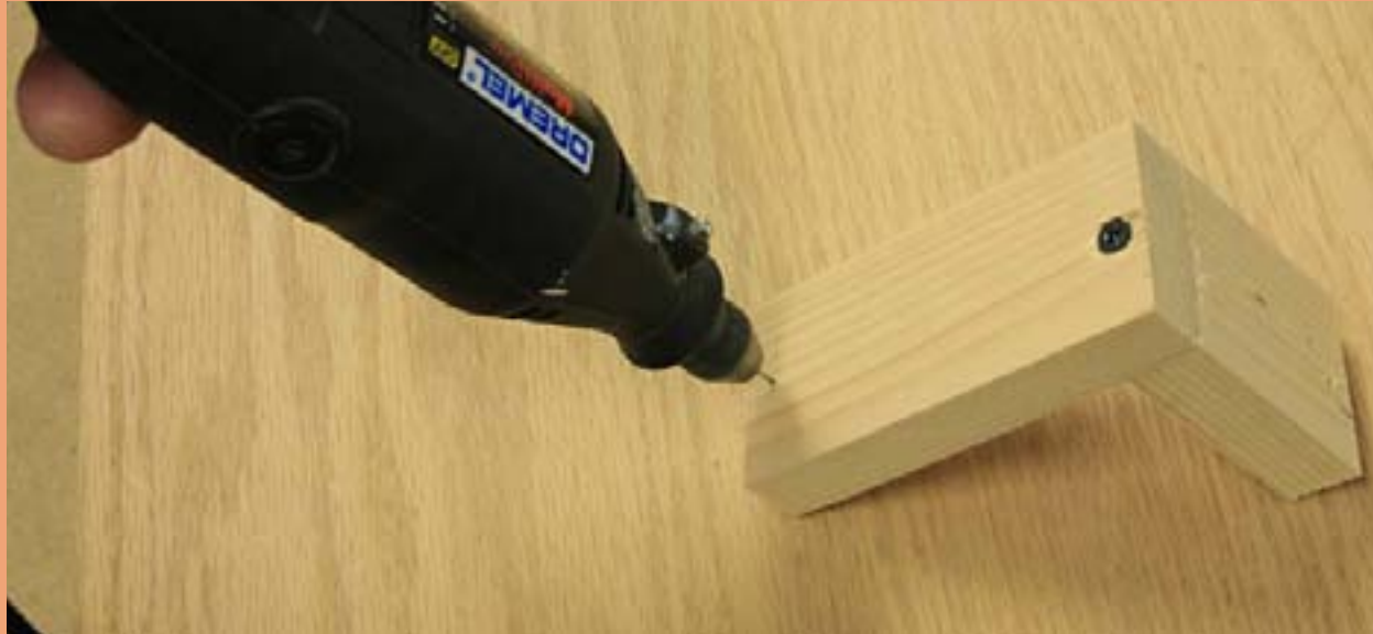
Figure 37: Drilling actuator wire hole in mounting bracket.
