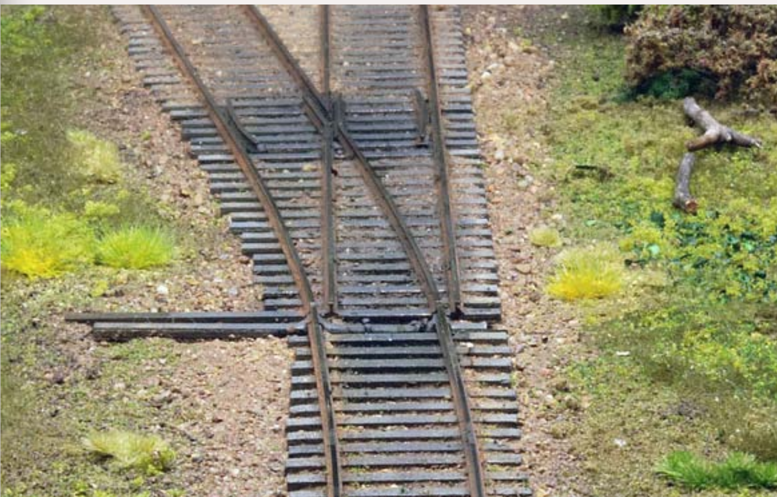
FIGURE 5: The bridge portion of a stub switch acts as a spiral easement into the curve of the diverging route by providing a larger radius at the start of the arc, and spirally getting sharper as it enters the frog of the switch.
