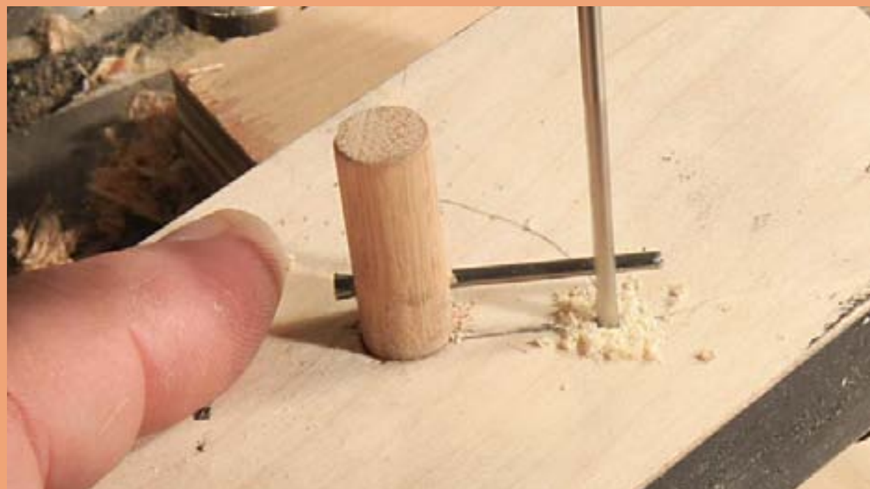
Figure 34: Drilling a travel stop hole.
