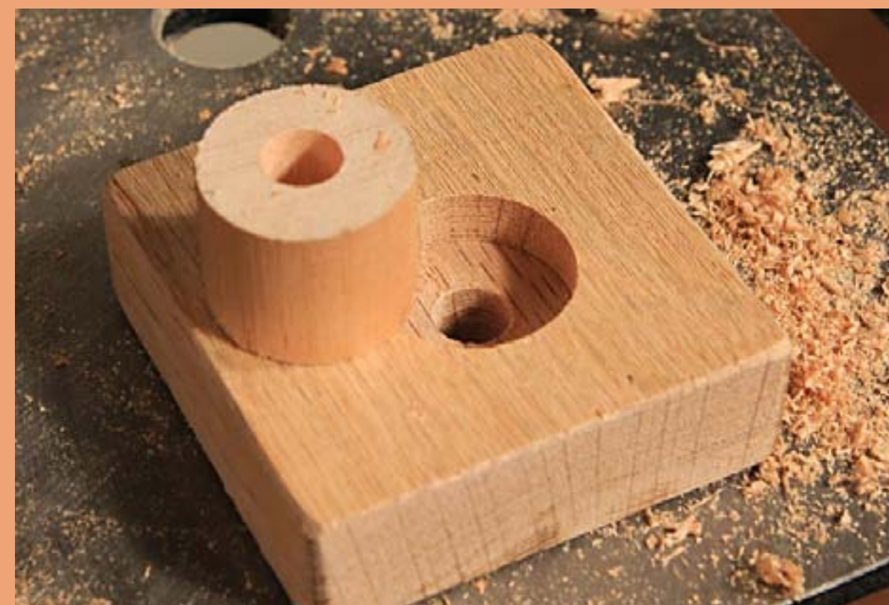
Figure 11: Knob with shaft hole and jig.
