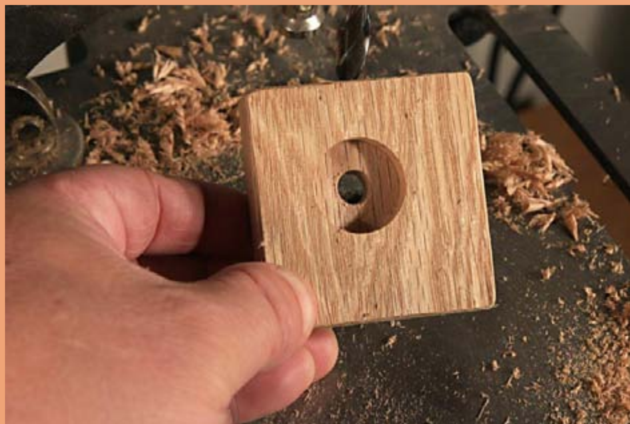
Figure 7: Completed shaft hole jig.
