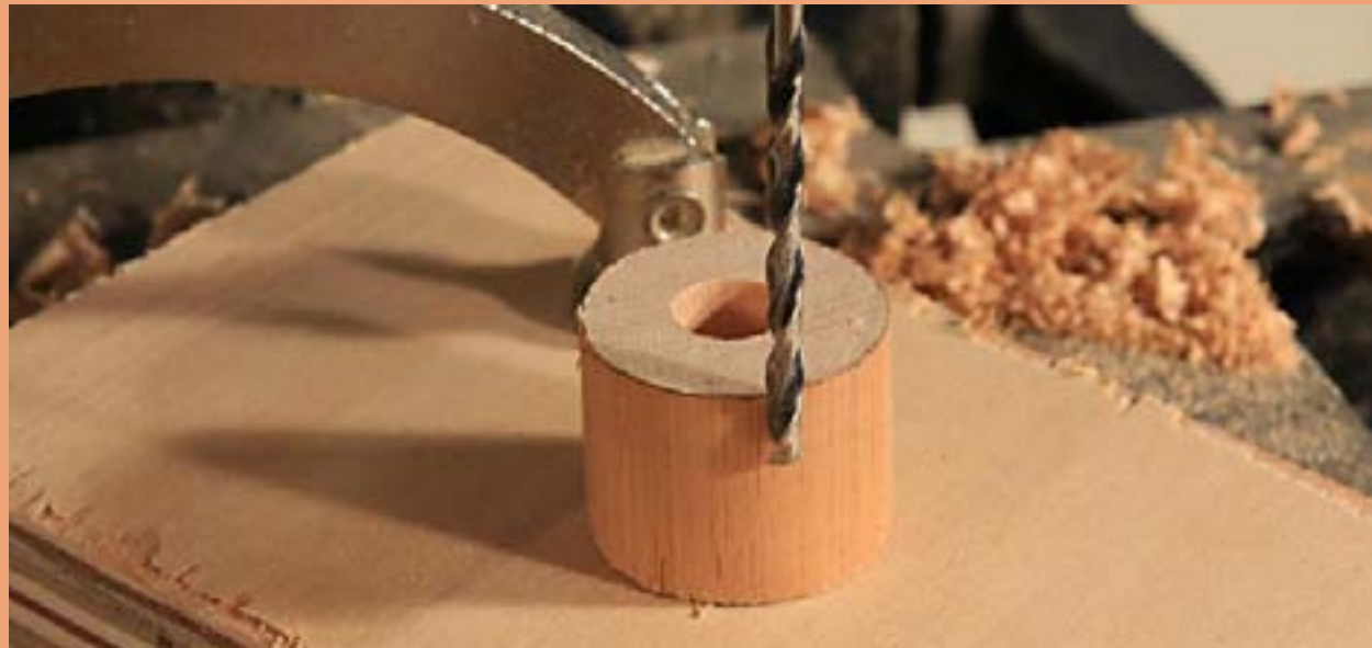
Figure 15: Setting locking pin hole depth.
