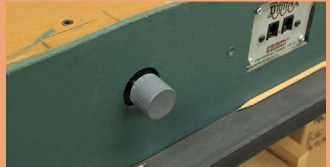
Figure 23: Turnout control installed behind fascia.
