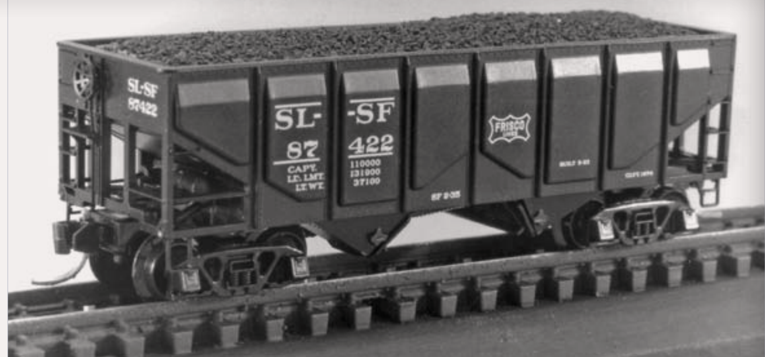
Figure 9: A Micro-Trains N scale model with simulated coal load painted and lettered to represent a Frisco USRA-design gondola in the 86000-89499 series as it appeared after rebuilding with panel steel sides. —Richard Hendrickson
