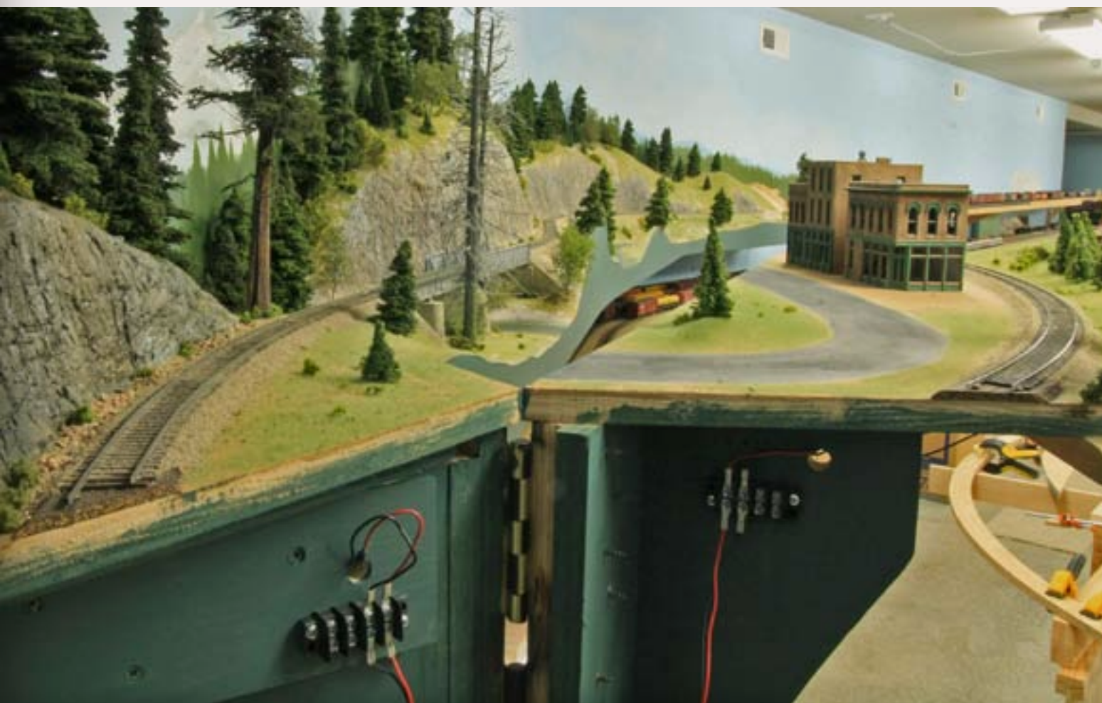
FIGURE 16: I used stranded wire between the barrier strips to power the bridge tracks. This is more reliable electrically than some sort of 'contacts'. Note the color coded wires.
