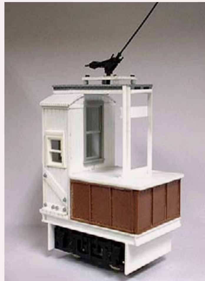
FIGURE 27: This early version with a trolley pole was examined and then the idea was discarded in favor of using a pantograph. Photo by Junior Yamachi.
