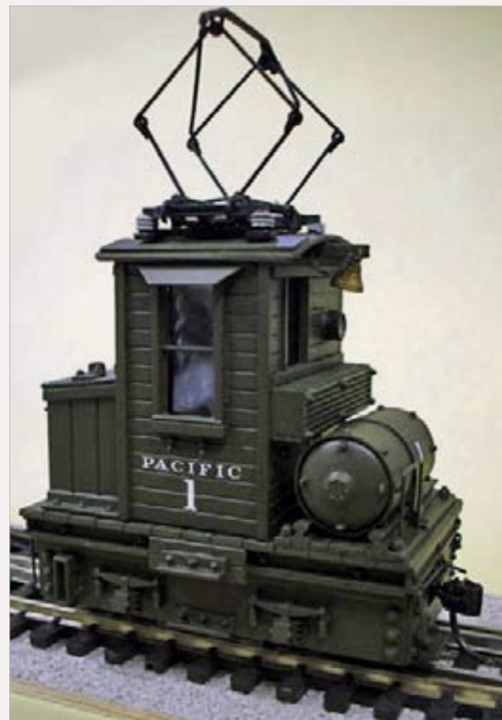
FIGURE 18: No. 1 electric motor began the mining industry expansion. Shown from the left side, the details are quite cleverly done. The pantograph is a Rivarossi part and the compressed air tank is an N scale container. No matter where you look, on this small model, there is detail for the eye to dwell upon. Photo by Junior Yamachi.
