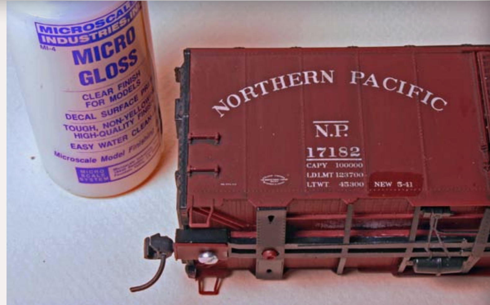
FIGURE 3: Microscale Micro-Gloss applied with a small paintbrush leaves a good surface for decals. In this case the "New" date is too old for the author's era so he'll replace it with a decal "patch" and new reweigh date.
