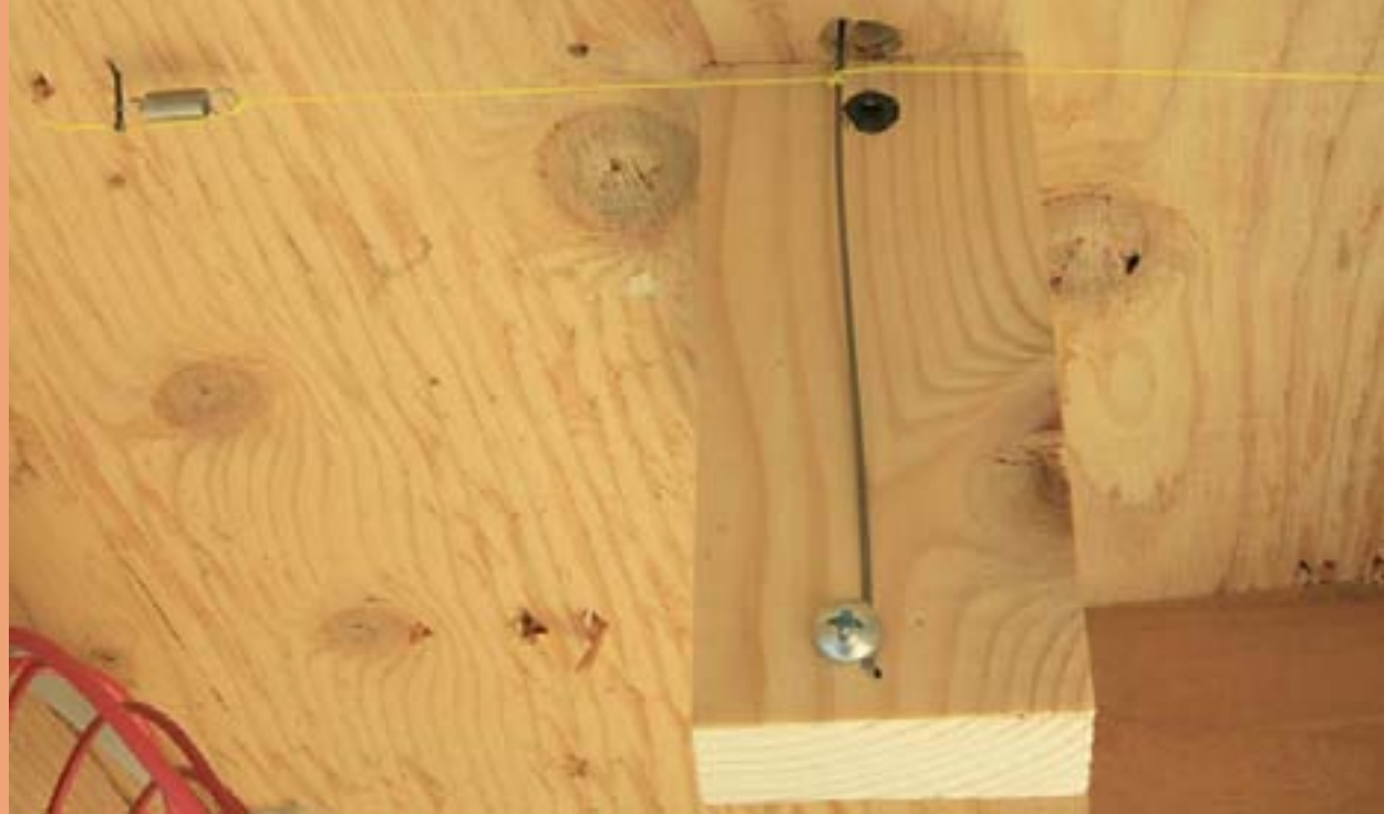
Figure 43: Switch points pulled by knob and shaft.
