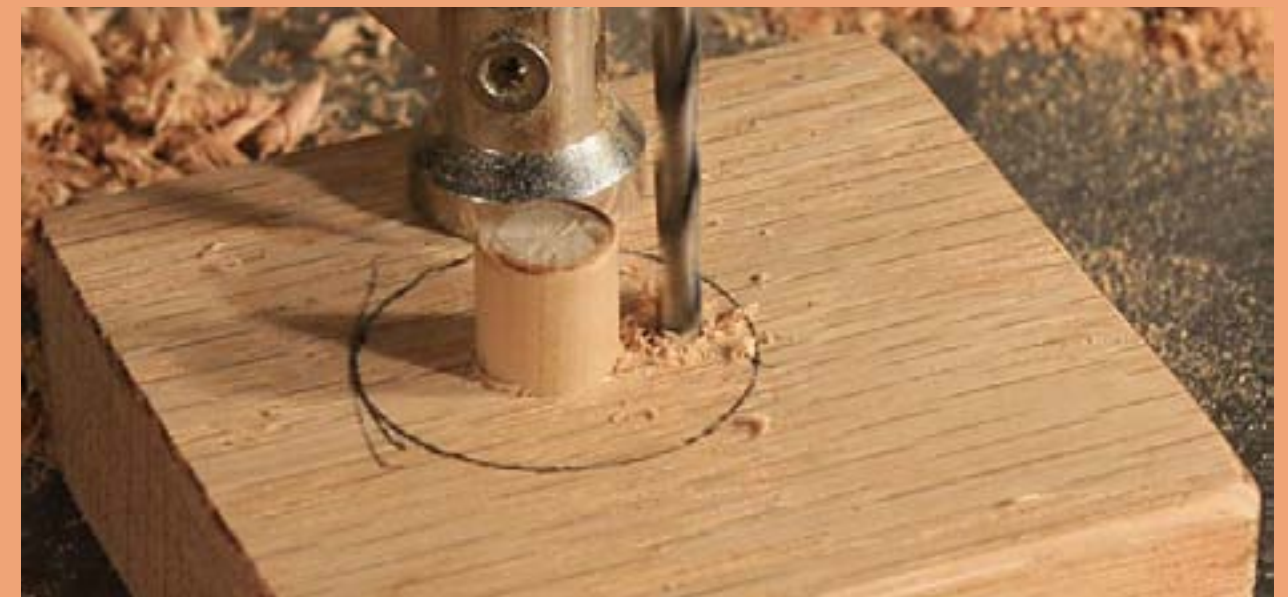
Figure 14: Drilling the locking pin guide hole (halfway between the outline and the shaft).
