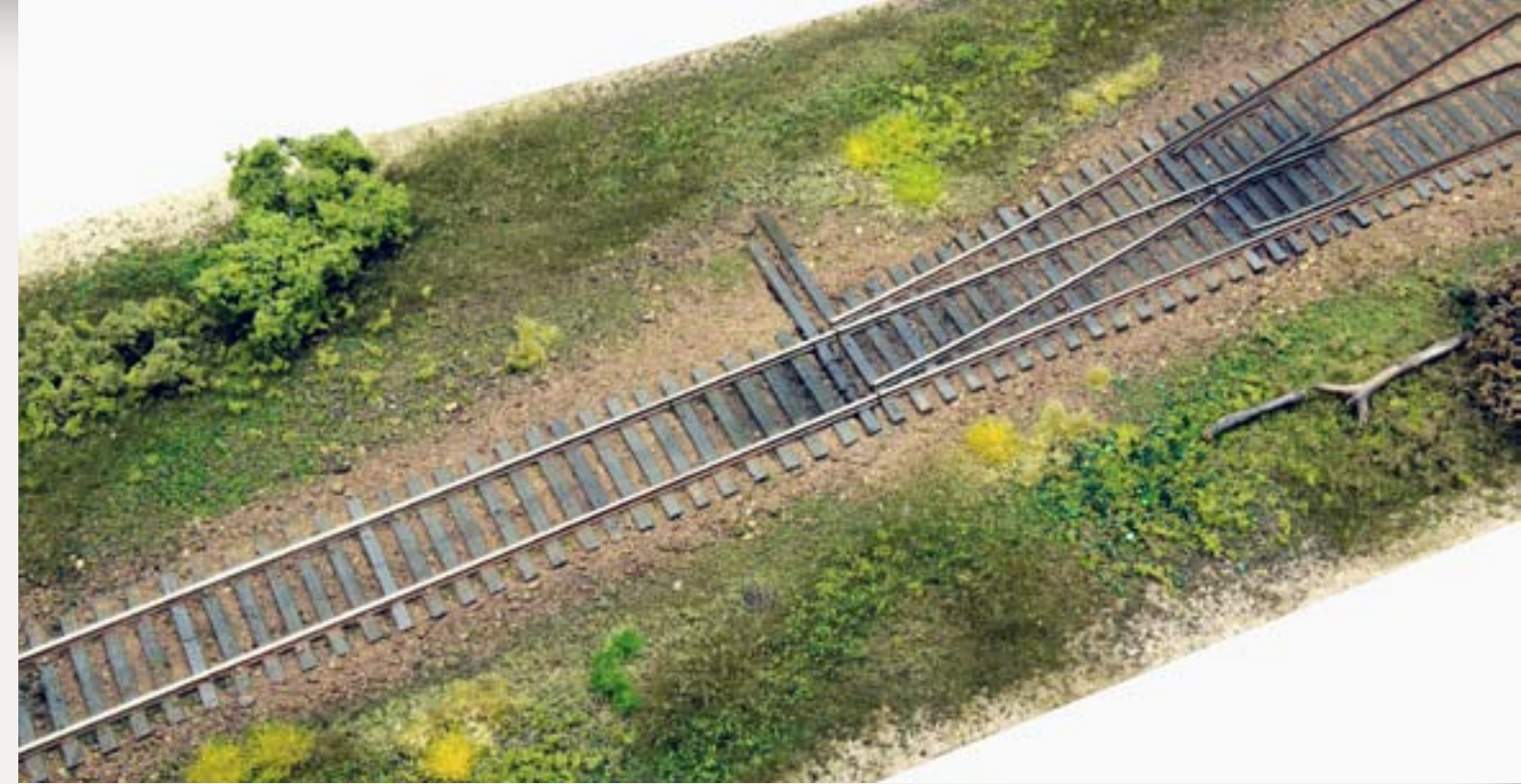
FIGURE 3: Instead of moveable switchpoints, stub switches have a “bridle” section leading into the switch. This section of track is literally bent into position to line up the rails with the switch. Shown above, the straight route is selected.
