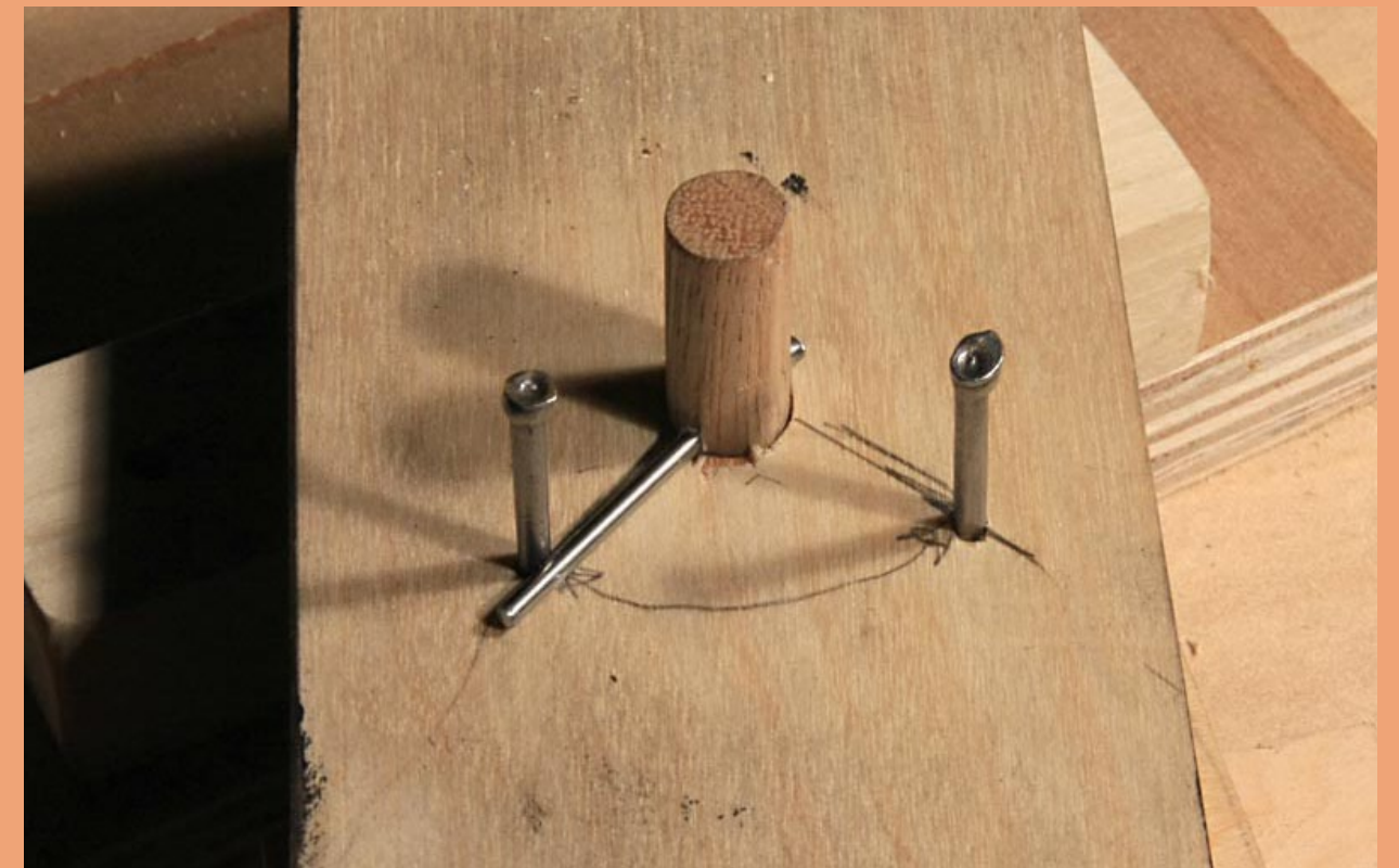
Figure 35: The travel stops installed in the holes.
