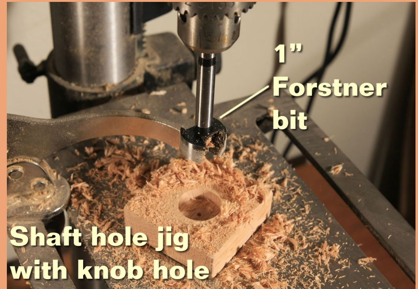
Figure 5: Shaft Hole Jig - drilling the hole to hold the knob.
