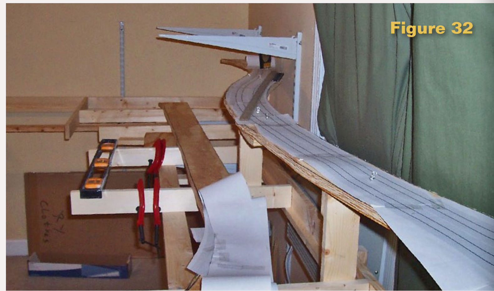
Figures 31 and 32: Sub-roadbed cuts with the templates in position for marking the centerline.
