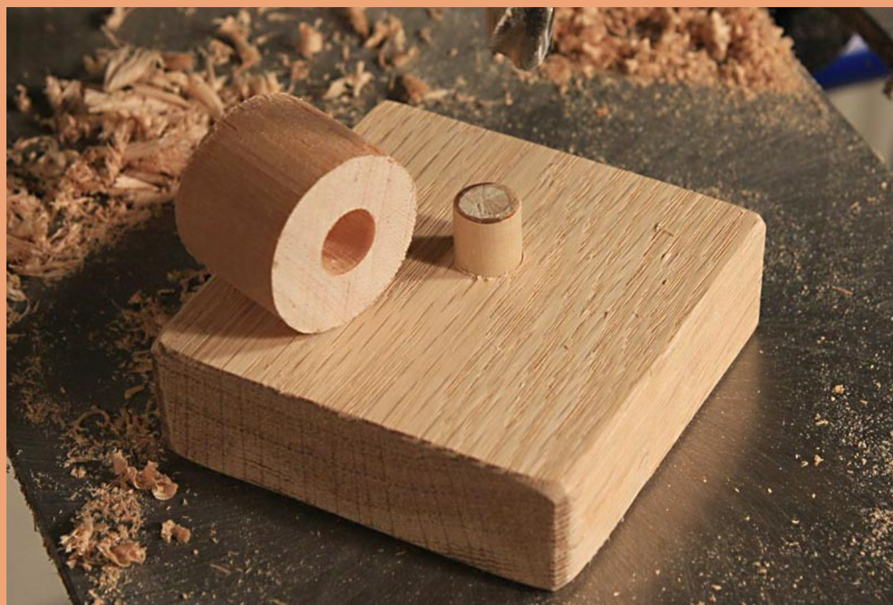
Figure 12: Locking pin jig with shaft installed.
