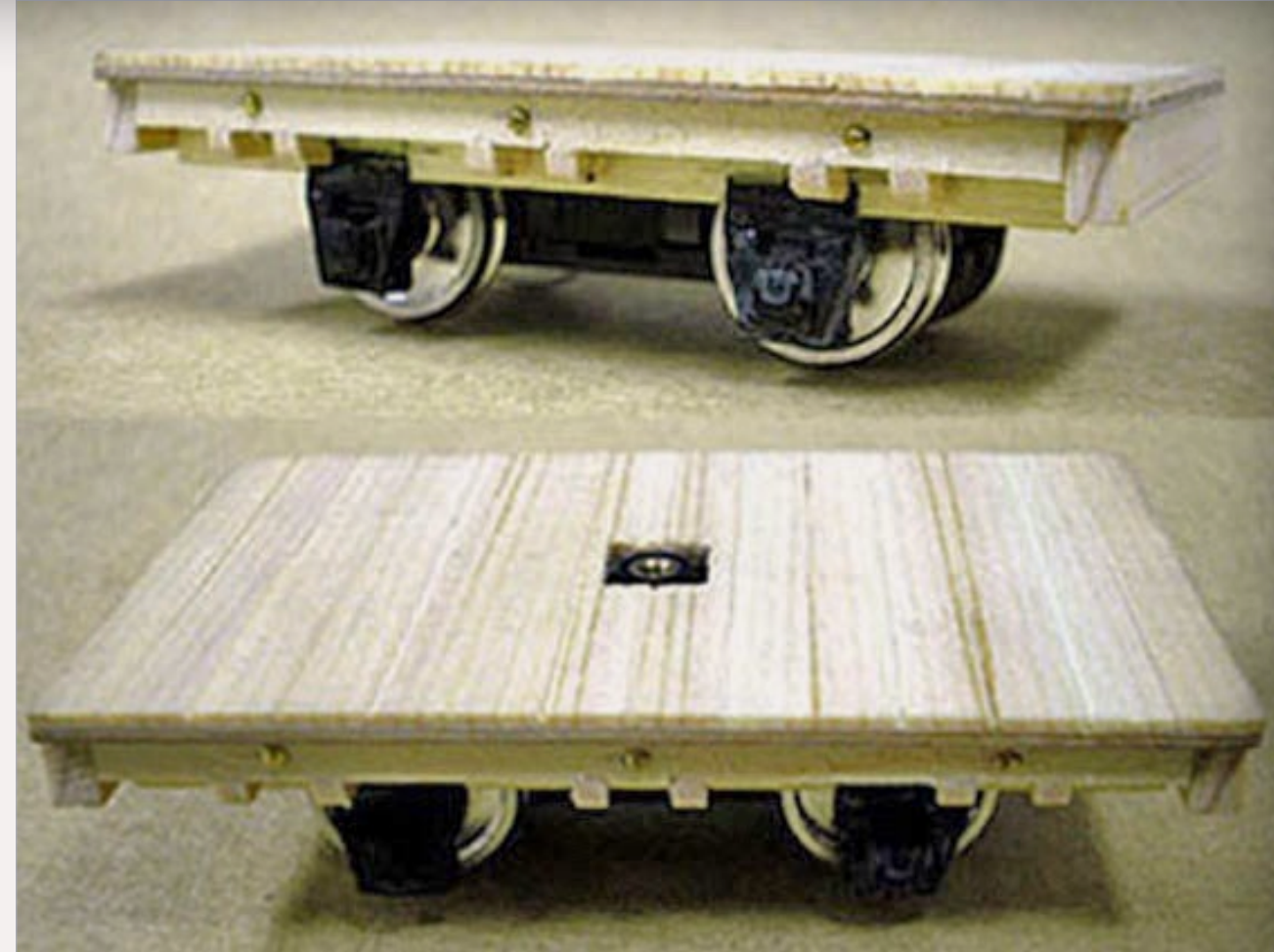
FIGURE 16: This is the early part of the construction, showing the deck over the SPUD power truck upon which No. 19 will be built. The chassis and floor were fabricated from cyprus wood strips and bars. Photo by Junior Yamachi.
