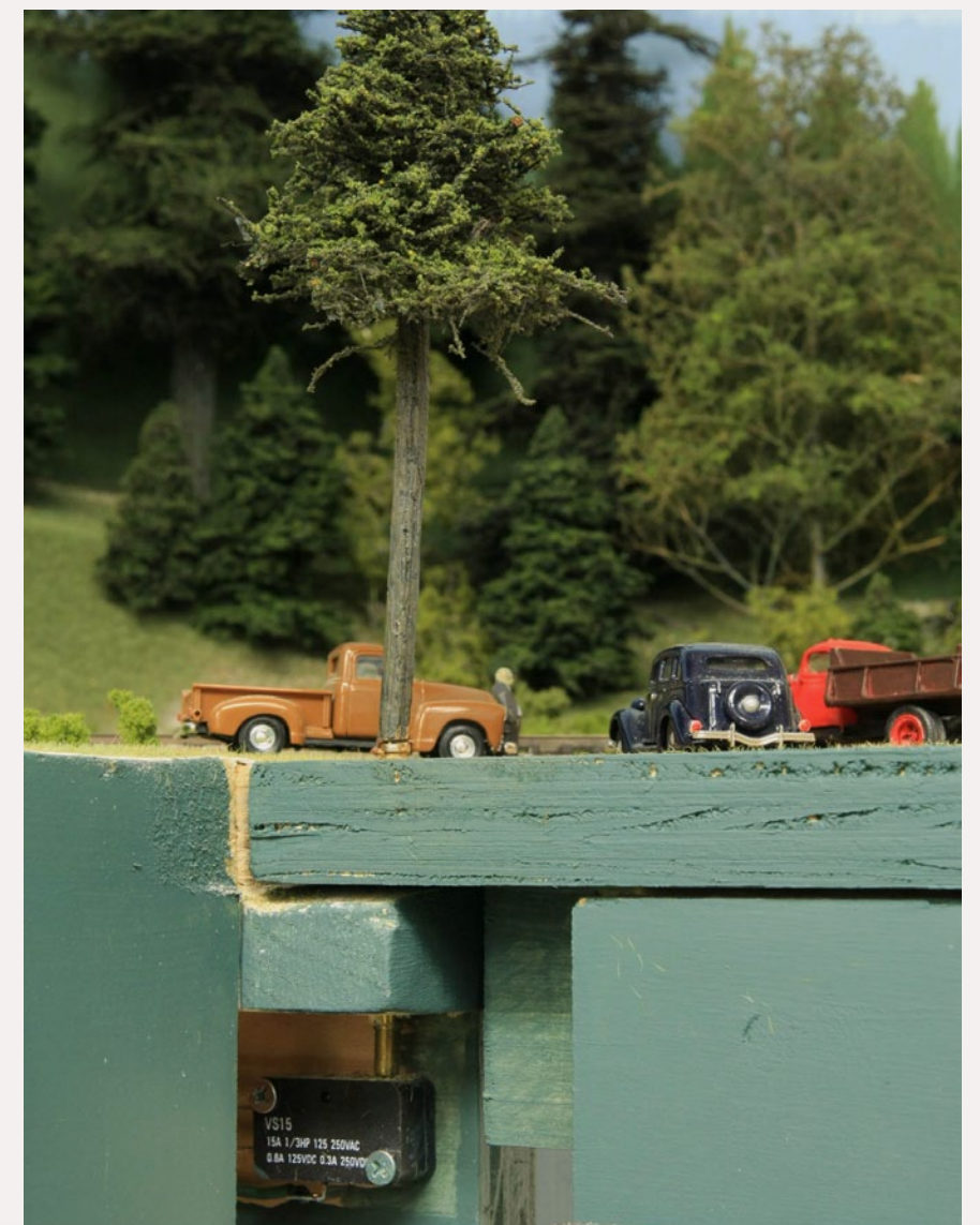
FIGURE 15: When closed, the bridge is locked in position with this pin. I made the pin from 1/8” brass rod which is inserted through brass sleeves pressed into the plywood. Using the sleeves avoids wearing the holes away by removing and installing the pin. The locking pin must be fully inserted to let the micro switch below route power to the tracks - a safety measure to prevent trains from taking a trip into the Gorge of Eternal Peril. I topped the locking pin with a small tree to disguise it.
