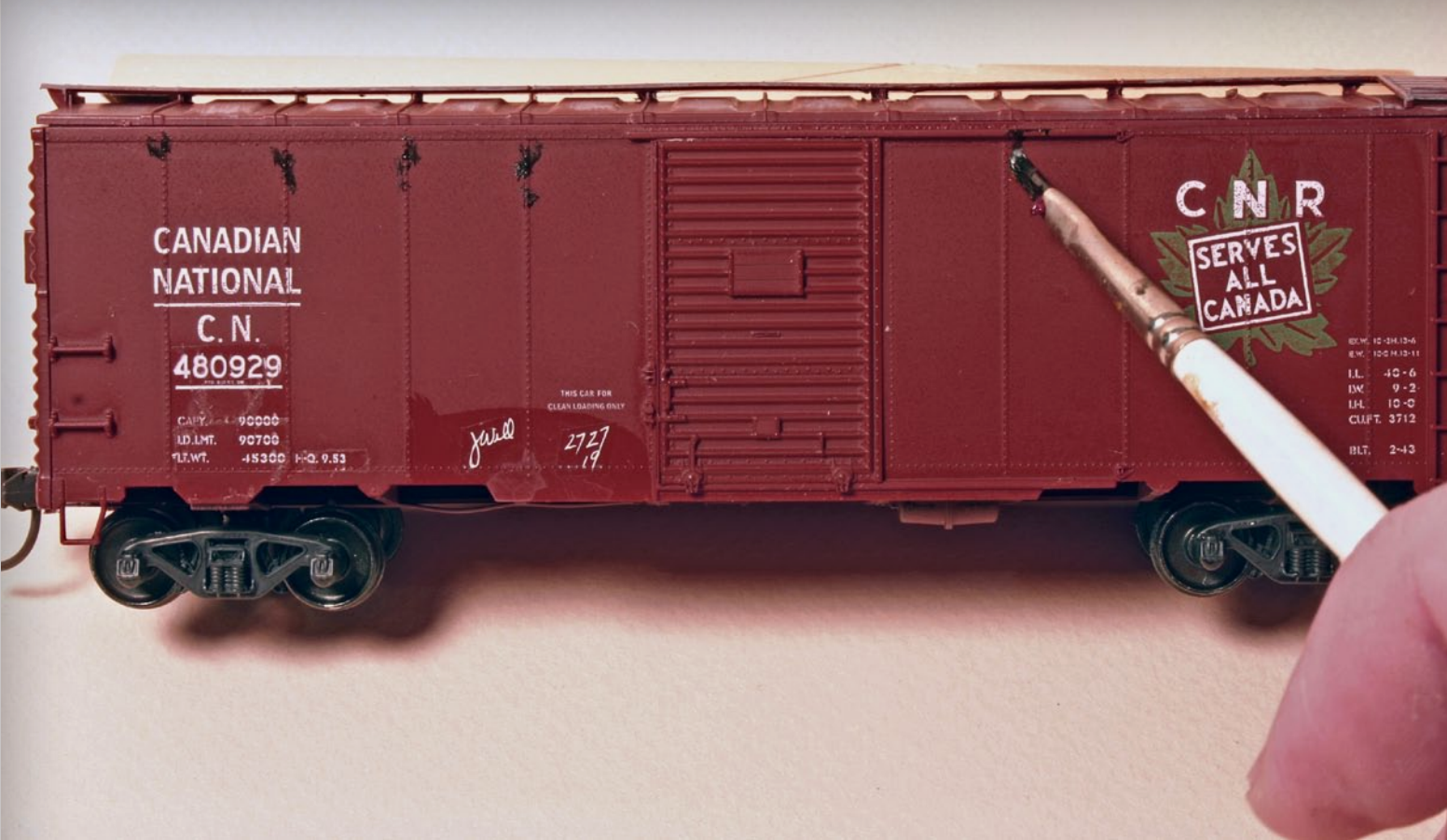
FIGURE 8: Start by dabbing a small amount of oil paint (in this case a mix of Burnt Umber and Raw Sienna) to the top of each weld line along the roofline of the car.
