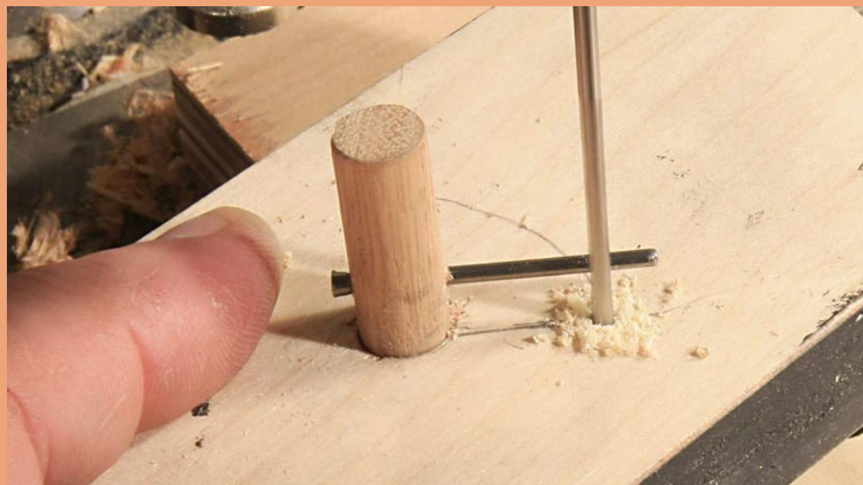
Figure 34: Drilling a travel stop hole.
