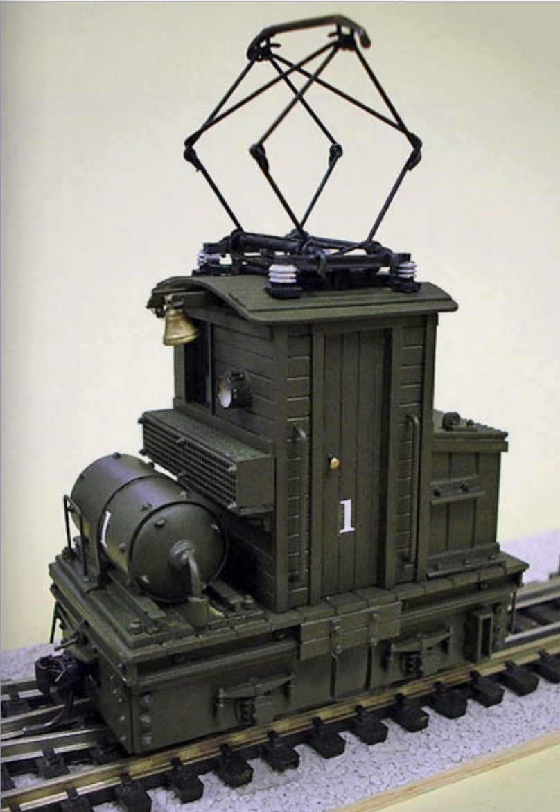
FIGURE 17: This diminutive steeple cab loco was the first mining motor built after the Surfside Traction Co. venture. This unit, seen from the right side, is smaller than the STCo. Trolleys. Photo by Junior Yamachi.
