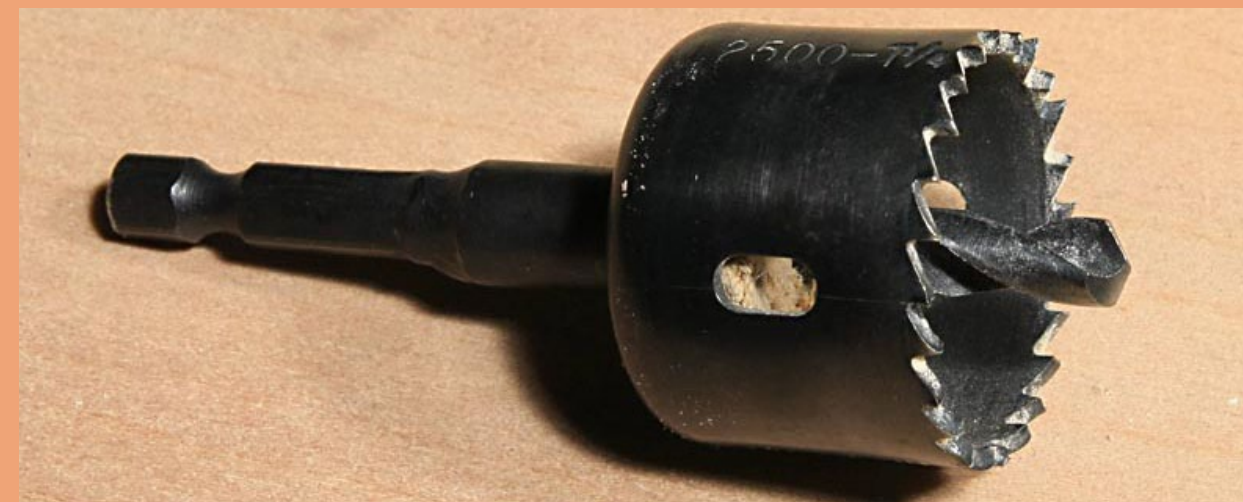
Figure 45: Hole cutter used when cutting knob-holes in fascia for behind the fascia mounting.
