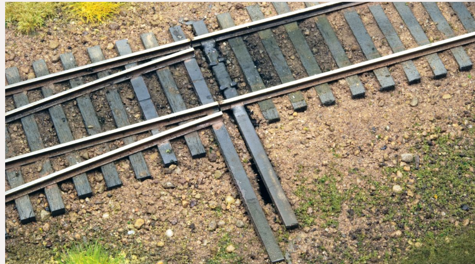
FIGURE 7: Alignment between the bridle rails and the rest of the turnout is critical in a stub switch. The prototype used a cast metal bracket to hold the ends of the rail of the turnout in correct gauge, and cast into this was a stop that would align the moveable rail of the bridle. For our models a different approach is needed, which the author covers in this article.
