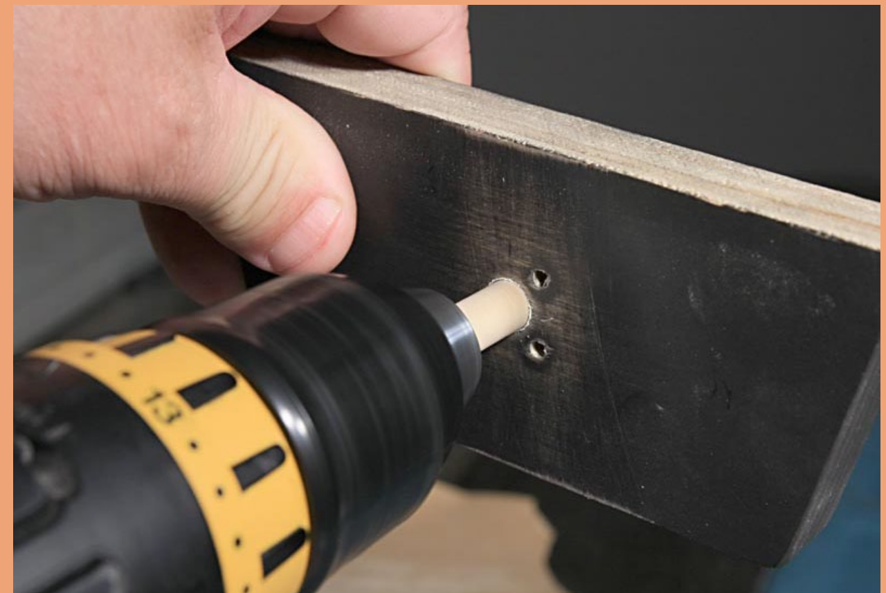
Figure 26: Burnishing a shaft in a panel hole.
