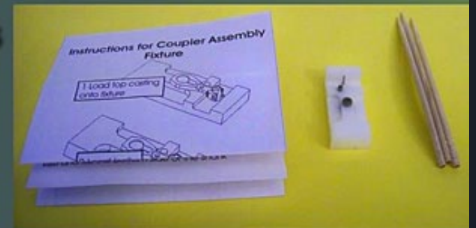
Figure 2: AFC coupler assembly jig with instructions and removal toothpicks. Used with EC87K normal shank coupler kits.
