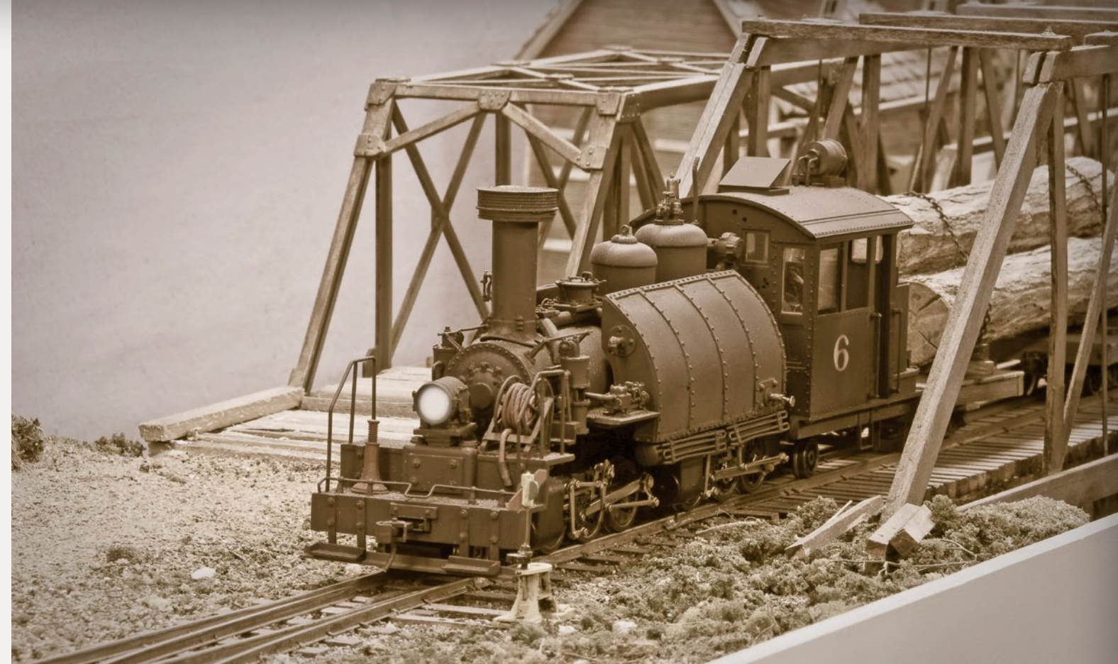
FIGURE 8: Les Davis' articulated engine crosses Deep Creek with a string of logging cars, on Steve Fisher's Deep Creek Railroad. This locomotive is an HO Mantua 2-6-6-2T converted to On30, with a Decoder and the adroit use of O scale parts. The kitbashed loco runs very nicely. The cab and back end were altered with the addition of a Forney cab. New tanks, stack and domes made up the rest of the conversion with a large number of detail parts added. Steve Fisher scratchbuilt the truss bridge. Photo by Geren Morrison.
