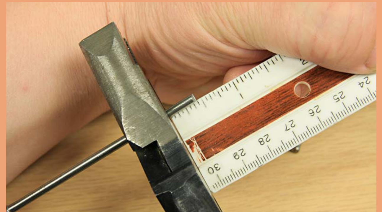
Figure 18: Cutting a locking pin from a 10d nail.
