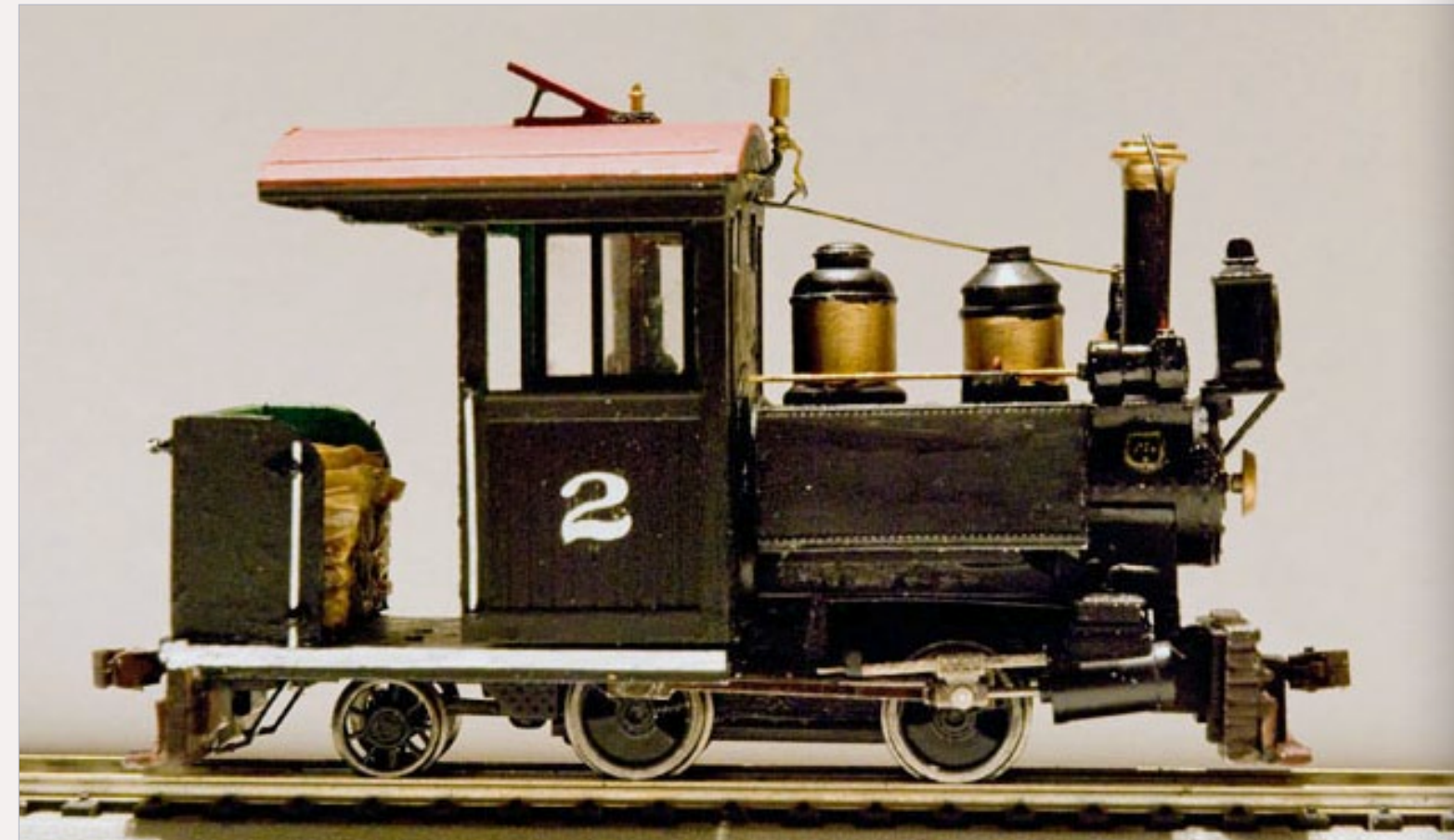
FIGURE 1: Dave Butler's kitbash of an On30 Bachman Porter using Backwoods Miniatures parts and a cut-down Forney cab results in a very elegant critter, almost too good looking! Photo by Dave Butler.
