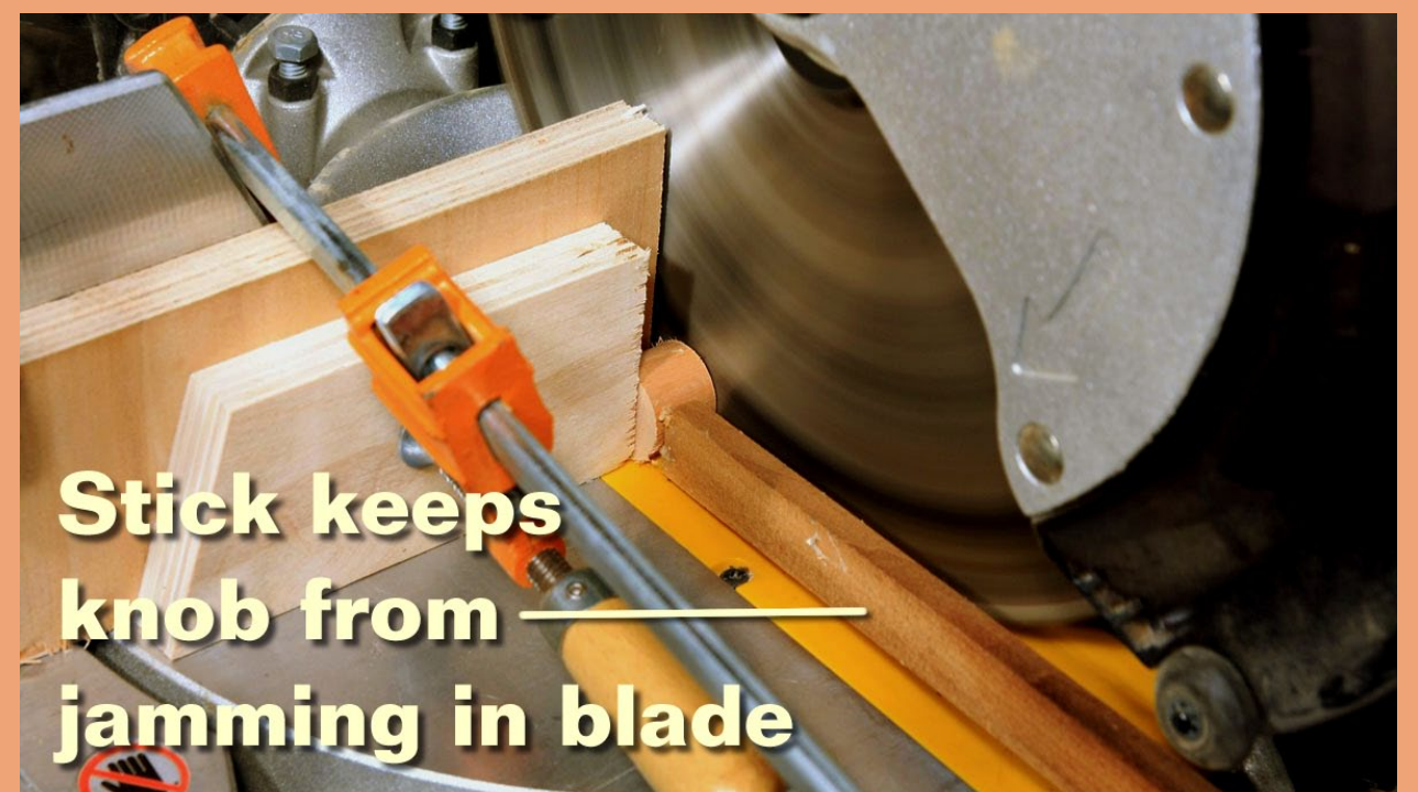
Figure 9: Cutting a knob from a 1" dowel.
