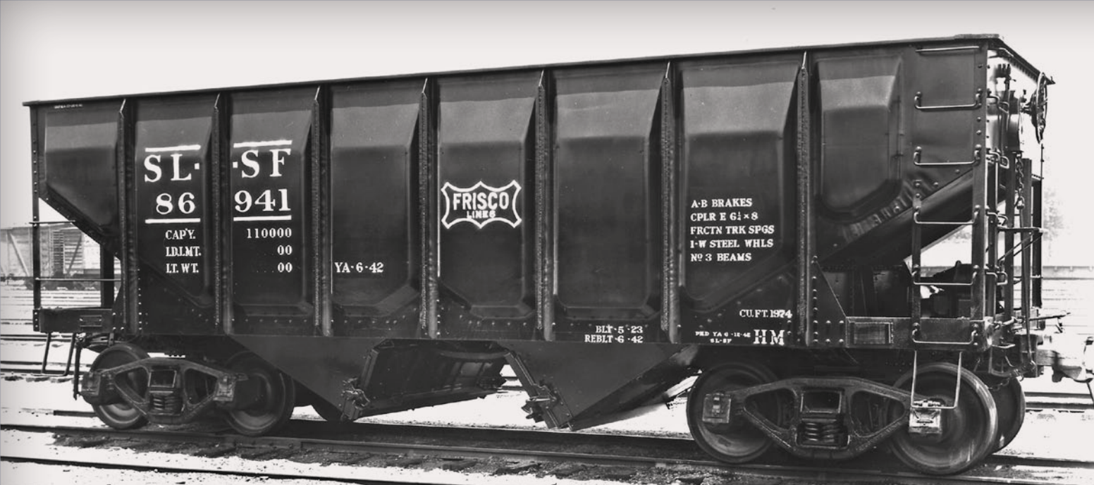
Figure 8: Rebuilt at the Frisco's Yale Yard (Memphis) shops in June of 1942, SL-SF 86941 was photographed just after it was rolled out of the paint shop and before it had been weighed and the weight data stenciled on it. The Ajax geared hand brake was new, but the ARA trucks and KD air brakes were original.
