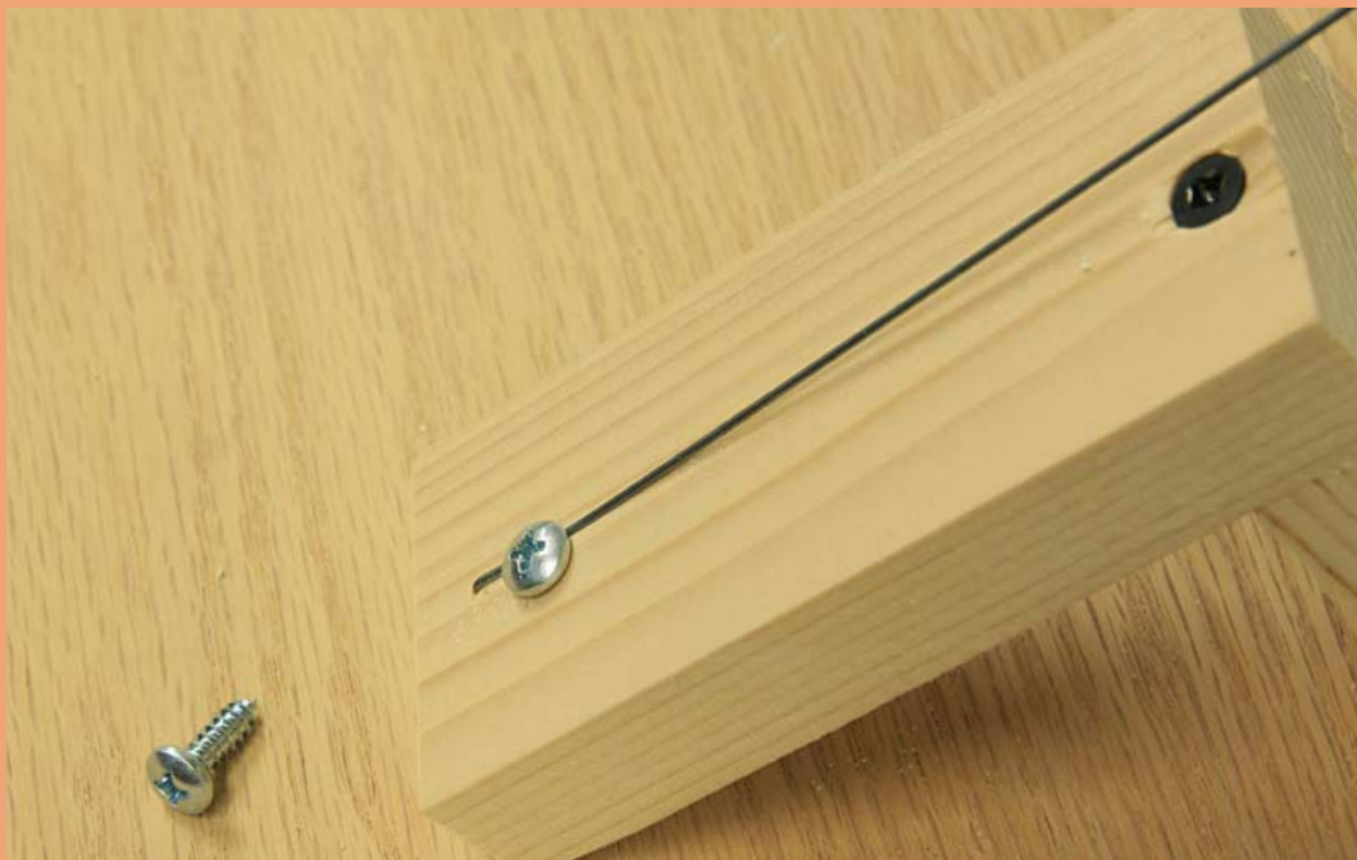
Figure 38: Actuator wire installed.
