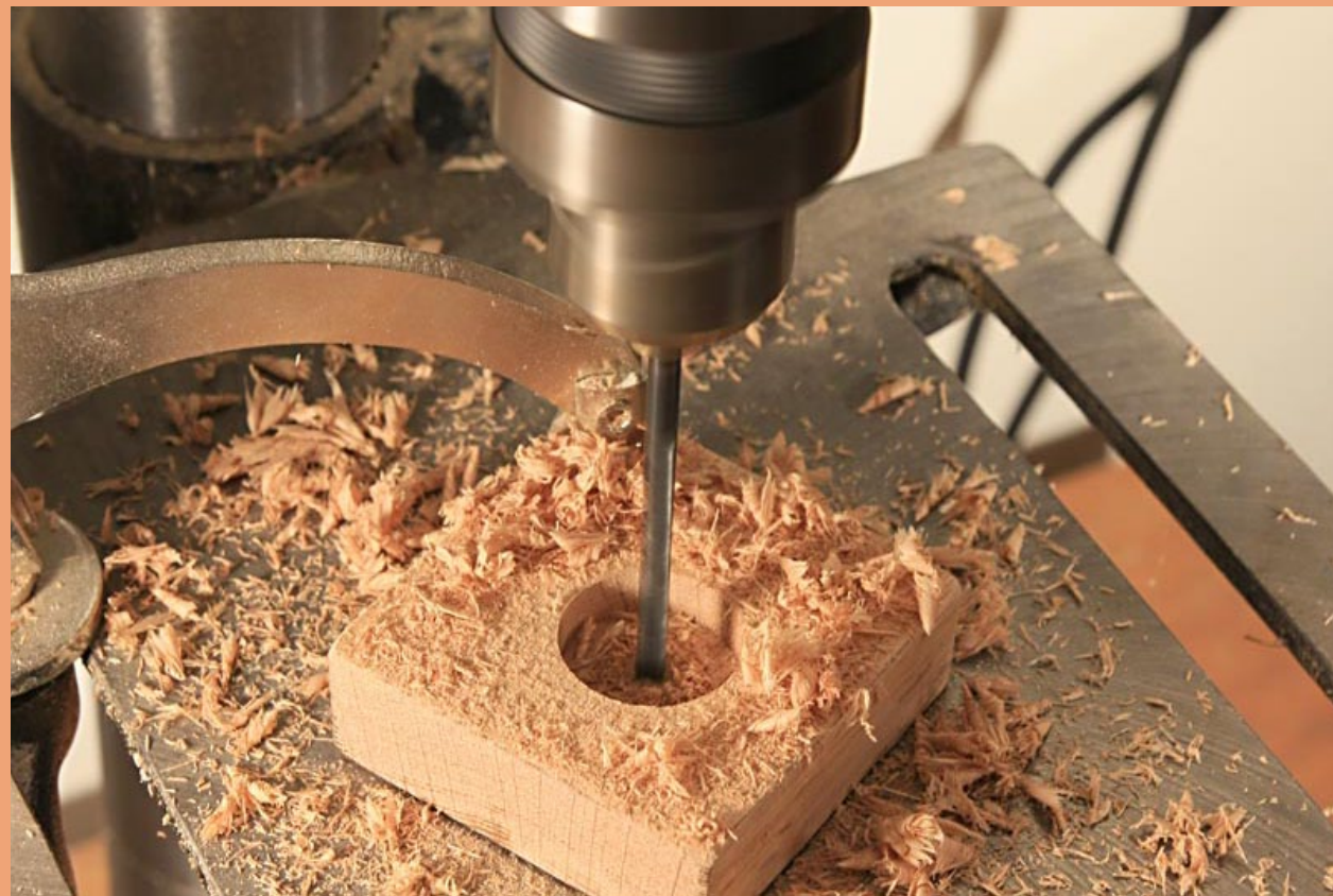
Figure 6: Pilot hole for the shaft.
