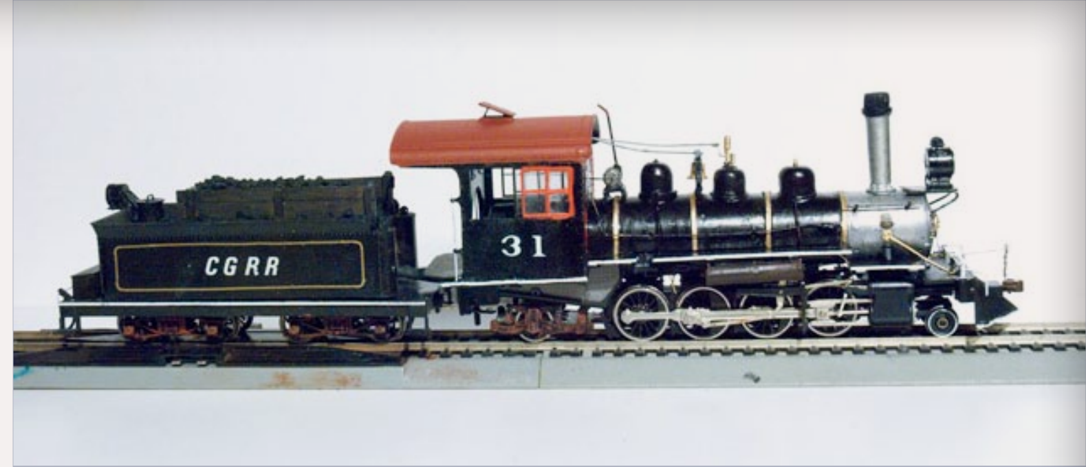
FIGURE 5: Dave created this On30 Mikado on the Athearn HO 2-8-2 mechanism. Photo by Dave Butler.
