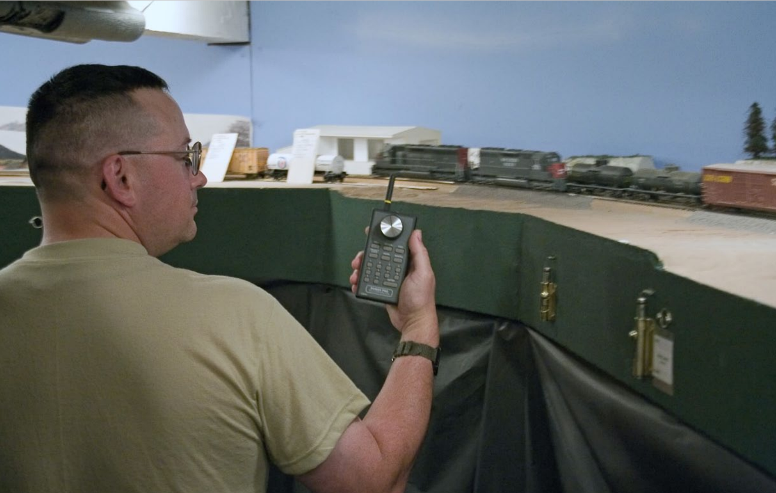
Figure 6: Ease-of-use is an important consideration when selecting a DCC system. Here we see Jeff Shultz using an NCE Cab 04R wireless throttle on Joe Fugate's HO Siskiyou Line layout. The NCE system uses plain English button labels like "Select Loco" on their throttles, which helps visiting operators like Jeff know exactly where to start in order to assign their throttle to a locomotive and run trains on Joe's layout.
