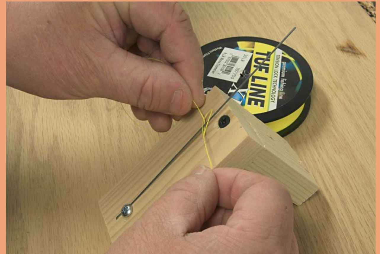
Figure 39: Attach fishing line to actuator wire.
