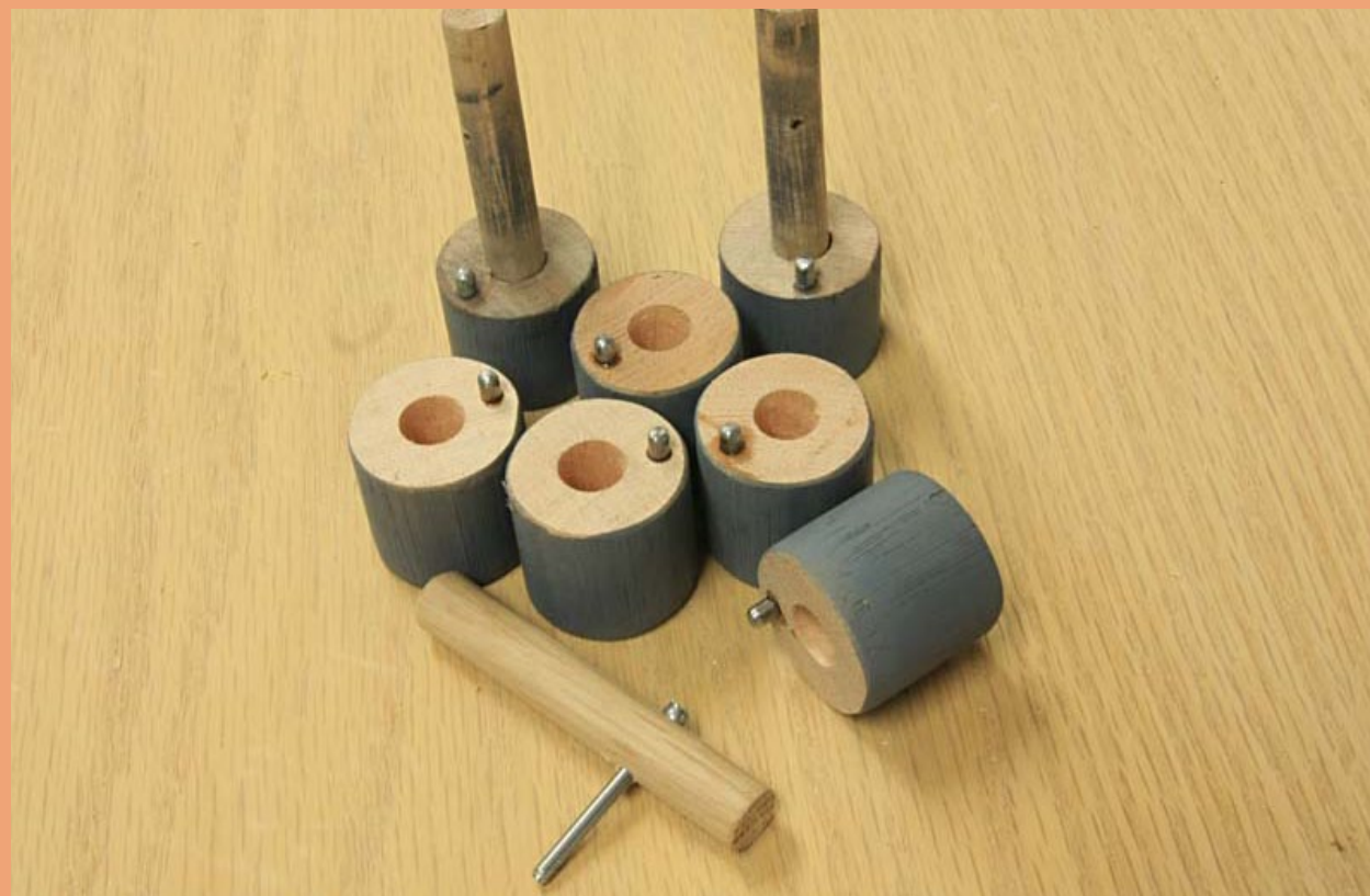
Figure 20: Knobs with locking pins epoxied in place.
