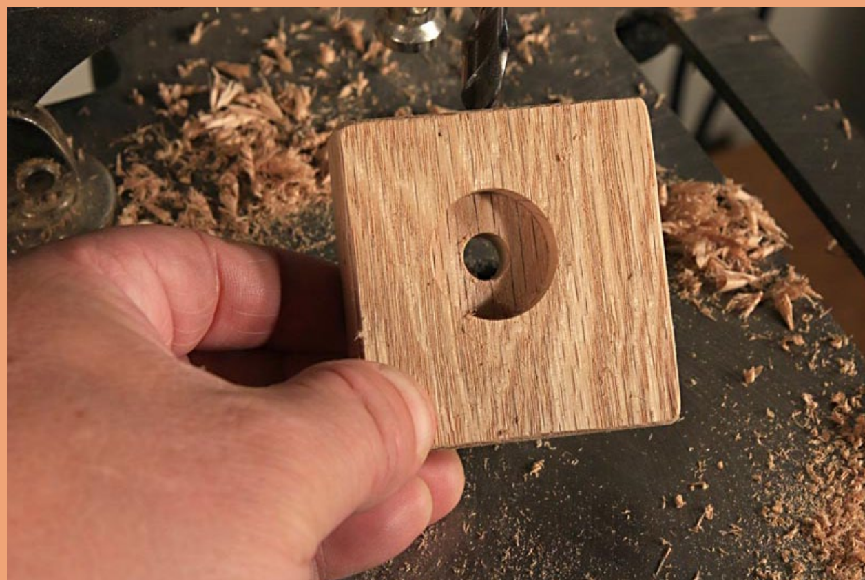
Figure 7: Completed shaft hole jig.
