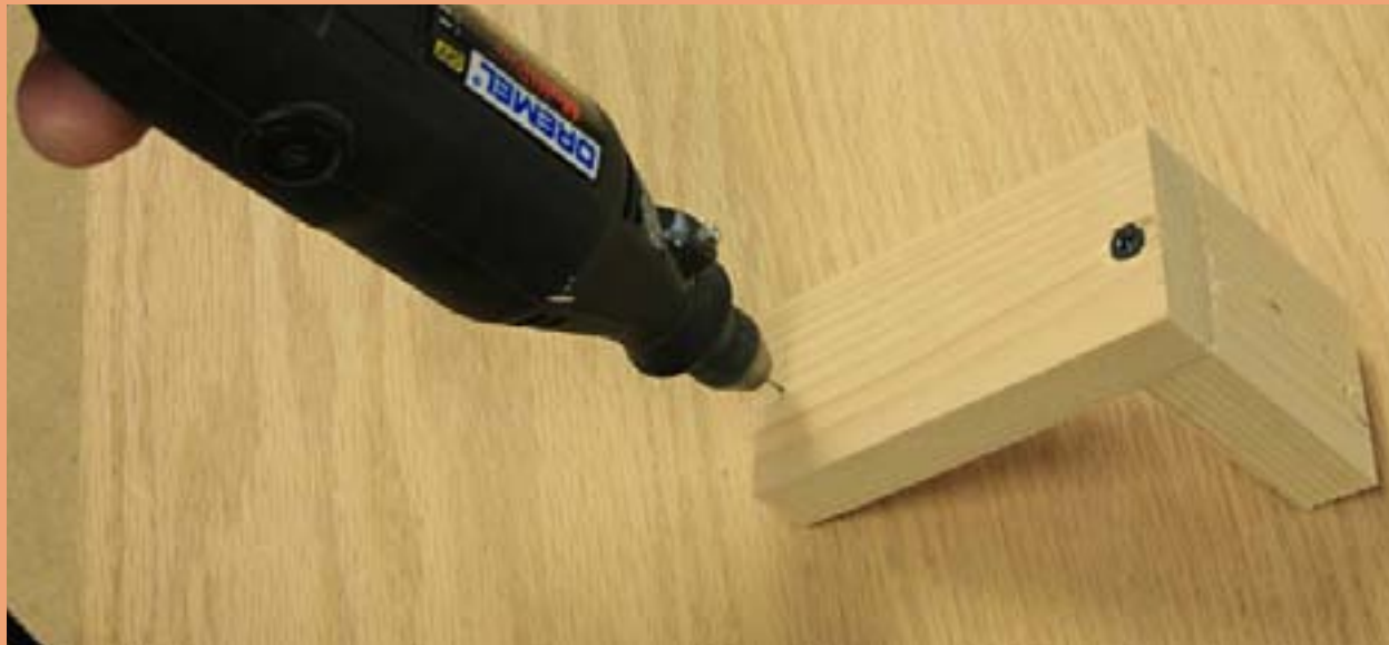
Figure 37: Drilling actuator wire hole in mounting bracket.
