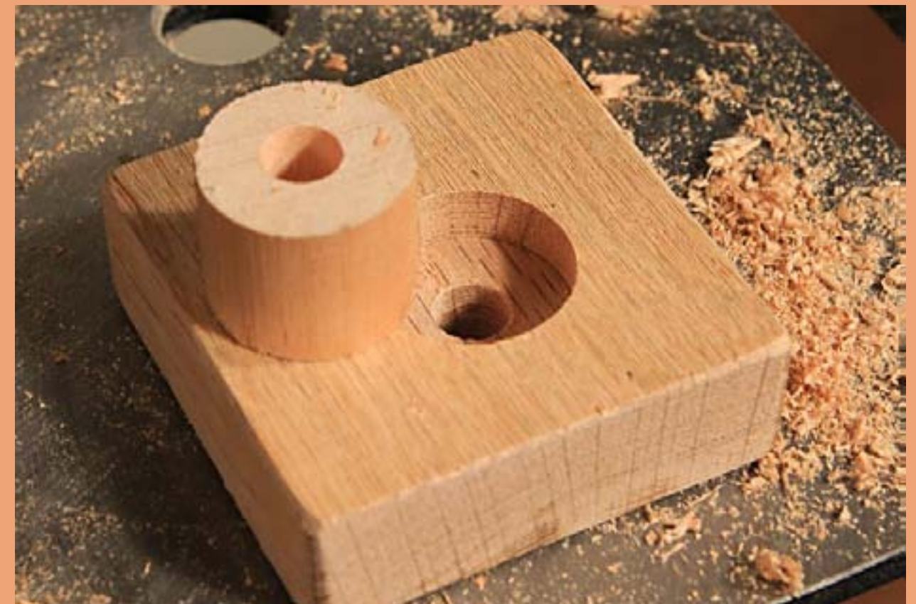
Figure 11: Knob with shaft hole and jig.
