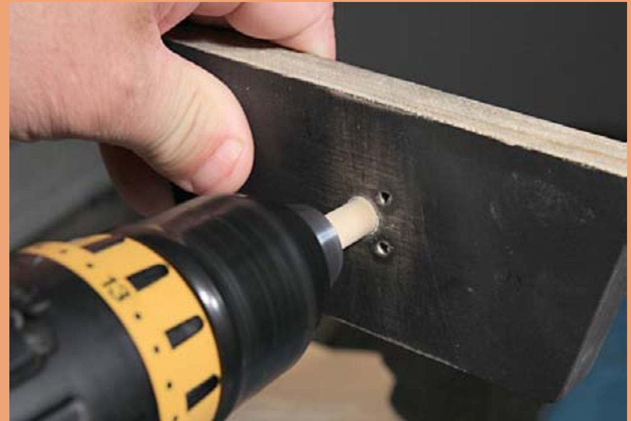
Figure 26: Burnishing a shaft in a panel hole.
