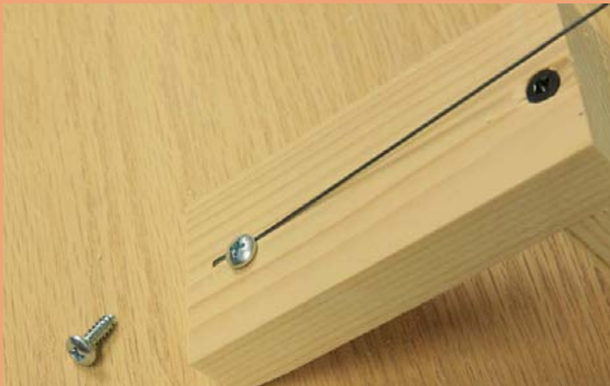
Figure 38: Actuator wire installed.
