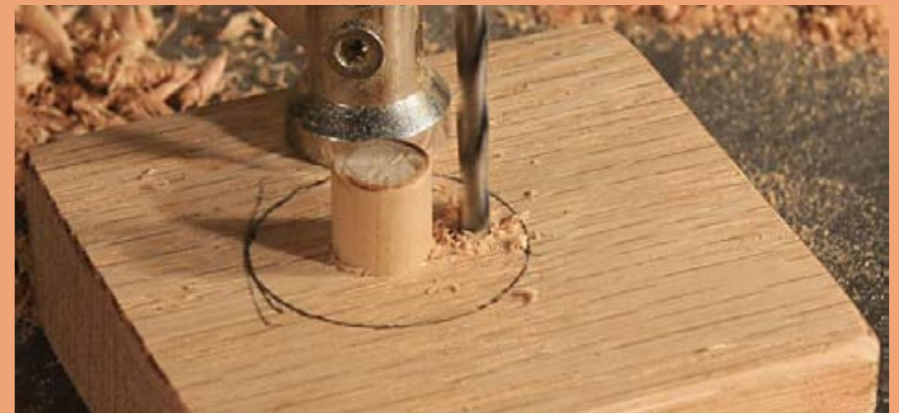
Figure 14: Drilling the locking pin guide hole (halfway between the outline and the shaft).
