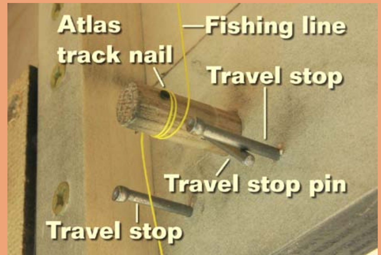
Figure 42: Line wrapped around the shaft.
