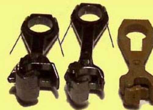
Figure 1: From left to right, a Kadee 148 "whisker" with #5 head, a #156 "long shank" with #58 head, and a Sergeant EC87A.
