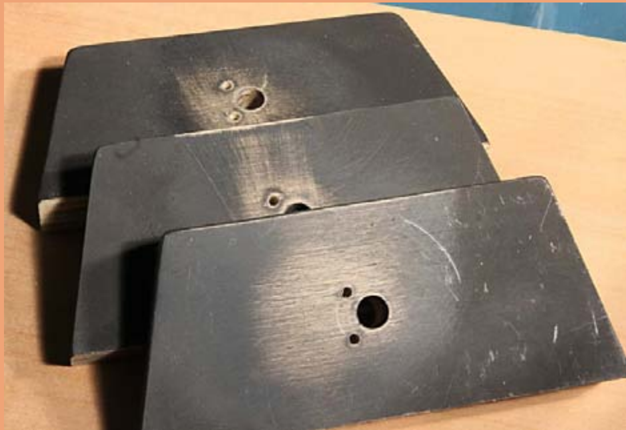
Figure 22: Panels with shaft and locking pin holes.
