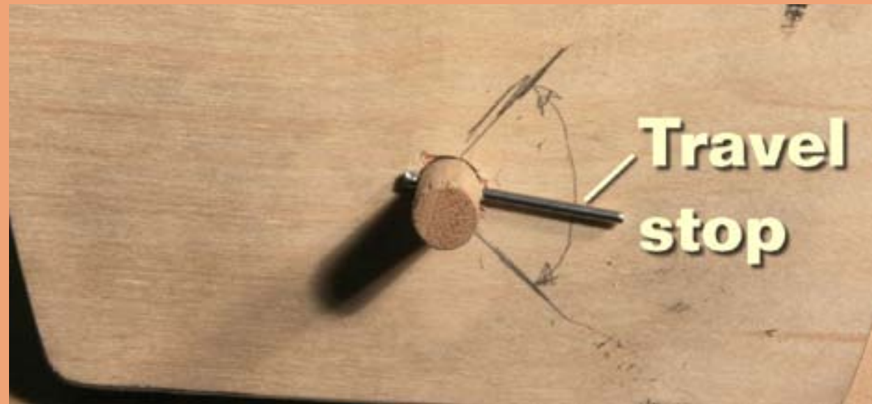
Figure 33: Travel stop range marked behind panel.
