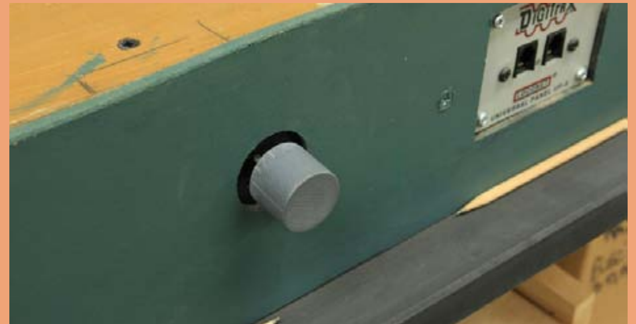
Figure 23: Turnout control installed behind fascia.
