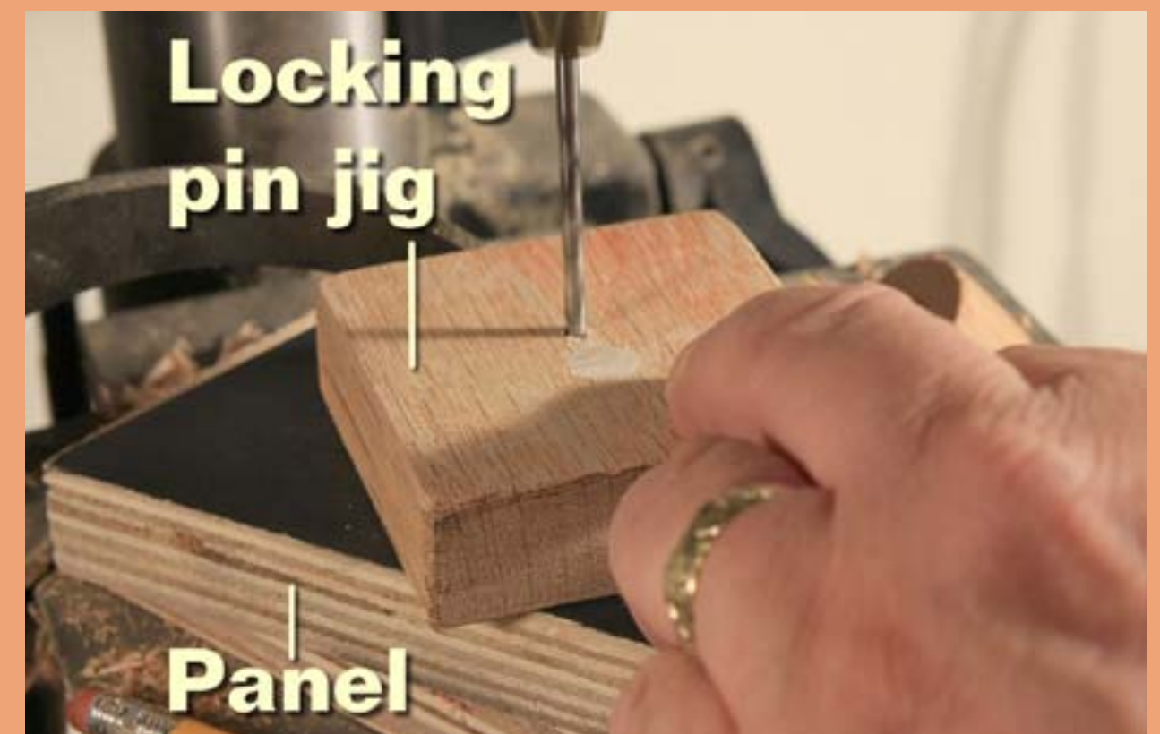
Figure 21: Drilling a locking pin hole in a panel.
