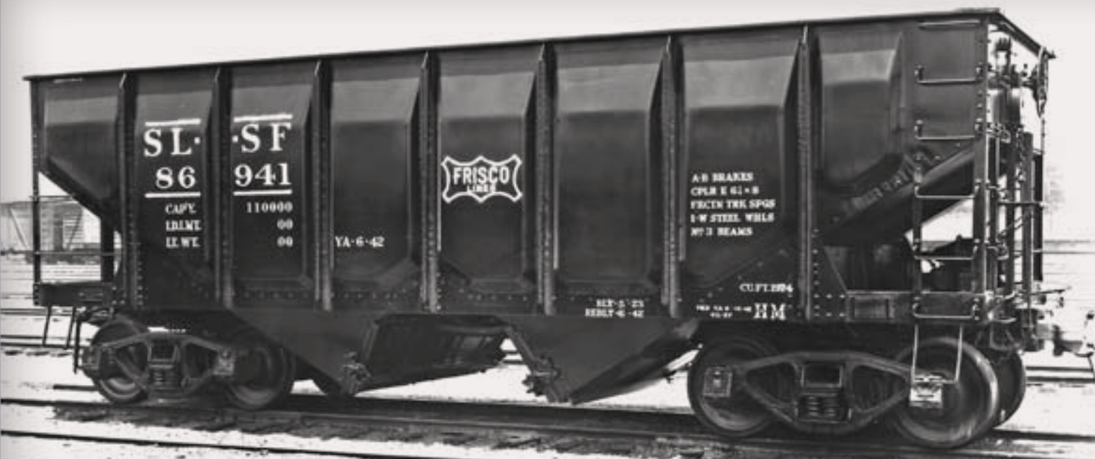
Figure 8: Rebuilt at the Frisco's Yale Yard (Memphis) shops in June of 1942, SL-SF 86941 was photographed just after it was rolled out of the paint shop and before it had been weighed and the weight data stenciled on it. The Ajax geared hand brake was new, but the ARA trucks and KD air brakes were original.
