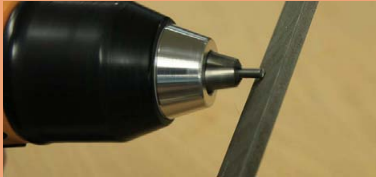
Figure 19: Deburring a locking pin.
