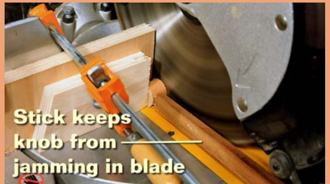
Figure 9: Cutting a knob from a 1" dowel.
