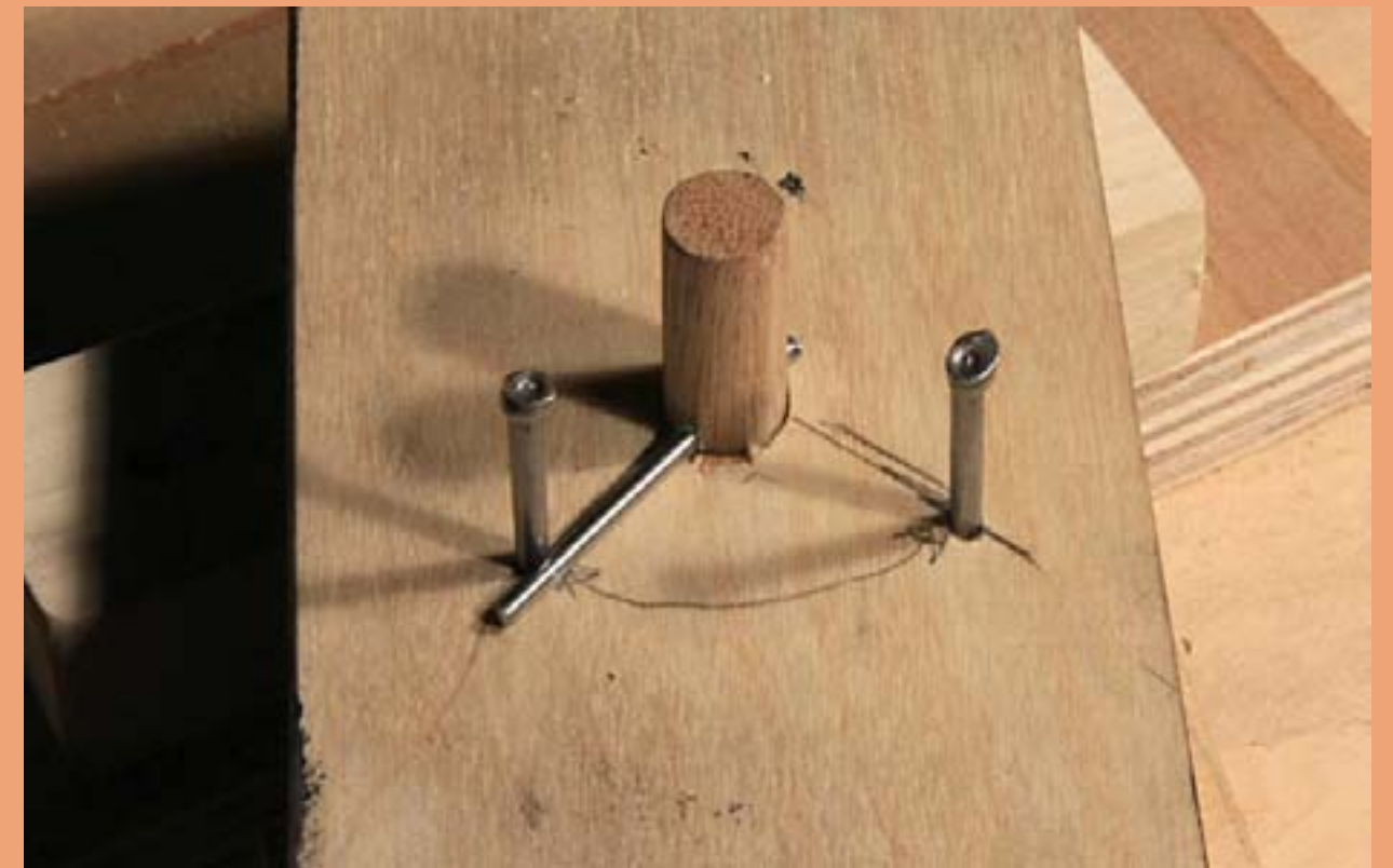
Figure 35: The travel stops installed in the holes.
