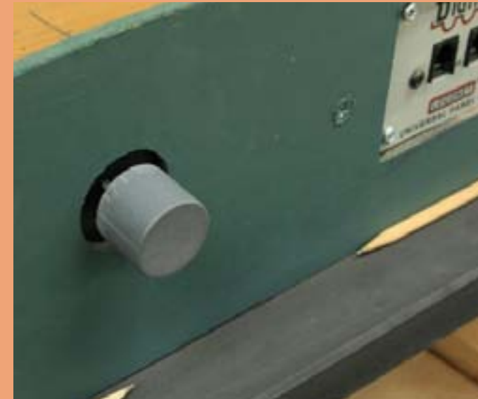
Figure 46: Hole in Fascia for knob.
