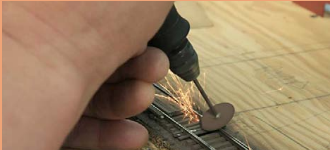
Figure 44: Trimming the actuator wire above the throwbar.
