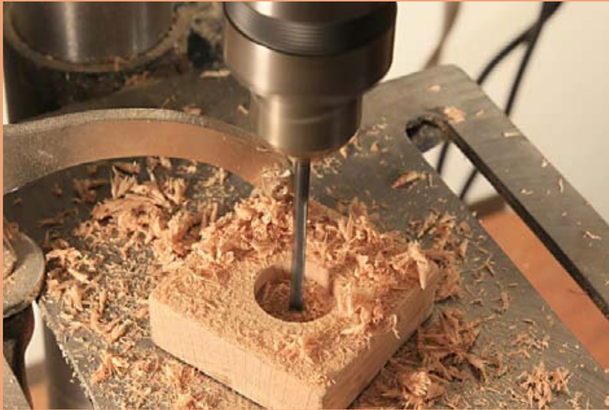
Figure 6: Pilot hole for the shaft.
