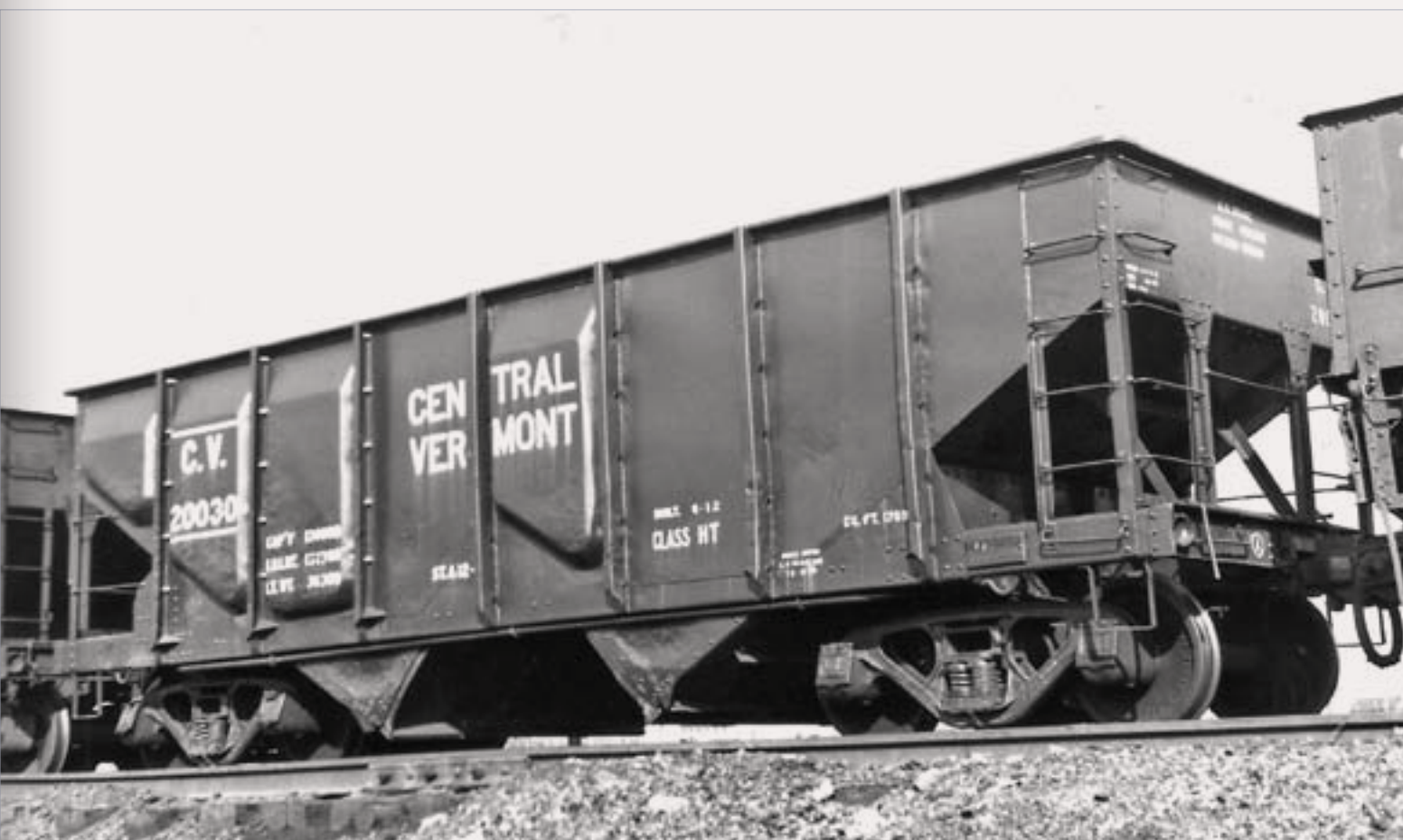
Figure 5 & 5a: The Central Vermont owned 200 steel hopper cars, built in 1912 and numbered 20000-20199, which were slightly smaller than the USRA hoppers. Starting in the mid-1930s, these cars were rebuilt with panel sides, new AAR cast steel trucks, and geared hand brakes.
