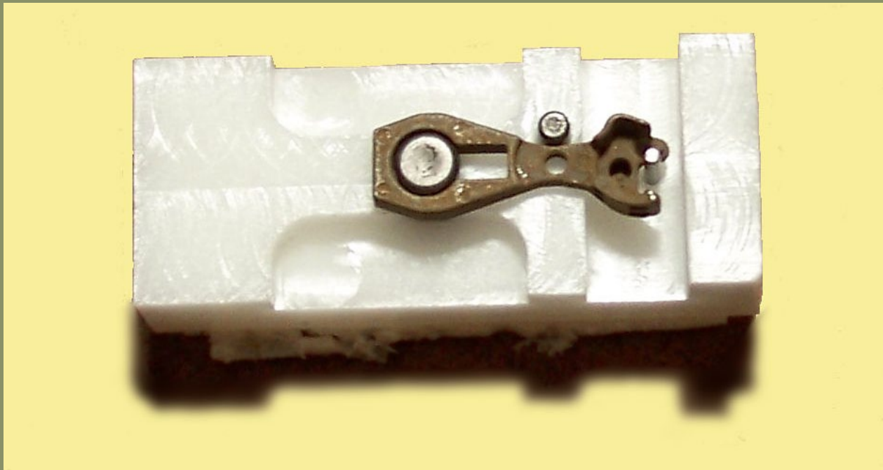
Figure 12 (Step 1): EC87K top in the AFC coupler assembly jig.
