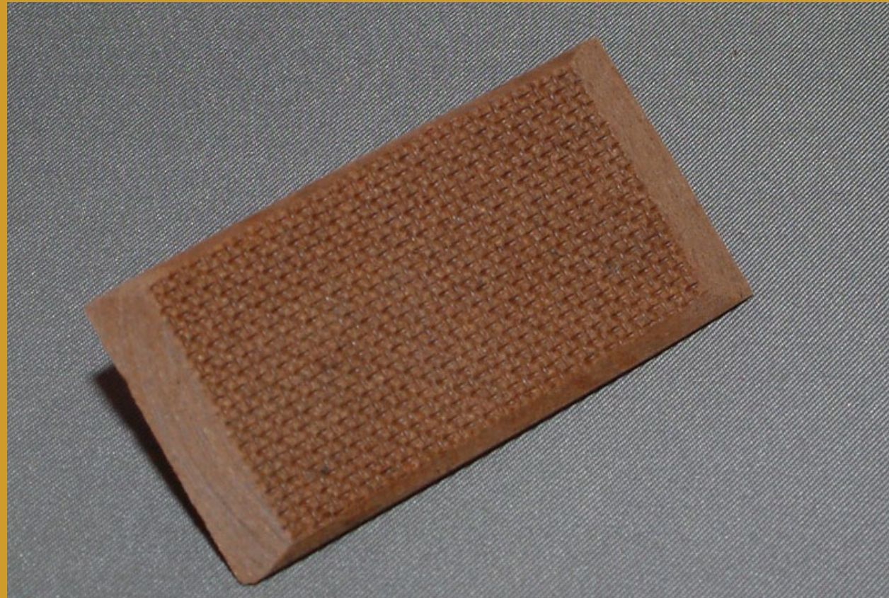
Figure 5: The cleaning pad with the edges beveled.
