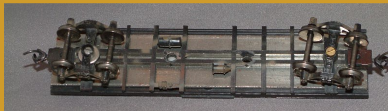
Figure 10: The car chassis underside with holes drilled for the pad.
