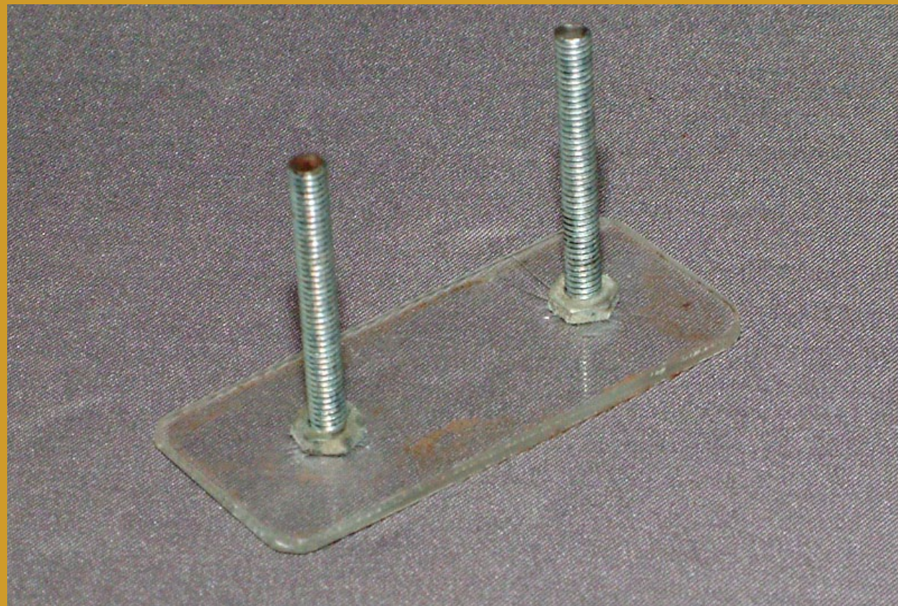
Figure 3: Nuts securing the rods in the plastic.
