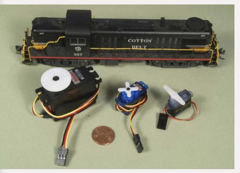
FIGURE 1: Three sizes of R/C servos with an HO scale locomotive and a penny for size comparison. From the left are a standard, mini and micro servo. All 3 servos have a standard 3-pole plug and despite their different sizes and all respond identically to standard R/C servo signals. The white servo arms can be replaced by a wide variety of different size and shapes for connecting to different devices. In this article I show a few uses for model railroads including turnouts and semaphores.
