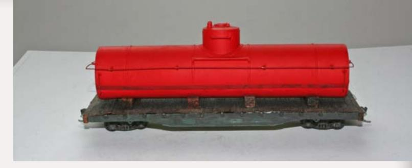
FIGURE 12: The tank car built on a flat car uses the same "flat" construction as the gondola. The length of the car is 20 feet and the tank is from a junk-box Lionel O27 trainset car. The tank, based on the venting and the horizontal courses is the style of the 1920s and newer. A very modern car.
