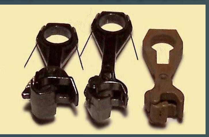
Figure 1: From left to right, a Kadee 148 "whisker" with #5 head, a Kadee #156 "long shank" with #58 head, and a Sergent EC87A.
