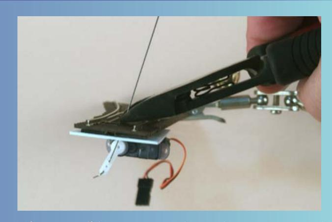
Before cutting off the excess wire, gently move the servo arm to one side as this pulls the wire down in to the hole. If you cut it off too close then when you move the arm to the side, the wire may pull out of the hole.
