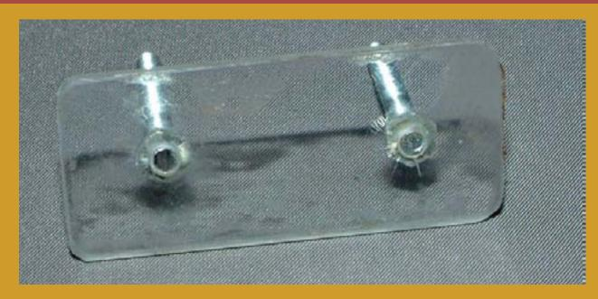
Figure 2: The plastic base for the cleaning pad with threaded rods flush with the sheet.
