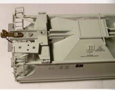
Figure 6: EN87K narrow shank coupler, assembled, mounted in **Genesis Trinity Covered Hopper.** Note friction spring against pivot pin.
