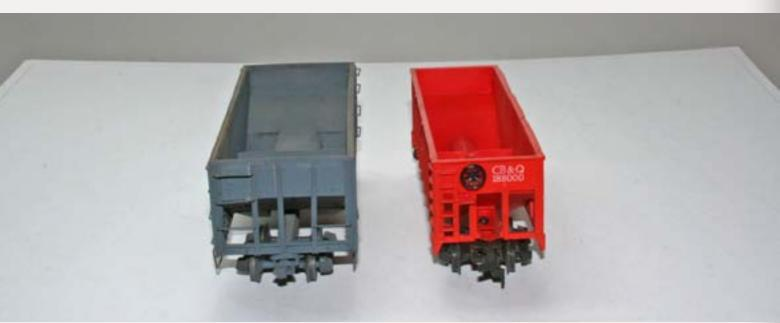
FIGURE 10: The red life-Like HO 55 ton hopper from which I made the On30 freelance 10 Ton hopper shows the car was widened and slightly raised in height but not lengthened. This is a small hopper and will be pulled by a small critter. Too massive a hopper car would look inappropriate in its intended setting and use.
