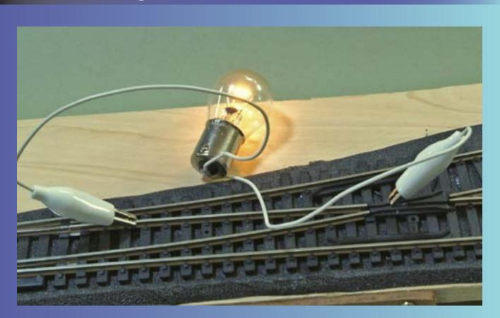
I am using a 12V automobile light bulb to test the frog circuitry. The turnout is in the closed position and the frog should be at the same potential as the closed rail. However, as you can see, the frog is connected to the wrong rail as the light bulb has lit, indicating a short.
