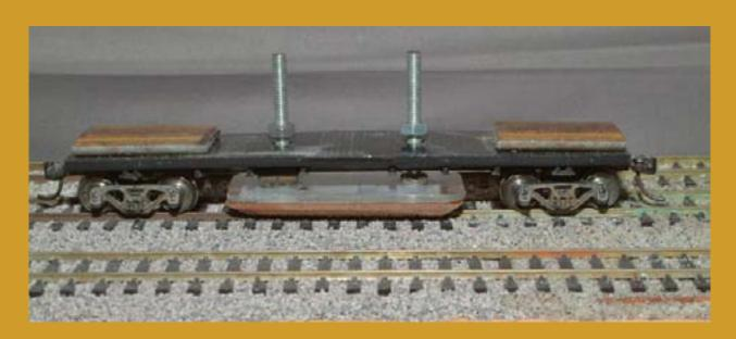
Figure 11: Setting the lower weight nuts. With the pad on the track leave space under the nuts.
