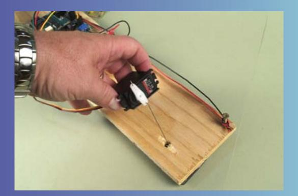
The servo is now attached to the subroadbed. You can clean the plywood surface of dust and loose particles with a piece of blue masking tape. Just stick it on and remove it a few times to pick up the loose particles. Push the wire through the hole and through the hole in the throw-bar. This is by far the trickiest bit in the whole procedure. If the layout can't be turned upside down, a small mirror can be used to aid this procedure by angling it so you can see up the hole and position the wire.
