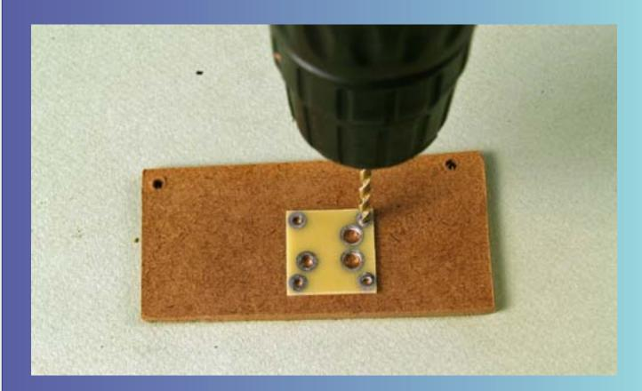
I am now going to mount the fascia controller on a small piece of hardboard to simulate a fascia. I am using the drilling template that comes with the fascia controllers to guide the placement of the holes.
