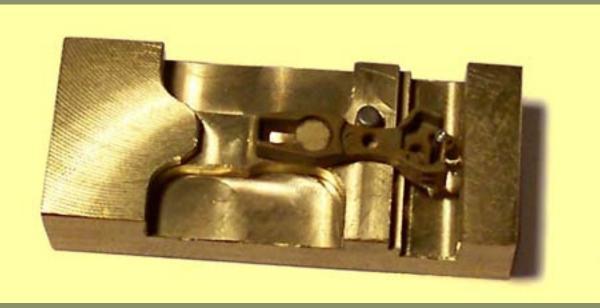
Figure 11a (Step 1): EN87K top in the AFN coupler assembly jig.
