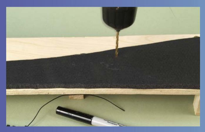
Drill holes for the feeder wires to poke through.
