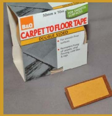
I stuck the Masonite pad to the plastic with double-sided tape. I used tape for smooth surfaces. The type for rough surfaces is a lot stickier and you may not be able to remove the pad. This allows the pad to be replaced. A little levering will remove the pad. I use it rough side down, partly because the smooth side will stick to the tape better, but also because I believe the rough side cleans better.
