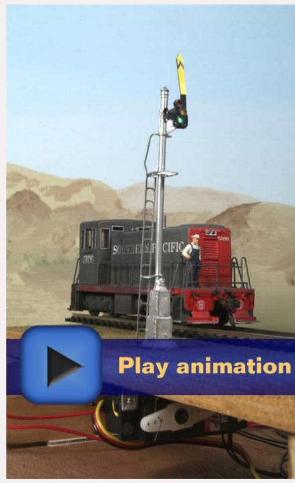
FIGURE 4B: A 3-position upper guadrant semaphore actuated by a servo being run through its paces by an inspection crew.
