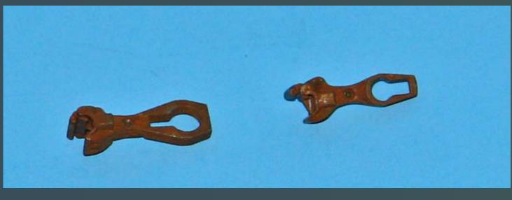
Figure 1: EC87 (left) and EN87 Couplers.
