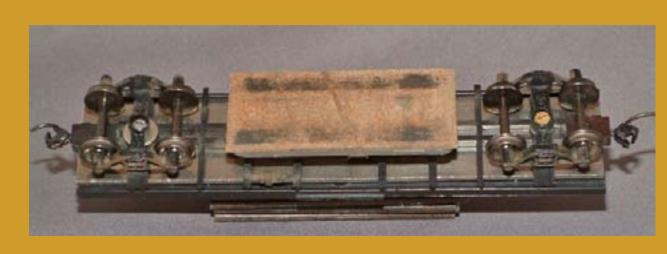
Figure 9: The car after doing its job. This is best cleaned off with sandpaper wrapped around a wood block.
