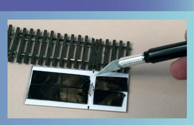
Double-sided tape applied to the styrene base ready for mounting on to the bottom of the turnout. Note how there is a slot in the tape where the throw-bar is going to fit. We don't want the throw-bar stuck to the tape or it won't move!
