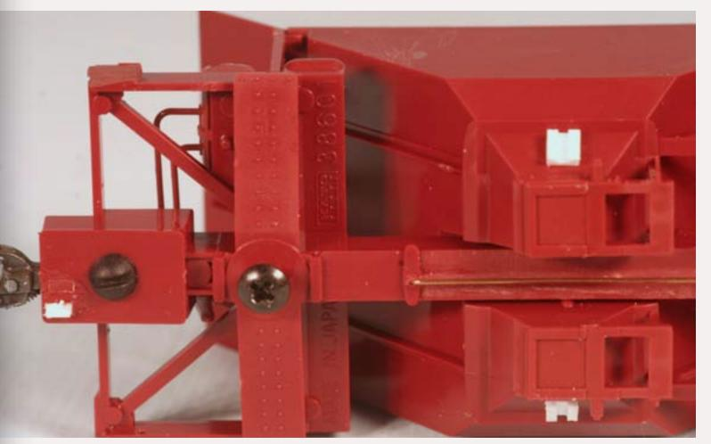
Figure 3: The appearance of the car when viewed in profile can be improved by scraping off the cast on brake rod with a chisel blade model knife. Replace it with a piece of .0125 phosphor bronze wire bent to fit into holes drilled in the centers of the cast on brake levers as shown.
