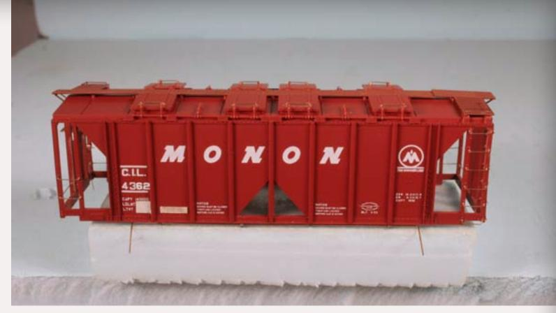
Figure 8: The train air line runs along the right side of the car when facing the "B" or brake end. The air line is made from .0125 phosphor bronze wire and is held in place with Athearn handrail stanchions. Small eye bolts can be substituted for the stanchions.
