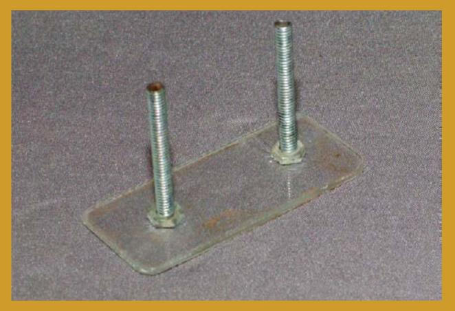
Figure 3: Nuts securing the rods in the plastic.
