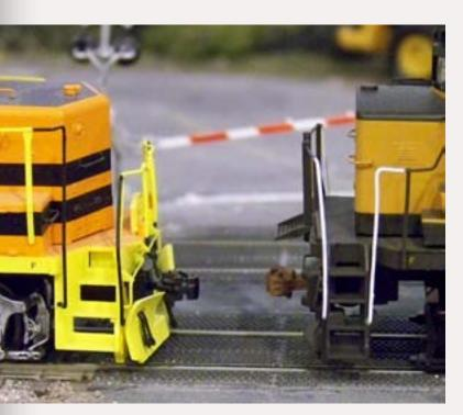
Figure 8: Kadee #148 coupler (left) in an Atlas GP38 and EN87A coupler mounted in an Atlas C425 (right).
