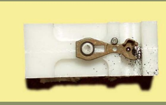
Figure 12a (Step 2): EC87K top with steel ball inserted. Sparkly stuff is Kadee powdered graphite lubricant.
