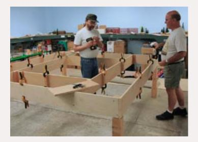
FIGURE 10: Construction of the helix table under-the-surface bracing.
