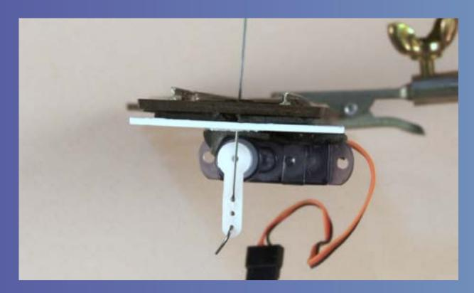
An end-on view of the mounted servo in the center position.
