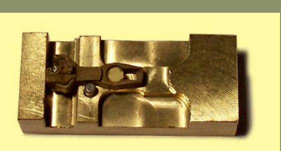
Figure 11c (Step 3): EN87K completed coupler with bottom plate CA'd on.
