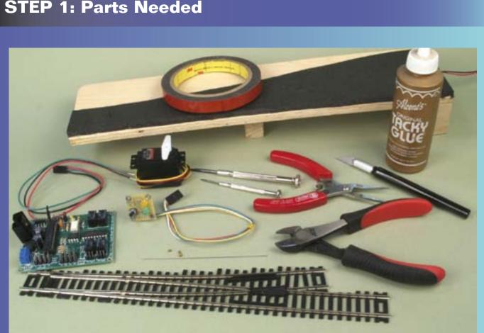
Parts needed for this project. An Atlas code 100 #6 turnout is shown. A standard size servo is in the center left. At the far left is a Tam Valley Depot Quad DCC Decoder and Servo Driver. This will let us drive the servos both with DCC and with the fascia controller shown just below the servo.
