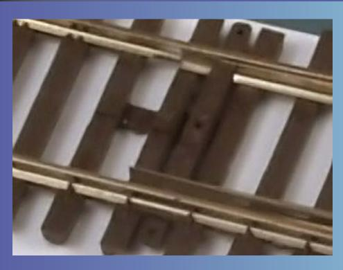
The micro-engineering turnout has a small hole in the middle of the throw-bar that will be used for the actuating wire. If there isn't a hole in your turnout then drill one with a small drill a little larger than the wire.
