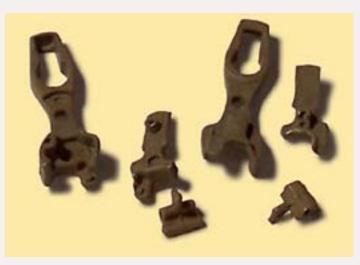
Figure 5: EN87K narrow shank couplers, pre-assembly. Pieces seen: top (with shank), bottom, and knuckle. Not shown: steel ball to lock knuckle closed and shank friction spring.
