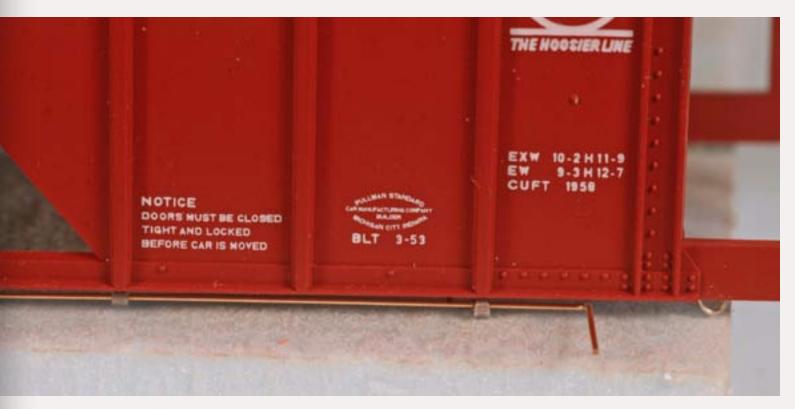
Figure 9: The newly added train air line is folded under the car side and secured with ACC. Also note the phosphor bronze towing loop that as added to the side sill. This is one of four such details added. The prototype cars were built by in March 1953 at on line customer Pullman Standard of Michigan City, Indiana as the nicely done factory painted lettering correctly depicts.
