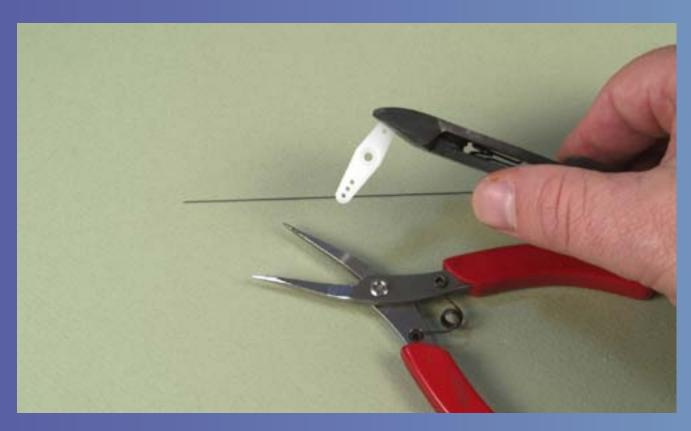
One end of the servo arm is shortened by cutting it off with diagonal pliers to give it sufficient clearance. Be certain not to cut the last hole.
