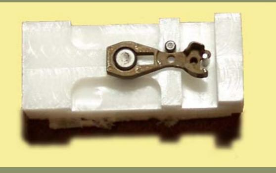
Figure 12 (Step 1): EC87K top in the AFC coupler assembly jig.
