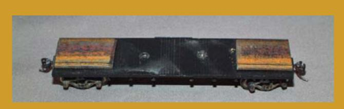
Figure 9: The car chassis, fitted with steel weights over the trucks.
