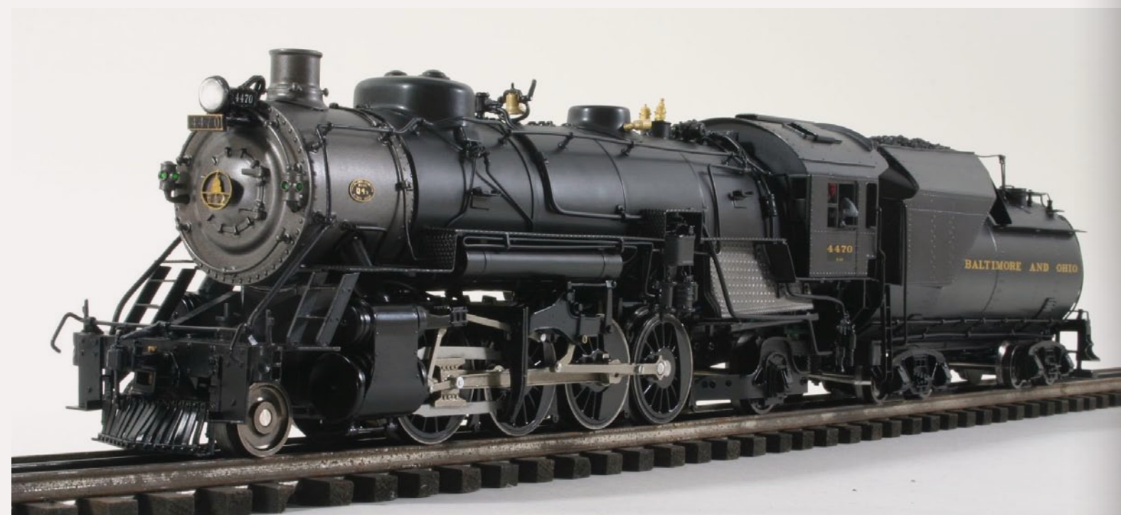
FIGURE 1: 3rd Rail Division of Sunset Models expects delivery this month on its O scale Baltimore & Ohio class Q-4b 2-8-2 steam locomotives. The hand-crafted brass models of the Baldwin-built Mikado will be offered in both two-rail and three-rail versions.
