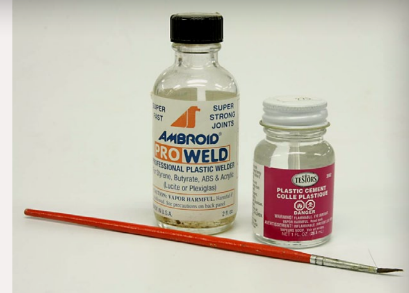
Figure 1: Two of the many types of solvent-based liquid plastic cements and a small paint brush suitable for applying the glue.
