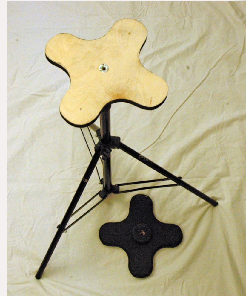
FIGURE 2: The top table is cut in the lobed shape to offer the best support for straight or curved modules while saving weight. Note the 1/4" x 20 insert in the center hole to securely attach the top to the light stand. The light stand may be equipped with friction screw fittings or snap clips for fast height adjustment. Photo by Kevin Hunter
