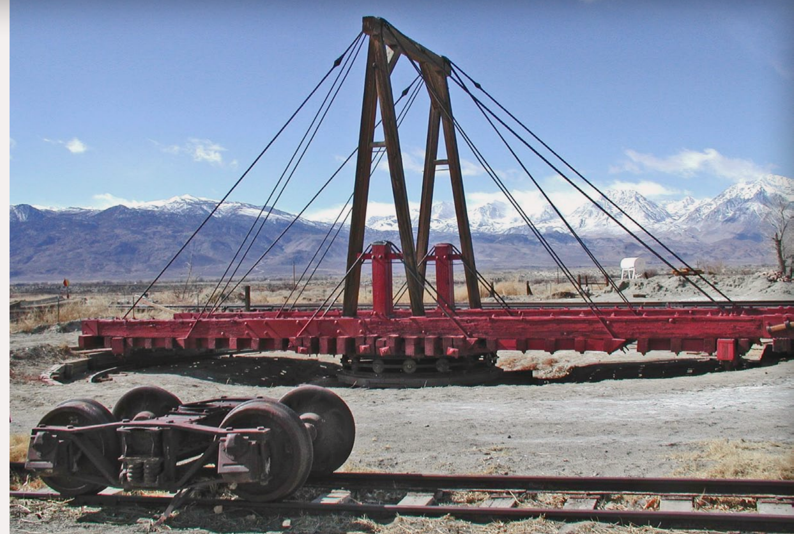
Figure 8: "Gallows"-style turntables turned the diminutive engines at Laws and Owenyo. The Laws Railroad Museum and Historic Site has preserved the turntable on-site, shown here with the snow-capped Sierras for a background. Courtesy, Laws Railroad Museum and Historic Site.
