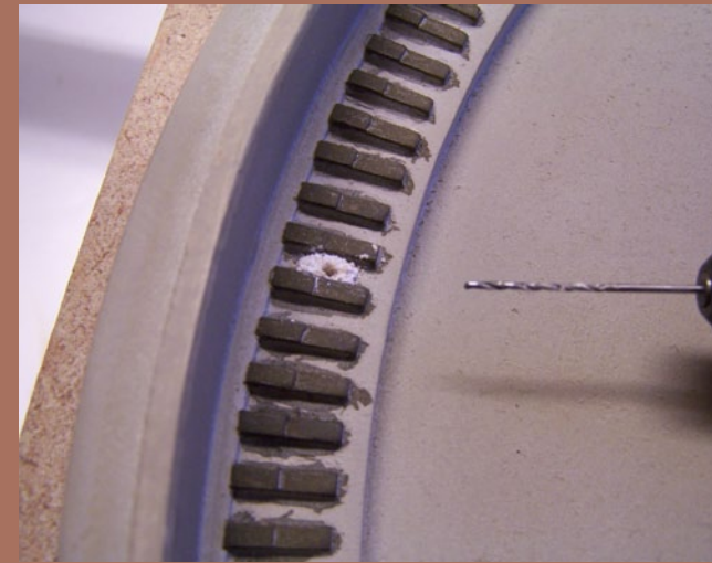
Figure 45: Drill hole in pit for wire.
