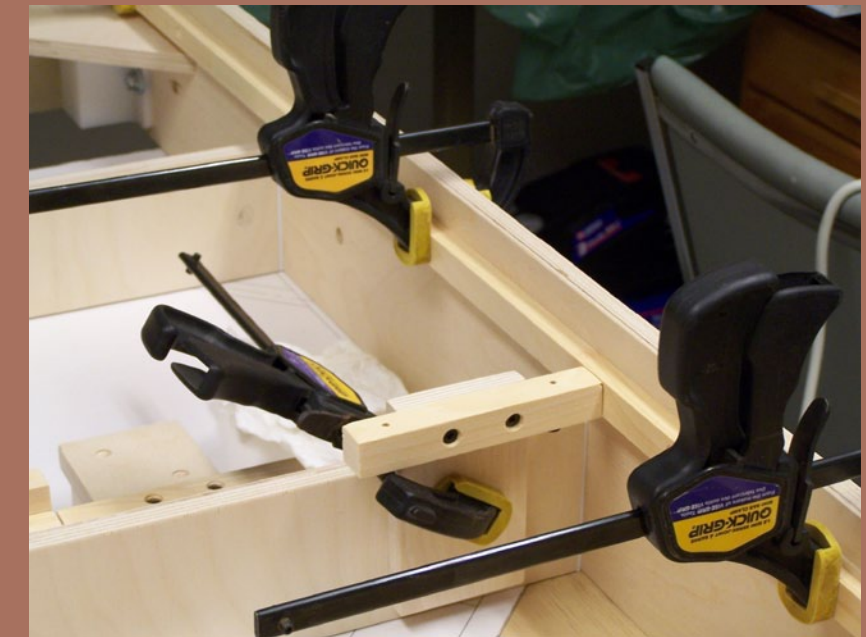
Figure 26: Cleats installed around the inside perimeter of the module.
