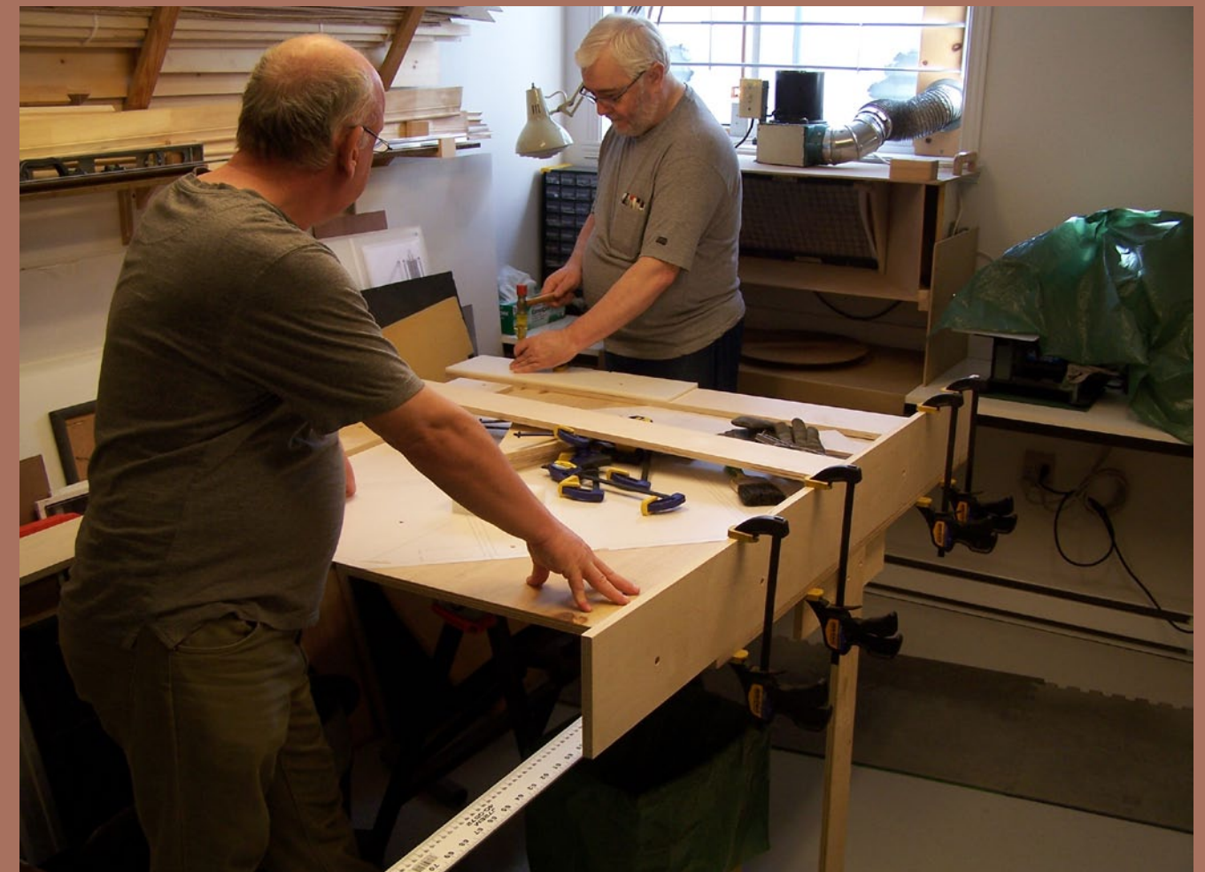
Figure 12: Using template to mark drill holes. Ray Assellin is holding the table steady.
