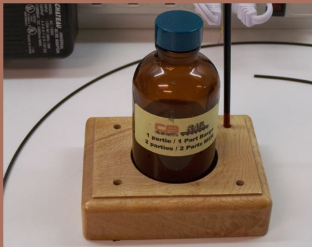
Figure 47: Barge cement and MEK mixture
