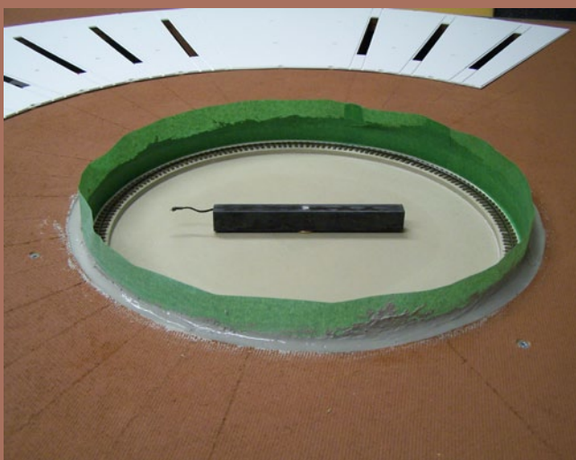
Figure 87: Latex caulk added around pit.
