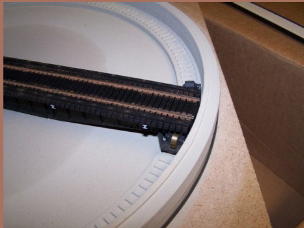
Figure 62: The other rail is wired to both trucks
