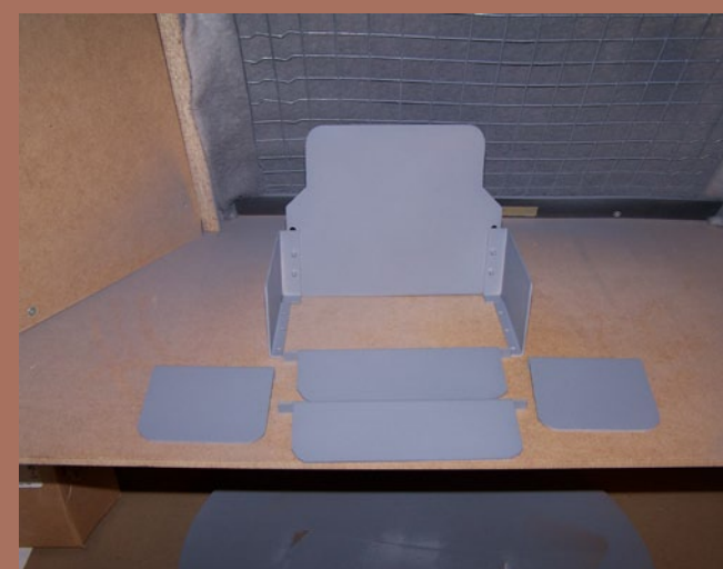
Figure 92: Primed support brackets & protective plates.
