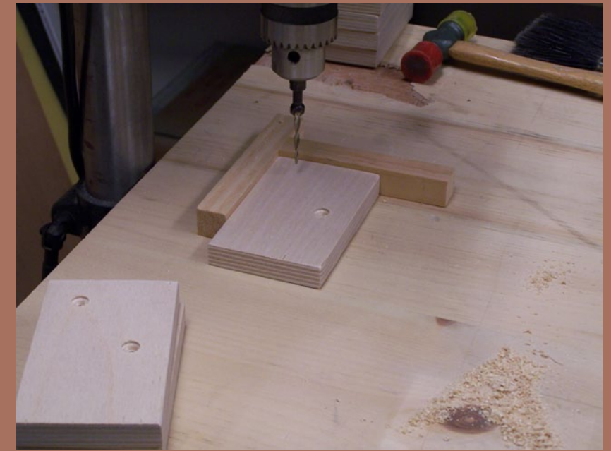
Figure 23: Pre-drilling the risers.
