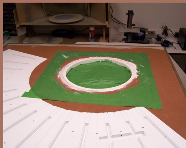
Figure 88: Hydrocal and tape for later sanding.
