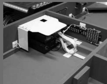
Figure 93: PTC III and APR mounted with Velcro inverted view with protective cover installed.
