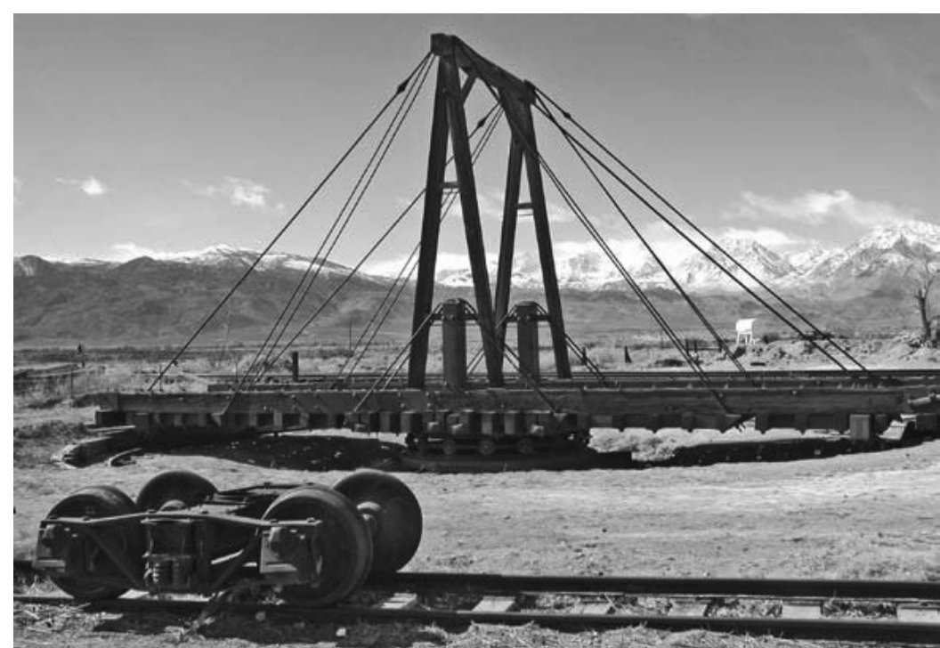
Figure 8: "Gallows"-style turntables turned the diminutive engines at Laws and Owenyo. The Laws Railroad Museum and Historic Site has preserved the turntable on-site, shown here with the snow-capped Sierras for a background. Courtesy, Laws Railroad Museum and Historic Site.
