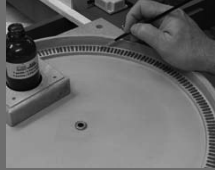
Figure 49: Apply mixture to ties.
