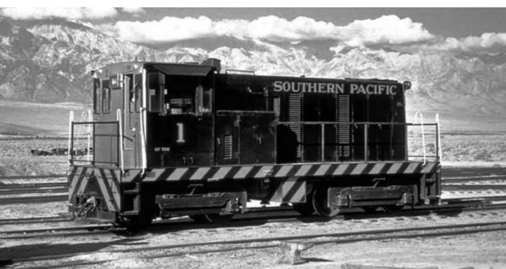
Figure 13: The beginning of the end for steam was the arrival of General Electric-built #1, dubbed the "Little Giant", in October 1954. In this as-delivered view, the 51-ton diesel wears a version of the S.P.'s then-current switcher livery. Rich Yoder Models is planning to release a model of SP narrow gauge #1 in On30 and On3: http://www.richyodermodels.com/ . Photo courtesy, Joe Dale Morris Collection.
