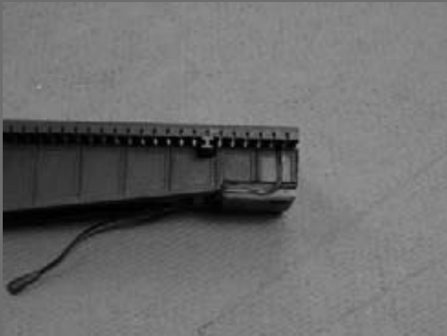
Figure 60: Bridge soldered other end of mini-connector to one rail.
