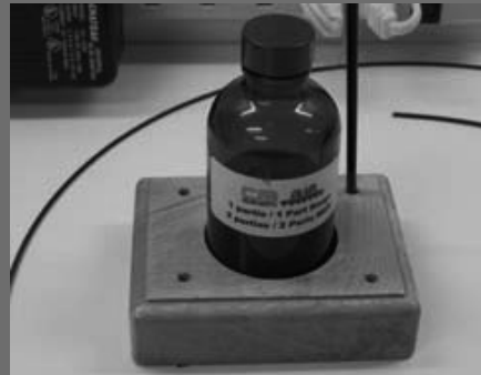
Figure 47: Barge cement and MEK mixture
