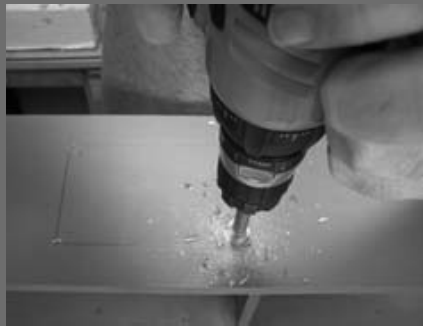
Figure 33: Used a Forstner drill bit .
