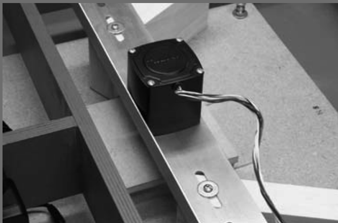
Figure 81: Stepper motor installed.
