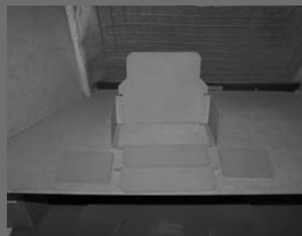
Figure 92: Primed support brackets & protective plates.
