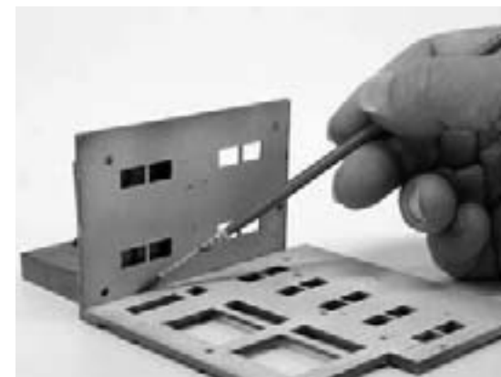
Figure 2: Using a brush to apply the liquid cement to an inside joint of a plastic building wall.
