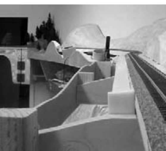
Figure 3: Charlie Comstock attaches his 3/16" masonite fascia to cleats at the end of the benchwork joists.
