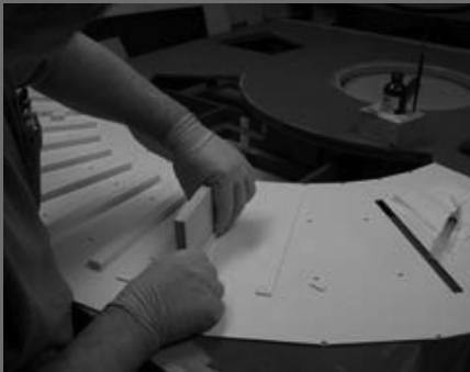
Figure 71: Assembling pit bottoms.
