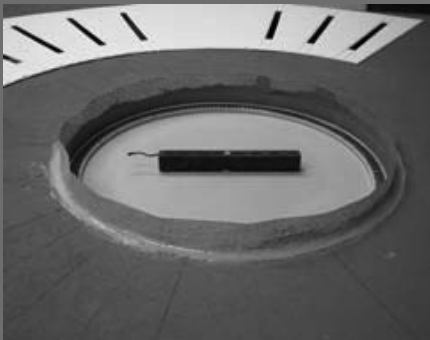
Figure 87: Latex caulk added around pit.
