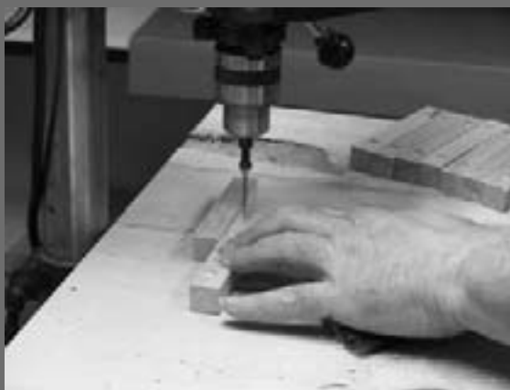
Figure 21: Pre-drilling the cleats.
