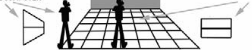
Figure 21: Keystone can also happen if you stand off-center from your subject, so try to position yourself directly in front of each window.
