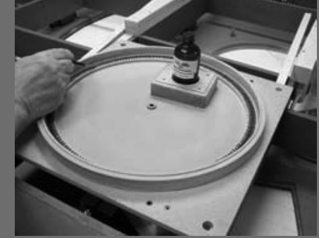
Figure 50: Install rails and add a generous dose of MEK.
