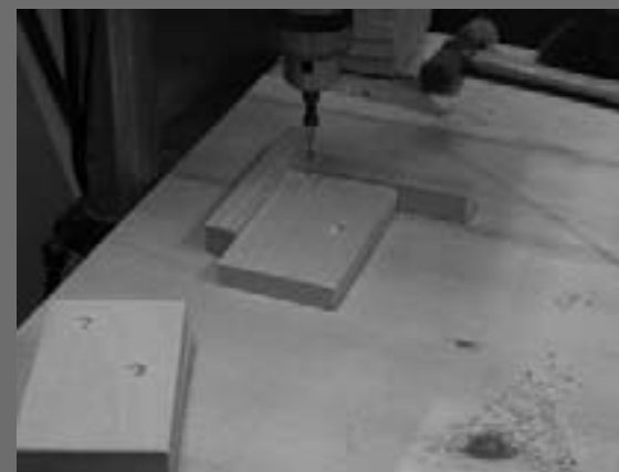
Figure 23: Pre-drilling the risers.
