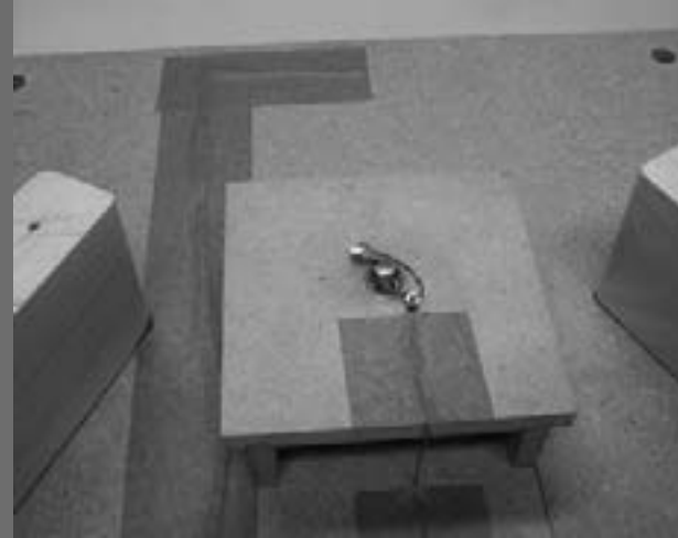
Figure 60: Bridge soldered other end of mini-connector to one rail.
