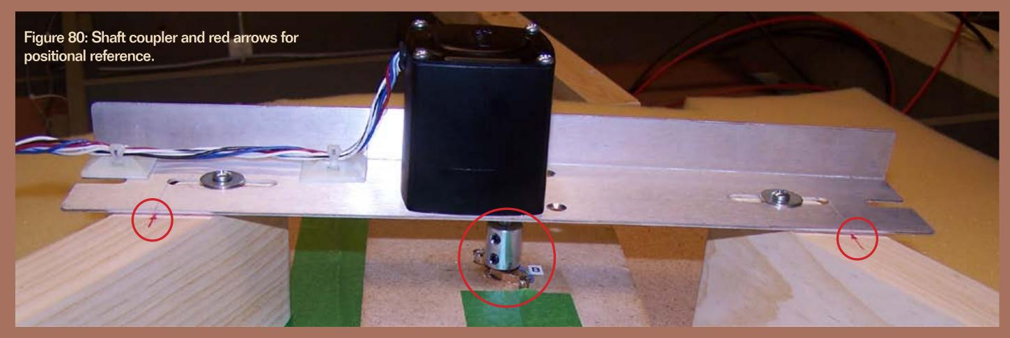
The turntable shaft is secured to the stepper motor via a bushing supplied by NYRS. It has two set screws. I attached the shaft to the stepper motor and measured the amount I had to cut off as shown by the arrows on Figure 82. I used a hack saw to cut the shaft to length and I ground a flat spot on
