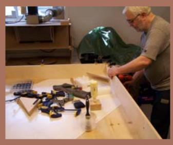
Figure 13: Assembling sideframe and gusset.
