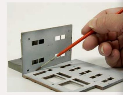
Figure 2: Using a brush to apply the liquid cement to an inside joint of a plastic building wall.
