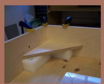
Figure 14: Gussets glued and screwed.
