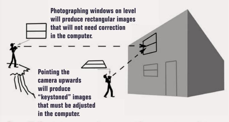
Figure 20: Keystoning occurs when you point the camera at an angle to photograph objects. Try to shoot with your camera level where possible.
