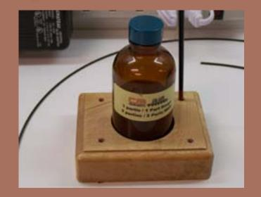
Figure 47: Barge cement and MEK mixture
