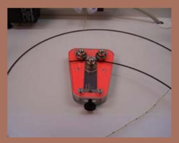
Figure 43: Fast Tracks Rail Bender.
