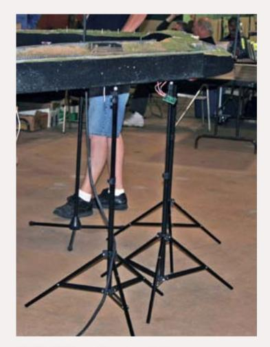
FIGURE 1: Each of the photographer's light stands (black legs) is supporting a module that is leveled along the rail and across the track. The white legs in the background are of a bipod module support that is only temporary and not nearly as strong.
