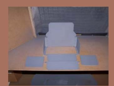
Figure 92: Primed support brackets & protective plates.
