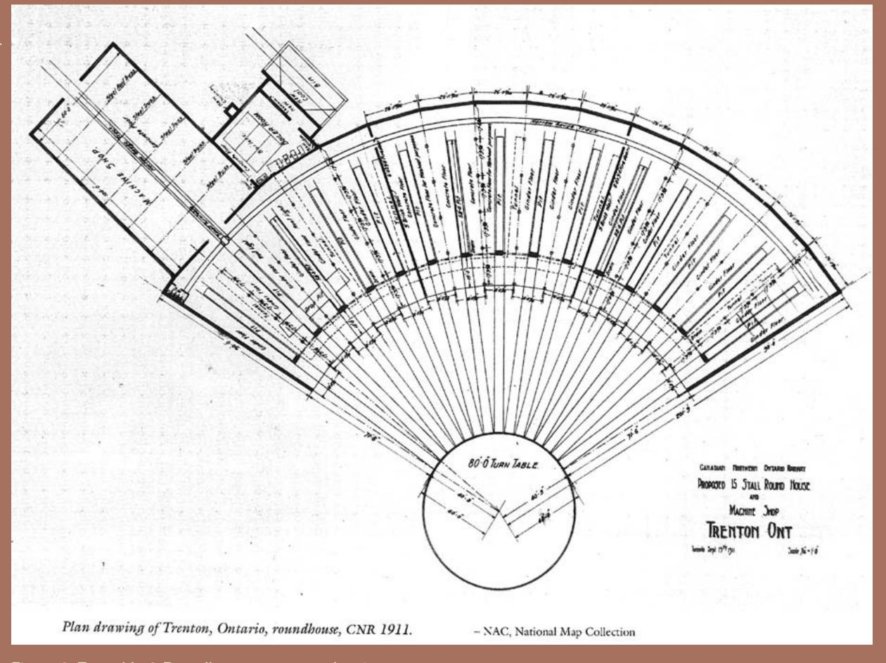
Figure 2: Turntable & Roundhouse prototype drawing.
