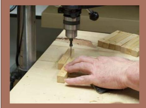
Figure 21: Pre-drilling the cleats.
