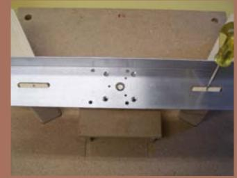
Figure 78: Centering mounting bracket.
