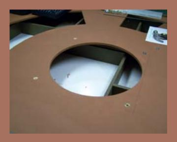
Figure 84: Positioning Tee Nuts from top of module.
