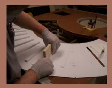
Figure 71: Assembling pit bottoms.
