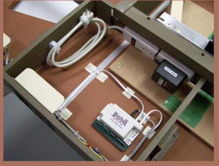
Figure 9: Electrical, DCC and electronic parts.
