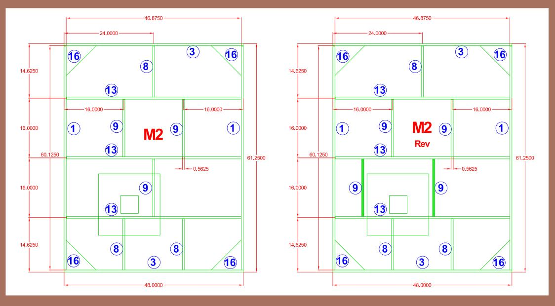
Figure 10: Module frame drawing – note the pieces moved in M2 Rev. Circled numbers are itemized Russian Plywood (furniture grade) framing parts of the module.
