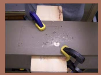
Figure 34: Used a backplate to help get a clean cut.
