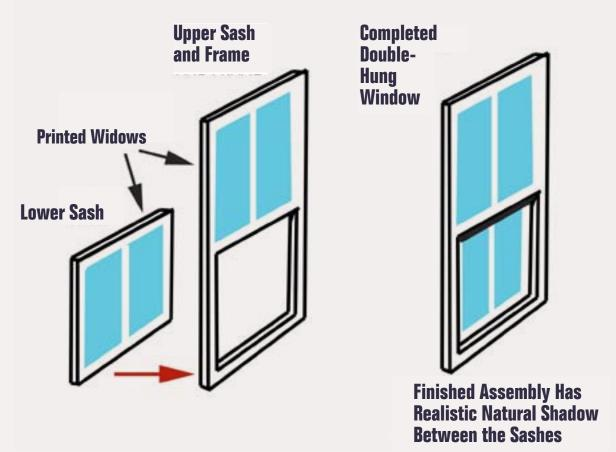
Figure 13: You can improve photo windows by recessing the lower panels of double-hung windows. Just glue the lower pane behind the upper one after mounting on .030" or thicker material. Framing-out the lower panel will give a very realistic effect.
