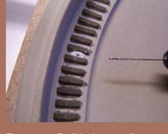
Figure 45: Drill hole in pit for wire.
