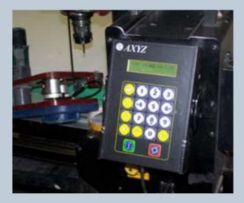
Figure 65: Router programming terminal.
