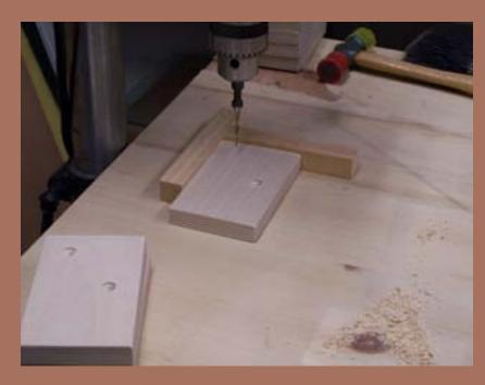
Figure 23: Pre-drilling the risers.
