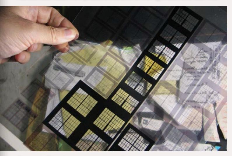
Figure 15: This photo shows graphically how dark-brown and dark-grey colors both transmit images right through them, leaving black window frames as the only realistic alternative.
