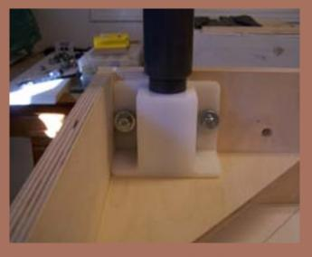
Figure 18: Plastic (UHMW) leg sockets.
