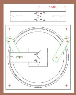
Figure 75: Detail drawing of motor assembly on base.
