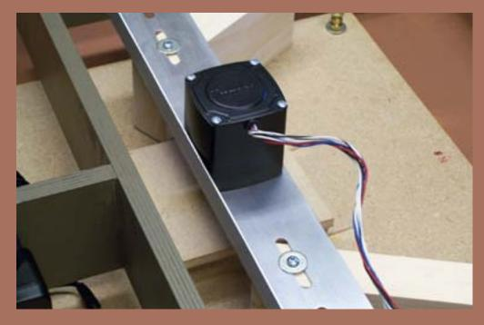
Figure 81: Stepper motor installed.
