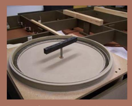
Figure 41: Center shaft with bridge base.
