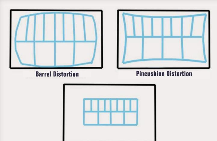
Distortion is minimized closer to the center of the viewfinder frame.
