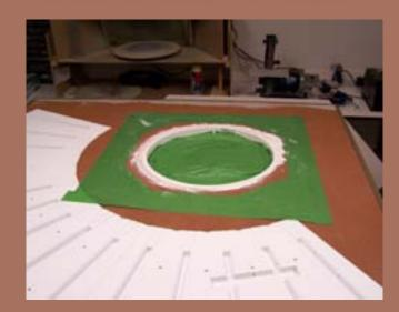
Figure 88: Hydrocal and tape for later sanding.
