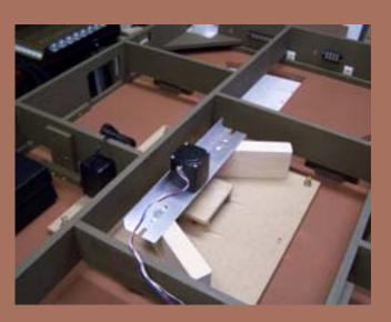
Figure 86: Turntable and motor assembly in place.
