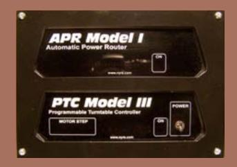
Figure 95: Fabricated faceplate.
