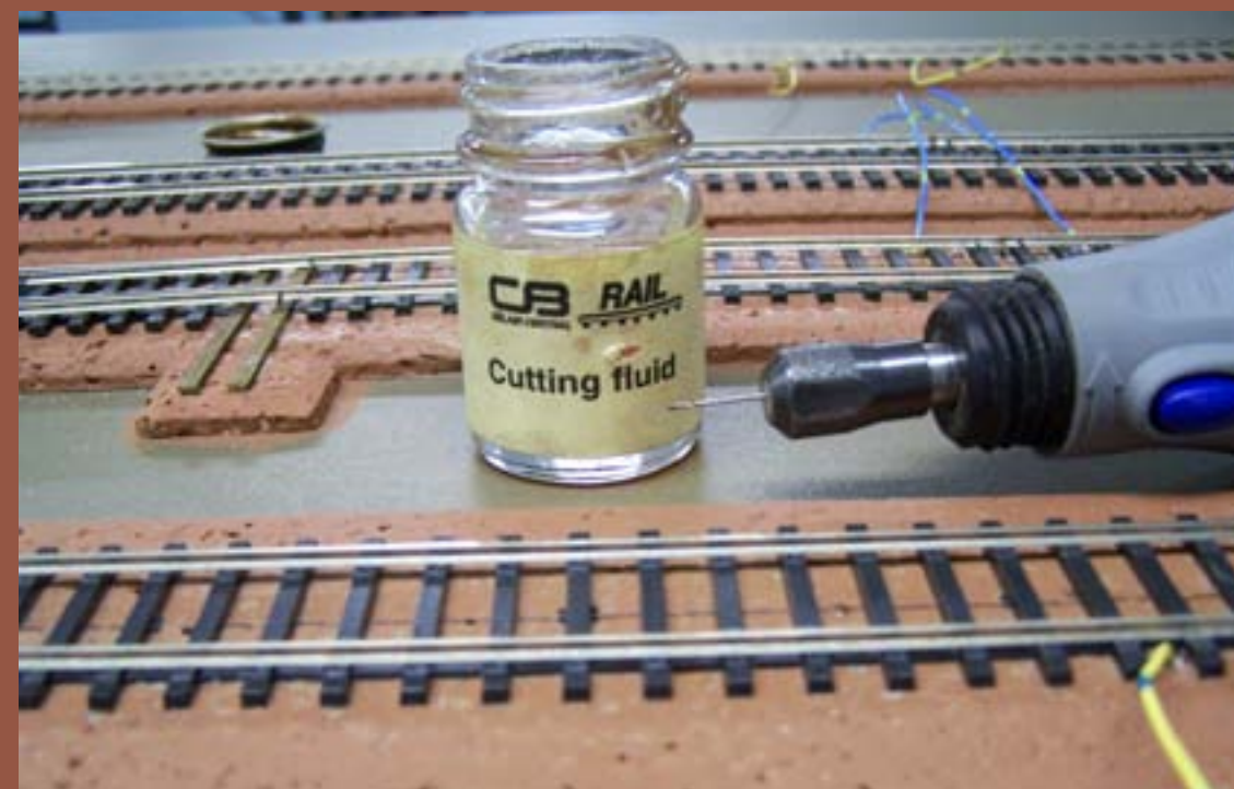
Figure 78: I measured the bare copper feeder wire and chose a # 72 drill.
