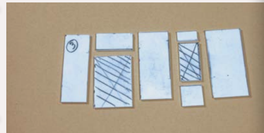
FIGURE 9: Discard the areas where windows and doors are going to be installed and then reassemble the walls. Here’s one of the walls showing the individual segments before the subwall has been reassembled.
