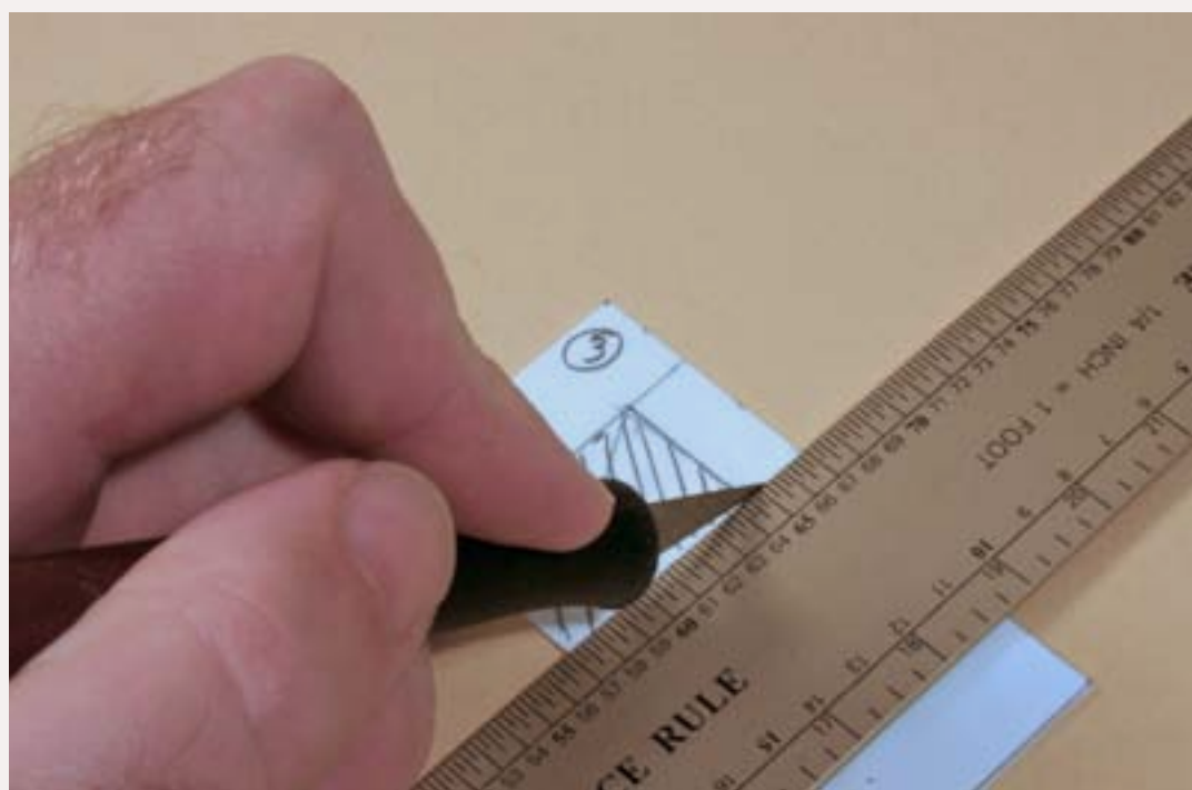
FIGURE 7: Using a sharp no. 11 blade and steel rule I scribed along the guidelines. The idea is to break the wall apart, remove the sections (with the cross-hatch marks) for the window and door openings, and then reassemble the wall pieces.
