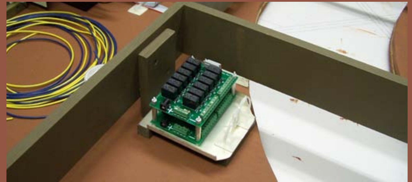
Figure 18: The APR (Automatic Power Router) 24 relays control turns power on or off according to bridge position for approach, storage and stall tracks.
