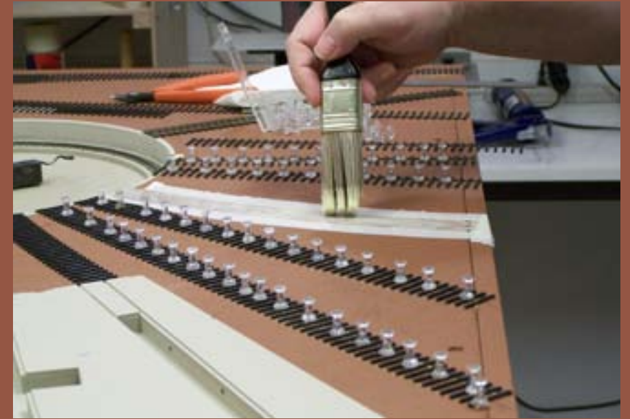
Figure 48: Apply a liberal amount of LePage yellow glue and smooth out with a brush.
