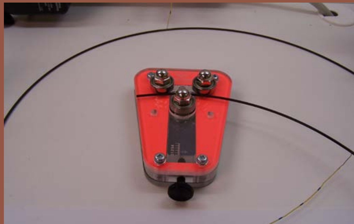
Figure 29: Bending the iron with the Fast Tracks rail bender.
