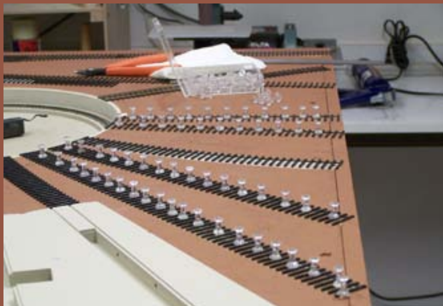
Figure 49: Remove masking tape and replace tie strip on centerline.
