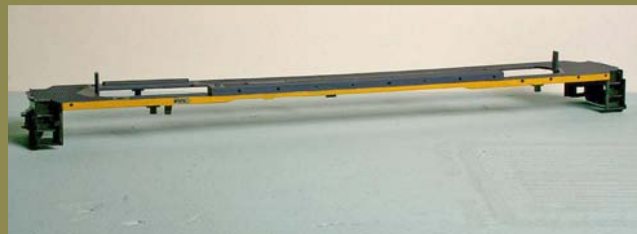
Figure 11: Sill stripe after full application of decals and touch-up paint.
