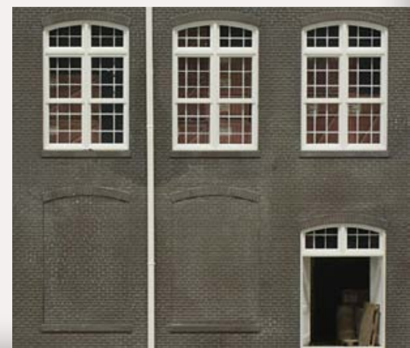
FIGURE 4: Ink jet 'crates' behind the windows hide the hollow interior of the building from view.
