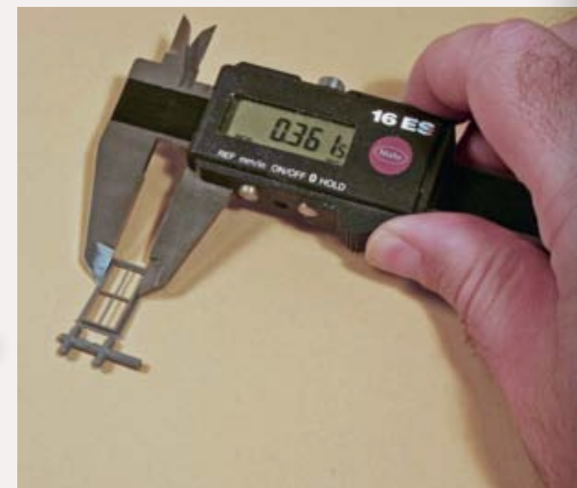
FIGURE 5: To determine the size of the window and door openings, I measured the castings with a caliper. Since this particular window is made for a frame building, I mounted it from the inside of the building (masonry structures don't have visible window frames on the exterior) and inverted the window so the upper sash is beyond the lower sash.
