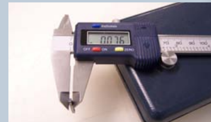
Figure B. CV mainline tie is the thickest.
