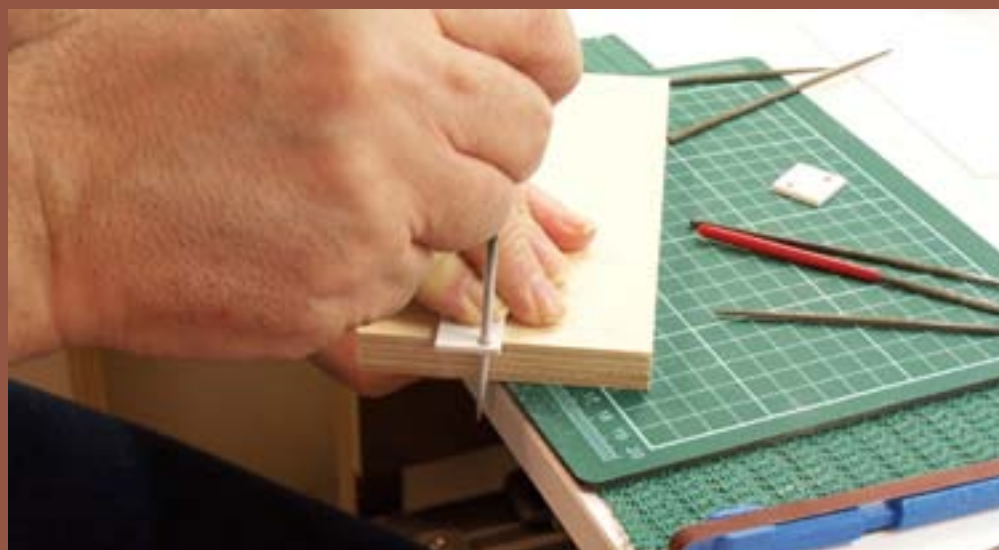
Figure 62: I prepared the styrene shims by using several thicknesses to get the right height.
