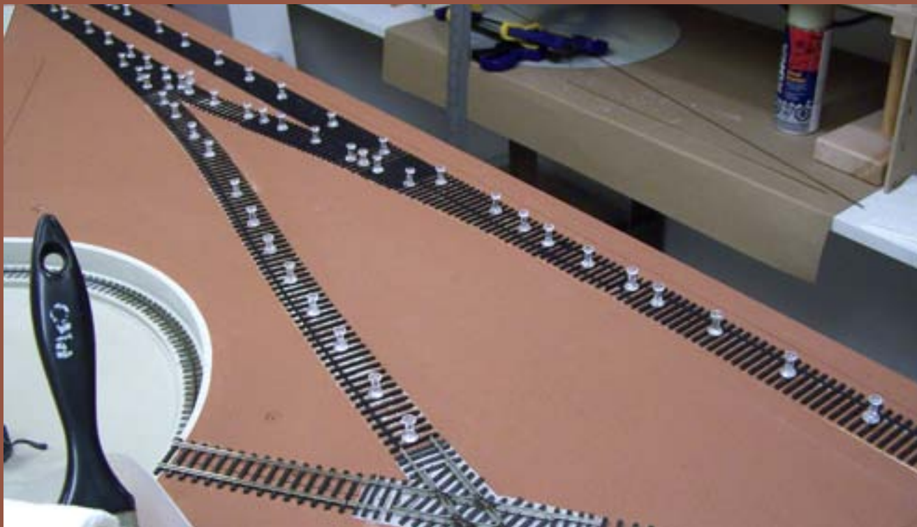
Figure 44: Masking tape removed – the tie strips remain pinned down while waiting for glue to dry.
