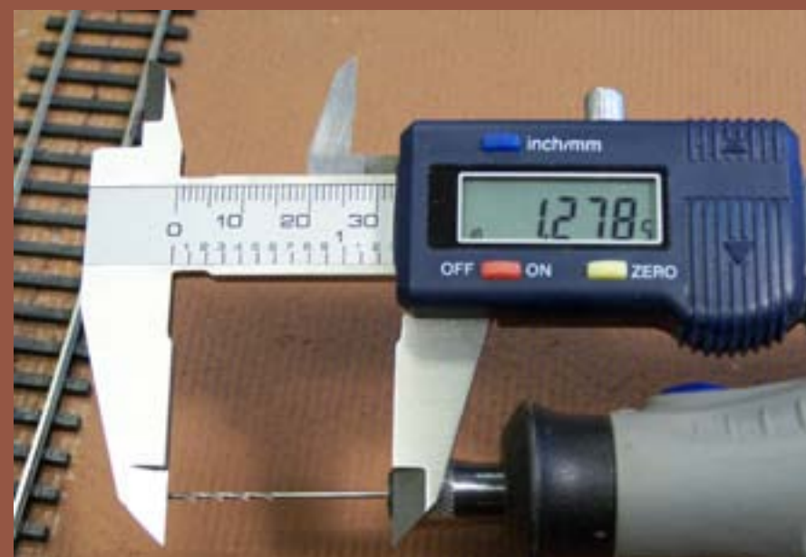
Figure 75: I made sure to adjust the length of the drill to penetrate my 1" thick subroadbed and roadbed.
