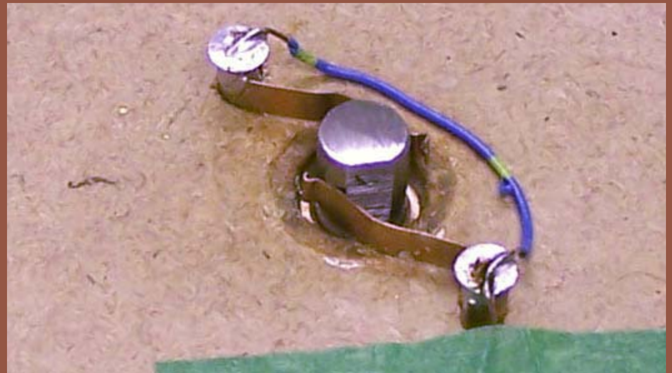
Figure 11: I soldered two 1/4" strips of phosphor bronze to two brass screws and bent them to act as wipers on the turntable shaft which I will use to power rail B of the bridge. I also soldered a wire between the two screws as insurance for a constant wiping action. I adjusted the tension on the phosphor bronze wipers by turning the screws and then added a drop of ACC to the bottom of each screw to secure them in place.
