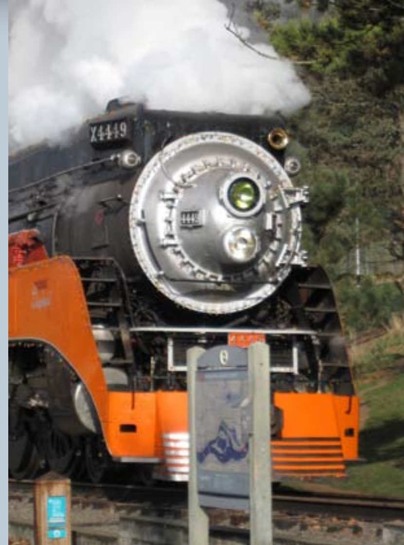
Figure 9: This photo was taken on December 13, 2009 while the 4449 was running a Holiday Express Train which is a fund raiser for the Oregon rail Heritage Foundation. Notice the Mars light is the as-delivered globe instead of the twin sealed-beam. Photo by Brandon Thompson.
