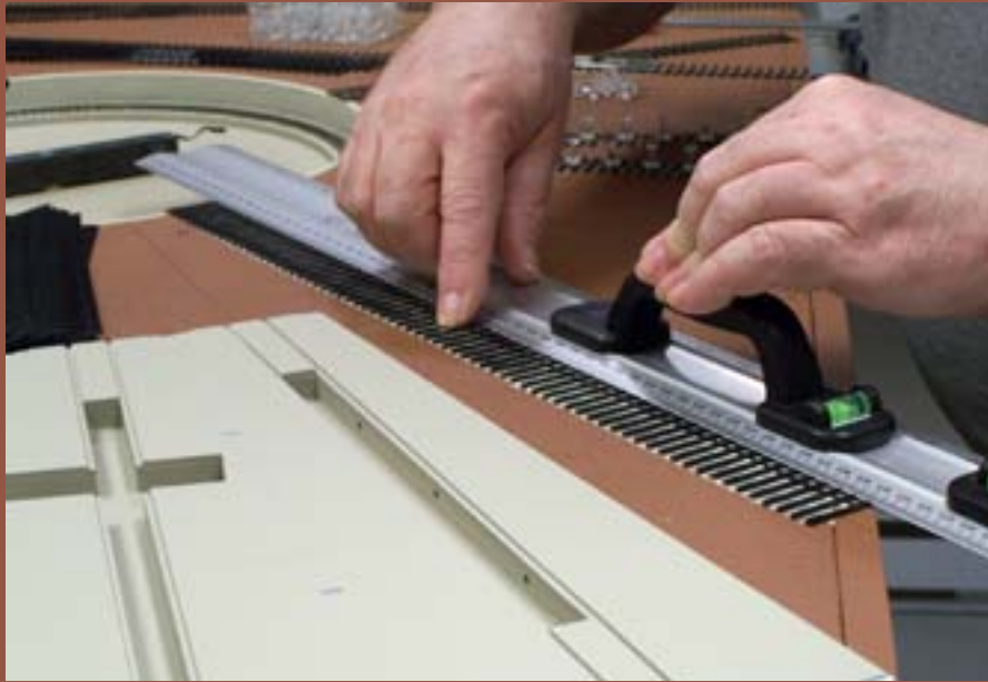
Figure 46: Use a straight edge to line up ties.
