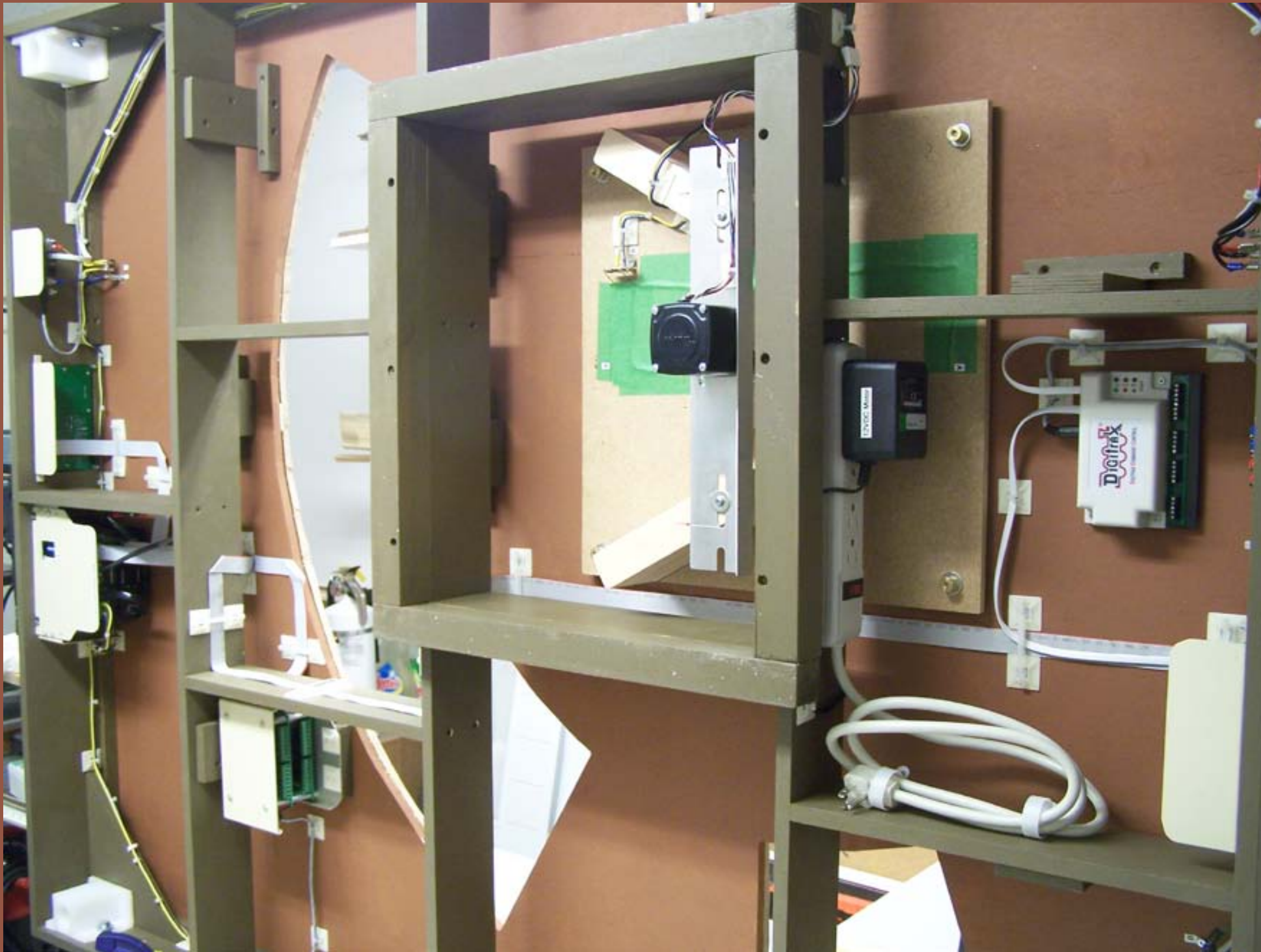
Figure 16: This is the final resting place of the turntable assembly. Due to the height of the stepper motor exceeding the 6" clearance available on the module, I had to add 2 by 2 pine shims all around it for protection.
