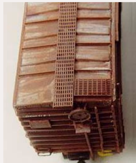
FIGURE 11: Model Memories ( www.modelmemories.com ) has see-through etched-brass roofwalks (AKA running bars) as replacements for out-of-scale molded plastic roofwalks. The HO scale roofwalks come in 2-packs and are available for 40-foot and 50-foot cars. They may be purchased direct through the above web site.
