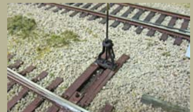
Figure 14: Switch stand minus the target.
