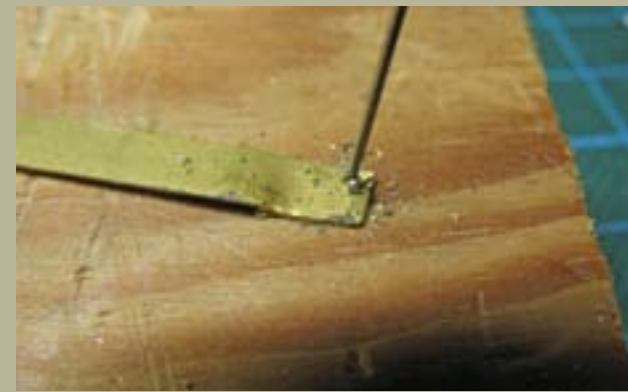
Figure 3: Drilling the #76 hole in the brass strip.
