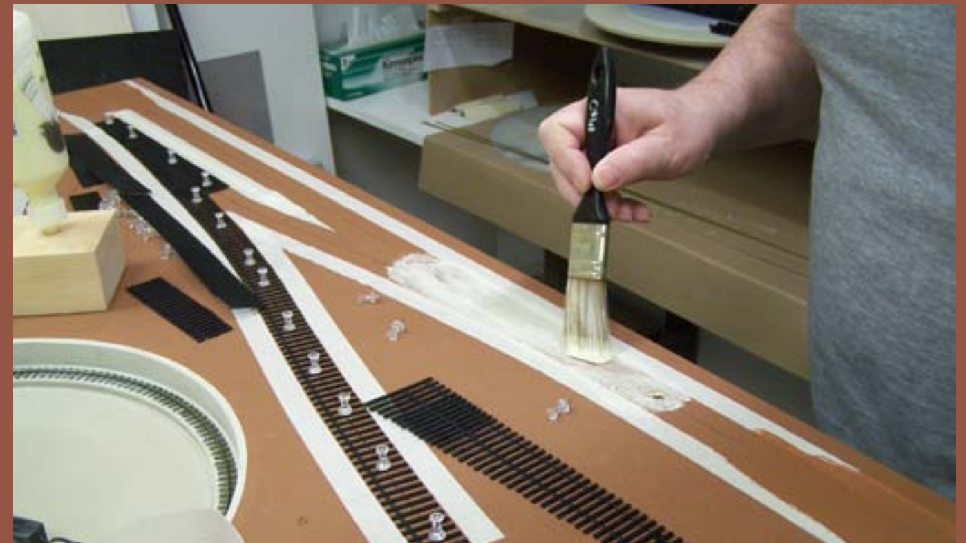
Figure 42: Spreading the glue evenly using a brush.
