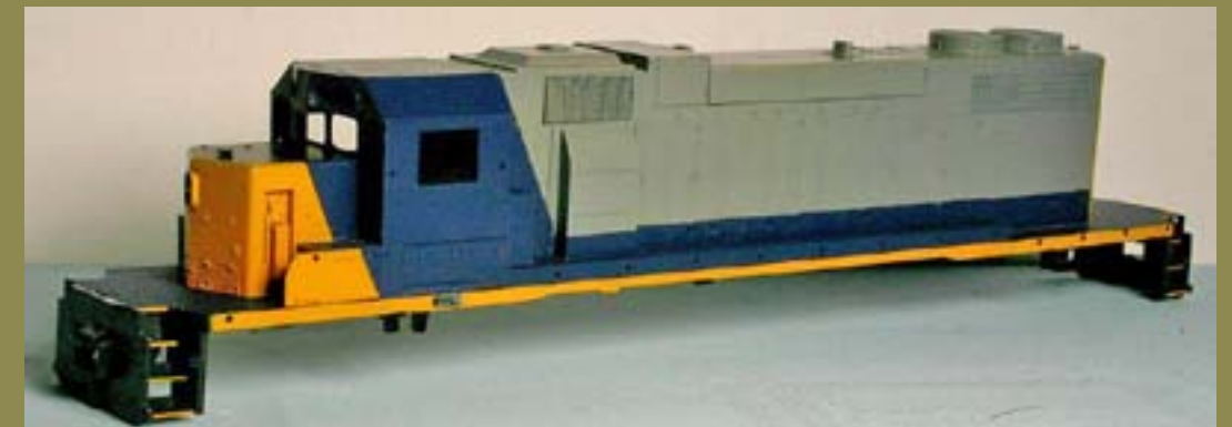
Figure 19: Painted body shell after gloss covering.
