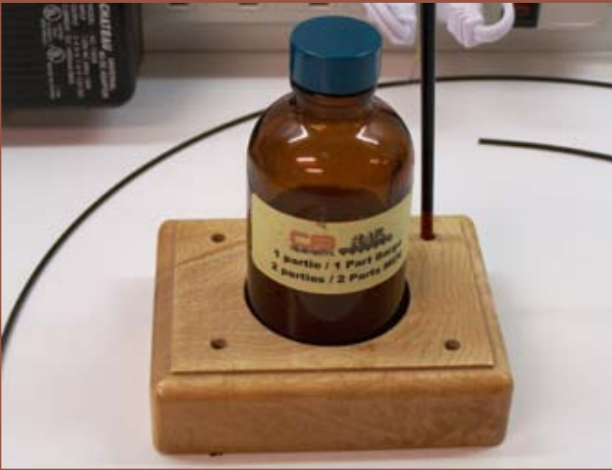
Figure 30: Barge Cement and MEK mixture in spill proof base.
