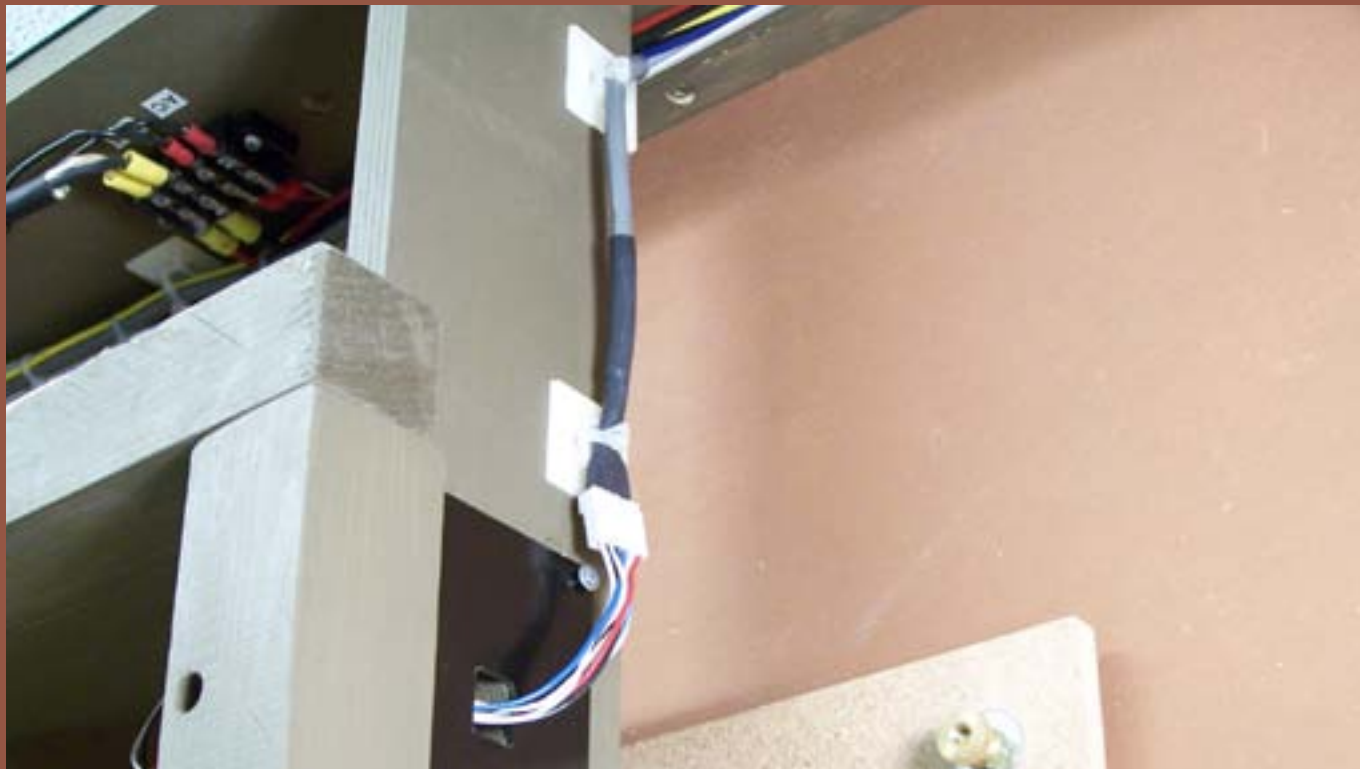
Figure 6: I used the NYRS 6' plug-in extension cable here. Don't try to "roll your own" extension, it just doesn't work, trust me!
