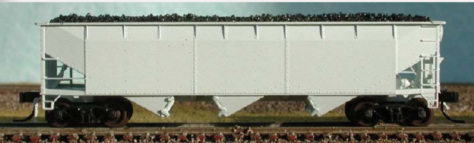
FIGURE 2: Here is an early look at an undecorated engineering sample of Bluford Shops ( www.bluford-shops.com ) forthcoming 70-ton 3-bay hopper. The design of the N scale model features a central die-cast assembly that incorporates the slope sheet, hopper-bay and sill assembly. The sides, ends, hopper doors, brake tank, valve and air lines and slope sheet braces are injection molded plastic. A separately molded vertical brake-rod and lever assembly are said to be a first on any N scale open hopper. Other features on this well-engineered model include body mounted brake hose detail, a coal load, body-mounted magnetically operating couplers, and either friction bearing or roller bearing trucks as appropriate for specific road names. Scheduled for availability this spring the cars are tentatively priced at about $18 each.
