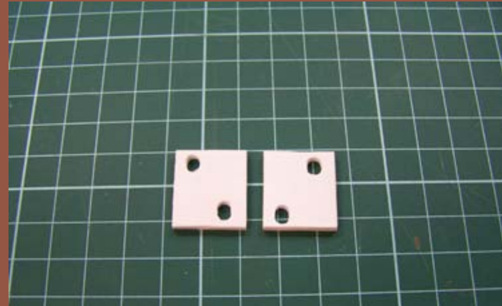
Figure 63: Laminated shims now ready for installation.
