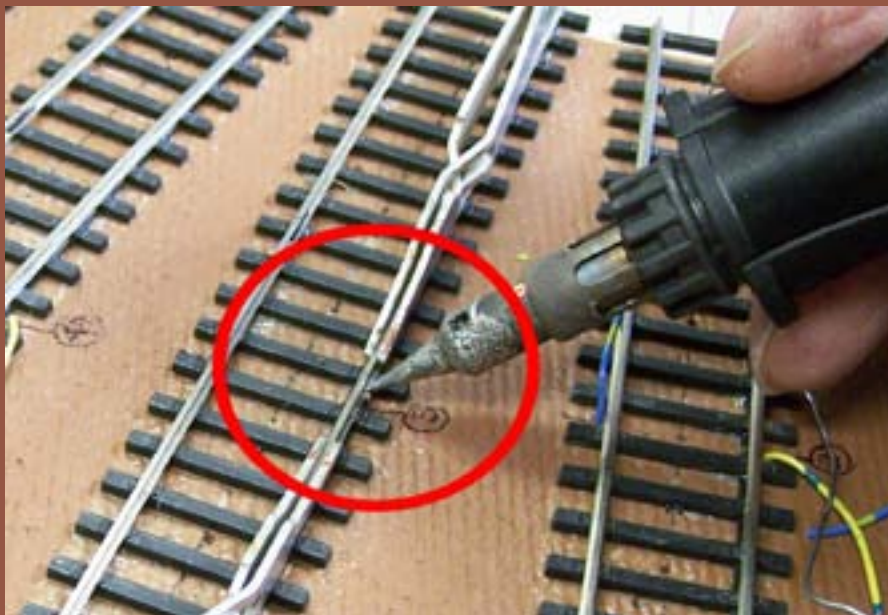
Figure 81: I used my Weller Cordless Butane soldering Iron, some heat sinks, rosin core solder and liquid flux to solder the feeder to the rail.
