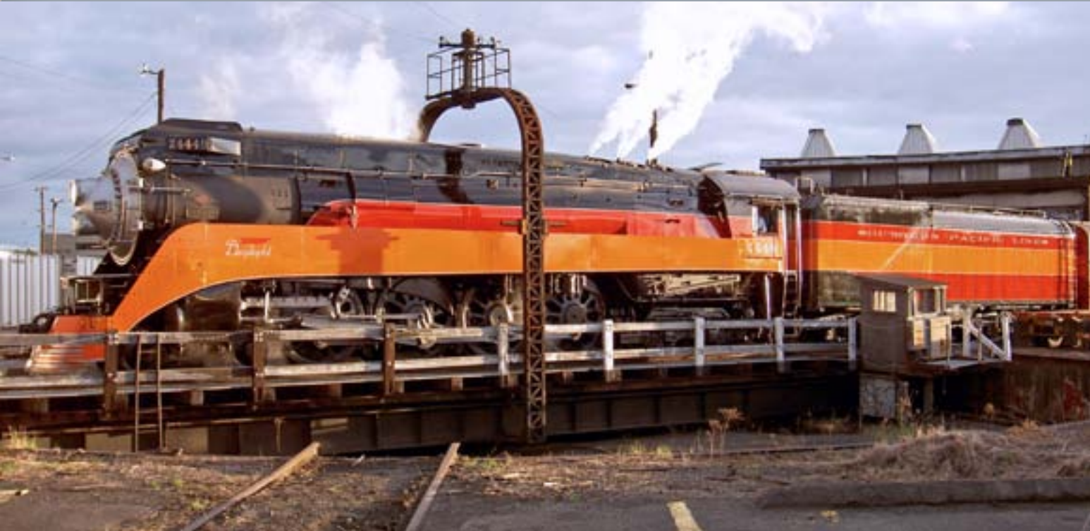
Figure 8: The 4449 on the turntable at Brooklyn Yard, in Portland on June 11, 2005 as the locomotive is preparing for a trip to Sherwood Oregon. Notice the small pre-1946 lettering and that the number boards have been moved from about halfway down the skyline to the front. This gave the locomotive an as-delivered appearance except for the improper twin sealed-beam Mars light that now has been replaced. Photo by Brandon Thompson.
