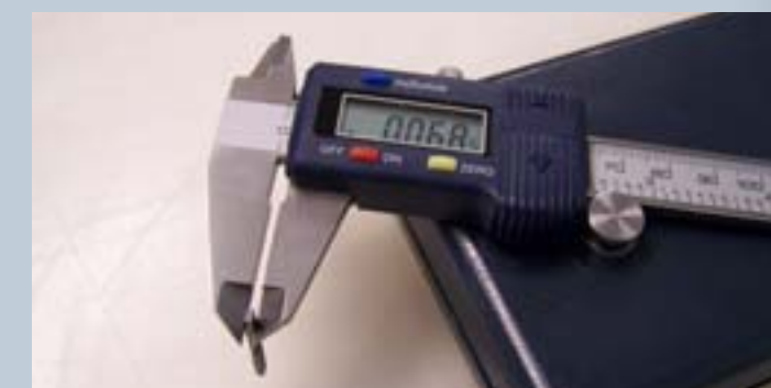
Figure C. CV siding tie is thinner.
