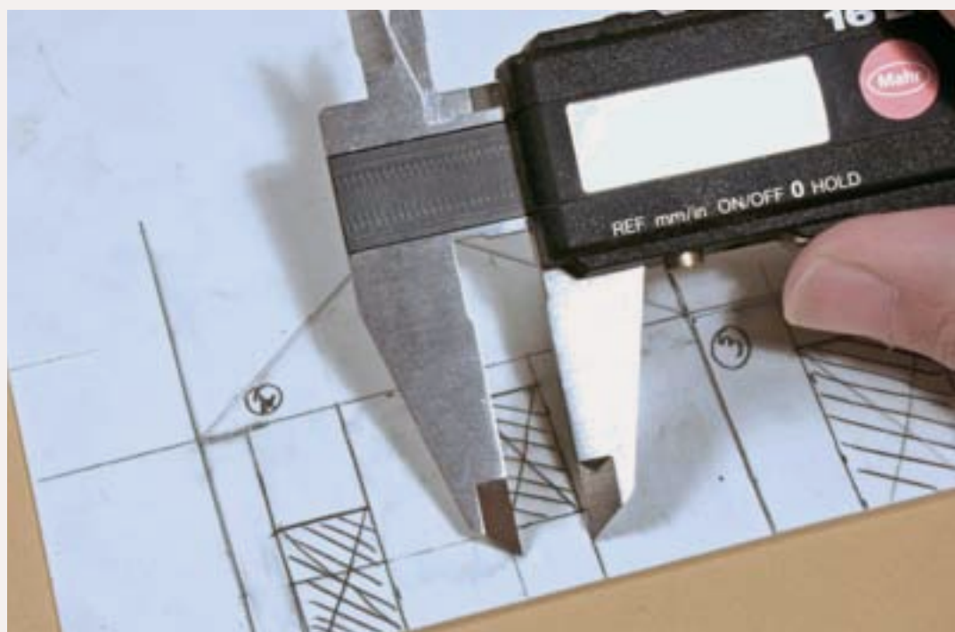
FIGURE 6: I transferred the measurement of the window casting directly to the plain styrene.
