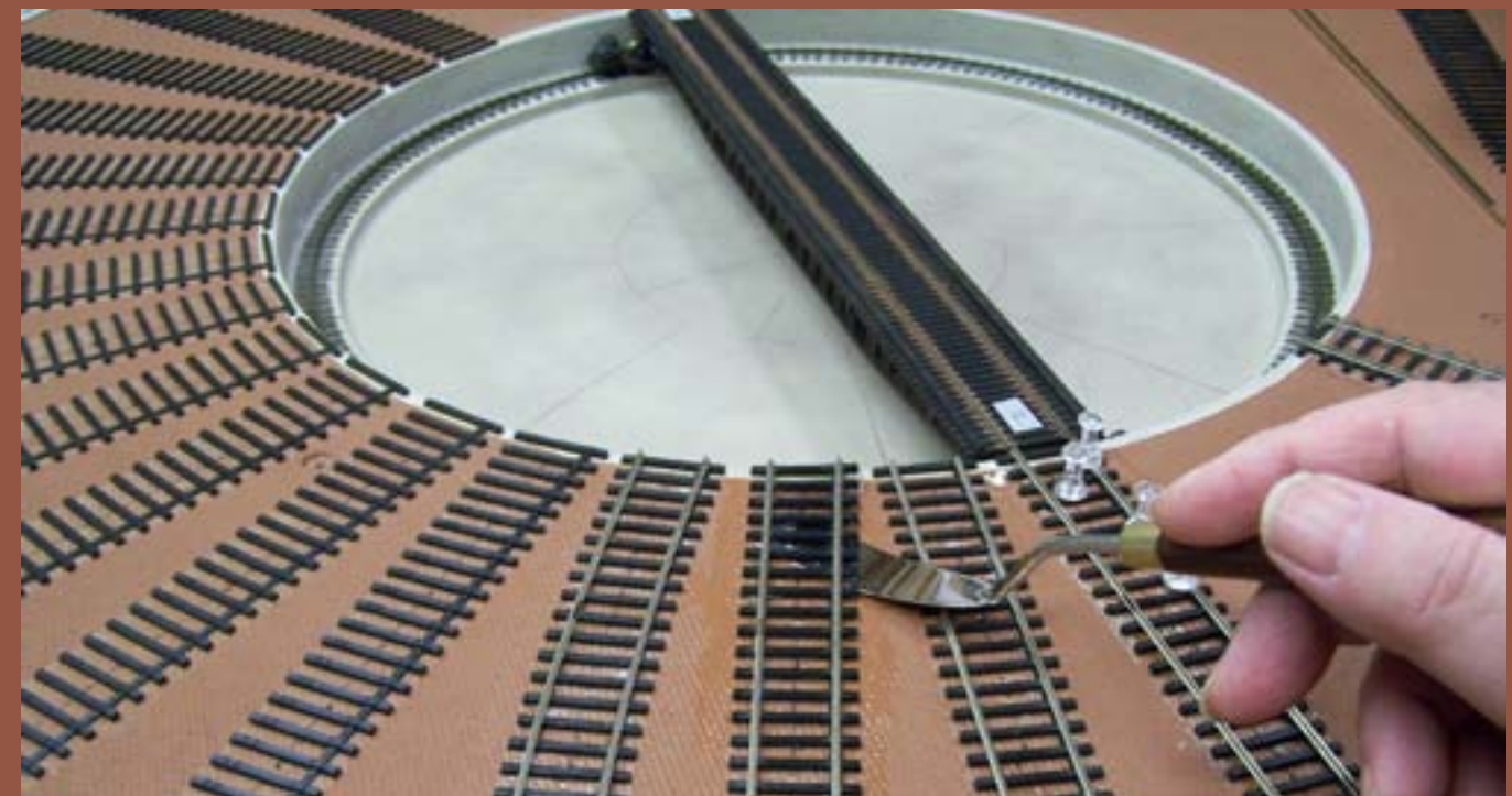
Figure 69: When the tie and rail assembly had soaked in the alcohol for about 10 minutes, lifting the whole assembly and moving it slightly was a snap.
