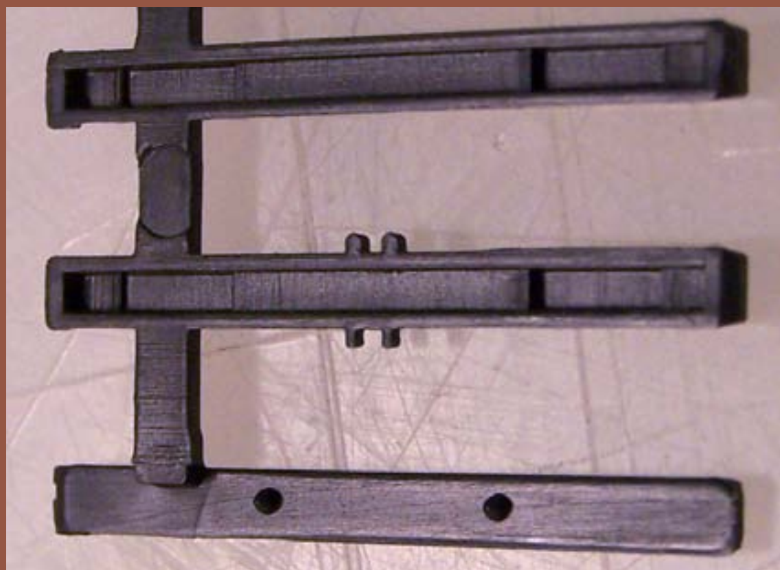
Figure 45: Bottom of CV tie strip showing hollow space.
