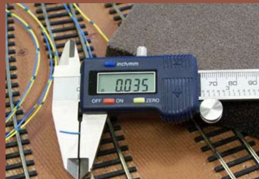
Figure 73: I measured the diameter of the feeder wires.
