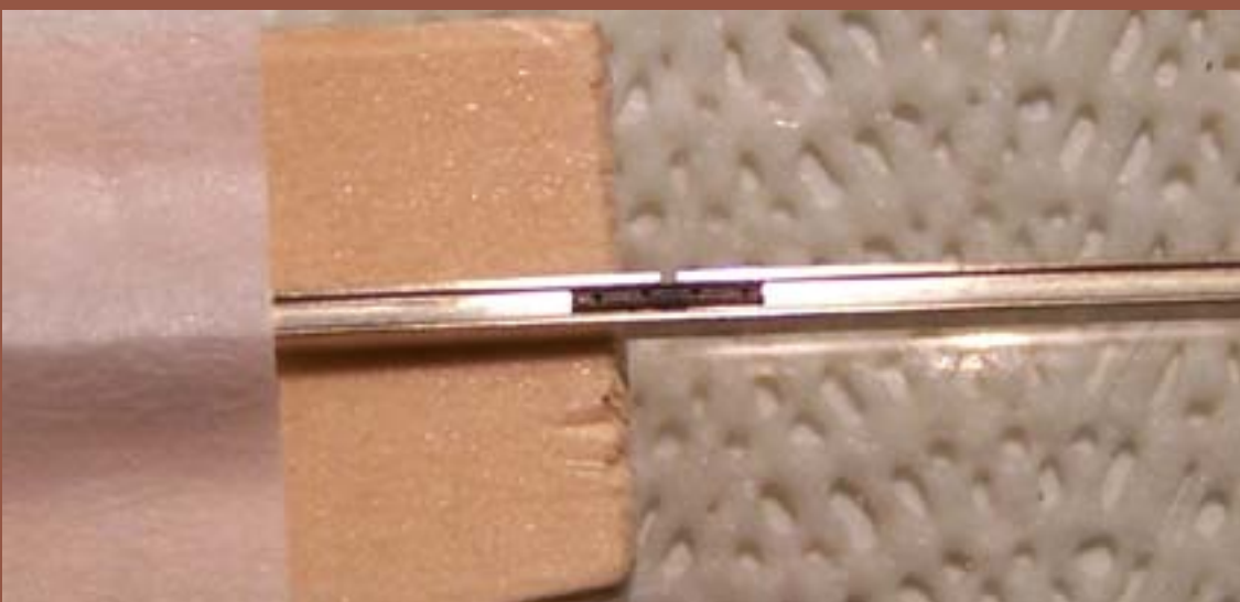
Figure 59: Rail joint bars glued at simulated rail joint.
