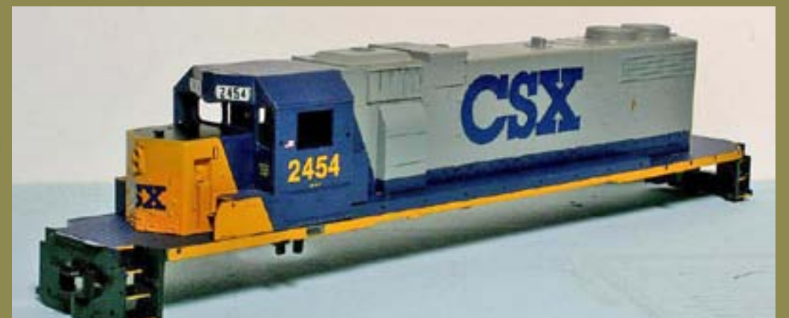
Figure 20: Body shell with Microscale decals applied.
