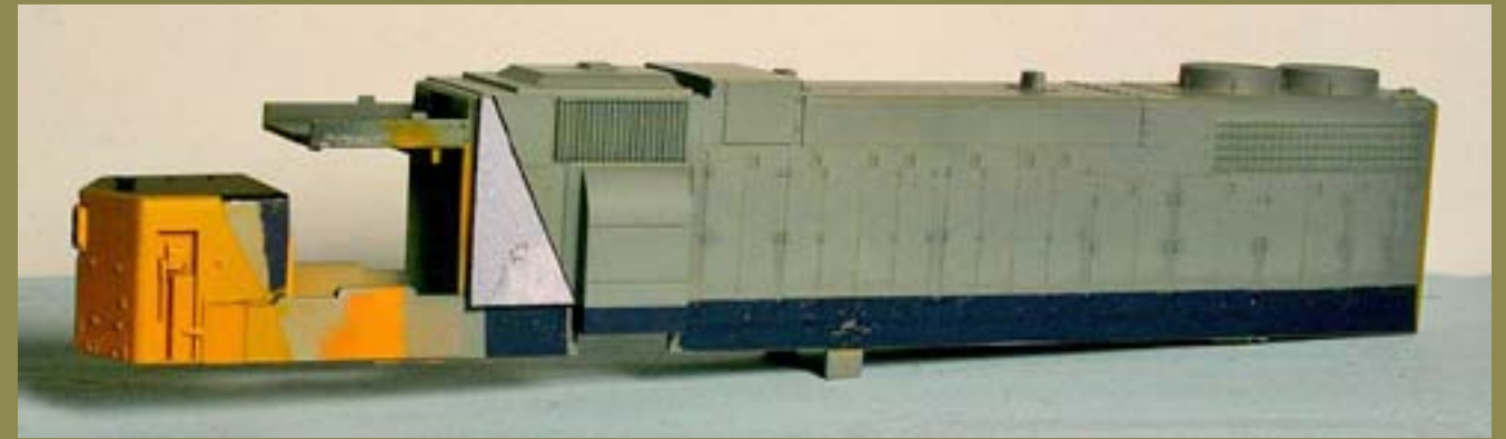
Figure 14: Marking-off a template for the angled blue section behind the cab.
