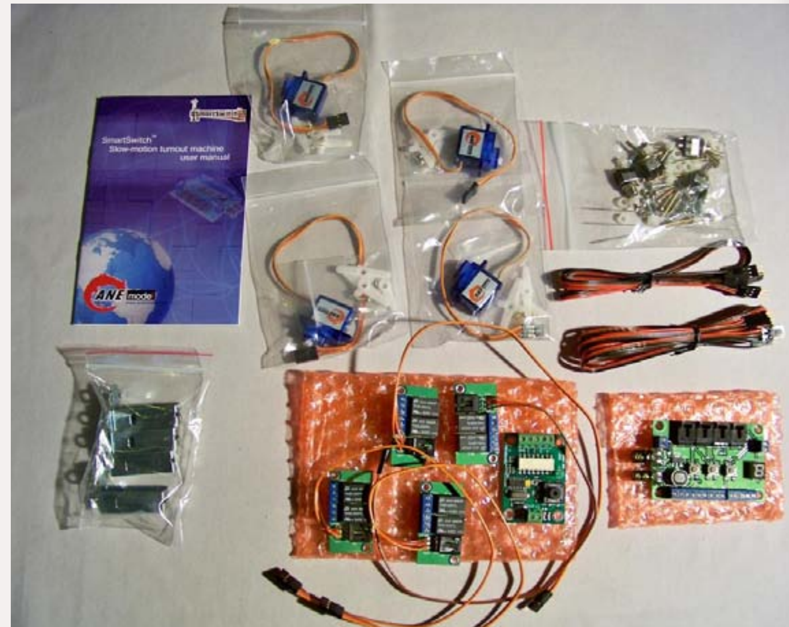
Figure 1: Contents of the A004 SmartSwitch + SmartFrog + Stationary Decoder set.
