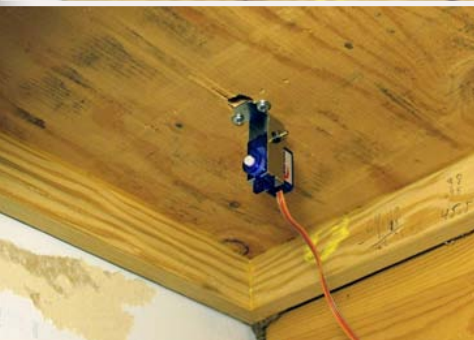
Figure 4: Servo installed in the bracket.
