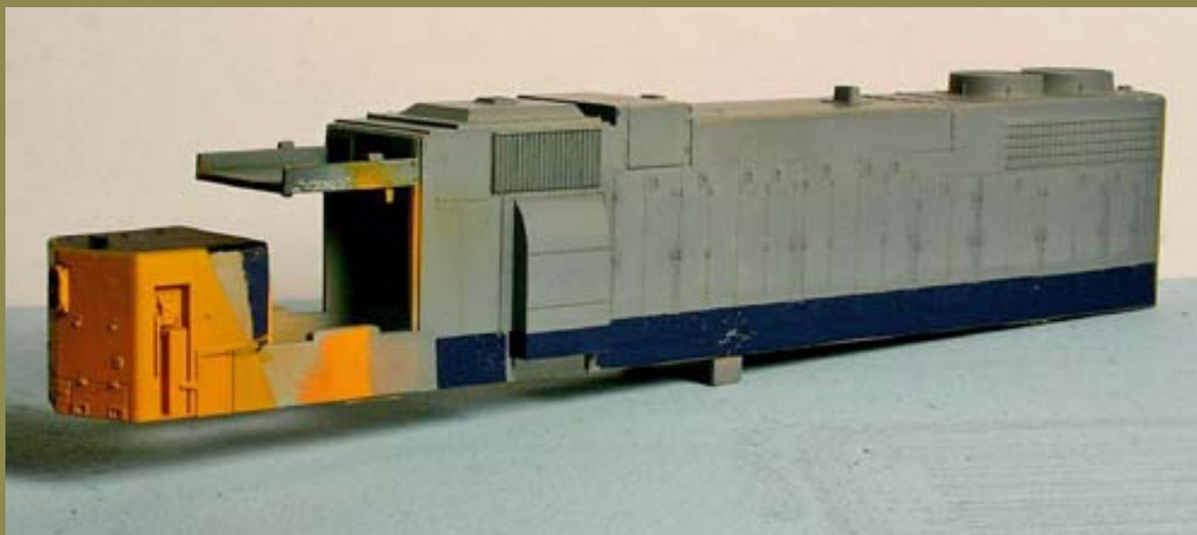
Figure 13: Left side bottom blue decal applied to long hood.
