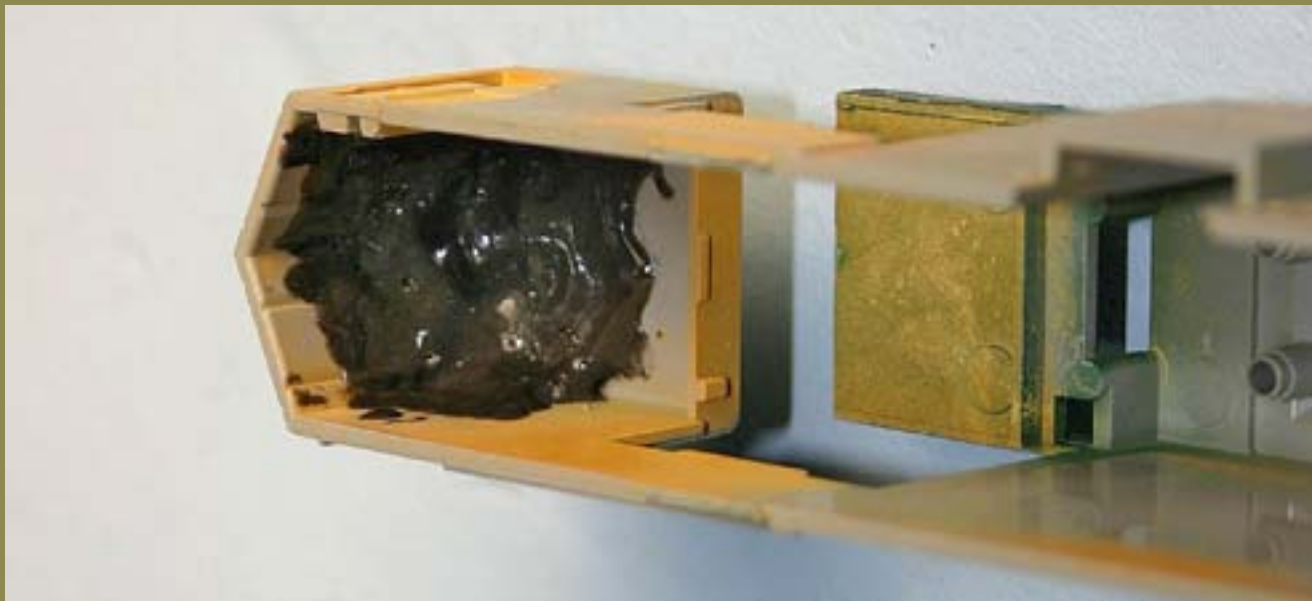
Figure 4: Steel epoxy applied to inner surface of nose section.
