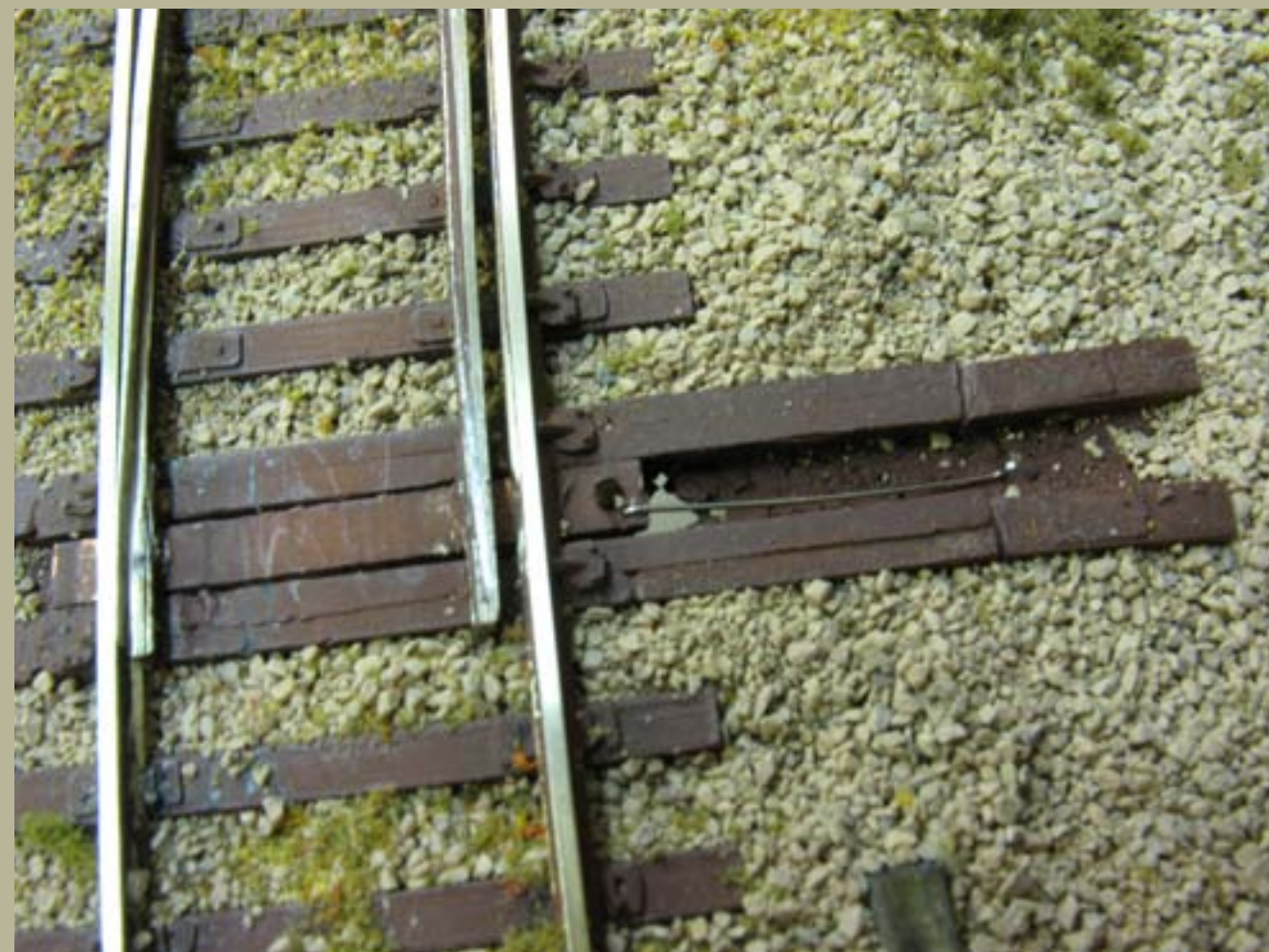
Figure 8: The steel wire from the throwbar to the switch stand.
