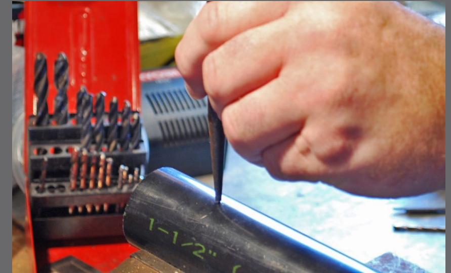
Figure 1.2: I set the cut pipe in my bench vise and used a center punch to create a centering divot to keep the drill bit from wandering.
