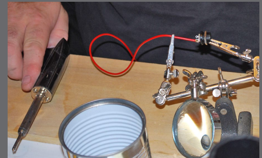
Figure 2.7: I soldered the positive lead to the jack's center terminal, the hand vise made that an easy task.
