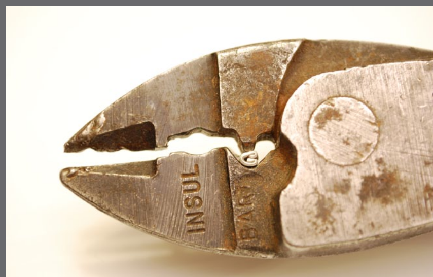
Figure 3.19a: I used the crimps to create a "pin" I could insert in the spade terminal wire end.
