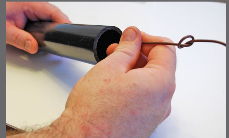
Figure 3.7a: Similarly, a knot in the scenic ground wire avoided stress being applied to wiring inside the handle.
