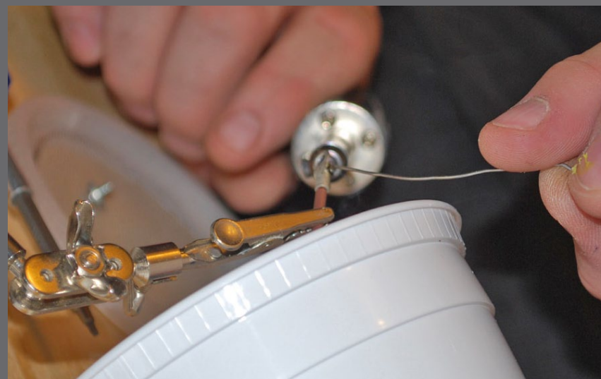
Figure 3.16: I soldered a male spade terminal onto the end of the charge wire.
