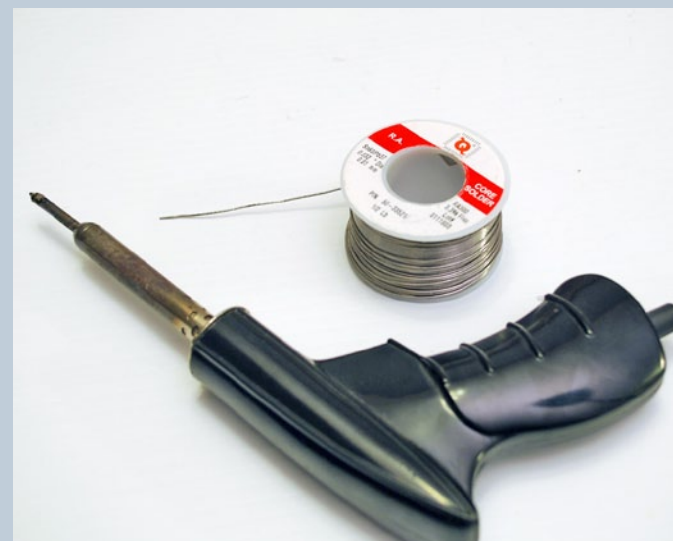
Figure A: My 35 watt iron and a roll of small diameter 63/37 lead based rosin core solder took care of the soldering for the projects.
