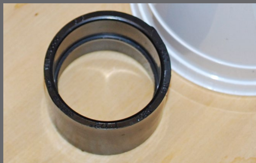
Figure 1.13: The ridge in the coupler must be removed so it will slide all the way onto the pipe.
