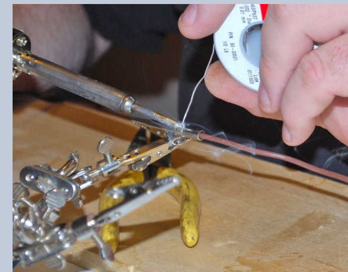
Figure F: With an iron in one hand and solder in the other, you're hard-pressed to hold the wire steady while soldering. The Third Hand Vise easily solves this problem.
