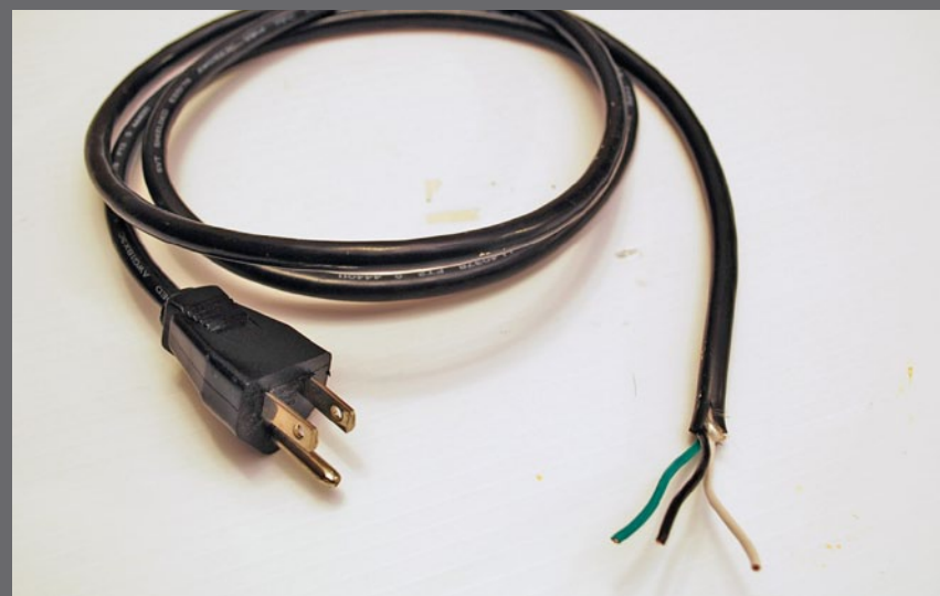
Figure 3.8: I stripped the sheath on the AC cord back to expose the wires, being careful not to cut the insulation on the individual conductors.
