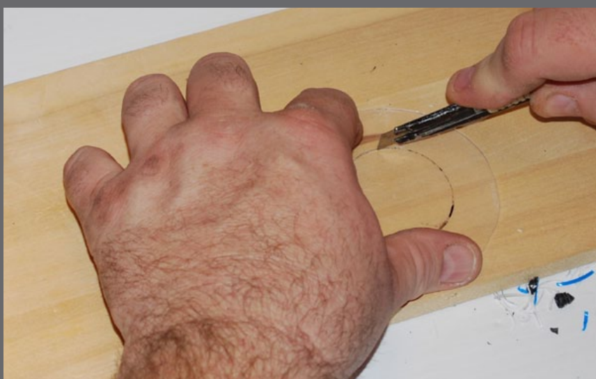
Figure 1.17: I cut the center from the lid cut out, making a washer for the pipe.
