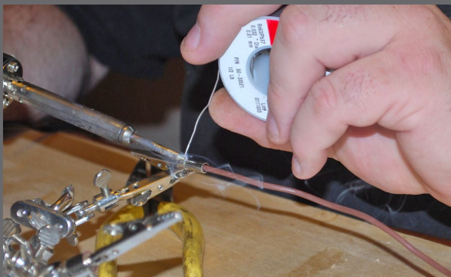
Figure 3.17: I soldered the alligator clip onto the end of the scenic ground wire.
