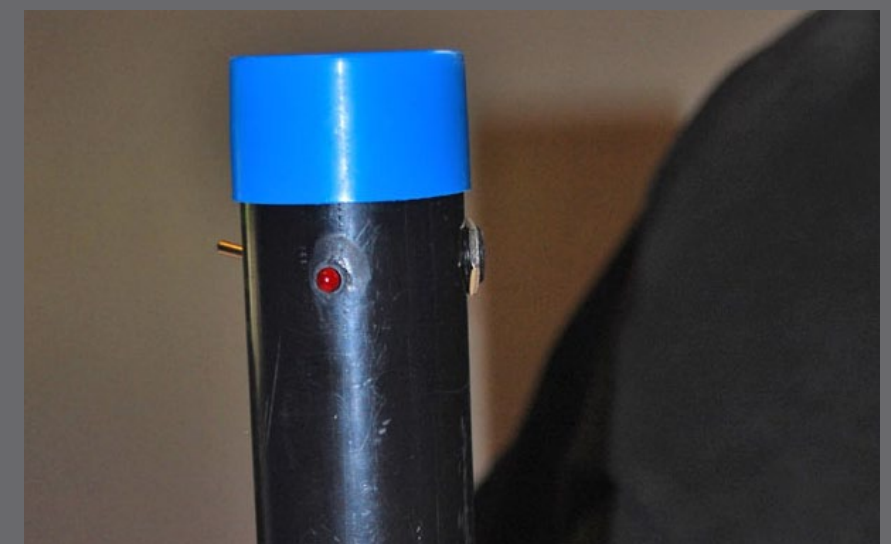
Figure 2.18: I slipped the second un-modified test cap over the end of the pipe to complete the build. I didn't glue the cap in place to allow ease of access later for servicing.
