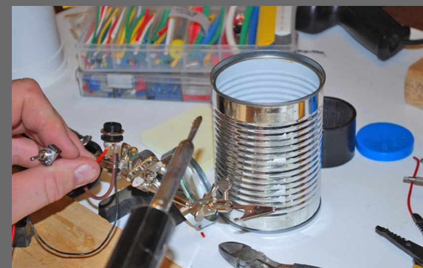
Figure 2.14: Soldering the scenic spike wire and the negative (black) ion generator wire to the chassis jack was a simple task with the help of my vise.
