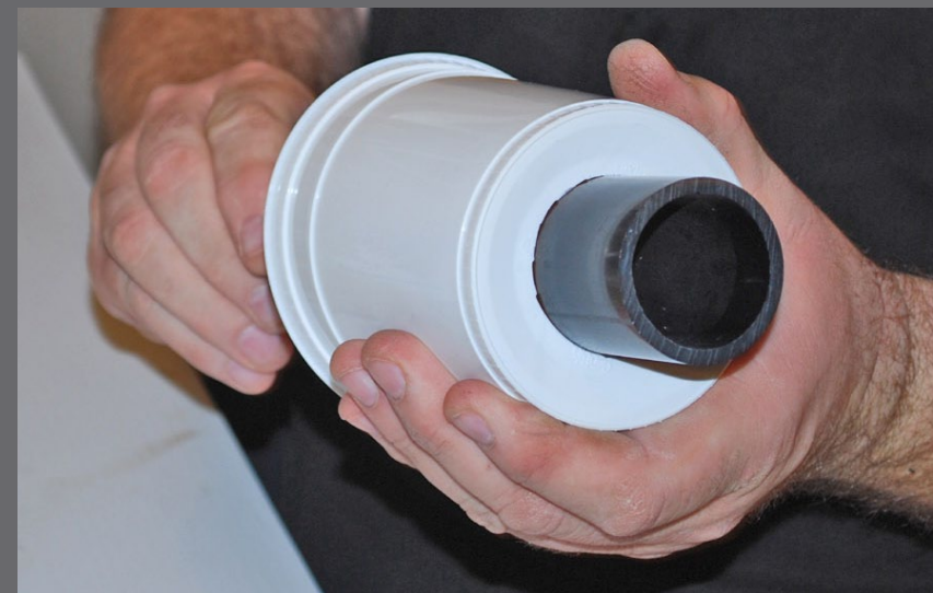
Figure 1.6: A tight fit between container and pipe is desirable. This looked close enough to me.
