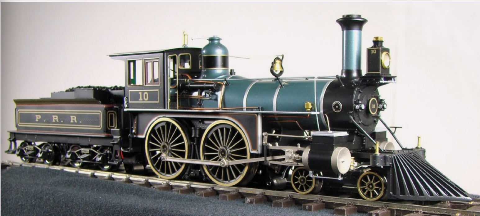
FIGURE 11: This beautifully handcrafted pilot model provides a preview of an O scale PRR 4-4-0 class D6 locomotive coming late this year from SMR Trains ( www.smrtrains.com ). A class D6a will also be available. These historically-important locomotives were built during the early 1880s for high-speed passenger service between New York and Philadelphia. The prototype engines were equipped with powered reverse, Westinghouse air brakes and high-speed water scoops under the tender to eliminate time-wasting stops at water tanks. Among the many features of the authentically decorated brass models are moving eccentrics and valve gear, a boiler-mounted Pittman motor and all-metal gears. The 2-rail model is wired for conventional DC operation with a plug-in harness to facilitate use of DCC. Priced at $1700, expected late this year, the models can be preordered now at a substantial savings. Visit their website for ordering details, technical and historical information and additional photographs.
