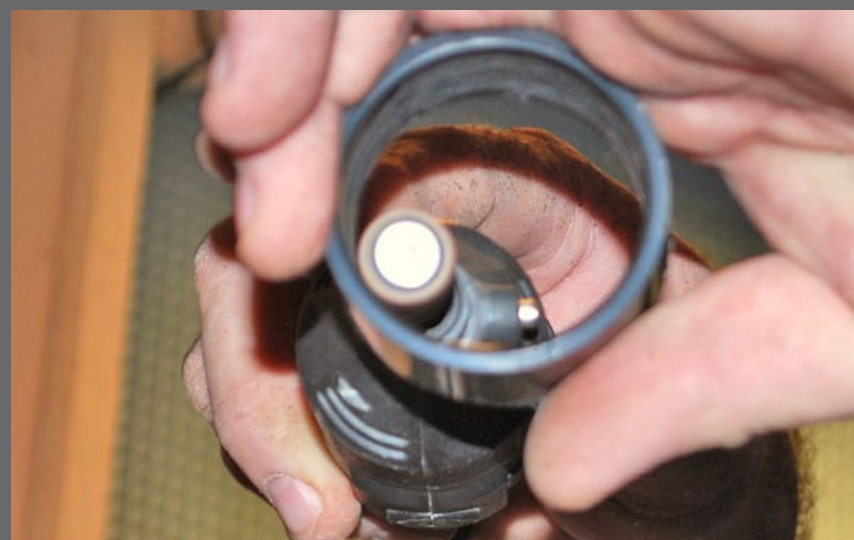
Figure 1.15: A sanding drum chucked in the Dremel smoothed the inner surface so the coupler would slide on without binding.
