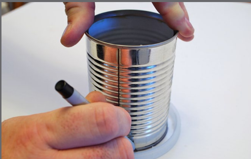
Figure 1.7: An appropriately-sized tin can makes a good marking pattern for the lid cut out.
