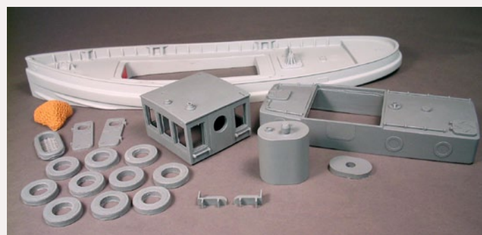
FIGURE 6: Frenchman River Model Works ( www.frenchmanriver.com ) has introduced a 1:48 scale 45-foot Harbor Tug ideal for O scale industrial waterfront scenes or funky On3/ On30 harbors. The superstructure, wheelhouse, tire bumpers, running-lights, smokestack, life float, doors, bow fender and waterline hull are all cast in resin. The windows and searchlight lens are laser-cut. Lead-free pewter castings include a mast, searchlight, anchor, horn, davit and bits. The completed model is 11.5-inches long.
