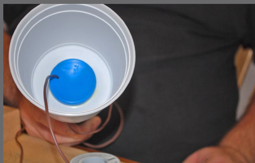
Figure 2.11: I fished a length of 16 gauge wire through the hole in the cap before making the solder joint with the charge wire.
