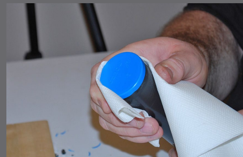
Figure 1.21: After setting the cap, I cleaned off any excess glue with paper towel.
