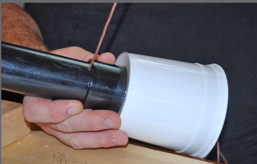
Figure 3.7b: I fished the scenic ground wire through the hole in the handle.
