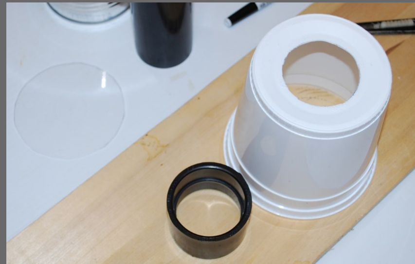
Figure 1.4: I used the inside of the coupler to mark the outside diameter of the pipe on the bottom of the container.
