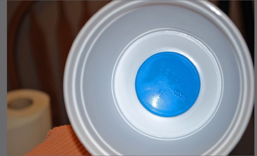
Figure 1.23: I applied a little Cyanoacrylate glue to the edge of the cap before seating it against the bottom of the flock jar.
