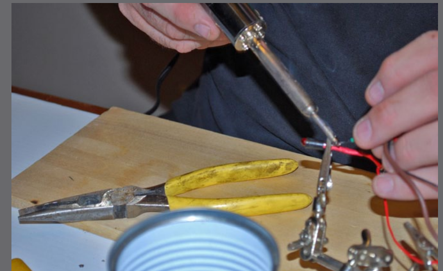
Figure 2.4: I soldered the LED wire leads on and added insulation to its bare leads to avoid shorts.
