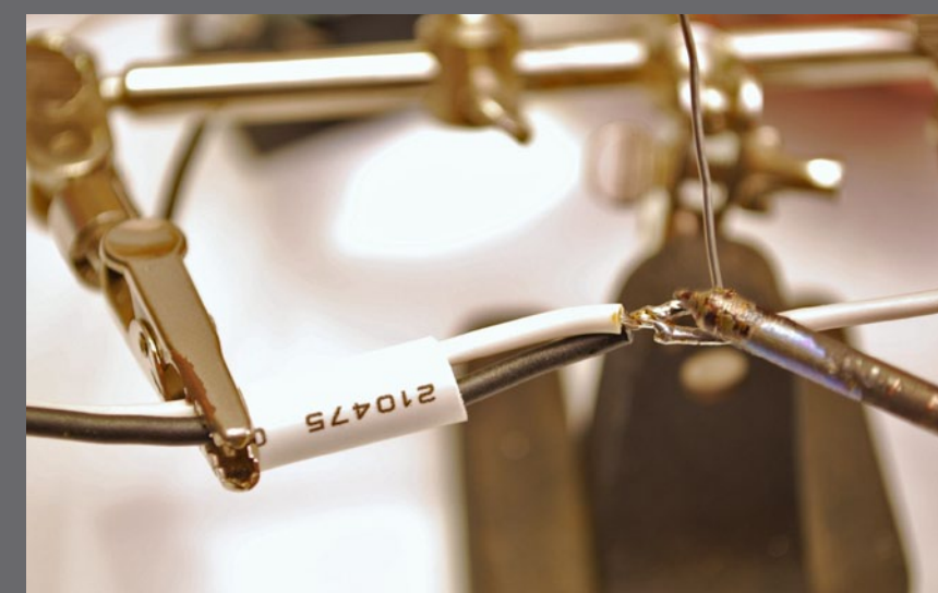
Figure 3.13: I soldered the common, (white) wire in the AC cord together with the white wire from the ion generator and the second lead on the neon indicator lamp.
