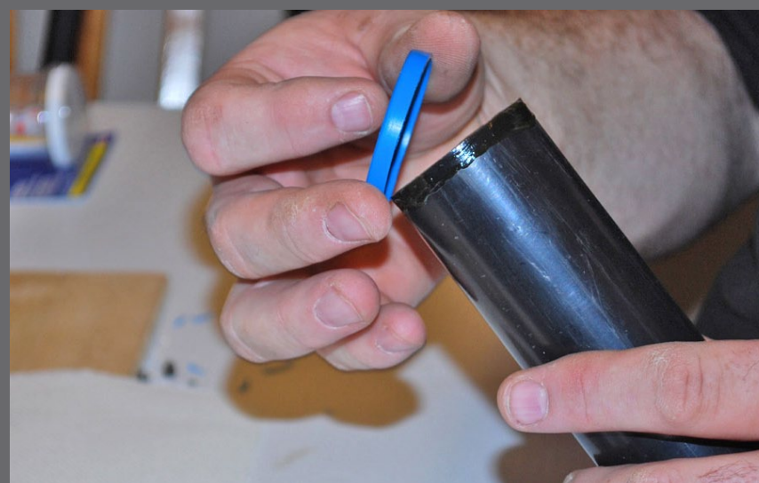
Figure 1.18: I used ABS glue that I had on hand to install the modified pipe cap on one end of the pipe.
