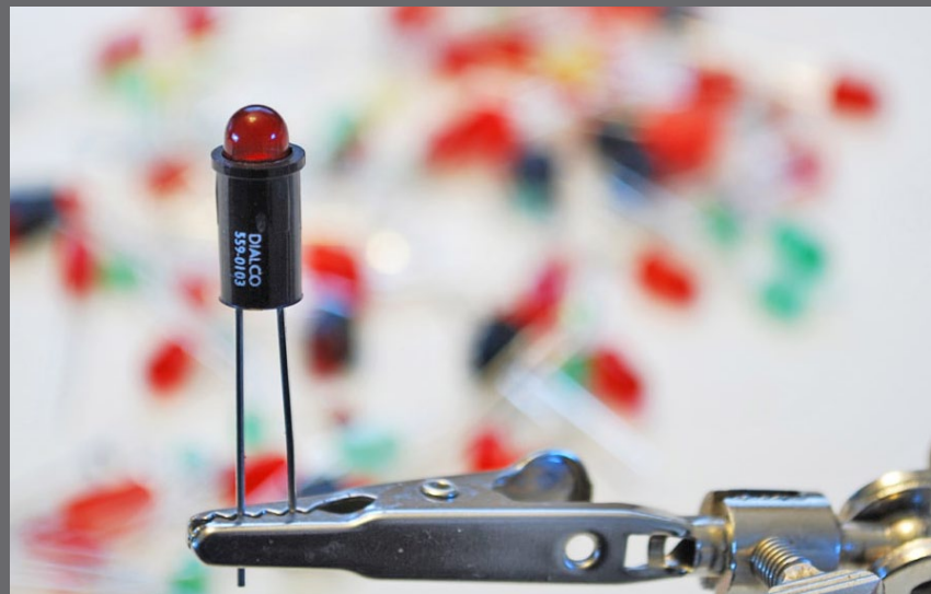
Figure 2.3: The Dialco LED I used has a built in resistor and is rated at 12 volts.
