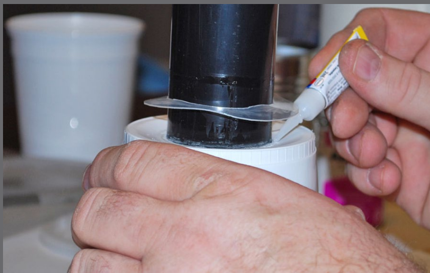
Figure 1.26: Before sliding the washer into place, I applied some CA glue.
