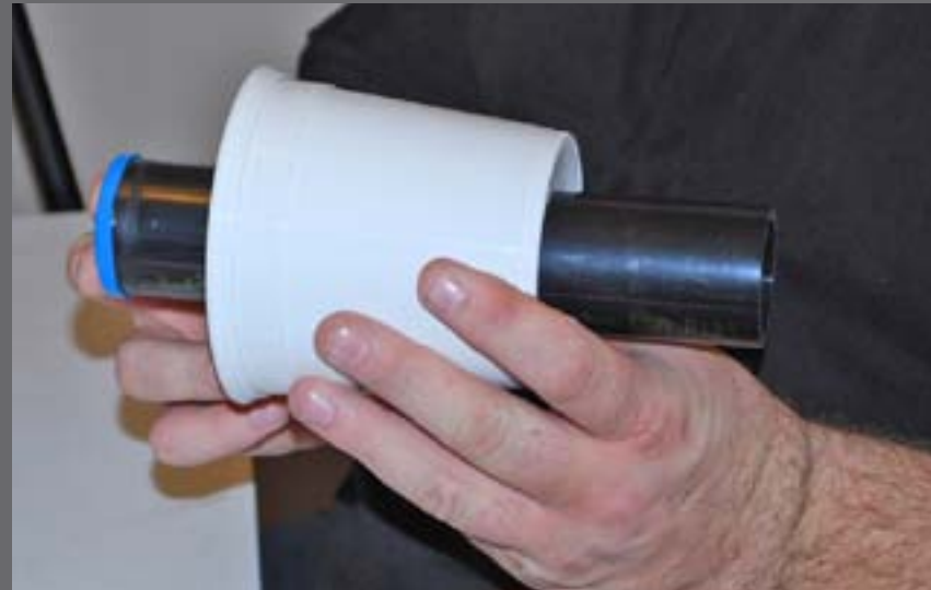
Figure 1.22: I slid the handle into the flock jar in preparation for gluing.
