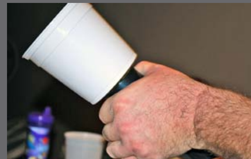
Figure 1.30: I slid the coupler down seating it firmly against the bottom of the flock jar.
