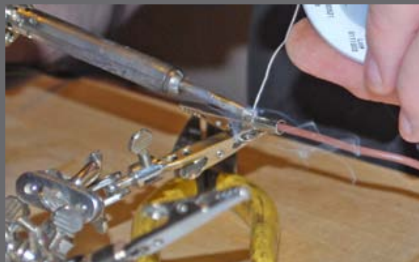
Figure 2.15a: I soldered an alligator clip to the wire end.
