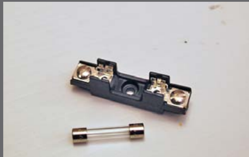
Figure 3.6: This project needs to be fused for safety. I used a surface mount fuse block I had on hand and a 1-amp fast-blow fuse.
