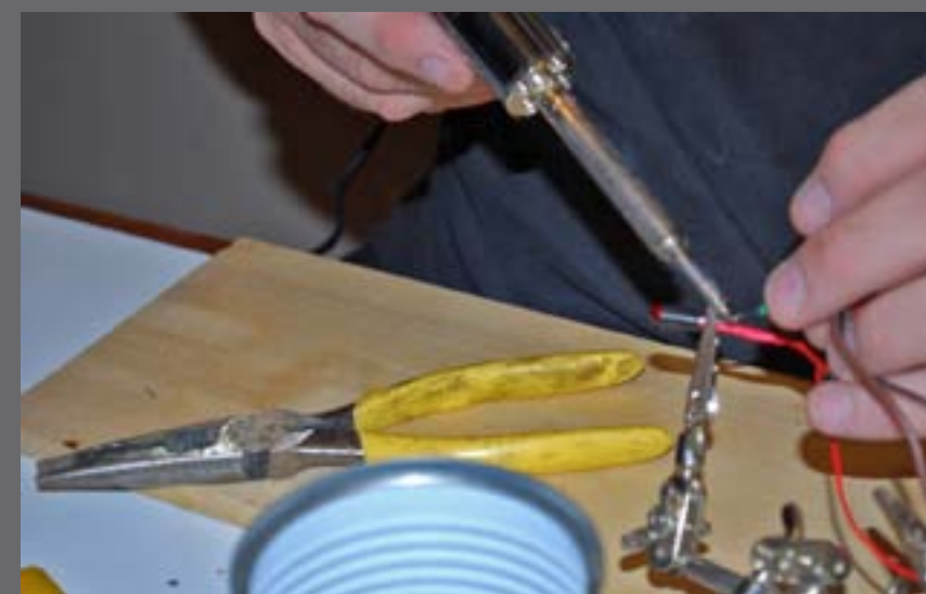
Figure 2.4: I soldered the LED wire leads on and added insulation to its bare leads to avoid shorts.
