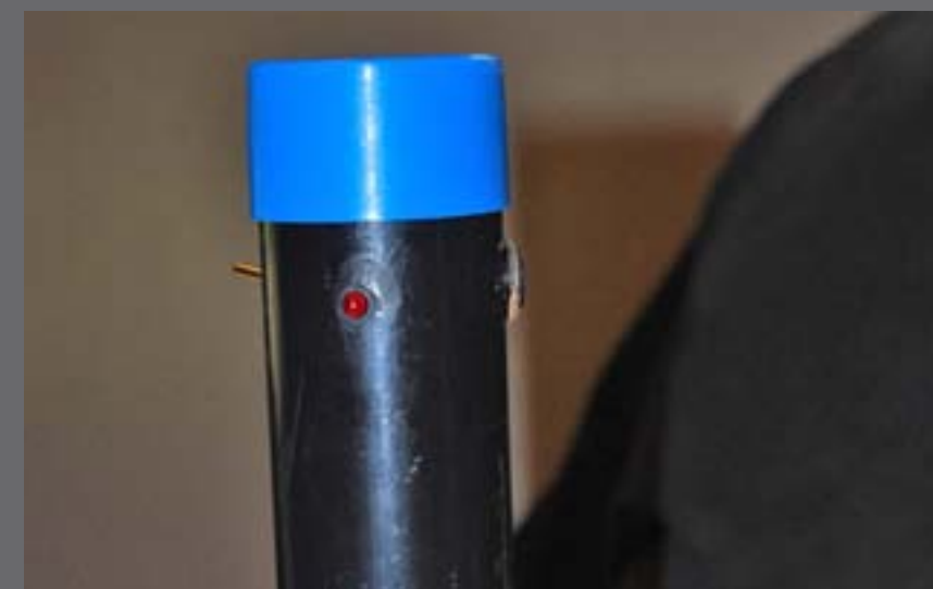
Figure 2.18: I slipped the second un-modified test cap over the end of the pipe to complete the build. I didn't glue the cap in place to allow ease of access later for servicing.
