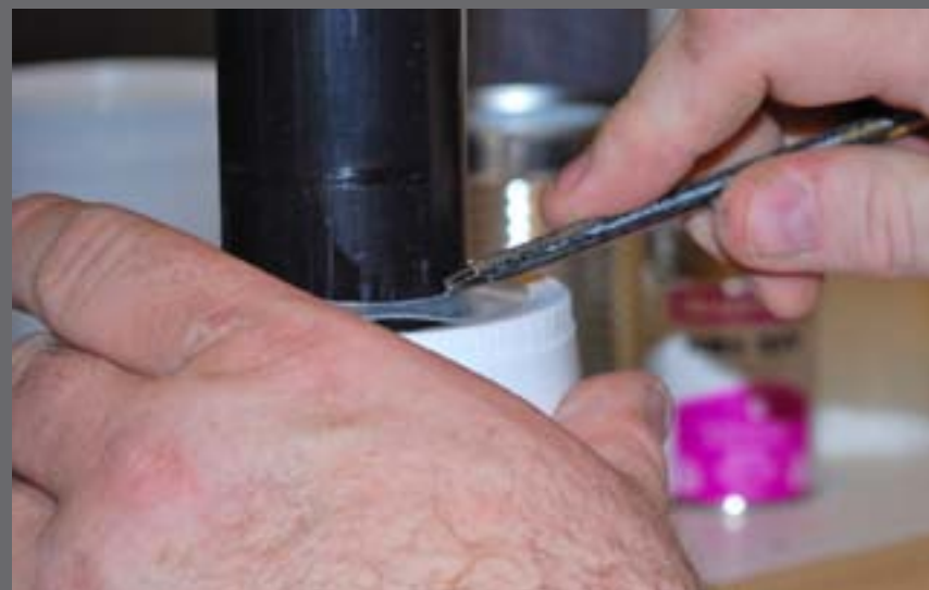
Figure 1.27: I used the end of my knife to press the washer into the glue.
