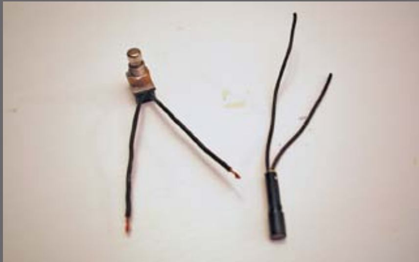
Figure 3.5: I salvaged the power switch and neon lamp for the project. Comparable substitutions can be found in the online tool & parts list.
