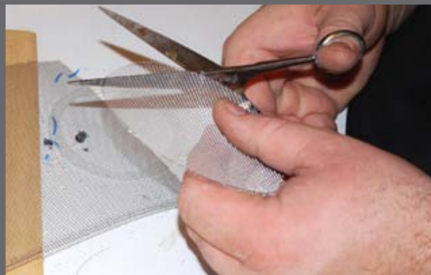
Figure 1.10: I cut the screen a bit large and trimmed it to a close fit.
