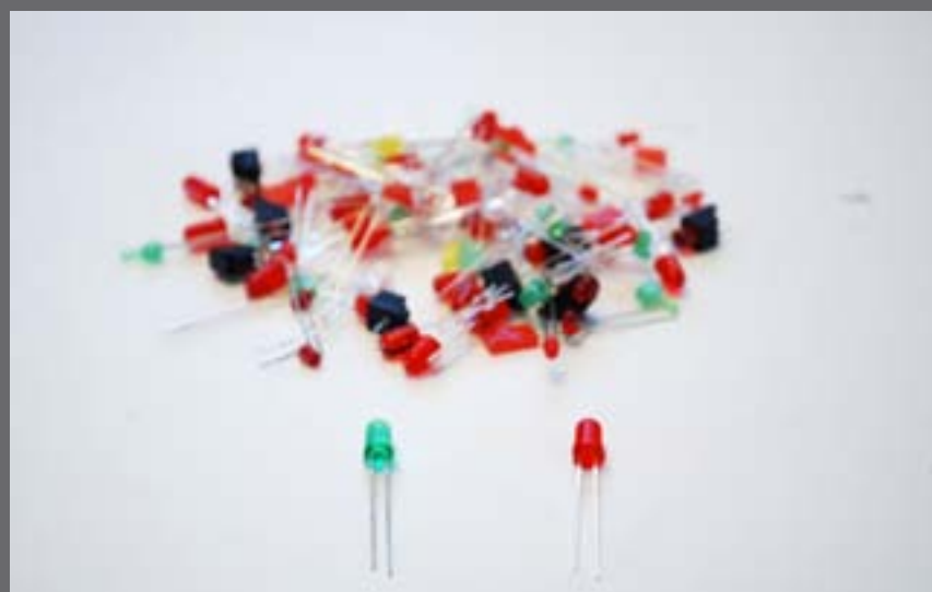
Figure 2.1: LED's come in many colors, shapes, and sizes and are identified in different ways. These two are identified by the shorter cathode (negative) lead.
