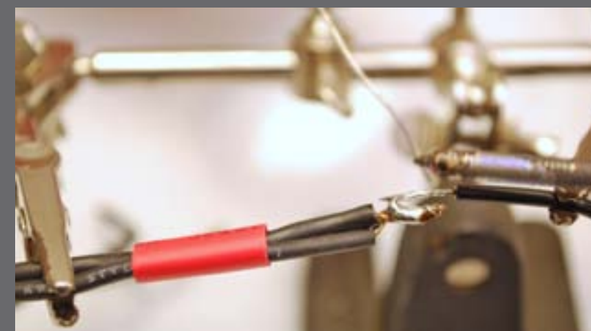
Figure 3.12: All of the soldered connections were tinned prior to soldering and insulated with heat-shrink. Here I am soldering the joint between the second switch lead, the neon lamp lead and the power lead from the negative ion generator.
