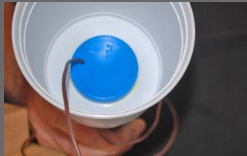
Figure 3.14: I substituted a 16 gauge stranded copper wire for the charge wire from the ion generator. I found the charge wire to be a bit fragile when removing the screen lid to add flock.
