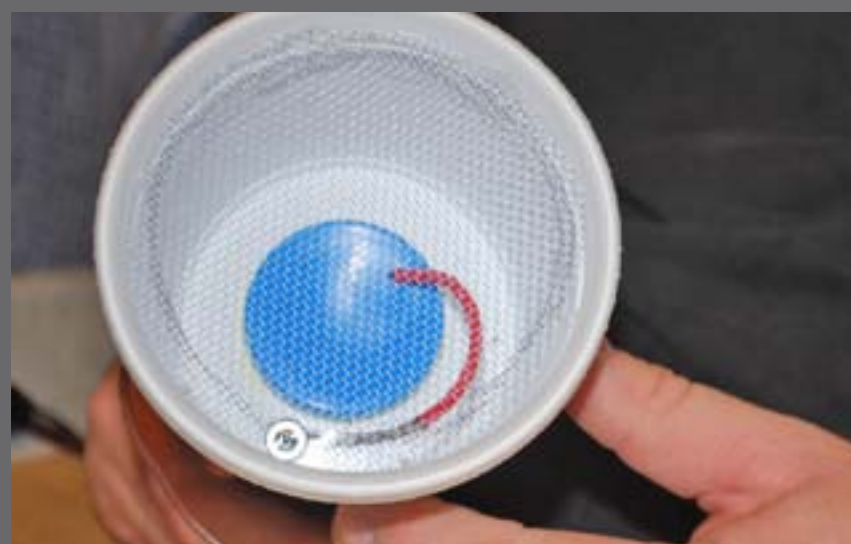
Figure 2.13: To complete the charge screen wiring I added red heat-shrink as a reminder of the shock potential here and used a machine screw and washer to make a solid connection with the screen.
