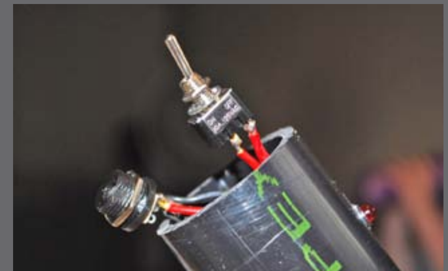
Figure 2.9: Red leads route power from the jack to the switch and then on to the LED and ion generator positive leads. With the positive portion of the component wiring complete, all that remained was to make the negative connections.
