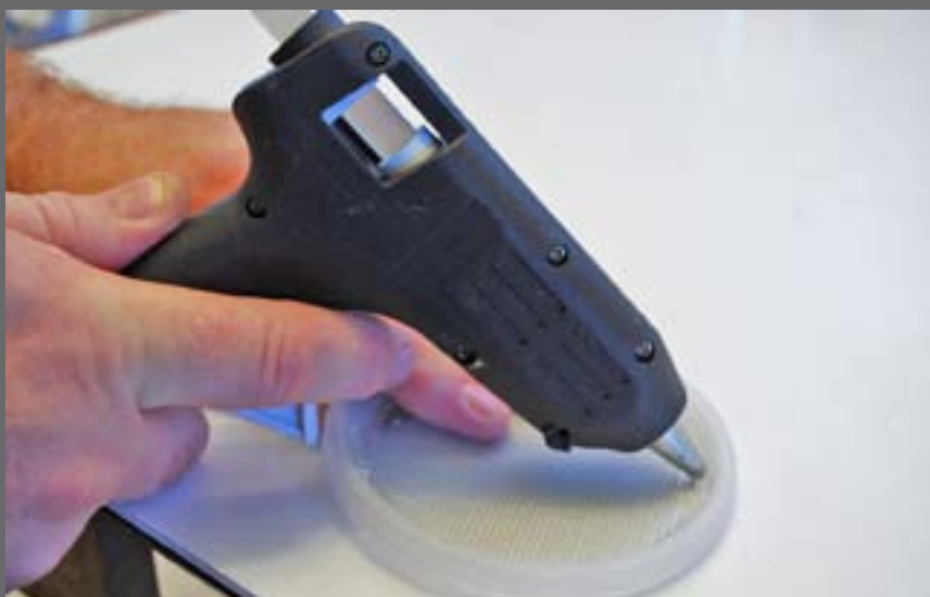
Figure 1.12: A quick bead of hot melt glue kept the screen from going anywhere.
