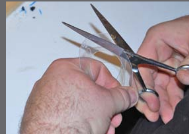
Figure 1.25: I cut a ring off the outer circumference to make the washer fit the jar.
