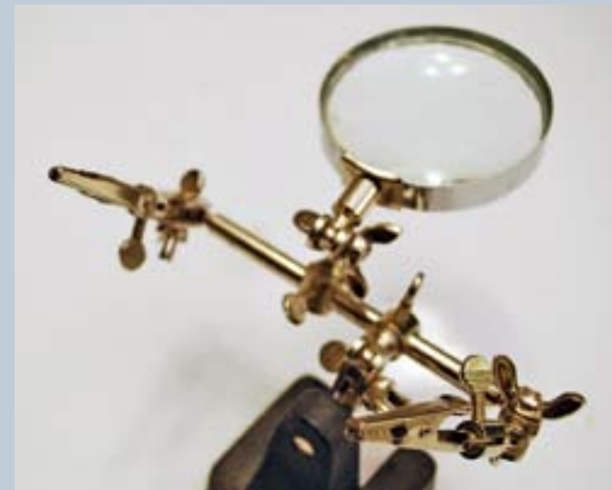
Figure E: A handy vise like this one can save a lot of headaches when soldering or doing anything that has your hands full and trying to position small parts for joining.
