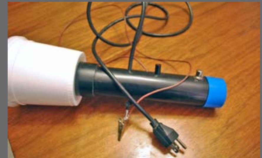
Figure 3.15: I slipped on the cap, finishing the internal wiring for the 120V applicator.
