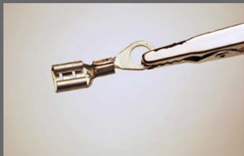
Figure 3.18: I made this custom terminal so I could remove and change screens quickly and easily without having to loosen the mesh contact screw.
