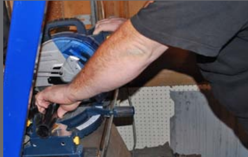
Figure 1.1: I used my compound mitre saw to cut the ABS pipe into 9 inch lengths. A hacksaw or even a crosscut wood saw will work well too.
