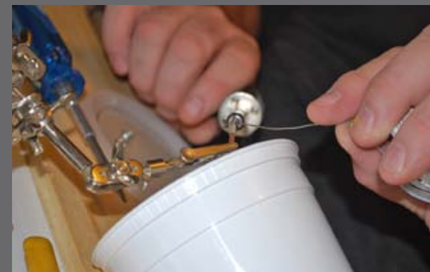
Figure 2.12: With the charge wire cut to length, I used my vise again to make short work of soldering the terminal end onto the charge wire.
