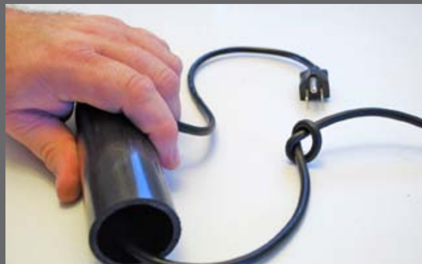
Figure 3.7: I tied a knot in the cord to act as a strain relief and avoid any tugging on the internal wiring.
