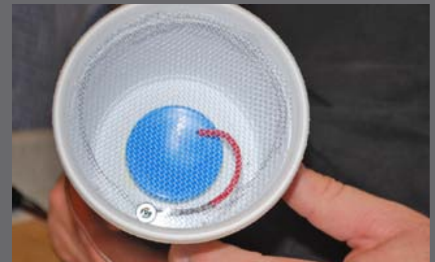
Figure 3.16a: I covered the charge wire in red heat-shrink as a reminder of the shock potential.
