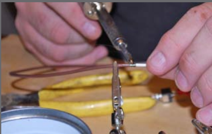
Figure 2.10: My vise helped me hold the two wires steady, side by side, while I soldered the heavier wire onto the delicate charge wire from the ion generator.
