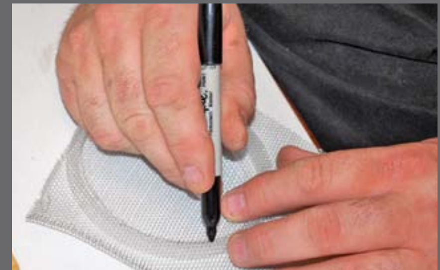
Figure 1.9: I used the container lid to mark the aluminum screen to approximate size.
