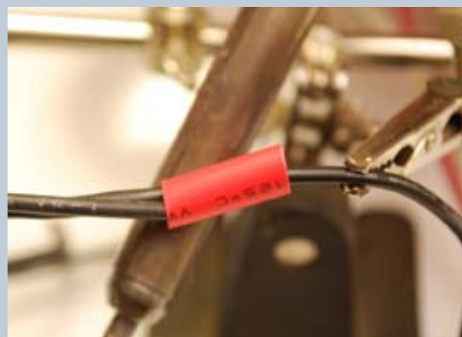
Figure G: Heat-shrink tubing, what a great invention! Slide it over a bare connection, apply a bit of heat and in seconds you have a tightly-wrapped, insulated connection. Covering small gauge wire connections with heat-shrink tubing helps avoid breakage from repeated flexing of fine conductors.
