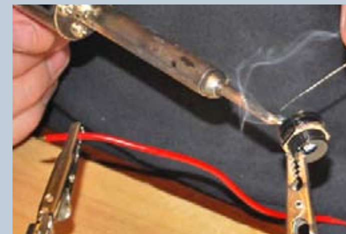
Figure D: Don't forget to pre-tin the component terminals with solder too.
