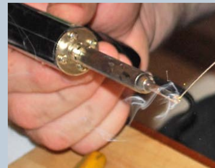
Figure B: Pre-tinning the soldering iron with solder is an important first step in assuring a strong electrically conductive solder joint is achieved.
