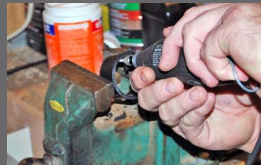
Figure 1.14: Using my Dremel and a multipurpose bit, the ridge just peeled away from the coupler's inner surface.
