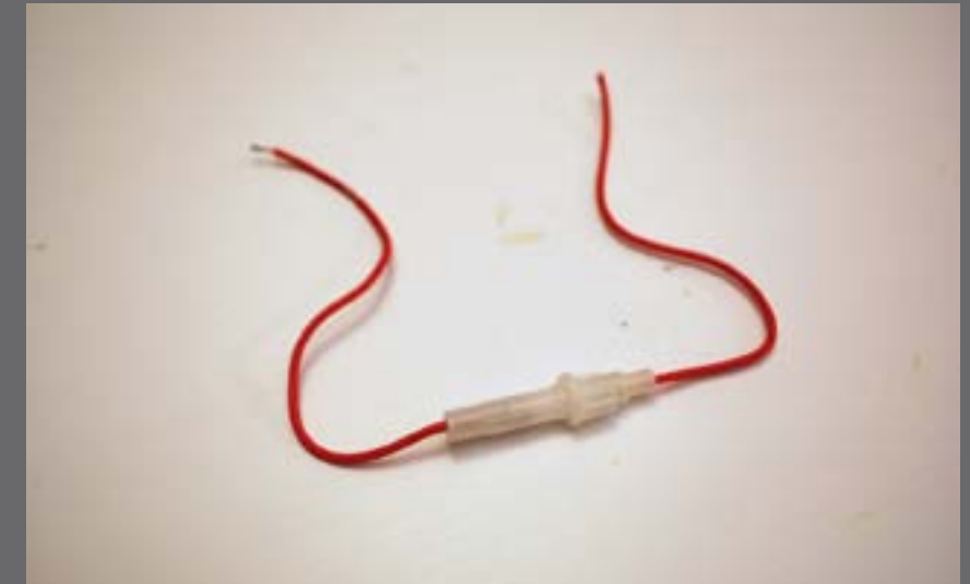
Figure 3.6a: An inline fuse holder rated for 120 volts is fine too.
