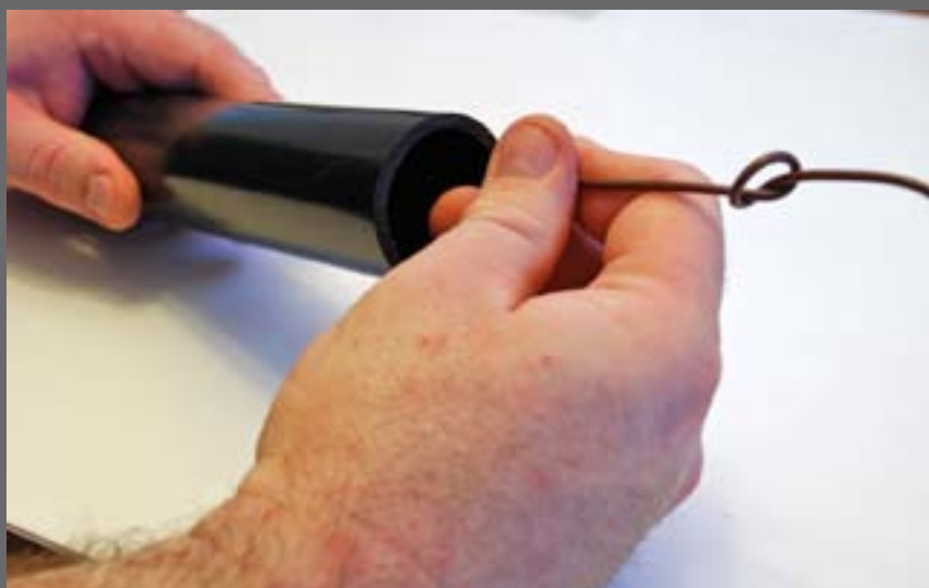
Figure 2.15: I used knots in the wire to act as strain relief inside the handle.
