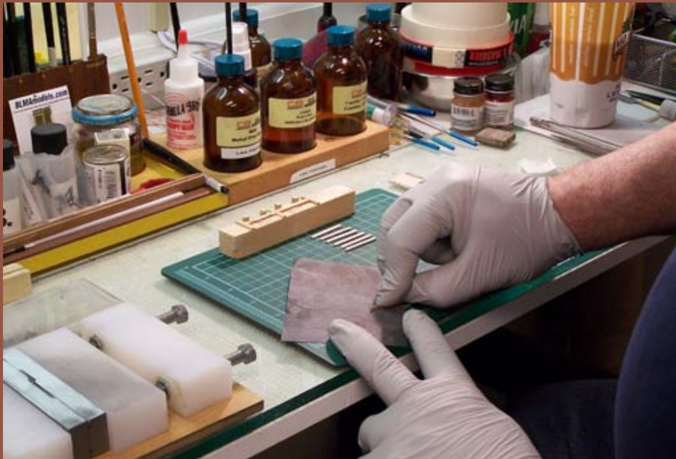
Figure 1: I use rubber gloves when sanding PC board ties to prevent glass shards from penetrating the pores in my fingers. I don't know if you have ever experienced tiny glass shards in your pores, but let me tell you, they are extremely annoying and practically impossible to remove.
