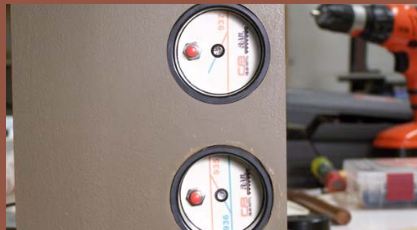
Figure 36: I test fit the push button/LED assemblies on the module.
