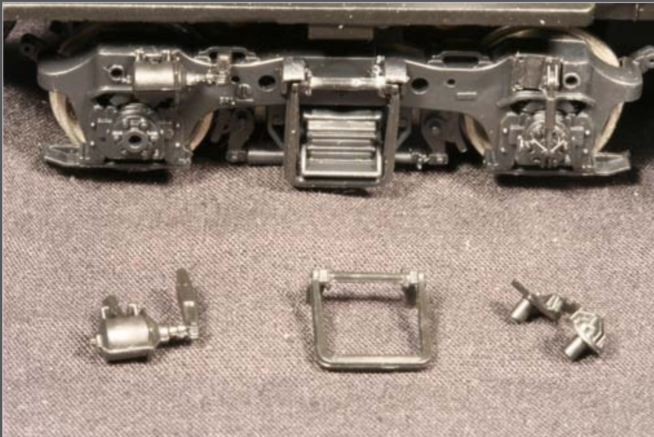
Figure 39: Athearn's locomotives come with basic truck details, but more can be added for a super-detailed model.
