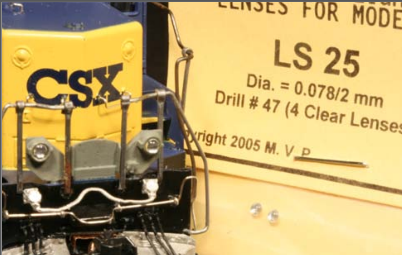
Figure 41: Modelers who do not wish to light their locomotives can opt for 'jewels' placed in the ditch light and headlight openings.
