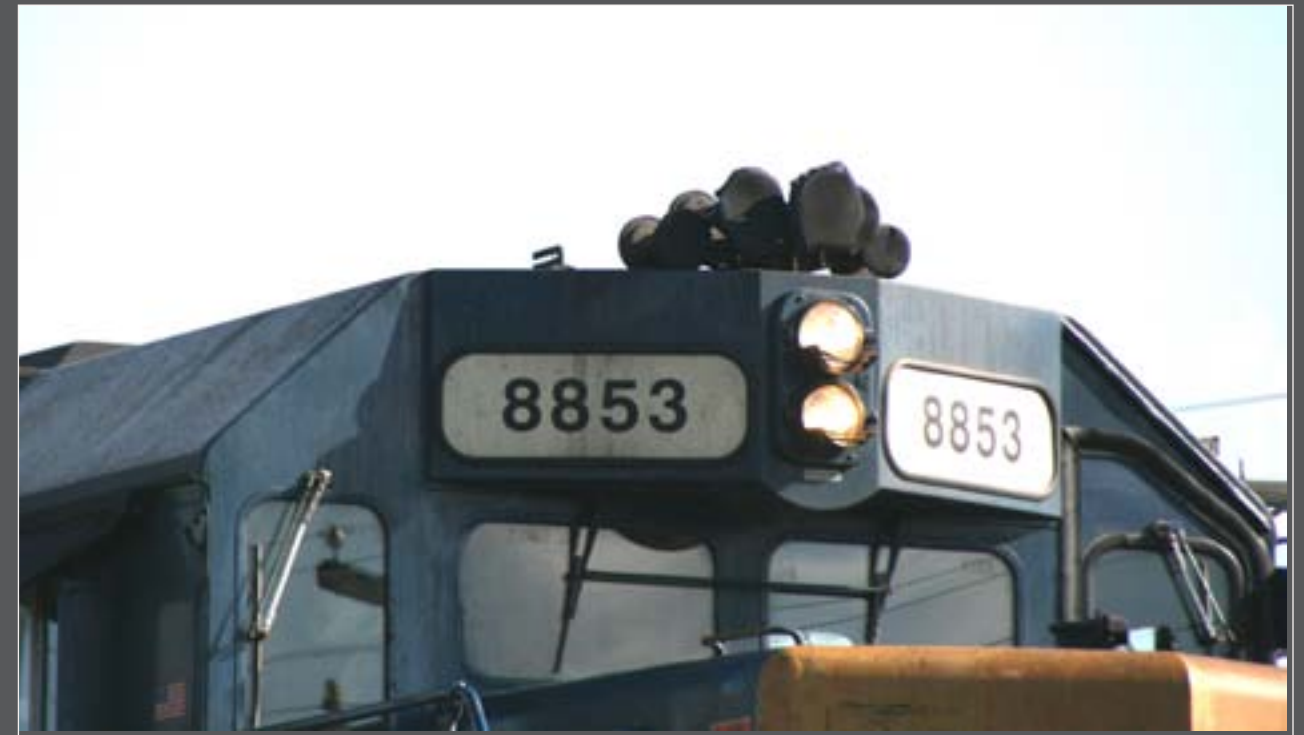
Figure 27: Roof details are often a mystery, as we often view the prototype at ground level. Several common details applied to cab roofs are a horn, radio antenna, and end-of-train antenna.
