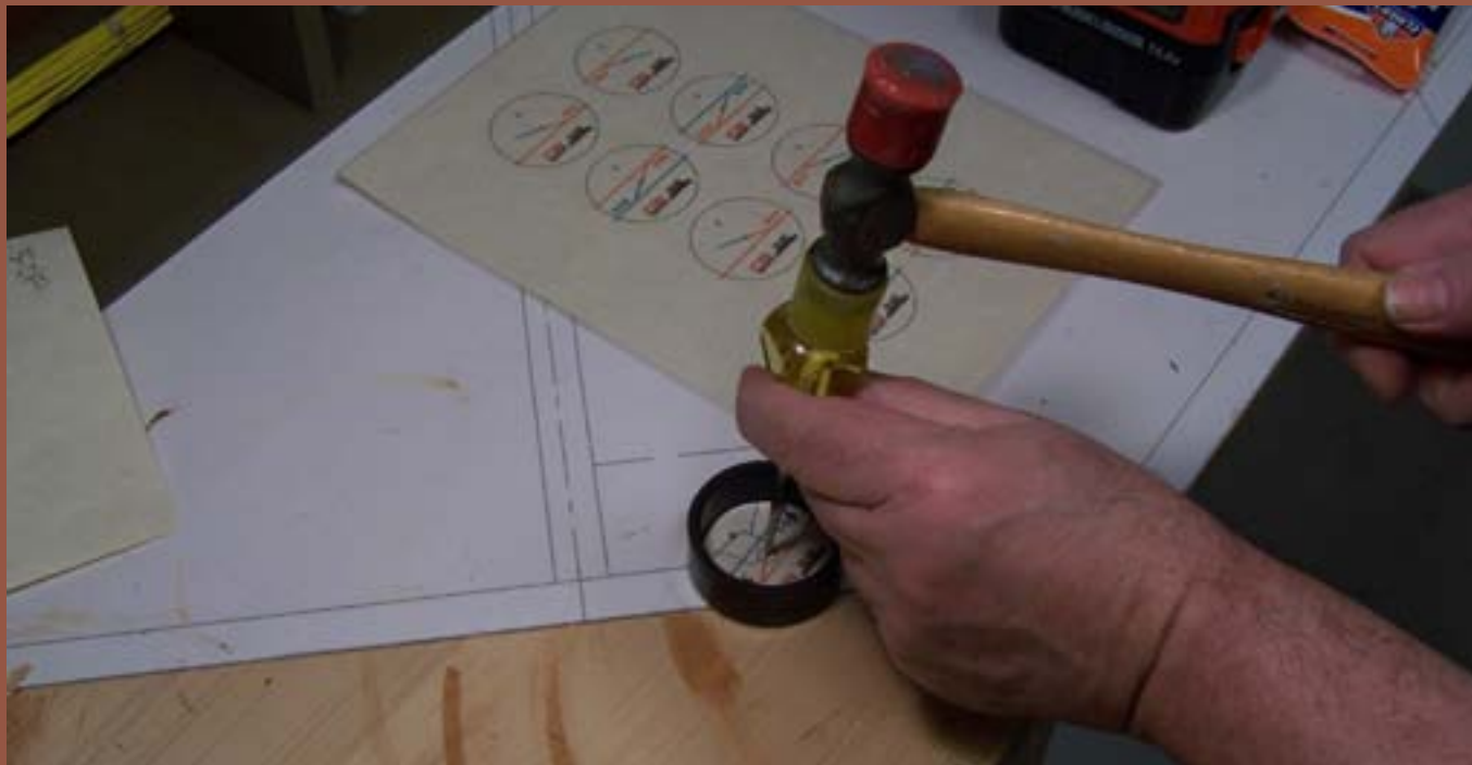
Figure 29: Using the label as the template, I marked the hole locations with a center punch.
