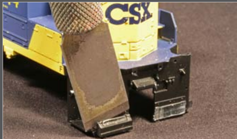
Figure 16: To properly mount a snowplow, the pilot face must be flush, requiring removal of footboards of any other protrusions.
