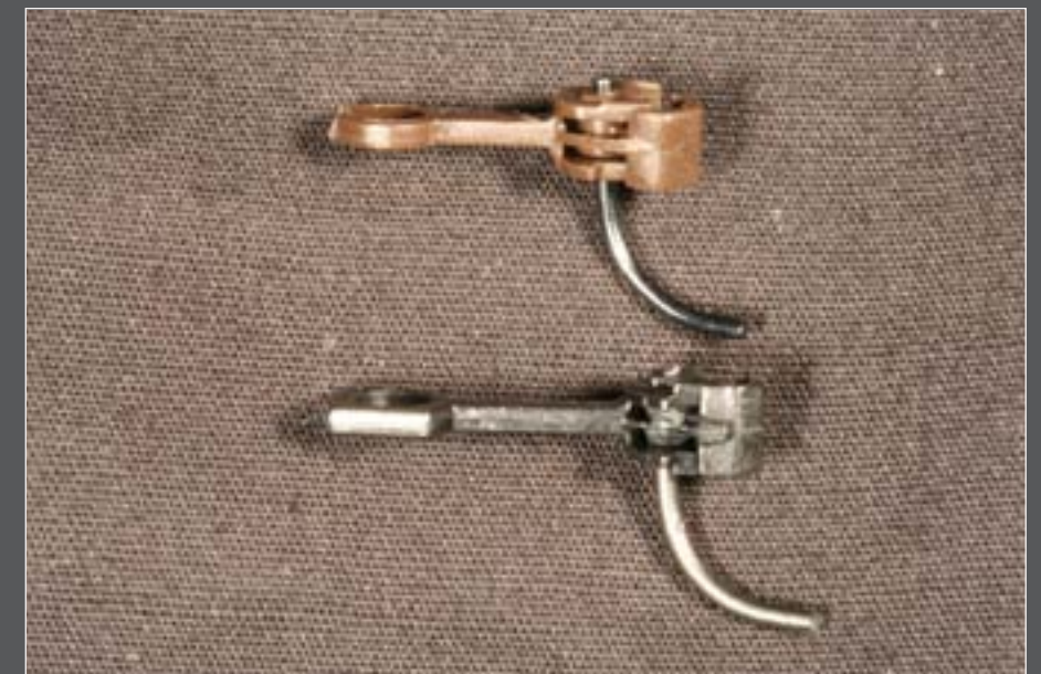
Figure 40: Adding a snowplow can interfere with factory couplers. Extended-shank couplers will project beyond the snowplow, easily correcting interference issues.
