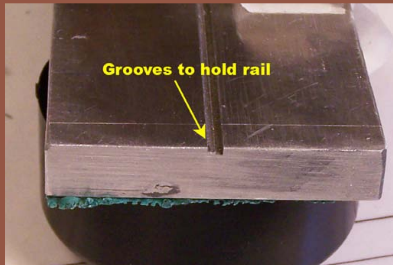
Figure 16: End view of jig. Groove on one side is for Code 83 and Code 70 on the other. The jig was built using a 3/8" piece of aluminum. I left a wide space in the middle for soldering. It really does a great job and also acts as a heat sink.
