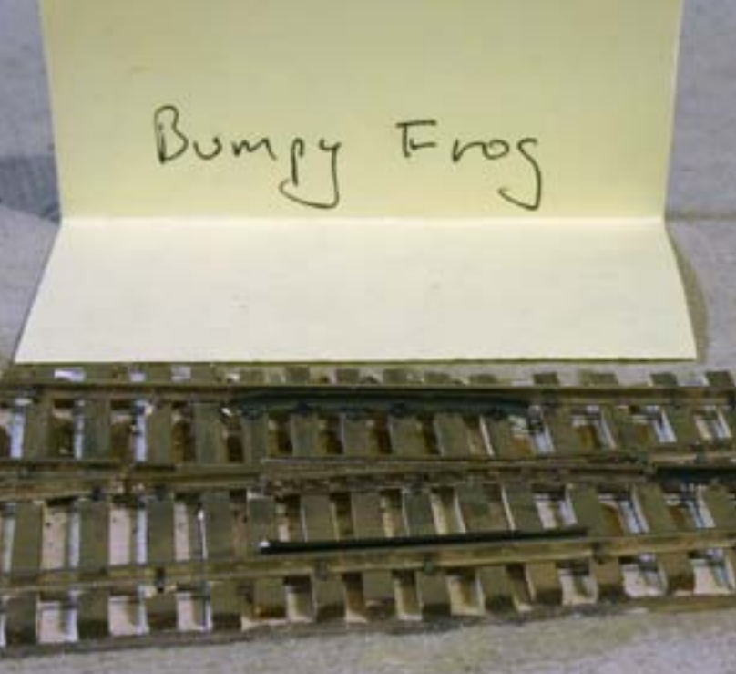
Figure 5: One of the crew noted a “bumpy frog” in Montville. I was fully prepared to tear up the turnout and rebuild it when I realized the frog was approximately – make that exactly – .015” lower than the other rails . . . someone (me!) had put a Details West code 55 frog in an otherwise code 70 turnout... Swapping it with a code 70 frog took all of two minutes. Marty McGuirk photo.
