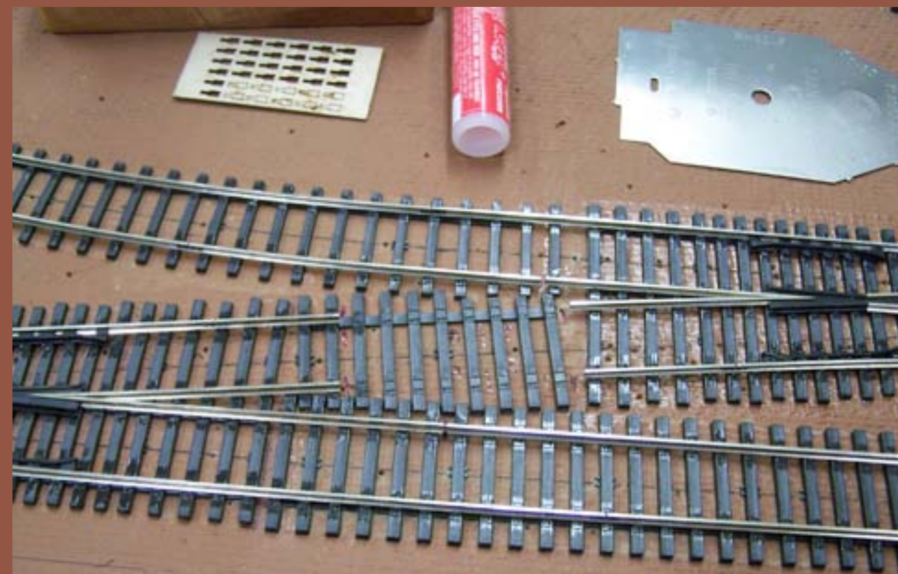
Figure 13: The main line track (in front) is Code 83, but the siding (in back) is Code 70. Transition rails are required to connect them.
