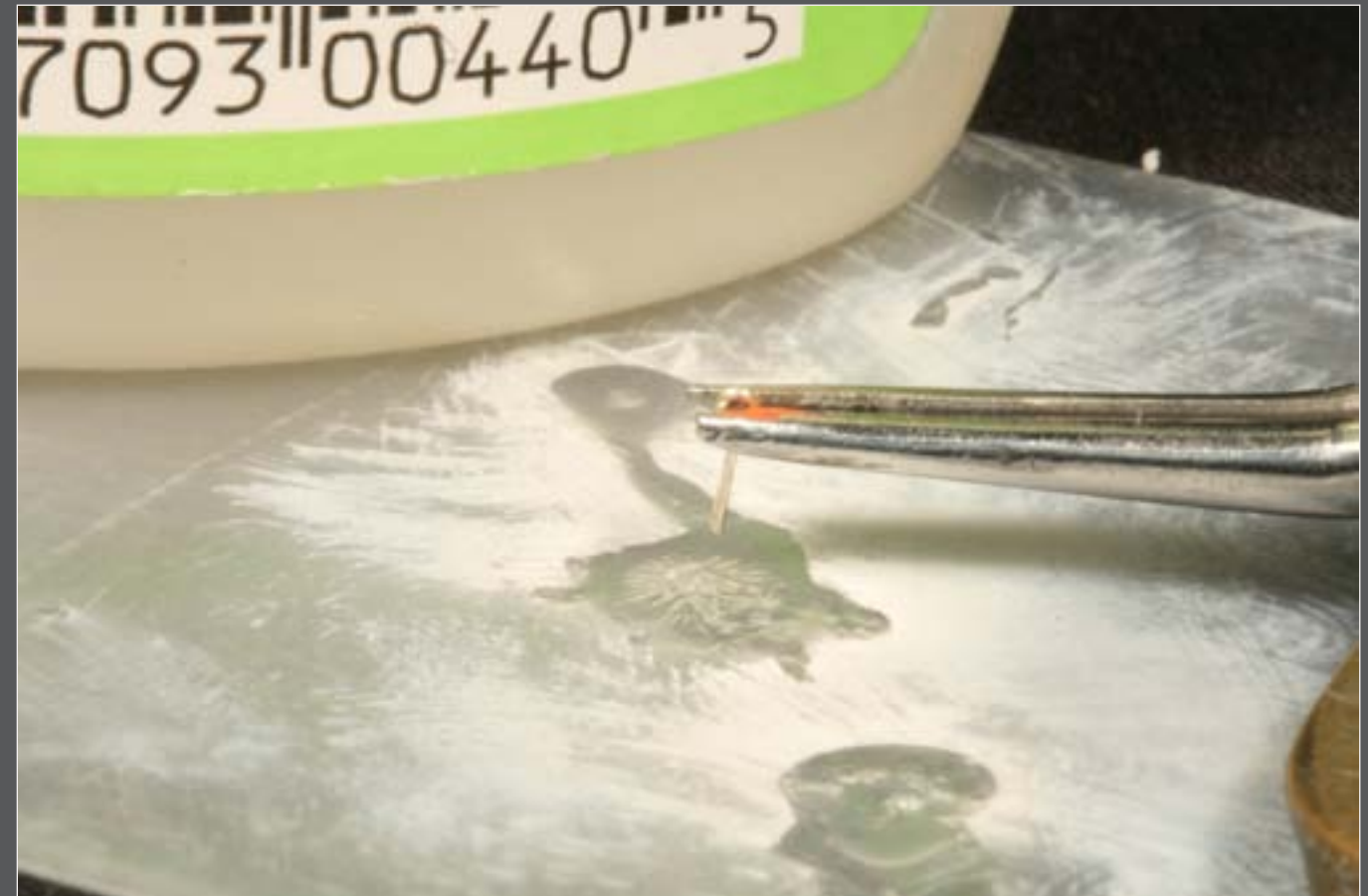
Figure 13: A good way to keep excess cement from marring the surface of your model is to apply the cement to a piece of scrap styrene, then dip the mounting stem into the cement rather than applying cement directly to the model.
