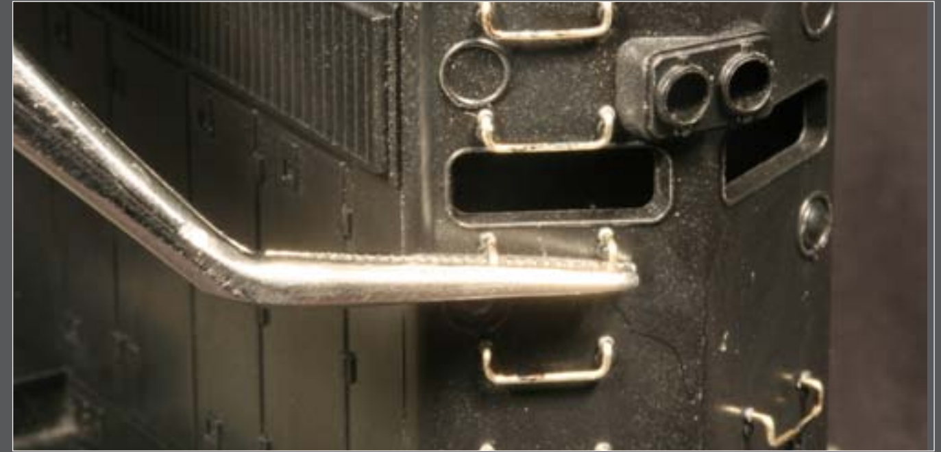
Figure 8: Once in place minor adjustments can be made to grabirons that are not level, gently bending them until they are properly aligned.
