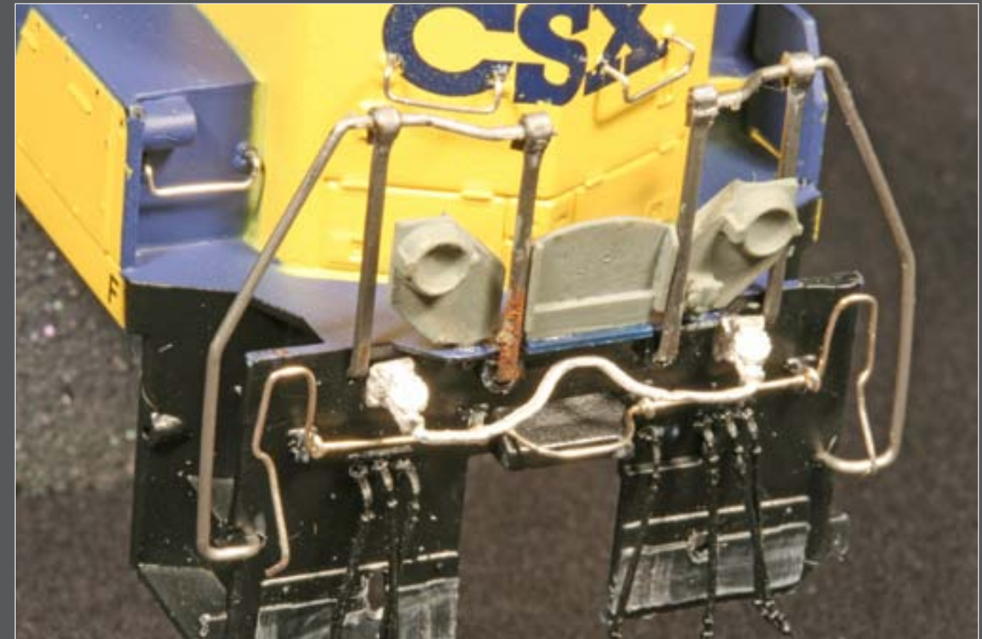
Figure 36: Metal MU cable castings will allow bending, giving the look of a cable tethered to the pilot of the locomotive.
