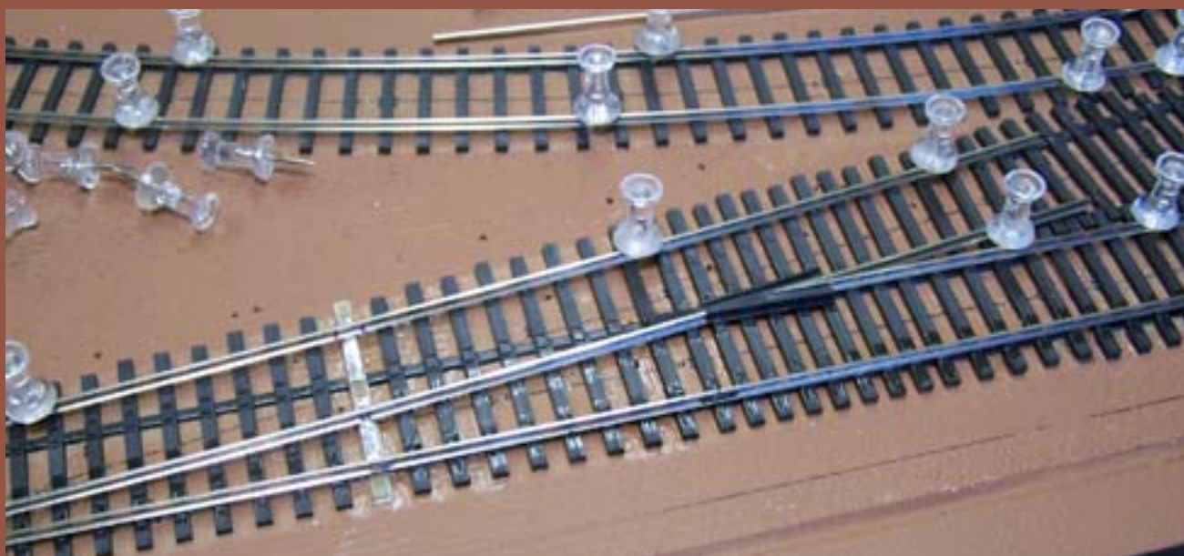
Figure 11: Then I installed the stock rails and added the frog and point rails.
