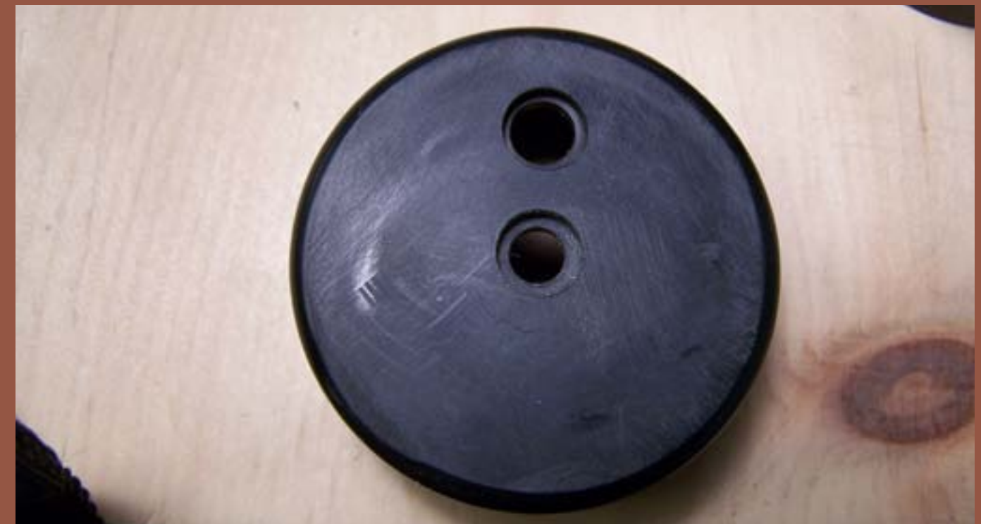
Figure 32: The holes countersunk and drilled, ready for the installation of the push button and LED.
