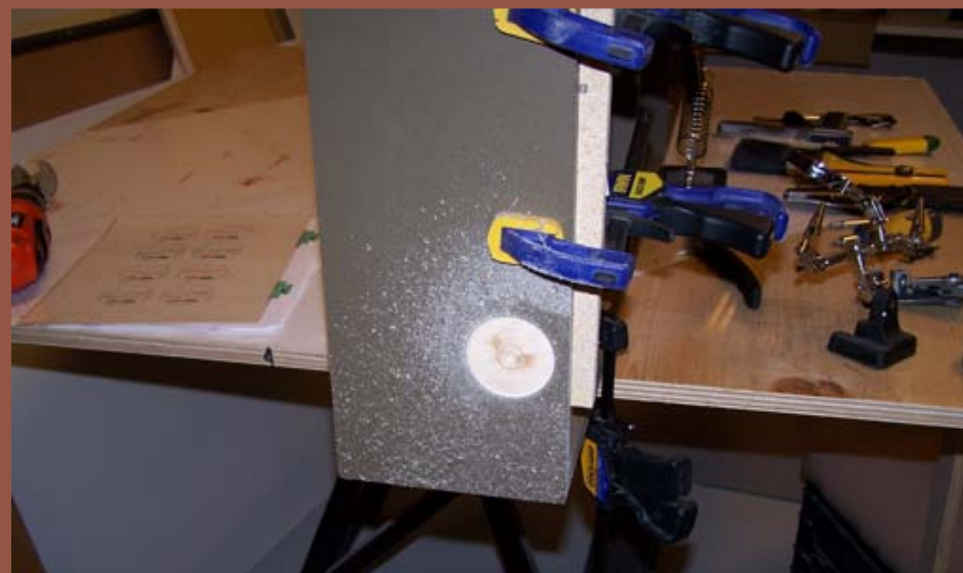
Figure 25: I Used a Forstner bit to drill the holes in the module sides.
