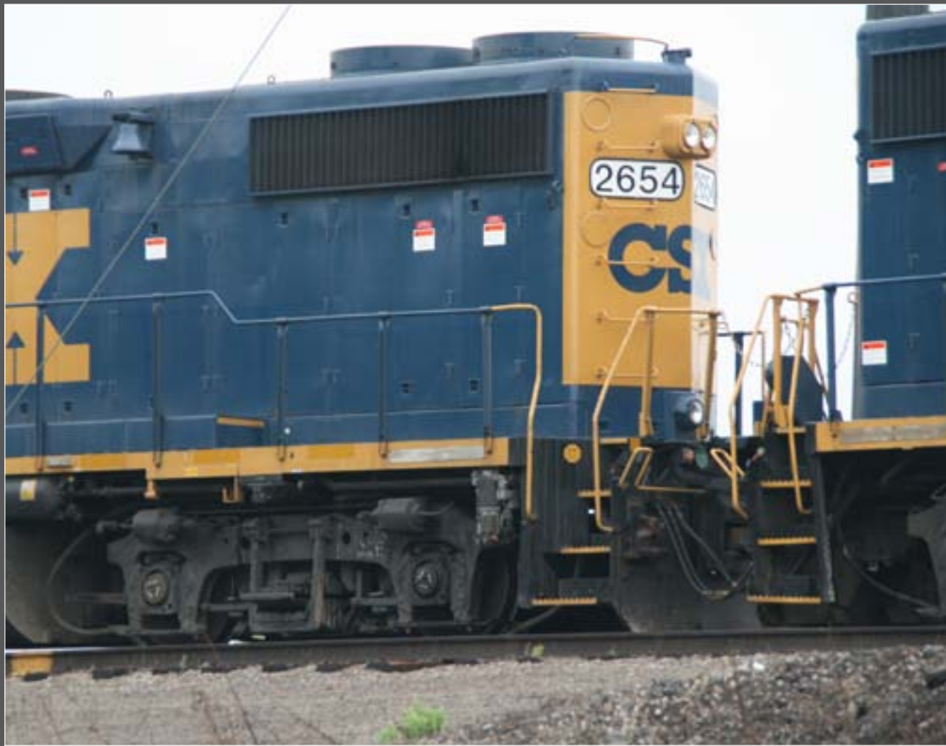
Figure 9: Visible in this photo are the lift rings and fan grab on the roof of this CSX locomotive.
