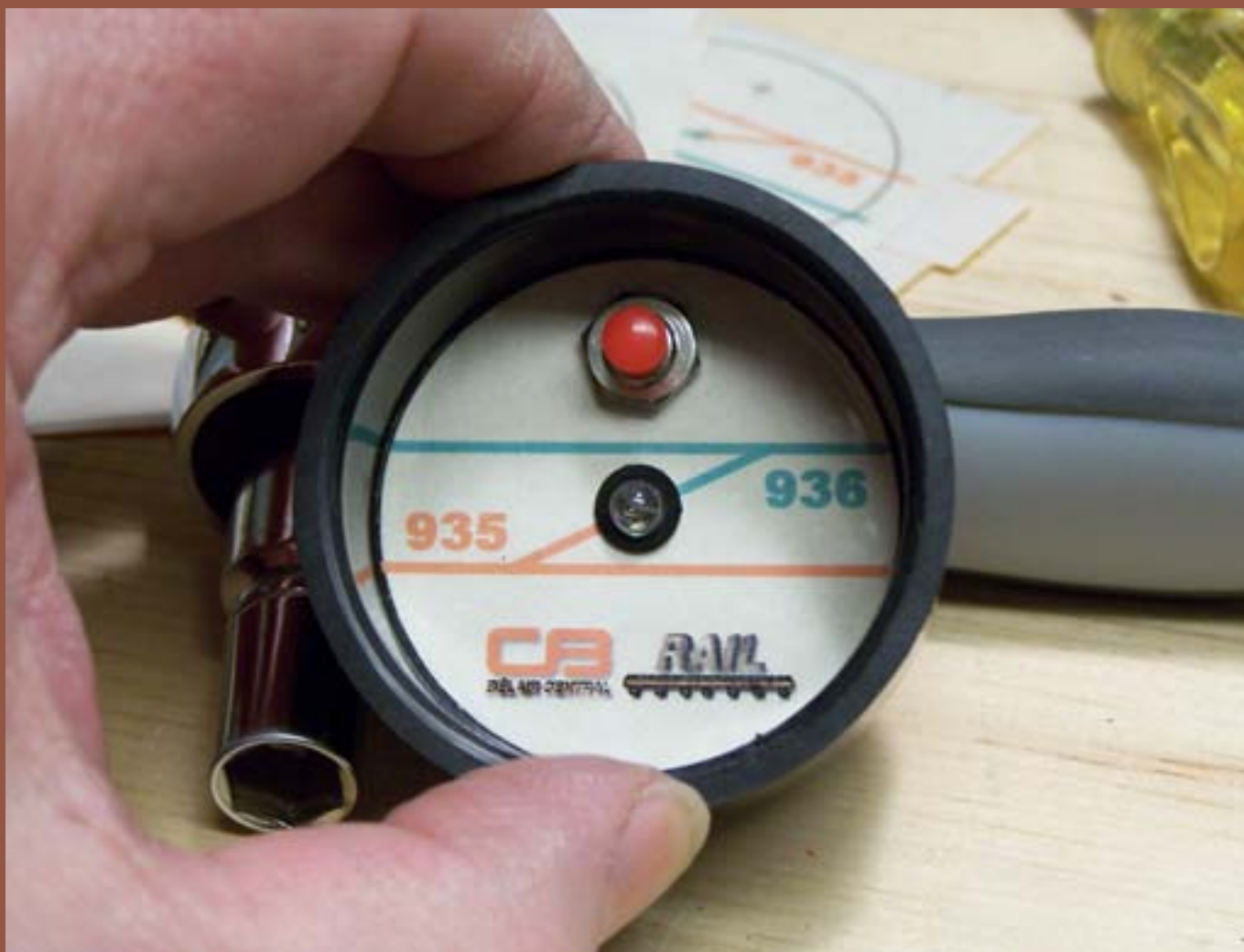
Figure 23: This is the final product. One push button and one Red Flashing LED with the Turnout numbers on the schematic diagram. Ok, so how did I get there?
