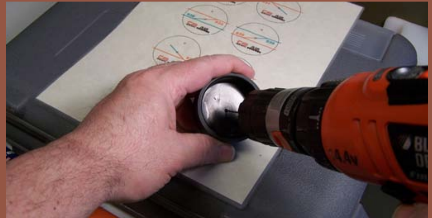
Figure 30: Using the punch marks as references, I drilled two 1/16" diameter pilot holes for the next step.
