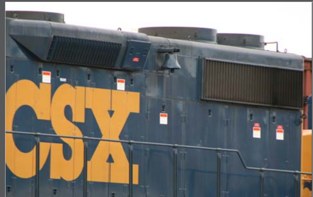
Figure 25: When purchasing a locomotive, each railroad had specific options that often were a ‘signature’ of the railroad. This hood-mounted bell was one option applied to Chessie System locomotives.
