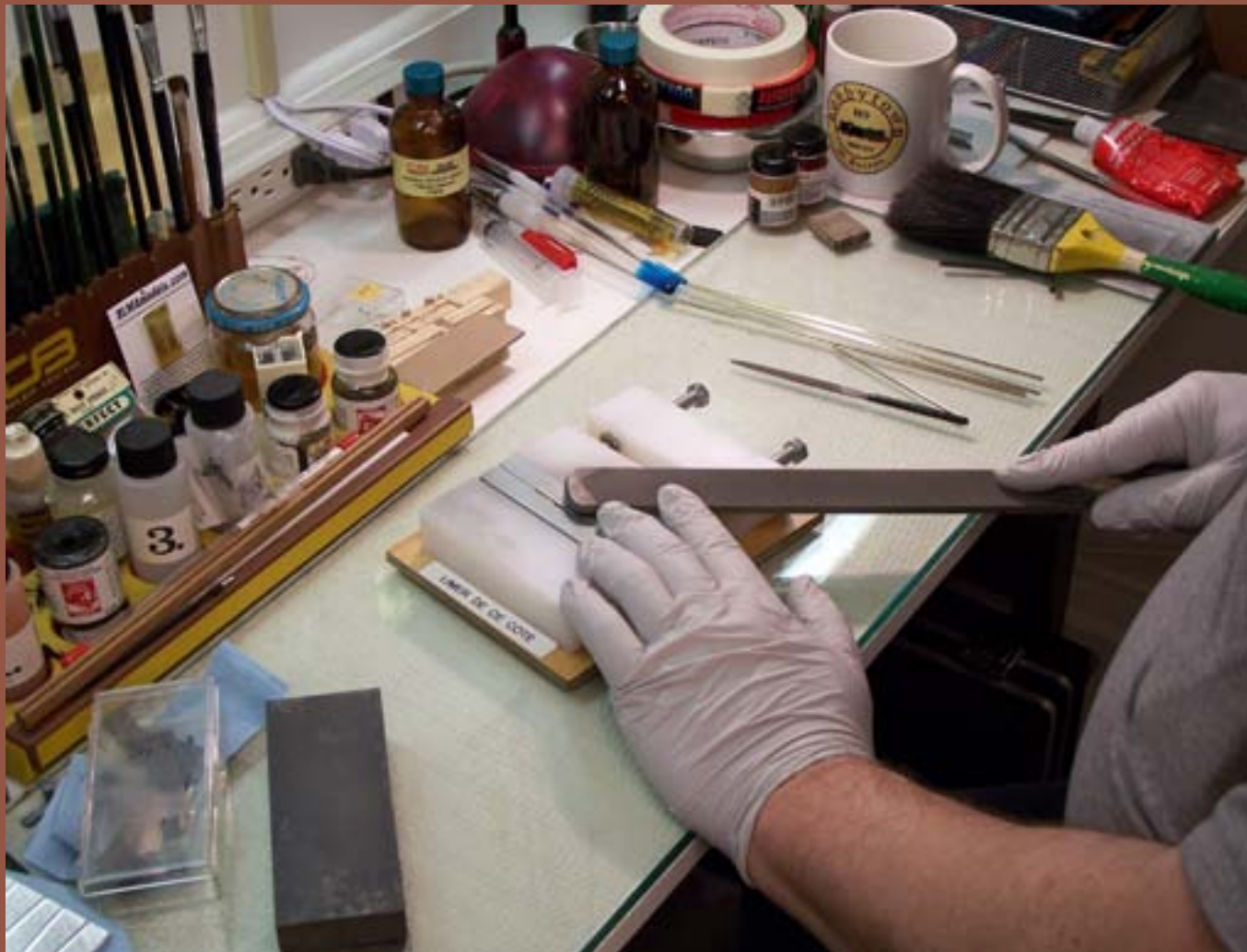
Figure 8: I filed the frogs and the points using the Fast Tracks point forming tool.
