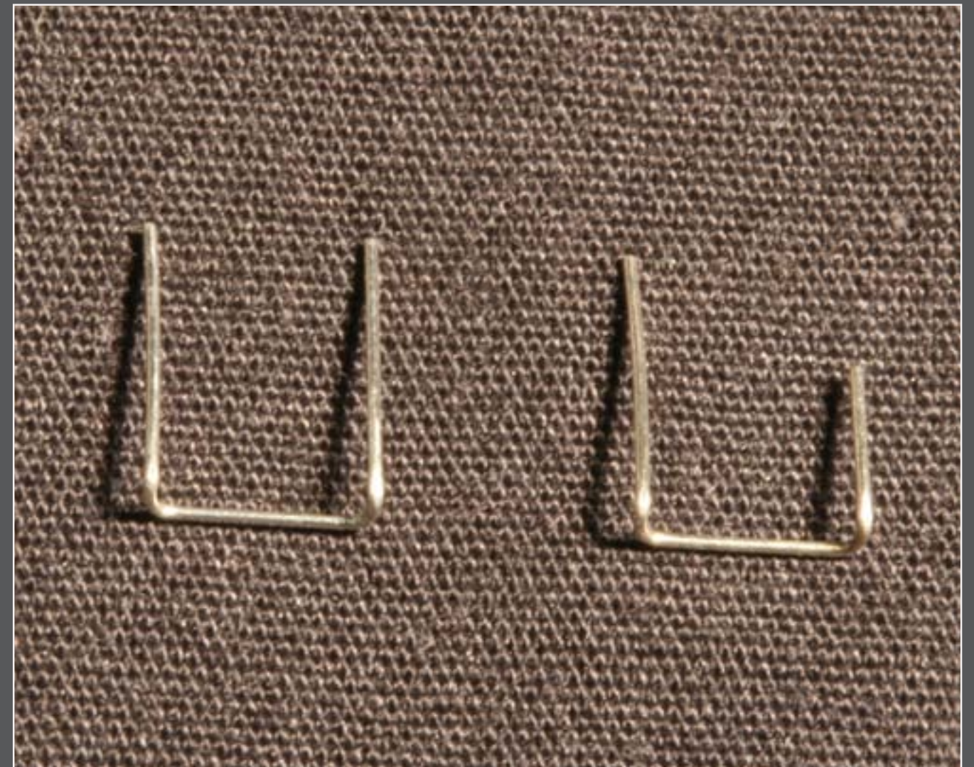
Figure 6: Cut one leg of a grabiron shorter to make it easier to mount.
