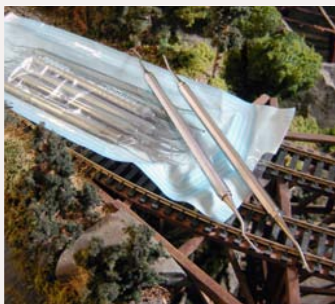
Figure 3: Assorted dental picks - useful for carving rocks or other scraping duties.
