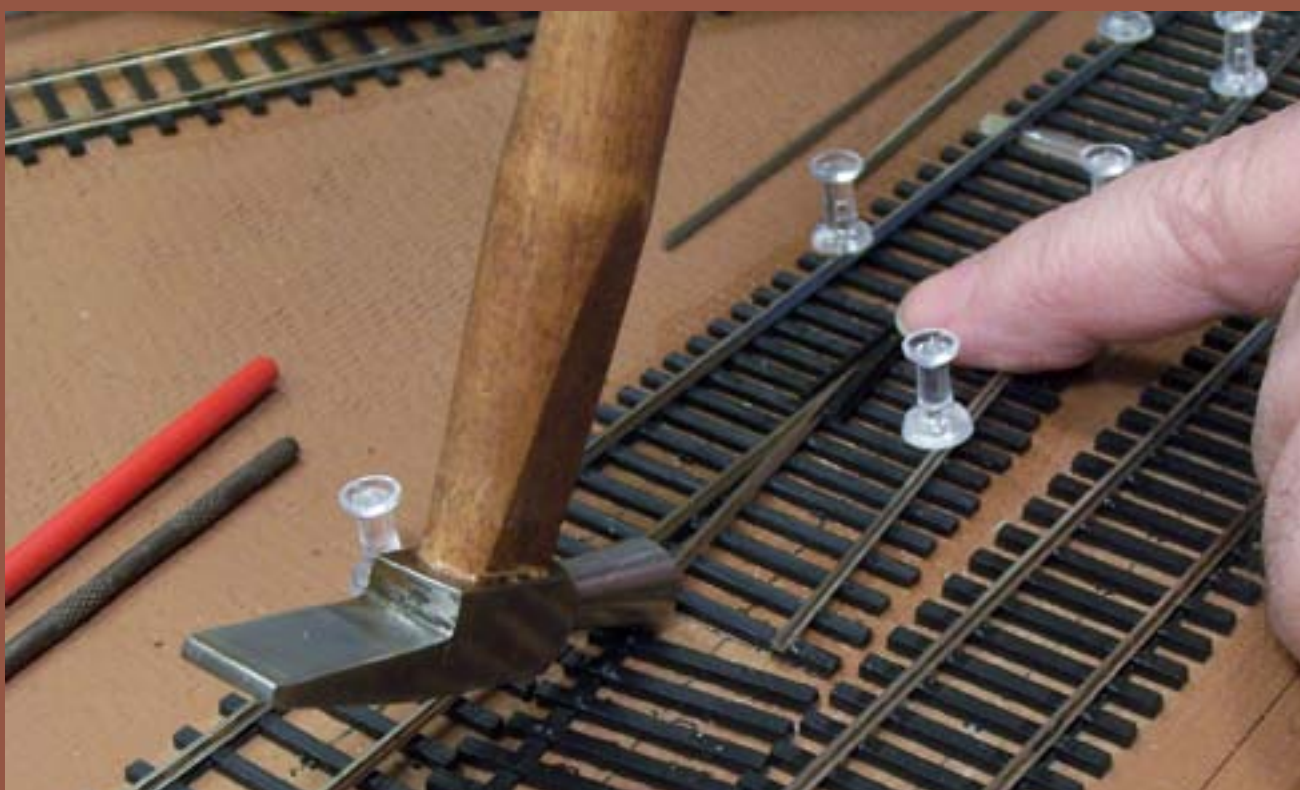
Figure 12: A few gentle taps seats the frog rails in the Central Valley frog casting. I prefer using this casting as well as Central Valley guard rails because they remain dark even after cleaning the track. Since they're plastic they won't shine like metal ones, for a more prototypical appearance.
