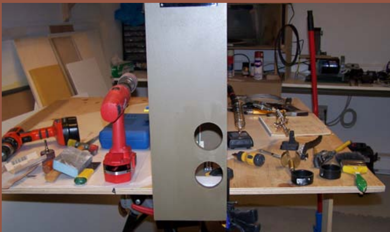
Figure 27: After careful sanding, I wound up with two perfectly sized holes.
