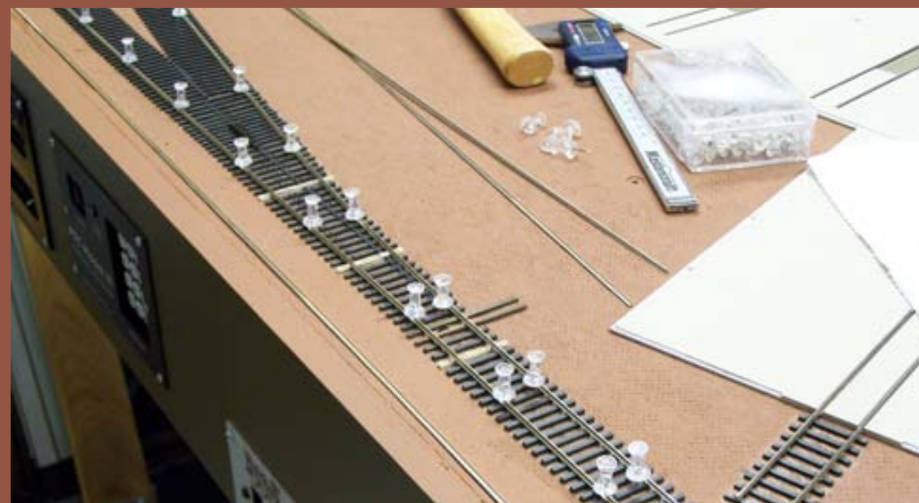
Figure 6: I measured and cut the stock rails. I like to use full-length stock rails as much as possible.
