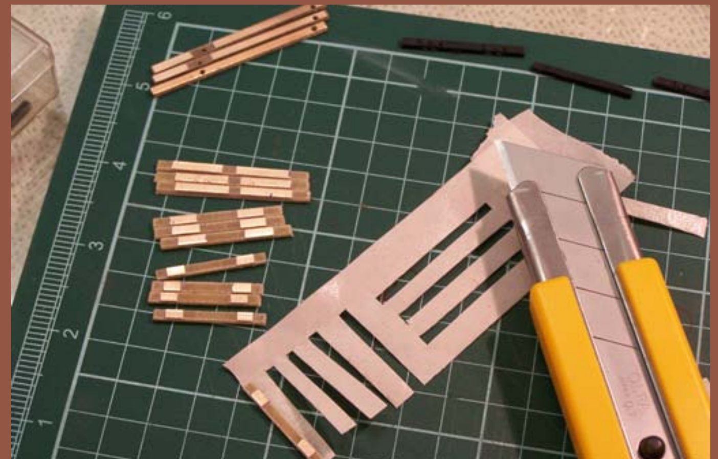
Figure 3: I prepared each tie by filing and adding two thicknesses of masking tape. This brings them to the proper thickness as I demonstrated previously in Part 2 of this article.
