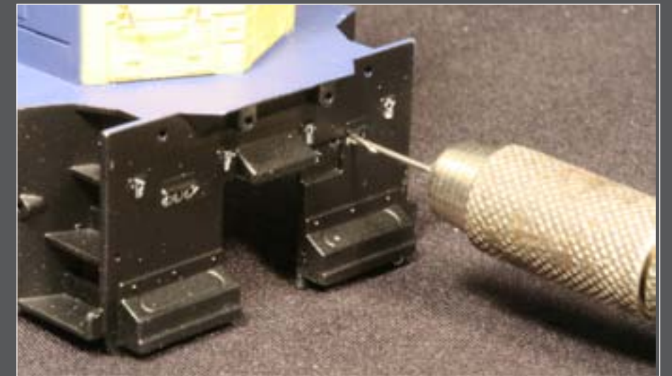
Figure 23: Adding MU hoses requires removing the ‘blanks’ cast on at the factory then mounting the hose castings into holes drilled through the blanks.
