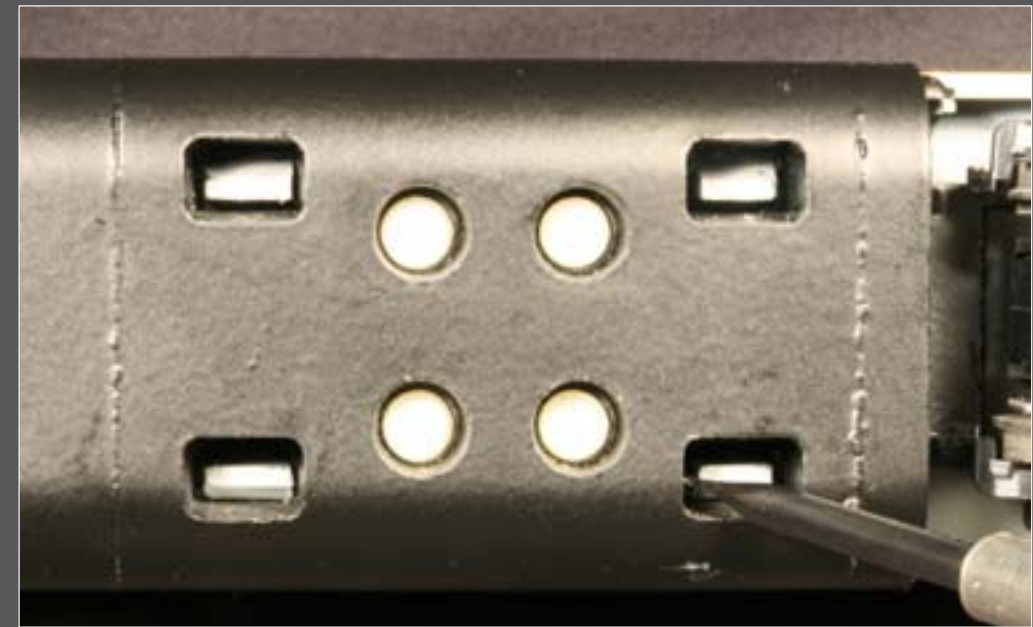
Figure 2: Athearn's blue box GP38, GP40-2, and GP50 models have tabs securing the shell to the frame. Removing the shell is as simple as pressing inward on the tabs while pulling the shell upward from the frame.
