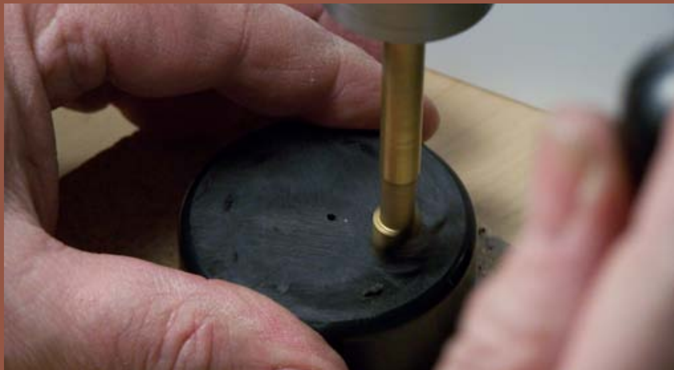
Figure 31: I countersunk the rear of each hole, using the pilot holes as references, removing just enough thickness so that I could install the hardware. Then I drilled a hole for each component.
