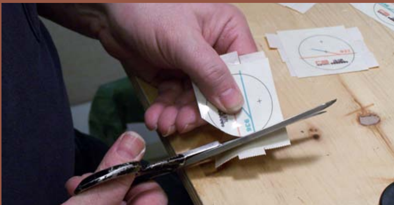
Figure 33: I laminated double-sided tape on the back of the labels and trimmed them to fit inside the end cap.
