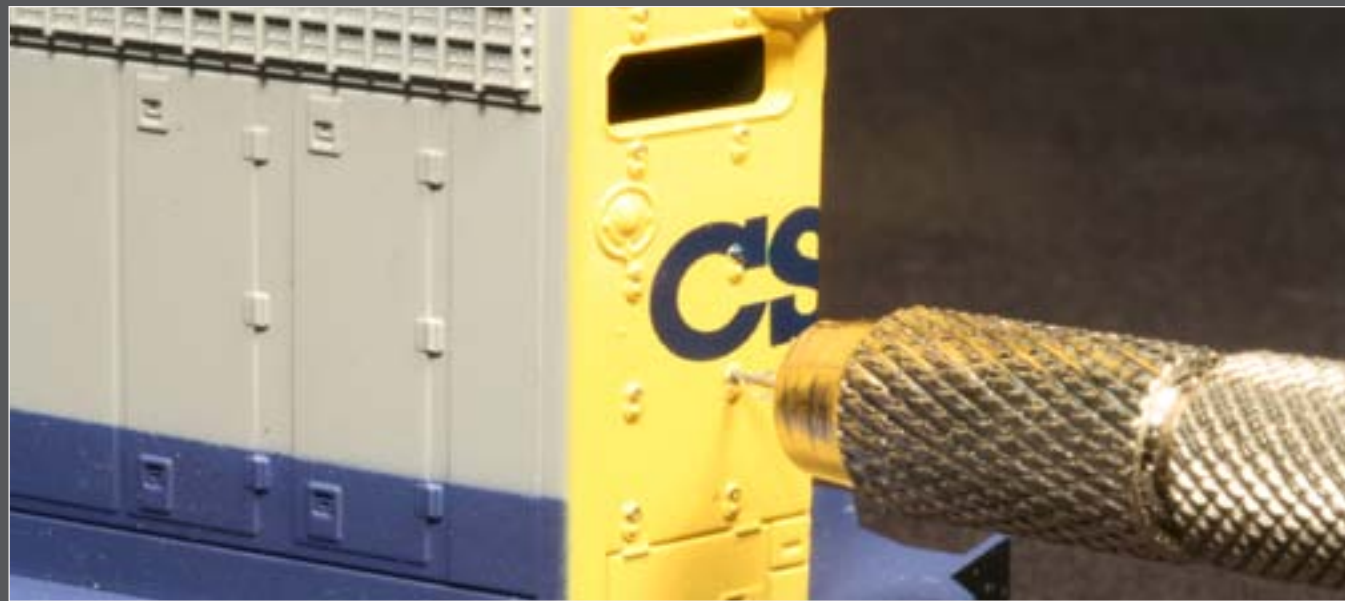
Figure 5: Many models feature a nut/bolt/washer cast into the shell plus a dimple where a hole should be drilled.
