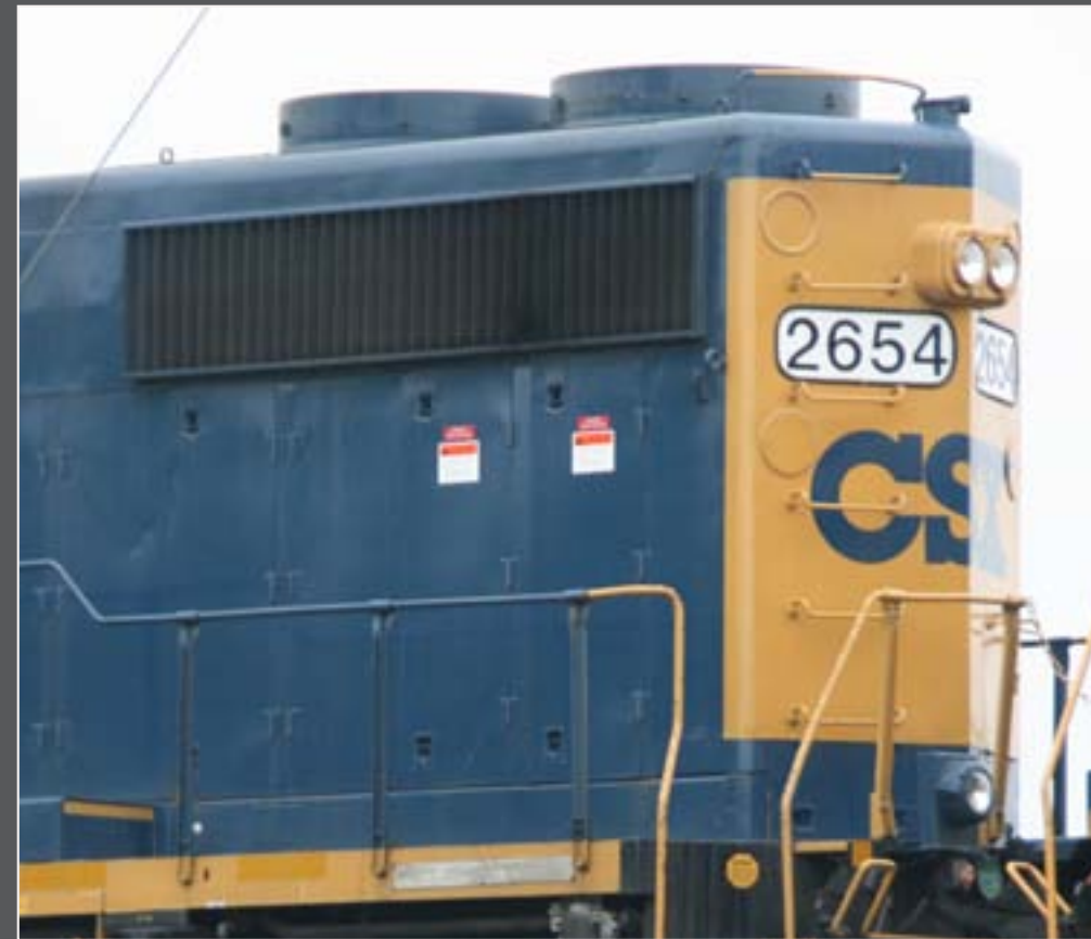
Figure 4: The photos of this CSX locomotive illustrate the placement of the grabirons at the front and rear of the locomotive. Using photos we can determine the accurate placement of these details.
