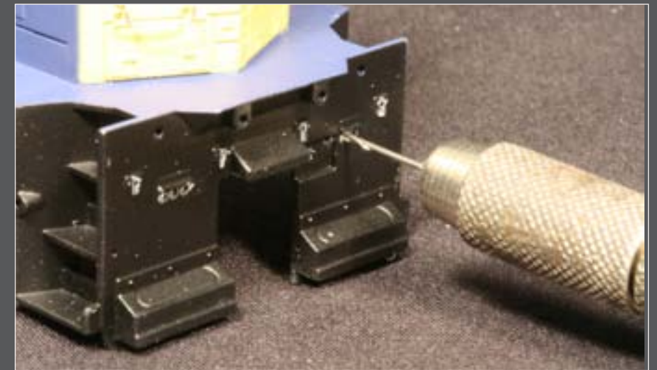
Figure 23: Adding MU hoses requires removing the 'blanks' cast on at the factory then mounting the hose castings into holes drilled through the blanks.
