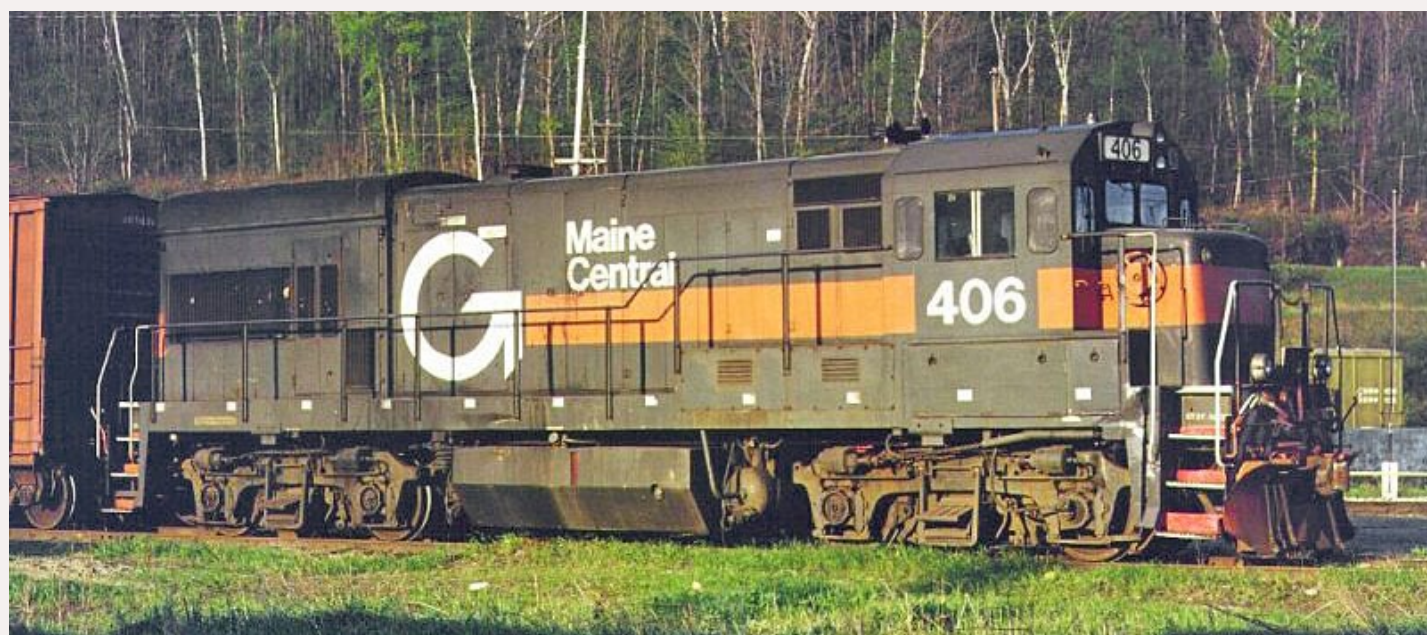
Figure 2: This prototype photo shows a standard late production U18, ex-MEC Guilford 406. For those of you who want to make the unit that is the most common, this would be your choice.
