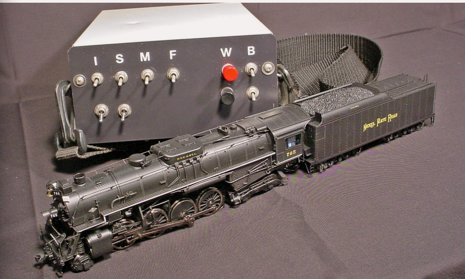
Figures 11 and 12: No steam engine is complete without the unique whistle and chugging sound of the locomotive. A portable sound box allowed the operator of this otherwise quiet locomotive to carry these unique sounds around the layout.
