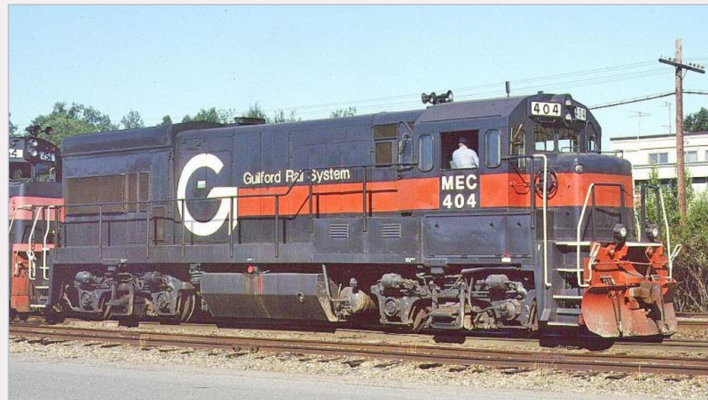
Figure 3: Because I can't resist a challenge, and like a unique model, the unit I modeled was GTI 404, which has a U25B nose that Guilford shop forces applied to to repair wreck damage. The nose has the distinctive class lights of a U25 located on the corners of the nose rather than squarely on the front of the short hood. Should you chose to do this unit, you'll need an old AHM U25C shell to get the correct class lights. The Stewart U25B shell is not correct for GTI 404. NOTE: As part of the kitbash for 404, I show how to recreate the seams that exist on the prototype where they welded the new nose in place!
