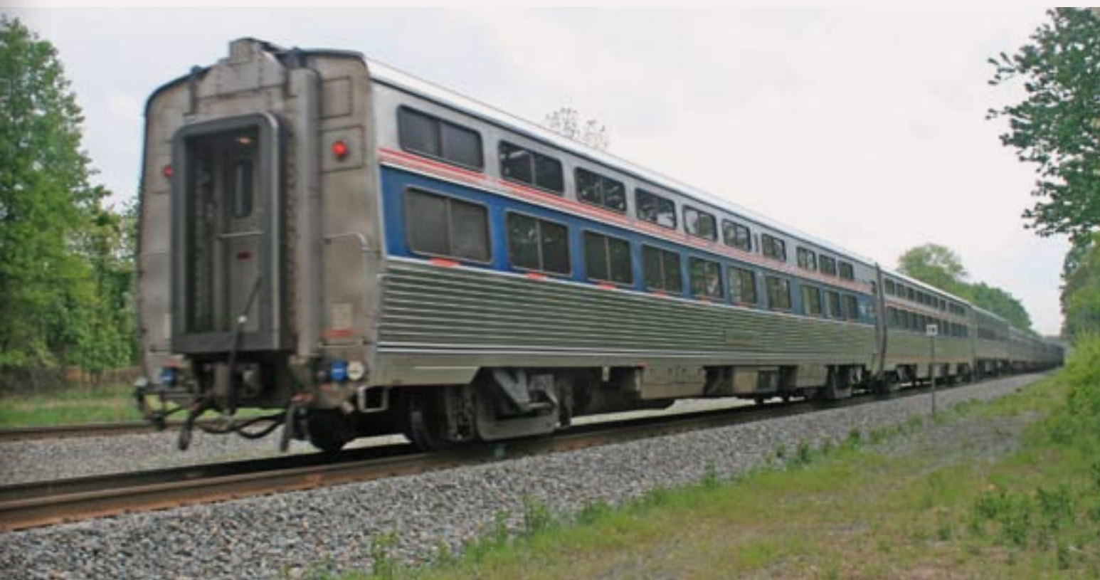
FIGURE 4: Showing off the unique paired windows that allow both occupants a view from their berths, two Viewliner Sleepers bring up the rear of the Silver Star.
