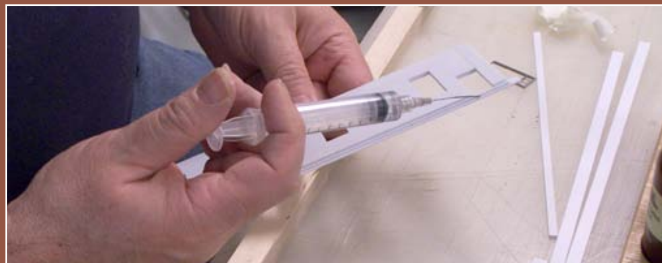
Figure 25: I use a syringe (available in pharmacies), with MEK (observe all cautions when using MEK) to weld my styrene pieces together. I prefer this method because it gives me more control over where the MEK ends up and it creates a very strong bond.
