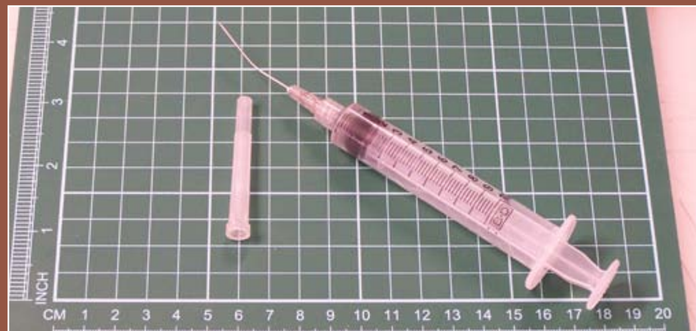
Figure 26: One trick I learned from the pros while I was working at my plastics supplier, was to bend the needle at an angle. This gives me much better control. With a little experience I can slide the needle along the joint and apply just the right amount of MEK without making an undue mess.
