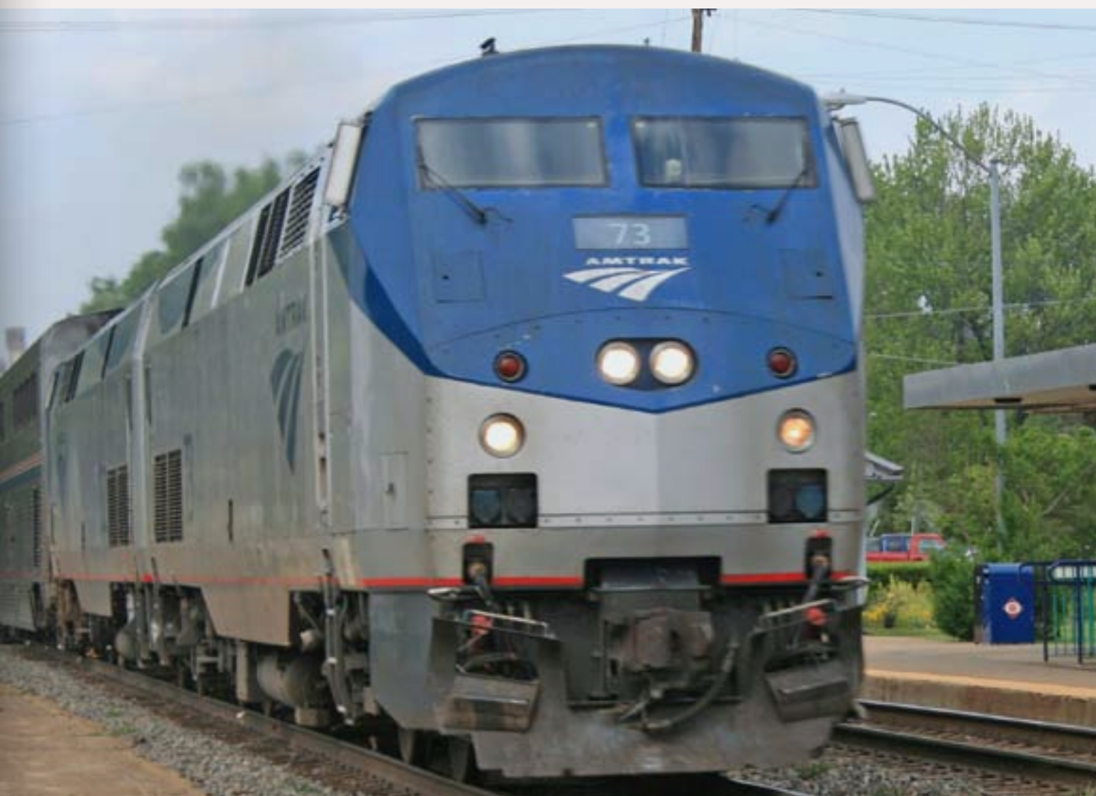
FIGURE 2: Amtrak #73, a P42 Genesis locomotive, heads south with the Auto Train and 33 cars.
