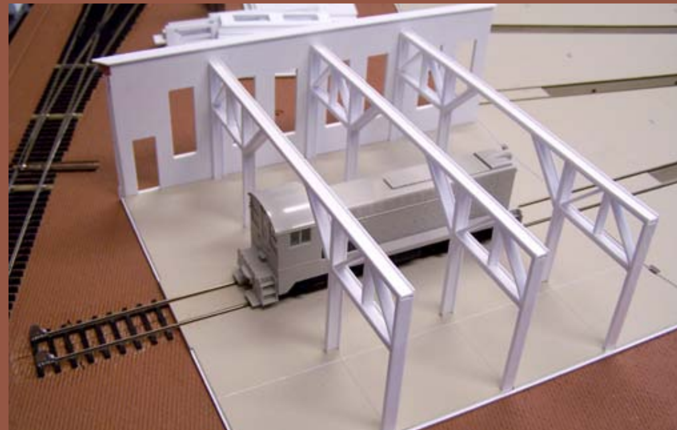
Figure 12: I built three trusses for the machine shop, using “I” beam and “C” channel strips from Plastruct.
