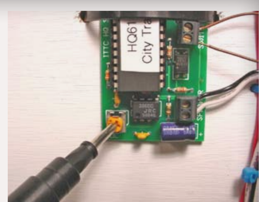
Figure 5: A speaker mounted under the layout will deliver the sound & controlling the speaker volume is easy using the variable resistor mounted on the module.
