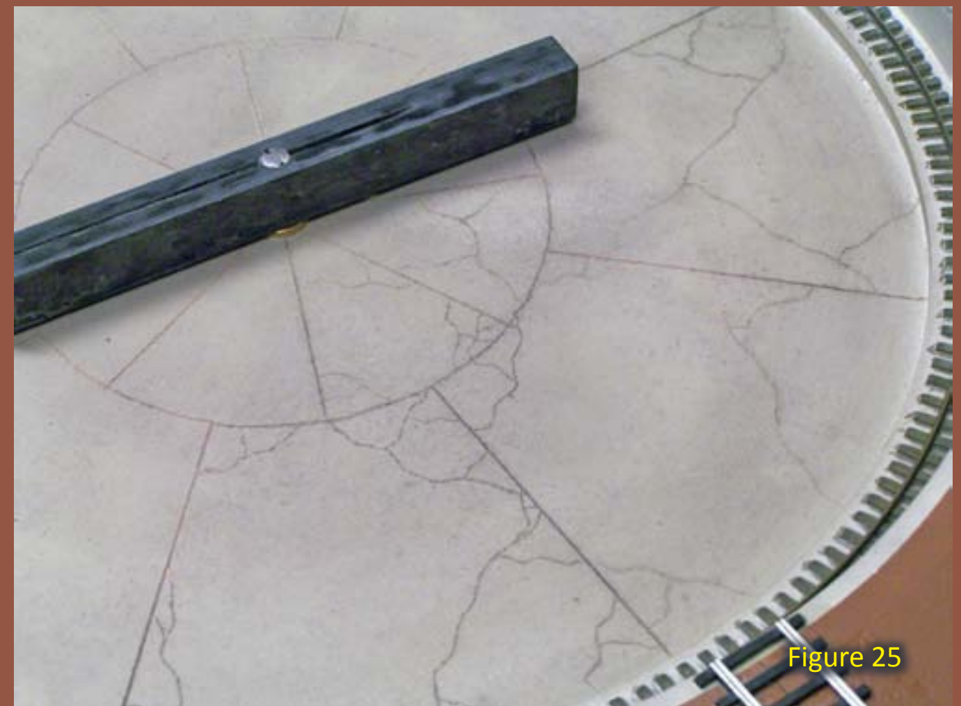
Figure 25: Using a Micro Mark scribe ( 50299 Tungsten Carbide Scriber ) I scribed cracks in the concrete (MDF) base in the Diamond Scale turntable pit.
