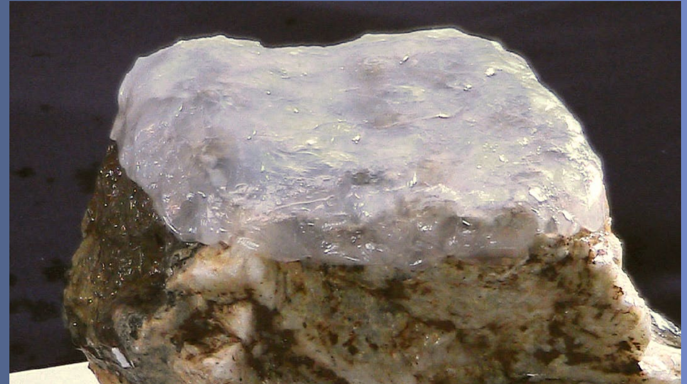
Figure 5. First layer of silicone smoothed out.
