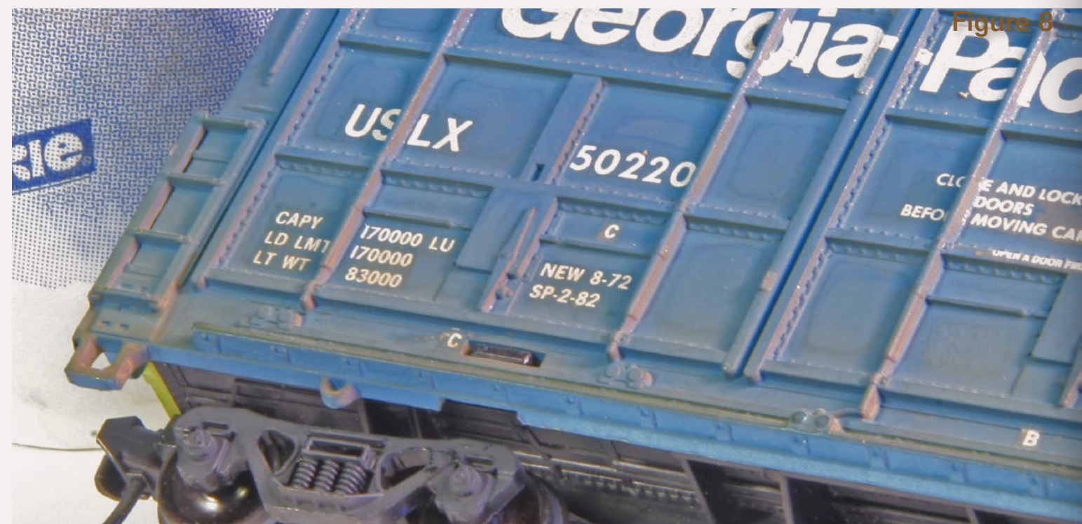
Figure 8: The results after the Dullcote. Notice the weathering looks a lot more subdued than it did in Figure 7. I happen to like the more subtle look of this weathering, but if I wanted something stronger, I would apply a strong second coat of weathering and then spray on more Dullcote. I sometimes add 3 or 4 layers of powder and Dullcote to get the look I want.
