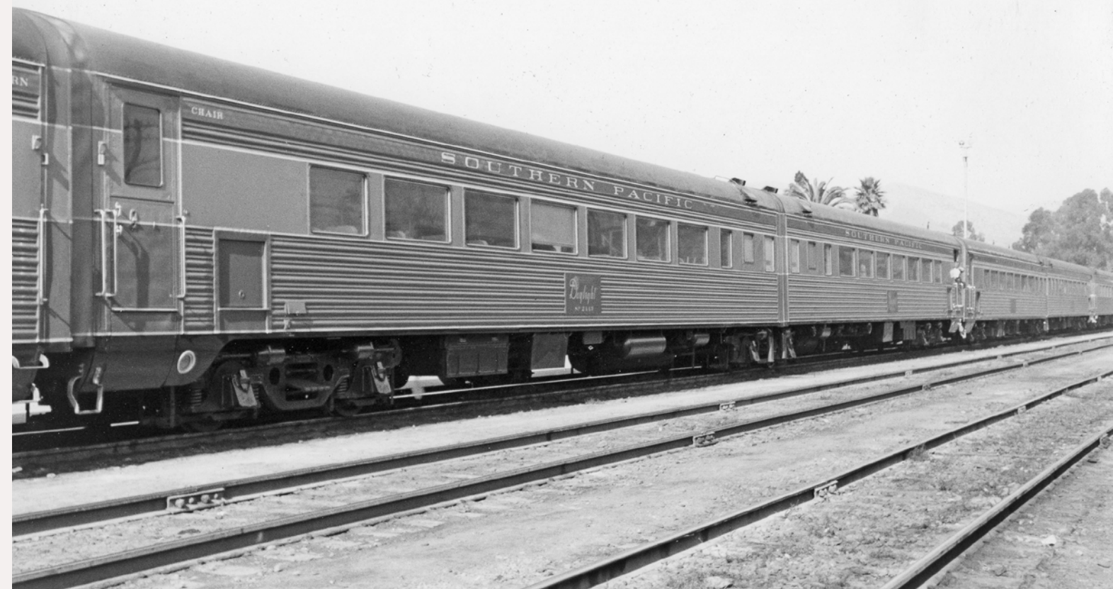
Figure 34: An articulated two unit chair car. The square recessed door next to the passenger entry is a dumbwaiter (also called a baggage elevator), it permits quick loading of passenger carry-ons without blocking vestibule steps at stations. The photo can be dated in the mid fifties – the car is still in Daylight colors but already has its skirting removed - photo courtesy Bob's Photos.
