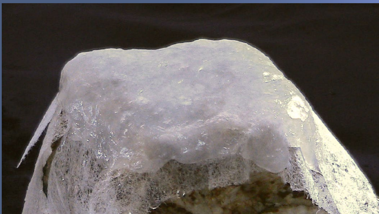
Figure 7. Applying second layer of silicone.
