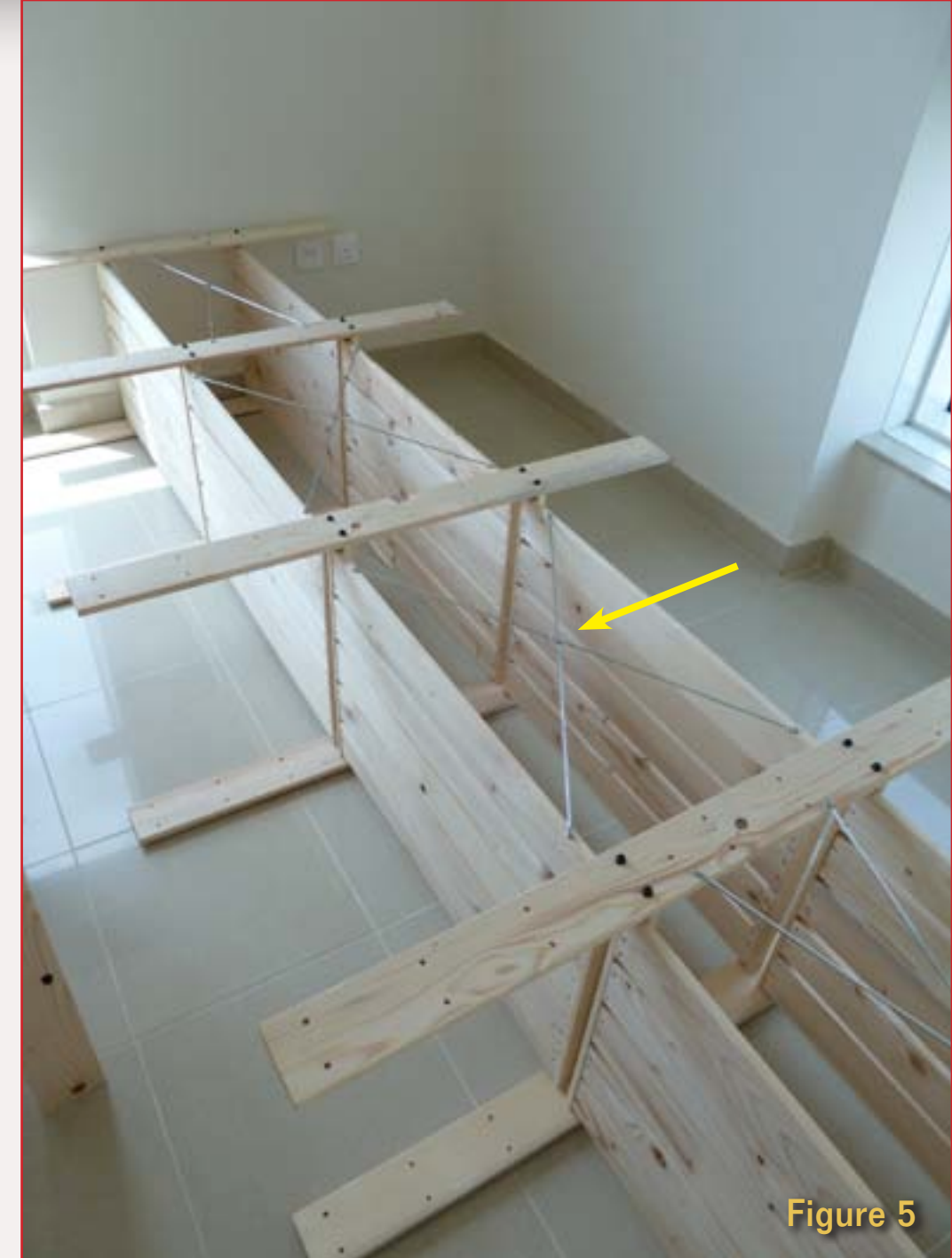
Figure 6: The metal cross braces didn't reach across every section, so I tied them into the shelves themselves. The one on the left is on the post, the one on the right, the shelf.
