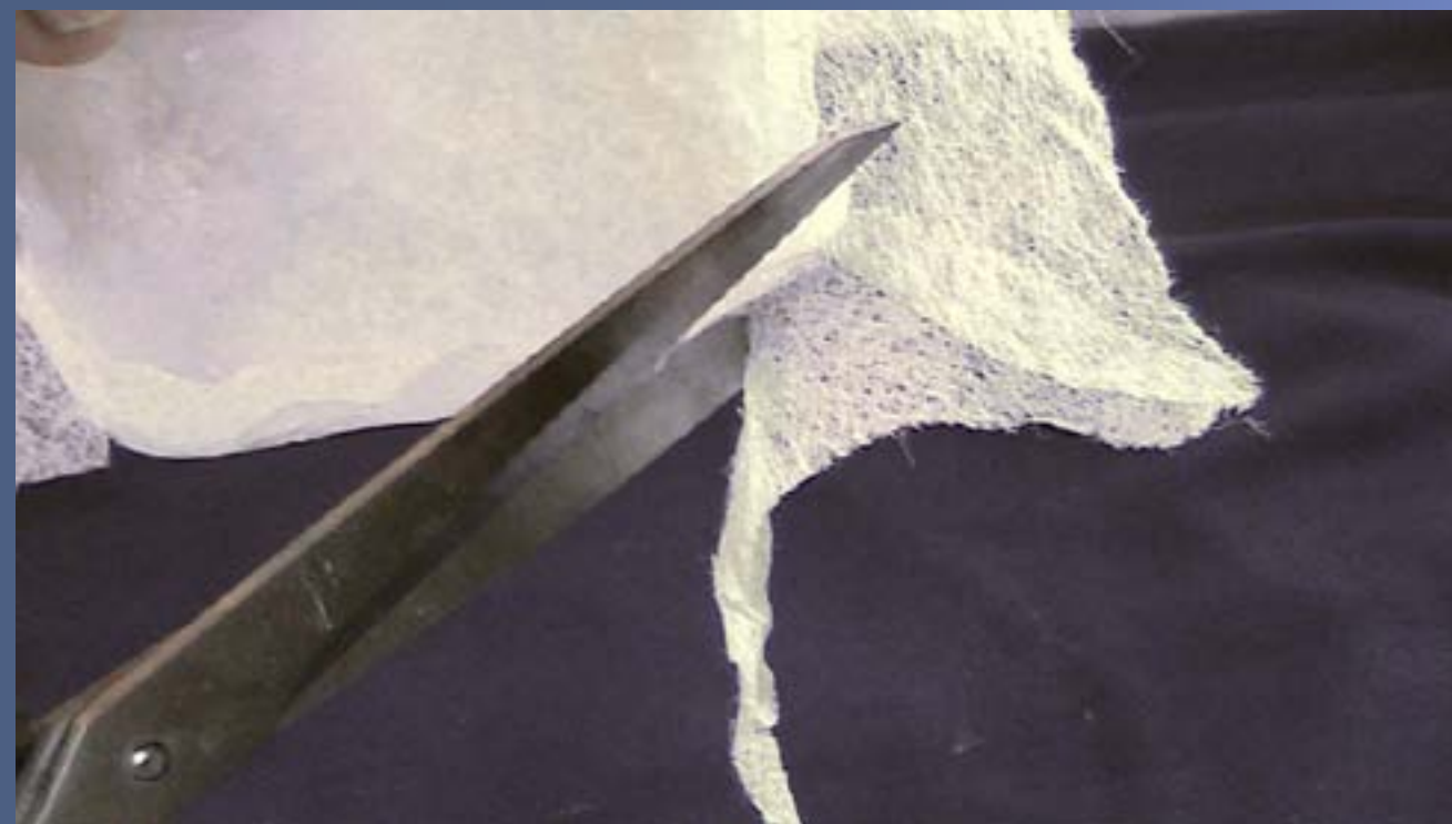
Figure 8. Trimming the mold.
