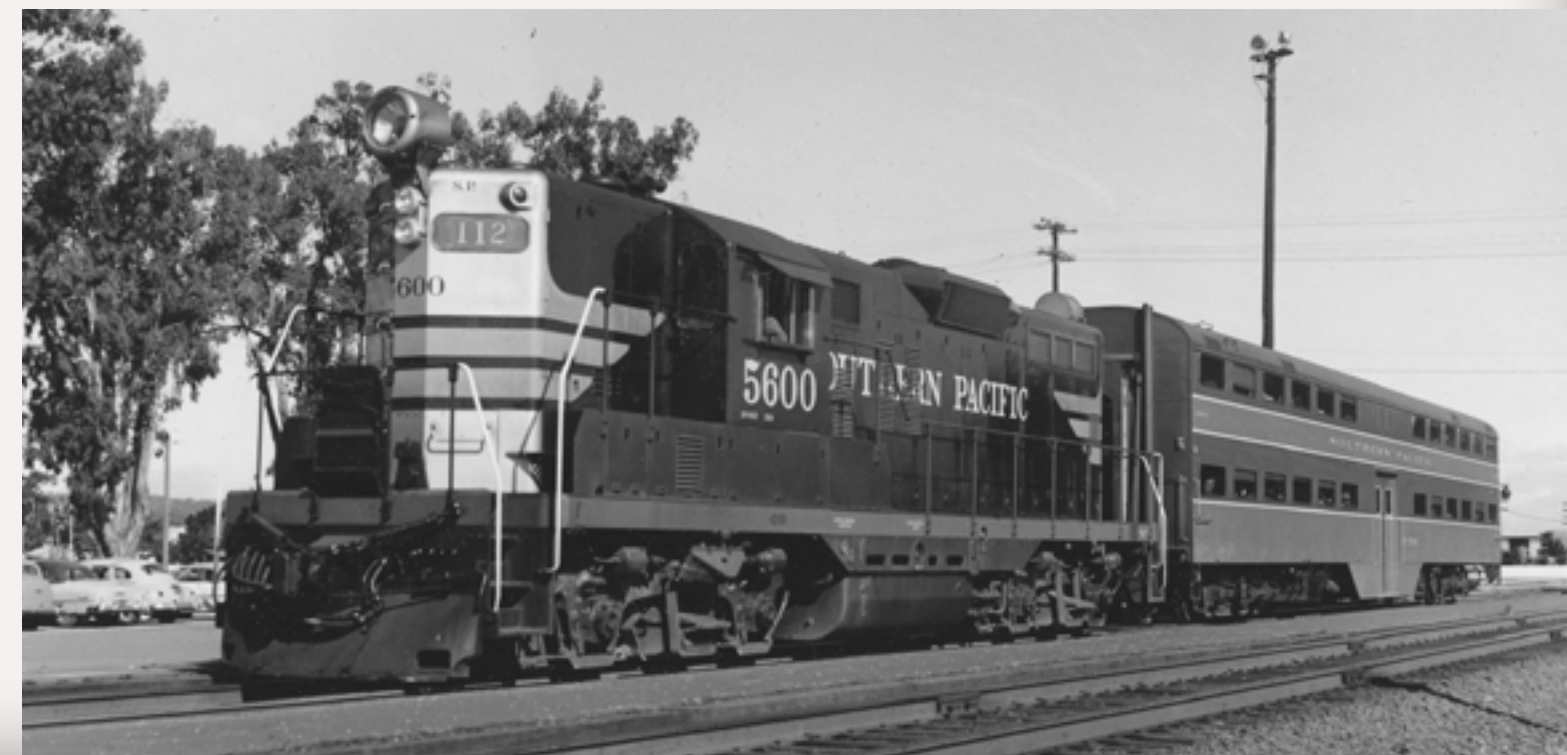
Figure 32: Engine 5600, a GP-9 in off hour commute service with a single gallery type bi-level car at Hillsdale, CA. The first group of SP passenger geeps such as this one had the older cast GP-7 handrail stanchions instead of the pressed metal ones used on most GP-9s. I missed this detail and will change my Proto 2000 models of this class - photo courtesy Bob's Photos.
