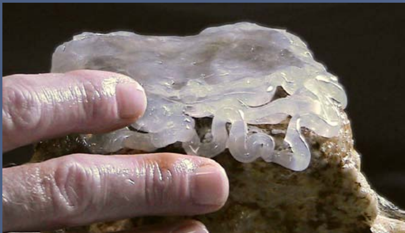
Figure 4. Patting the silicone into place.
