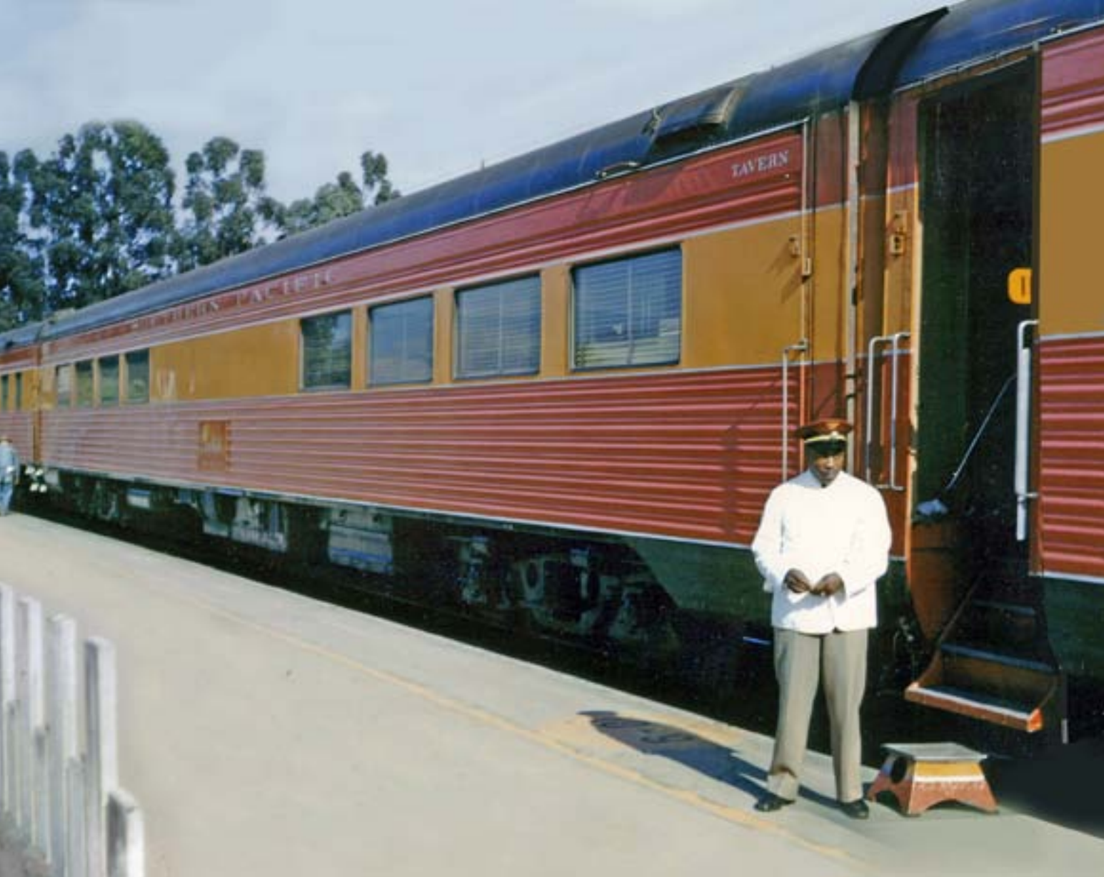
Figure 33: The Daylight pauses around 1955. A tavern car is shown with the car attendant of the parlor car on the right, with his Daylight painted passenger step. The door is swung inwards to open it, then the trainman or car attendant presses a foot treadle which lifts the vestibule trap cover (hinged floor section) and rotates the steps down into position - photo courtesy Bob's Photos.
