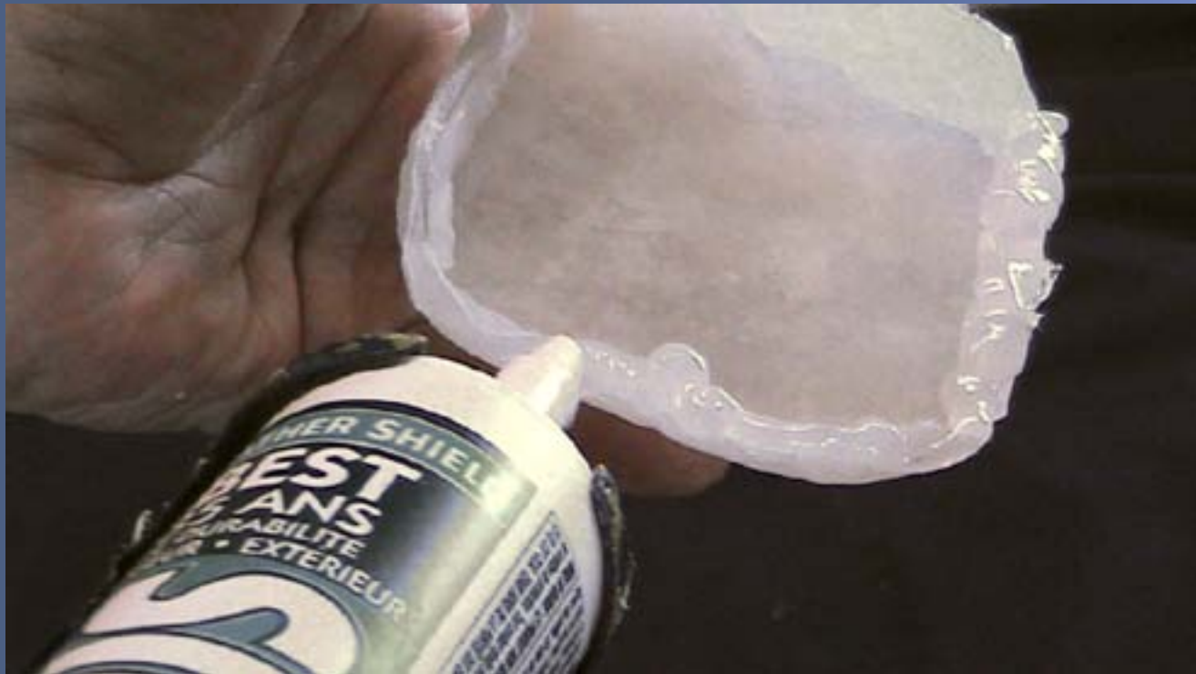
Figure 9. Applying the edge bead.
