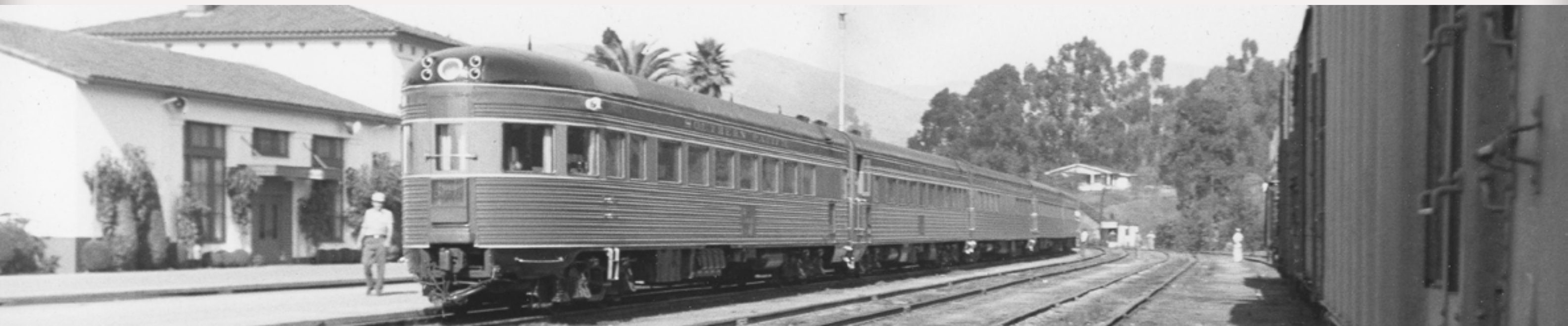
Figure 35: A mid 1950s view of the Daylight leaving San Luis Obispo, CA. This view shows the parlor observation car with its red neon tail sign. Notice the triple bolster trucks. San Luis is close to the mid point between San Francisco and Los Angeles. In the days of steam, locomotives were changed here - photo courtesy Bob's Photos.
