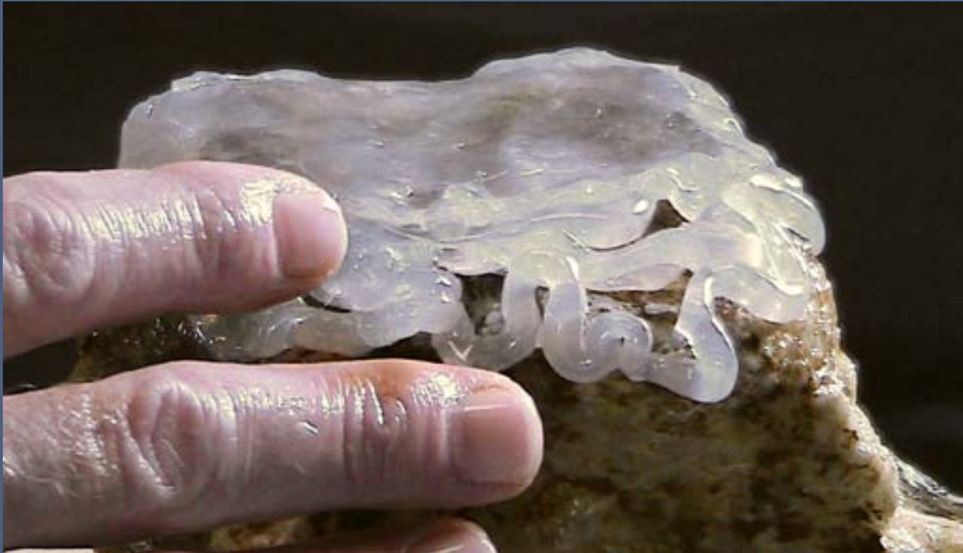
Figure 4. Patting the silicone into place.
