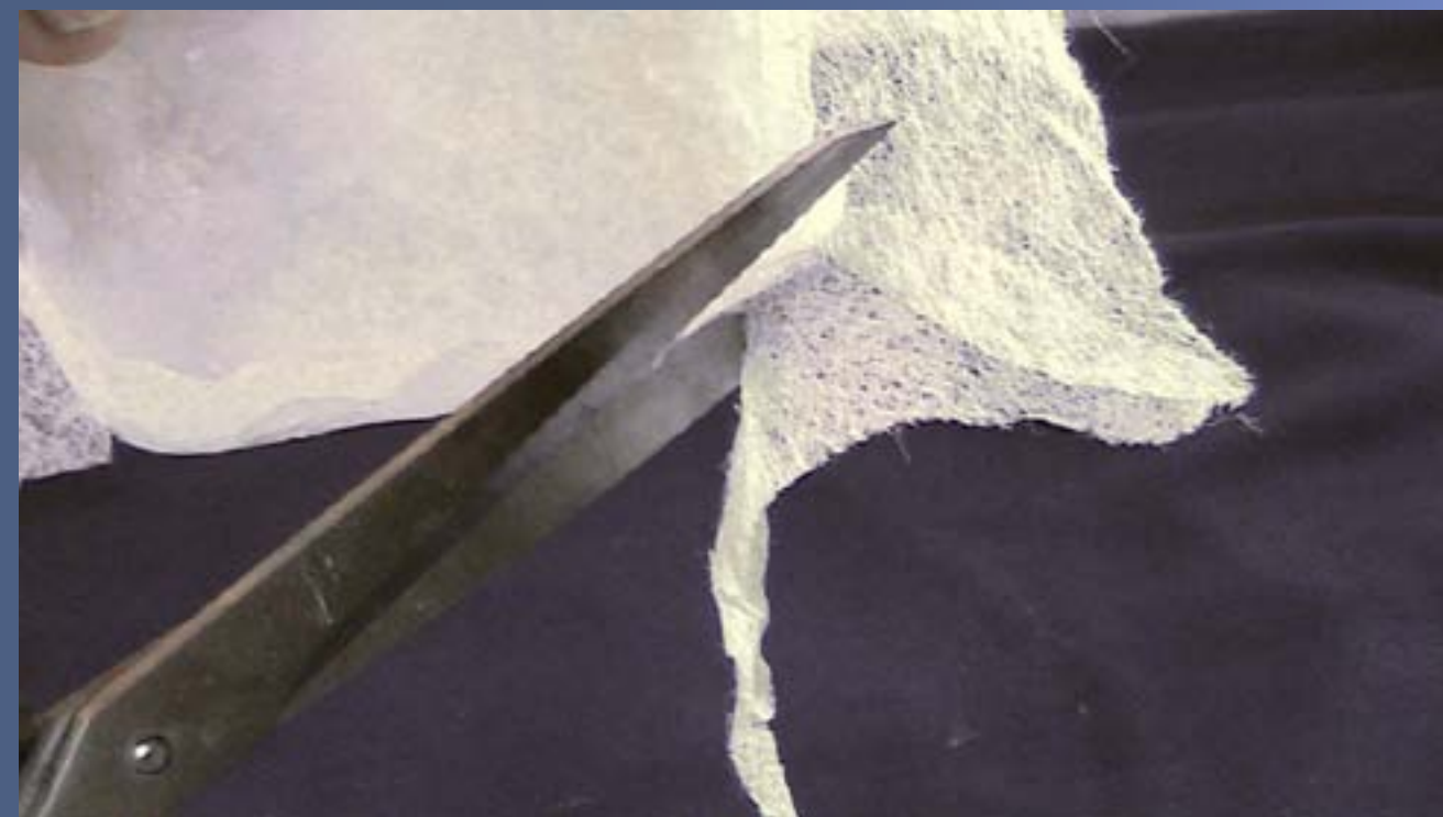
Figure 8. Trimming the mold.
