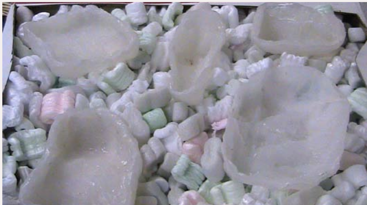
Figure 13. Foam “popcorn” keeps the molds level.
