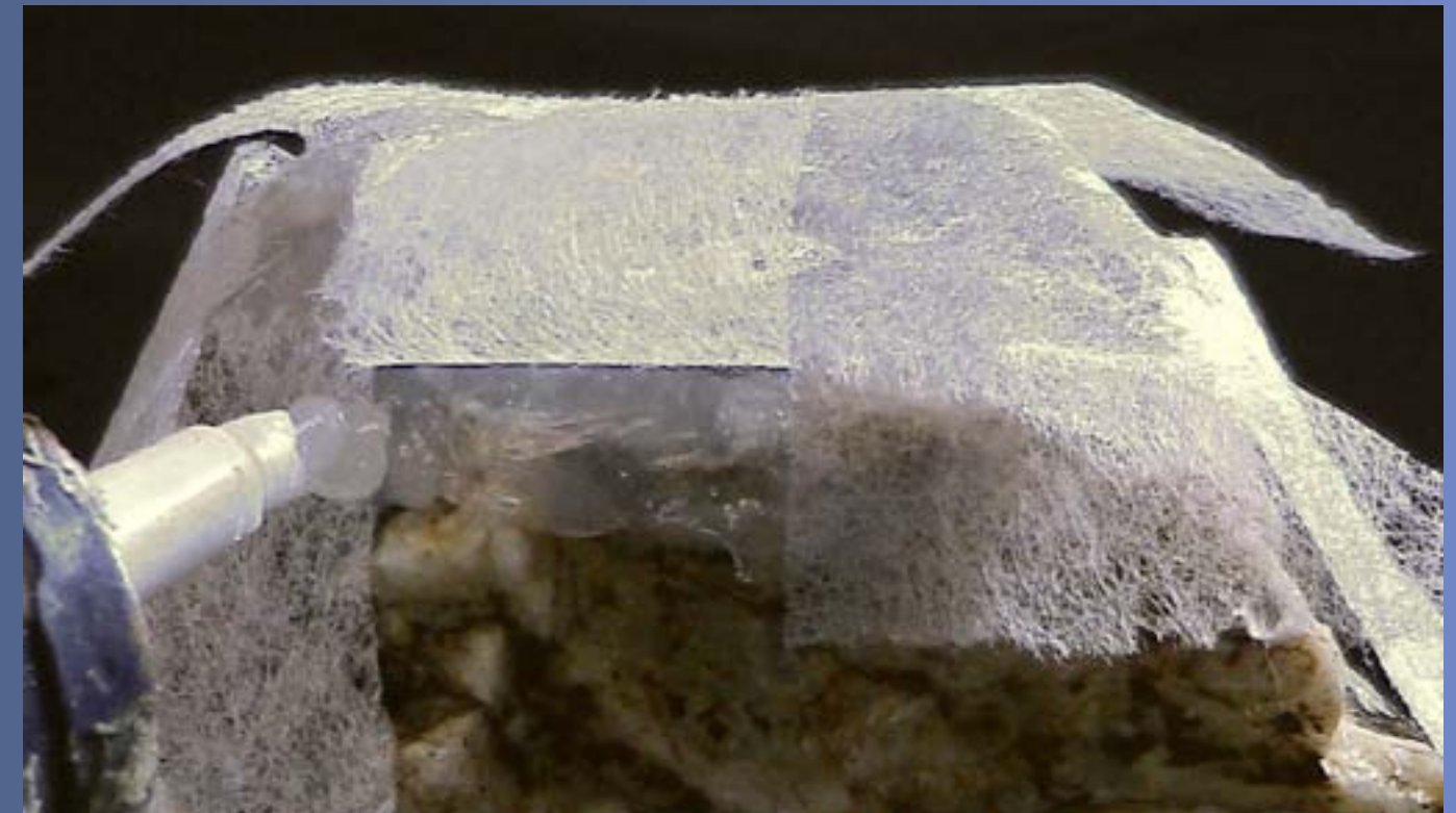
Figure 5. Folding and securing corners with silicone.
