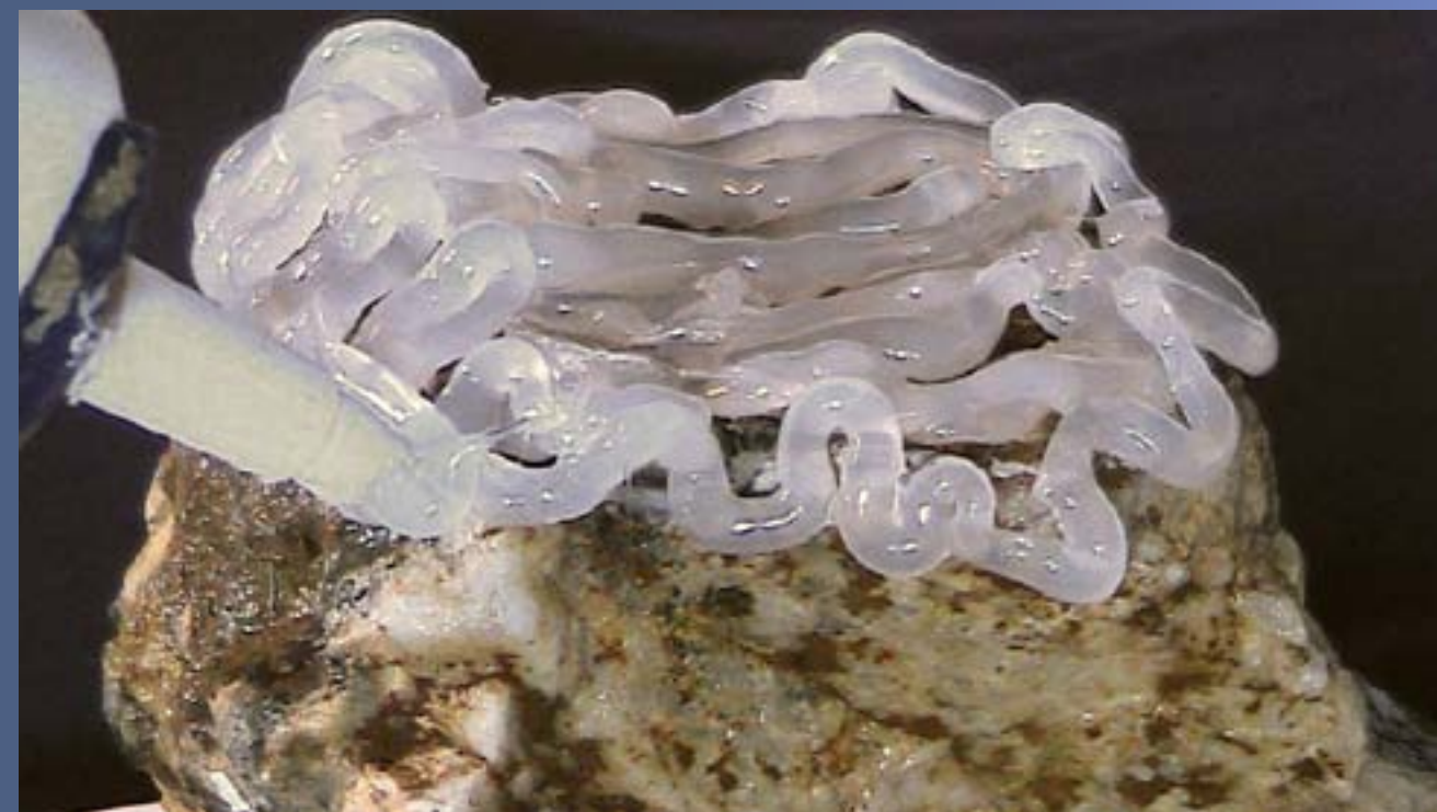
Figure 3. Placing silicone beads onto the wet master.
