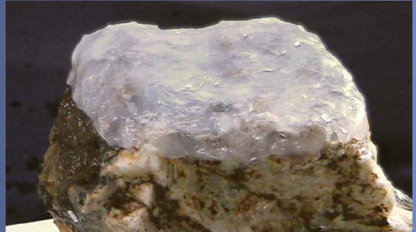
Figure 5. First layer of silicone smoothed out.
