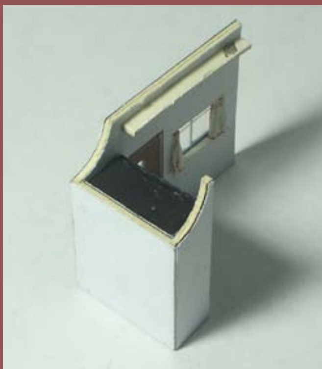
Figure 16. Kitchen area roof piece.
