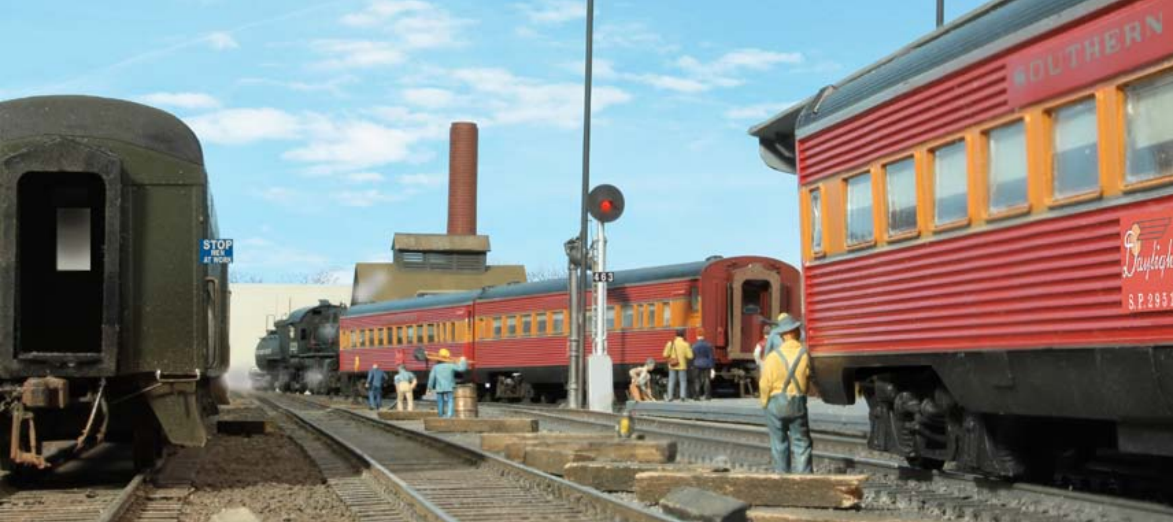
Figure 19: #1221 with its two chair cars backs onto 5 track, clearing the switch. The switch will be lined for the platform 5 track and the cars will be pushed into place on the Daylight. Next, 1221 uncouples and reverses, moving to track 4 where it can back to the roundhouse.
