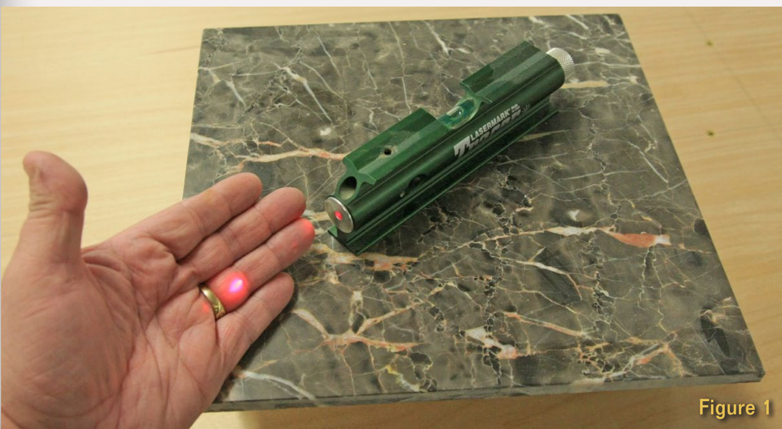
Figure 1: My ultra-simple laser-level platform.
