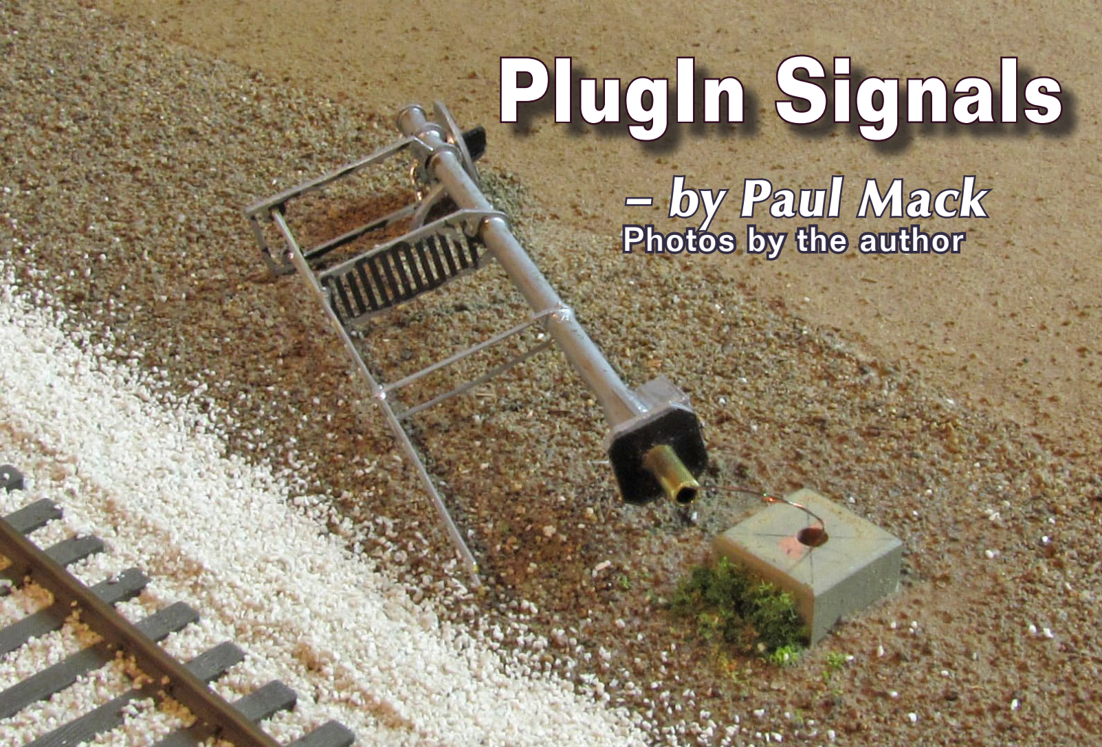
Figure 1: Signal is removed from its base showing the original mounting tube and wires going under the module.
