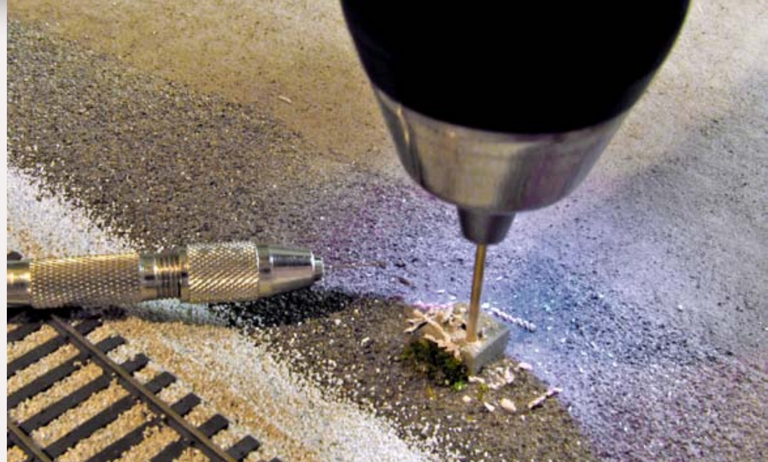
Figure 4: I used a 1/16 drill bit in a cordless drill to drill out the base for the header pins.
