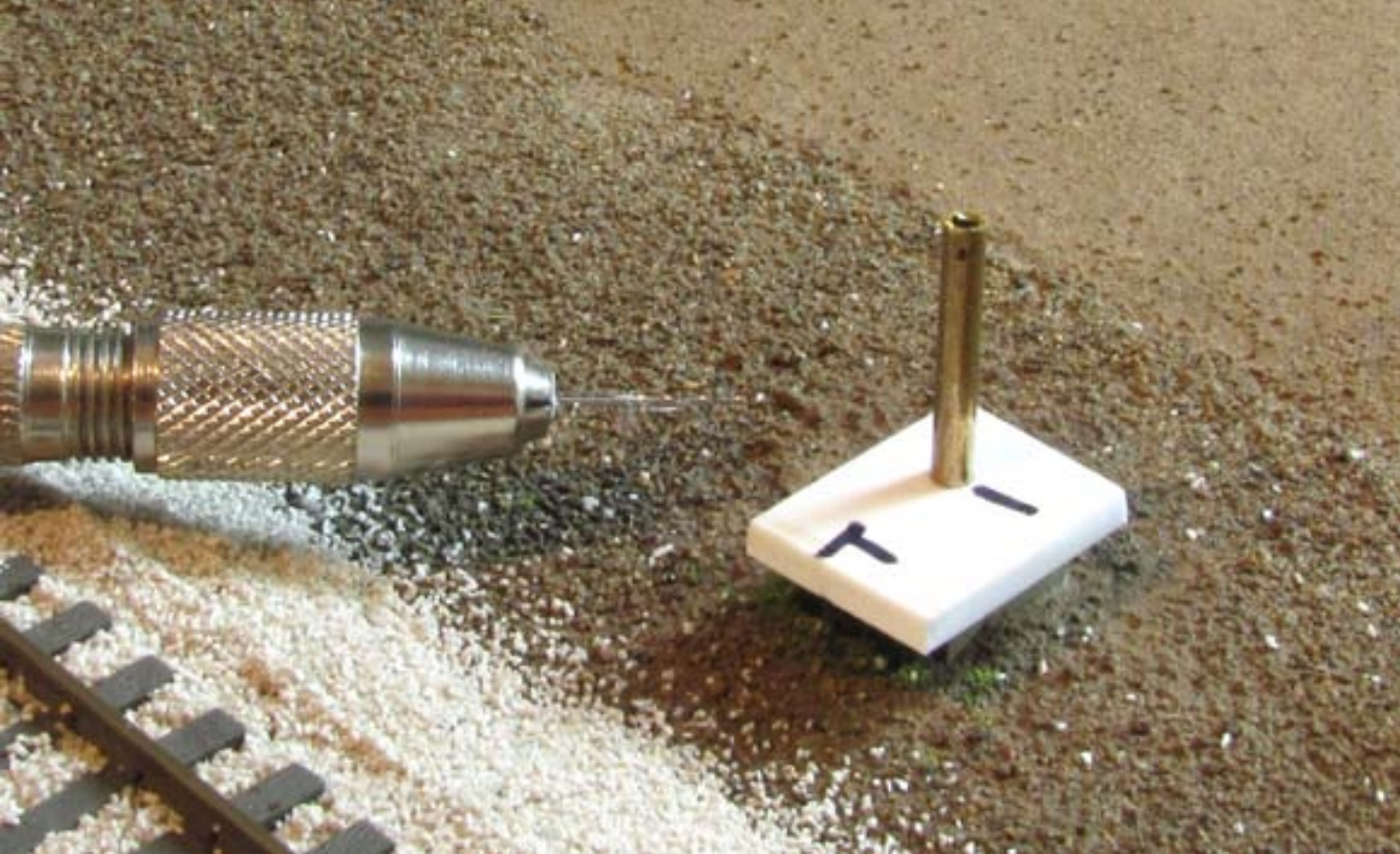
Figure 3: The signal base in photo 02 could be used, but there is room on the jig to indicate front and back so it is easier to keep track of alignment.
