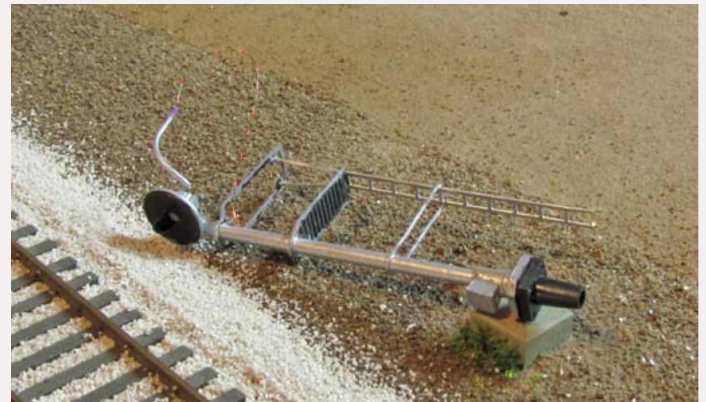
Figure 2: The signal mast has another Oregon Rail Supply base mounted to it for drilling where the molded on bolts are. The extra base was also used to make the jig in the next photo.
