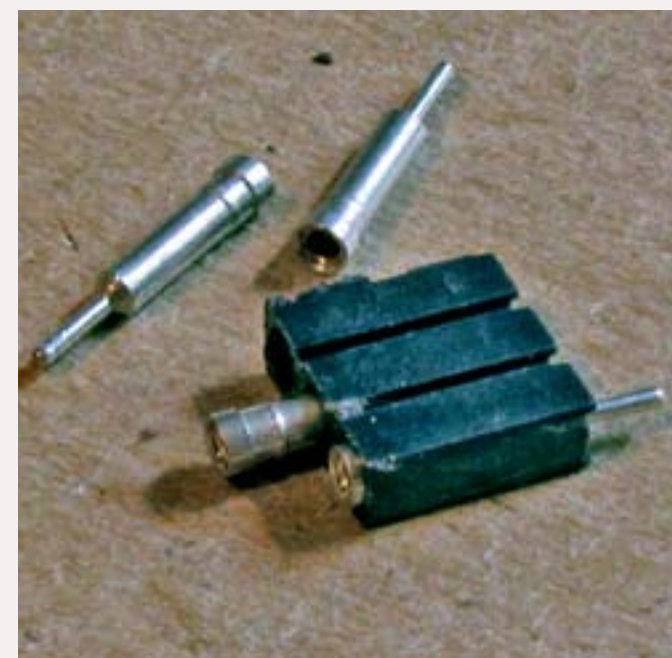
Figure 9: The header pins.
