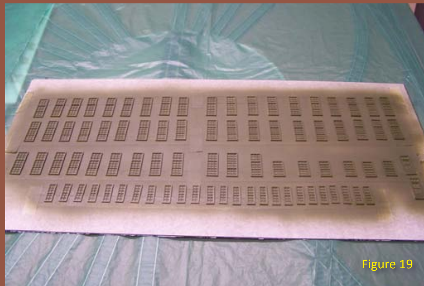
Figure 19: On the Tichy windows and doors, I used True Line Trains acrylic paint, I waited 24 hours before painting the opposite sides. The Tichy castings are grey styrene and do not require any priming.
