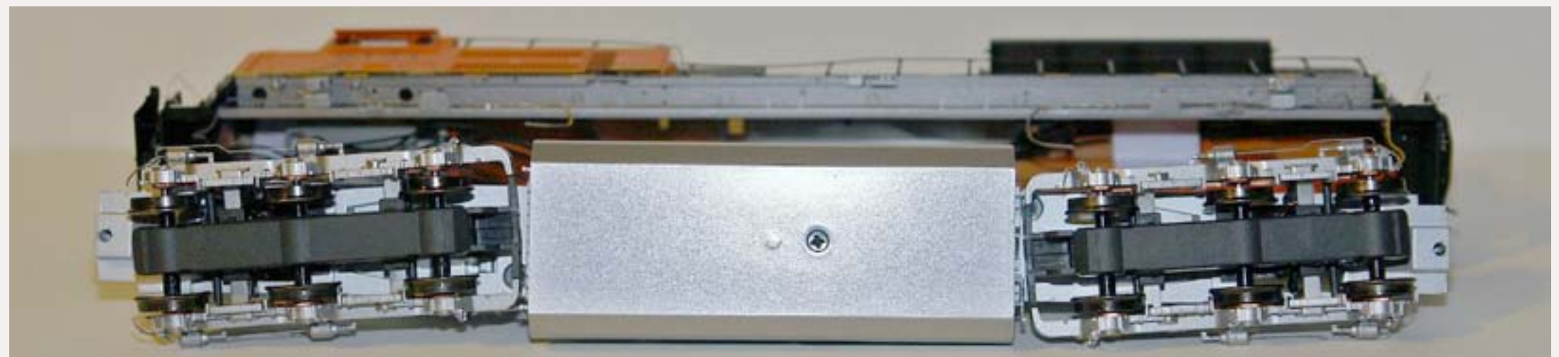
Figure 2: Bottom of chassis, showing standard Genesis trucks.
