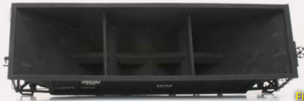
FIGURE 8a: EBT #1074 4-bay hopper was kitbashed from Quality Craft Models 3-bay hopper kits.
