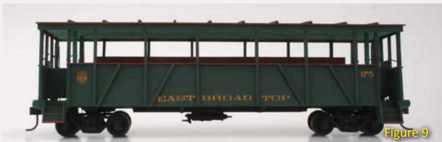
FIGURE 9: EBT #175 tourist open passenger car with a roof. This car was kitbashed and scratchbuilt from strip wood and uses the roof and floor from a Quality Craft Models outside braced wooden box car kit.
