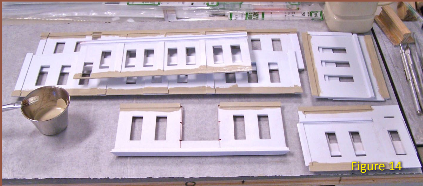
Figure 14: I used my usual latex concrete color for the foundation, applying it liberally because I knew I would need to mask them before applying other colors or the brick paper.
