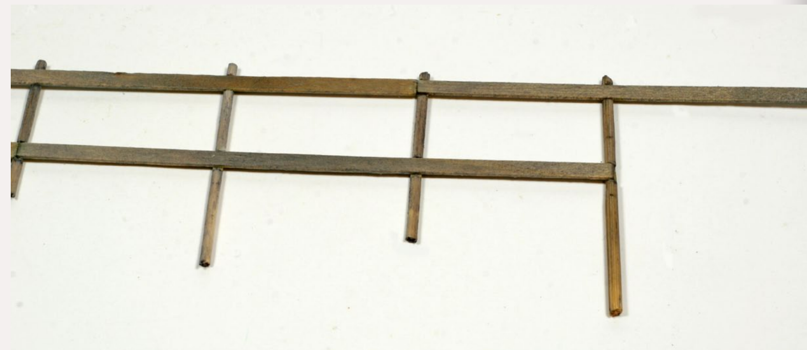
FIGURE 9: The post and stringers are shown stained and assembled. Joints in the stringer are located over a post but always splice the upper and lower stringers on different posts.
