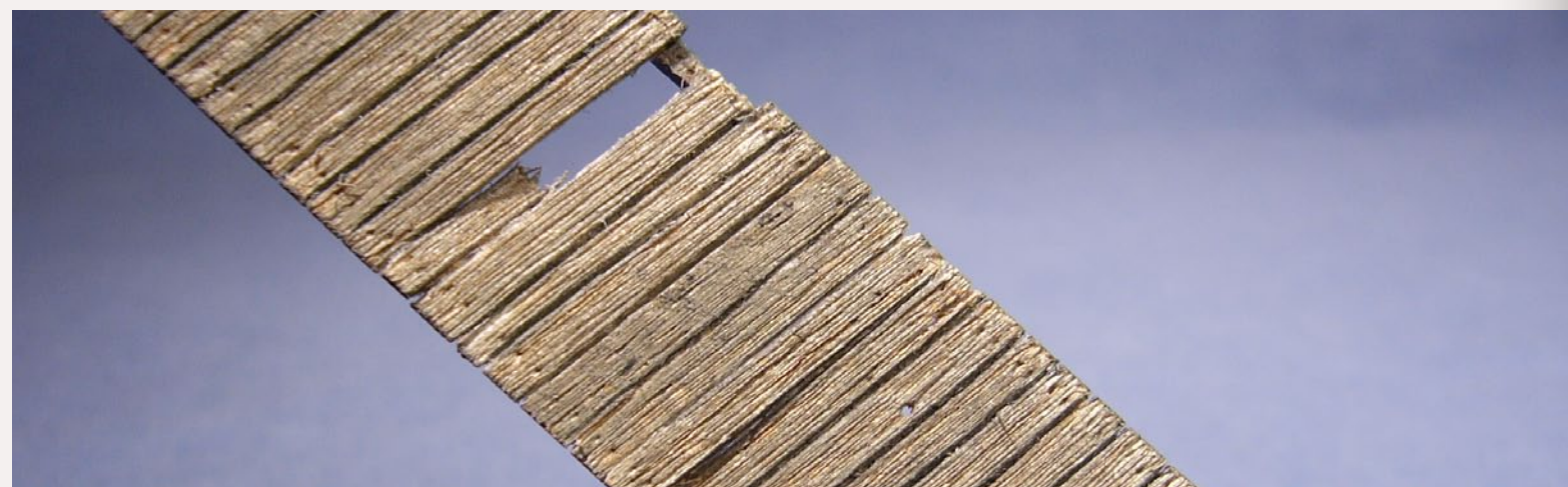
Figure 5. Cut away and lift a few planks with an X-acto knife, create knot and nail holes with a dental pick, a pin or a small awl, and stroke a brass bristled brush along the grain to deepen the effect. Be careful not to overdo the brass brushing as balsa wood is very soft.
