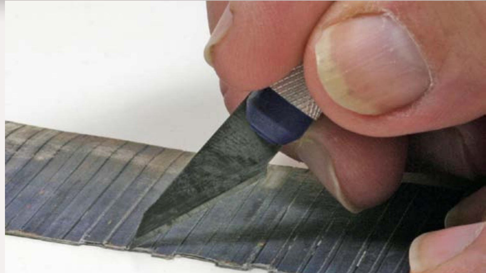
FIGURE 4: The tops of the fence boards are trimmed so that some of the boards are longer than others. Don't overdo this feature, less is more.
