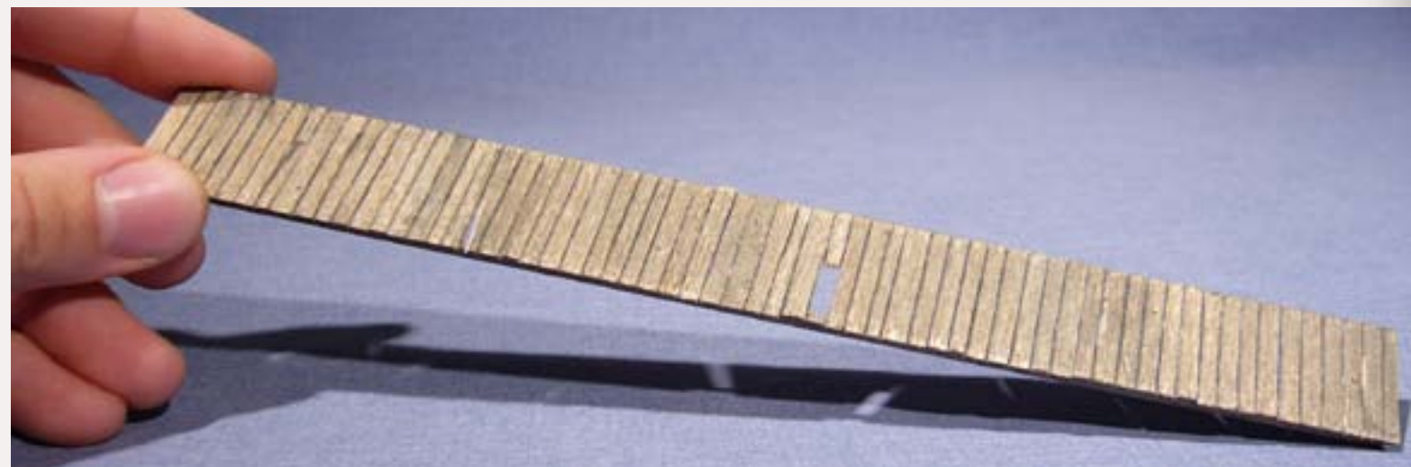
Figure 4. I created a long platform by gluing several balsa sections on top of long basswood strips. At this stage I enhanced the illusion of individual planks by notching the edge of the wood between the lines to vary the length of the 'planks and removing a plank or two.
