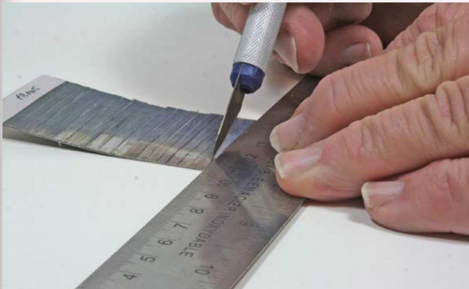
FIGURE 3: The Clever Models weathered boards are color printed on heavy card stock and two sheets are glued back-to-back so both sides of the fence will have detail. After cutting the fence strip from the master sheet, a dull blade is used to indent the lines representing the individual boards, and a darning needle indented the nail holes.
