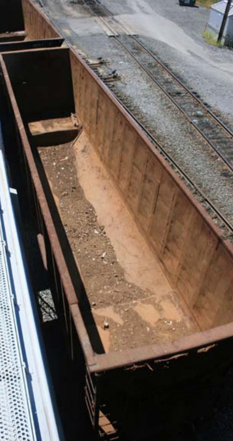
FIGURE 2: This rotary dump hopper shows the remains of its previous load, in this case dirt and gravel.
