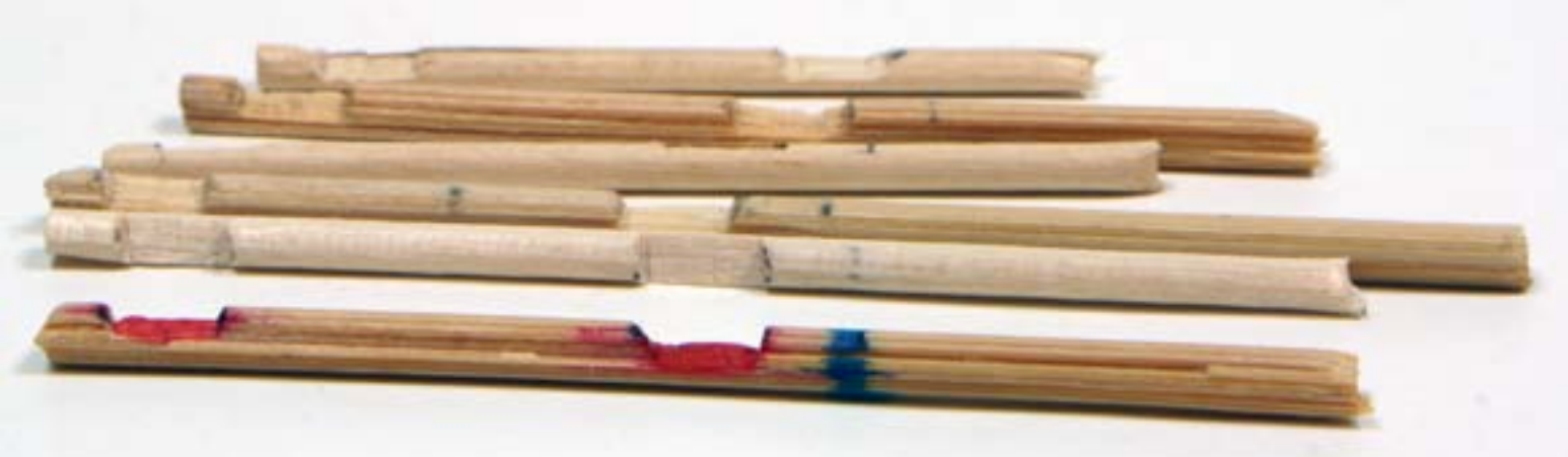
FIGURE 2: These posts were cut from 1/16" birch and bamboo skewers. I like the bamboo as they are stronger and easier to shape. They are a little bigger than the birch and need to be shaved down. The (red) notches are cut the width of the coffee stirrers used as the stringers, and the depth of the cut is deep enough that the 2" X 6" stringers are flush with the post. Stain all the boards at this step.
