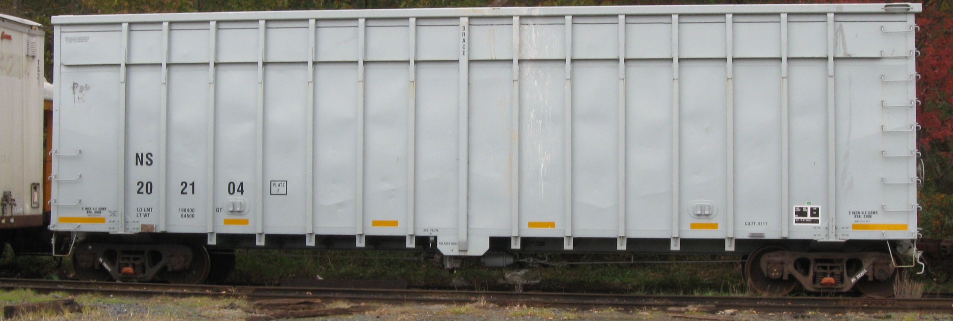
Figure 1: This NS C&D hopper looks like a “new” car, however close examination reveals the outline of the dual hopper bays, giving away its heritage as a former Airslide covered hopper (see all 3 pictures).
