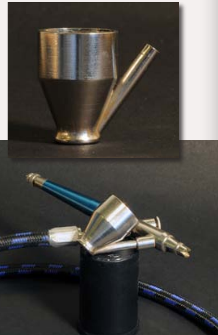
Figure 2: A color cup is a good way to handle small quantities of paint and is particularly useful with thinned-down weathering colors. On this single-action brush, the top button controls the airflow and the screw at the back adjusts to control paint flow.
