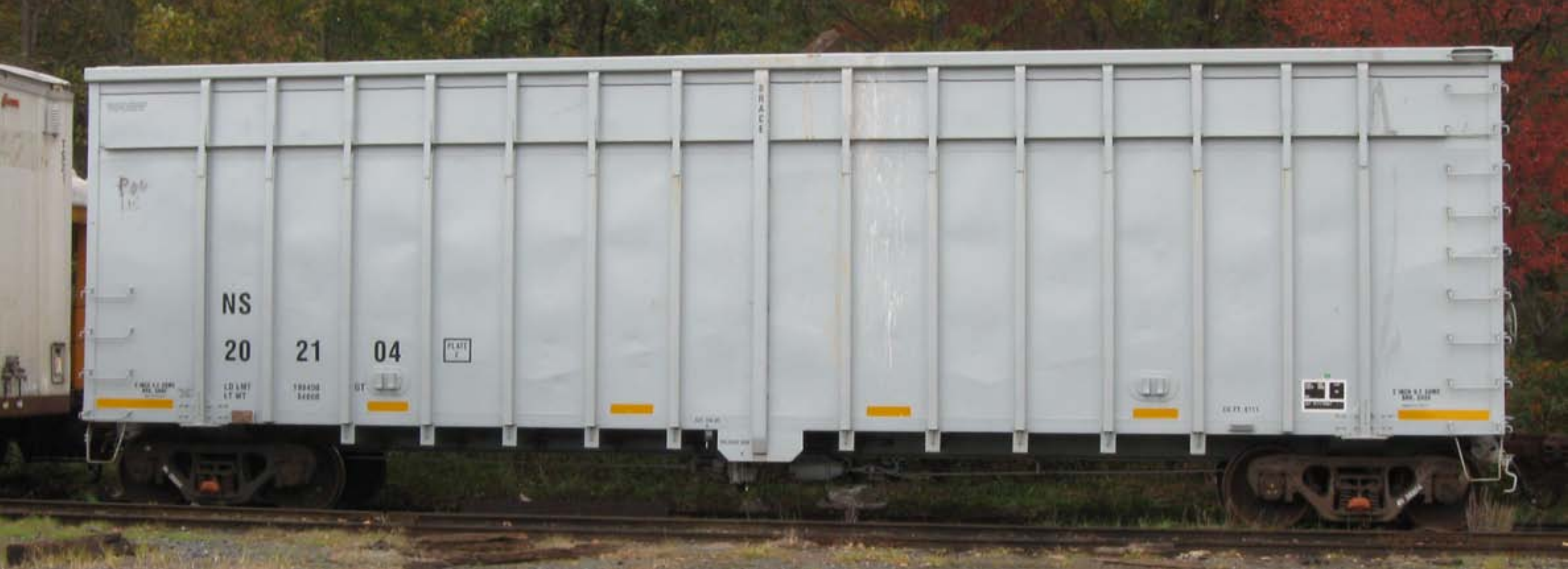
Figure 1: This NS C&D hopper looks like a “new” car, however close examination reveals the outline of the dual hopper bays, giving away its heritage as a former Airslide covered hopper (see all 3 pictures).
