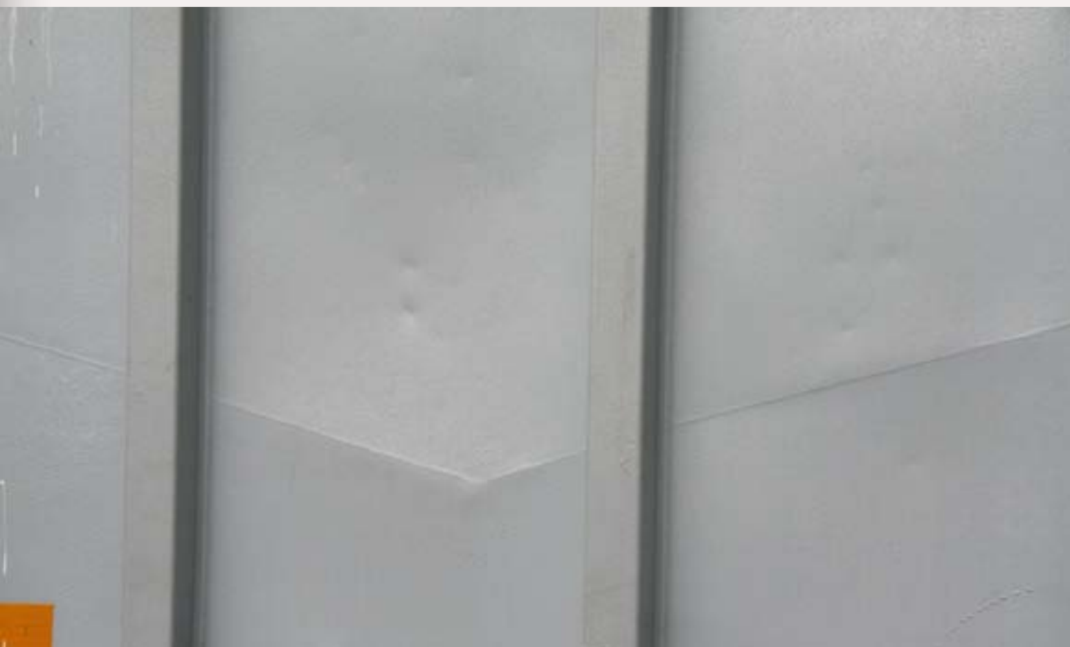
Figure 1: This NS C&D hopper looks like a “new” car, however close examination reveals the outline of the dual hopper bays, giving away its heritage as a former Airslide covered hopper (see all 3 pictures).
