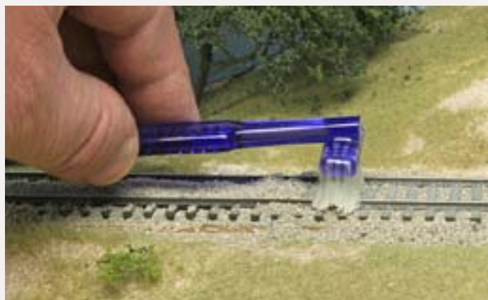
Ballast rake at work.
