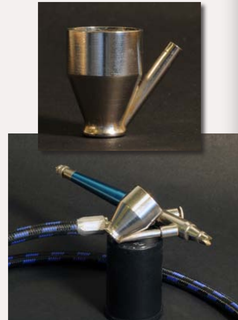
Figure 2: A color cup is a good way to handle small quantities of paint and is particularly useful with thinned-down weathering colors. On this single-action brush, the top button controls the airflow and the screw at the back adjusts to control paint flow.
