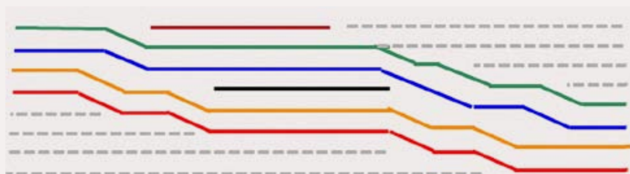
FIGURE 5b: Re-aligned crossovers allow adjustment of track locations without an obvious “S” curve. When applied in multiples, they can move tracks north and south as desired.
