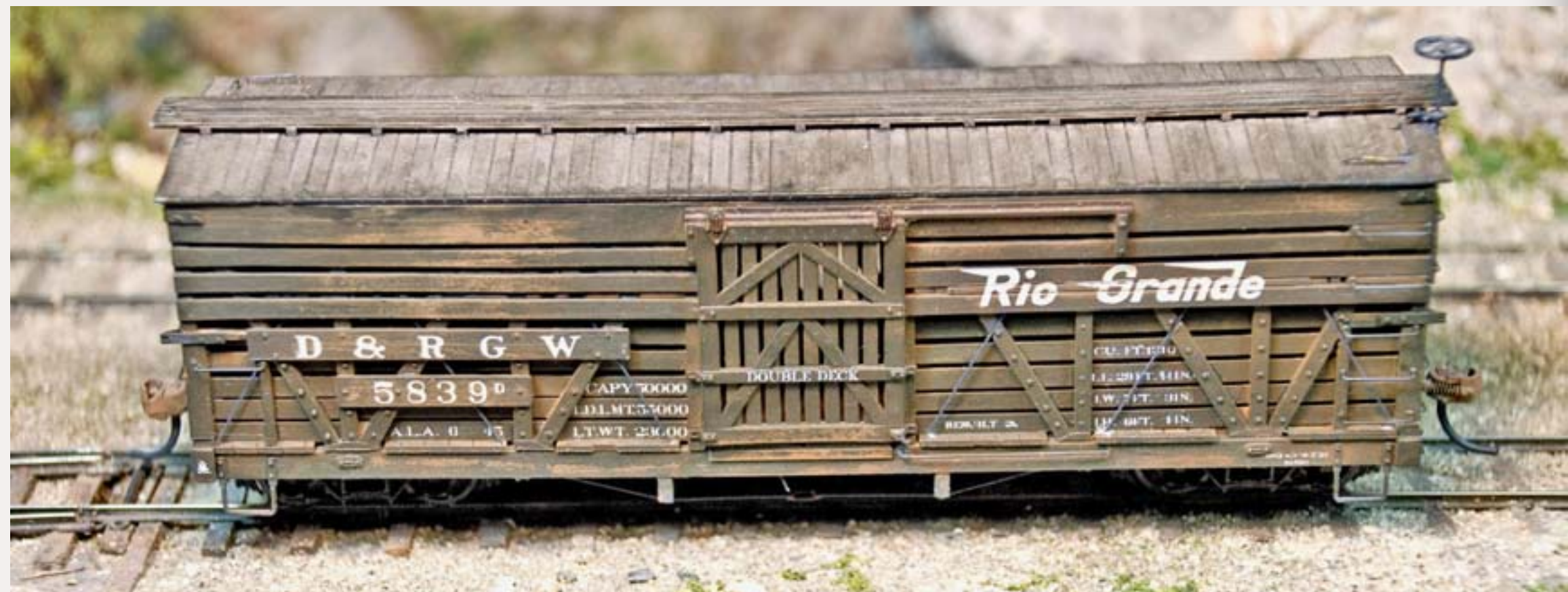
Figure 6. Watercolor pencils are used to simulate worn wood.
