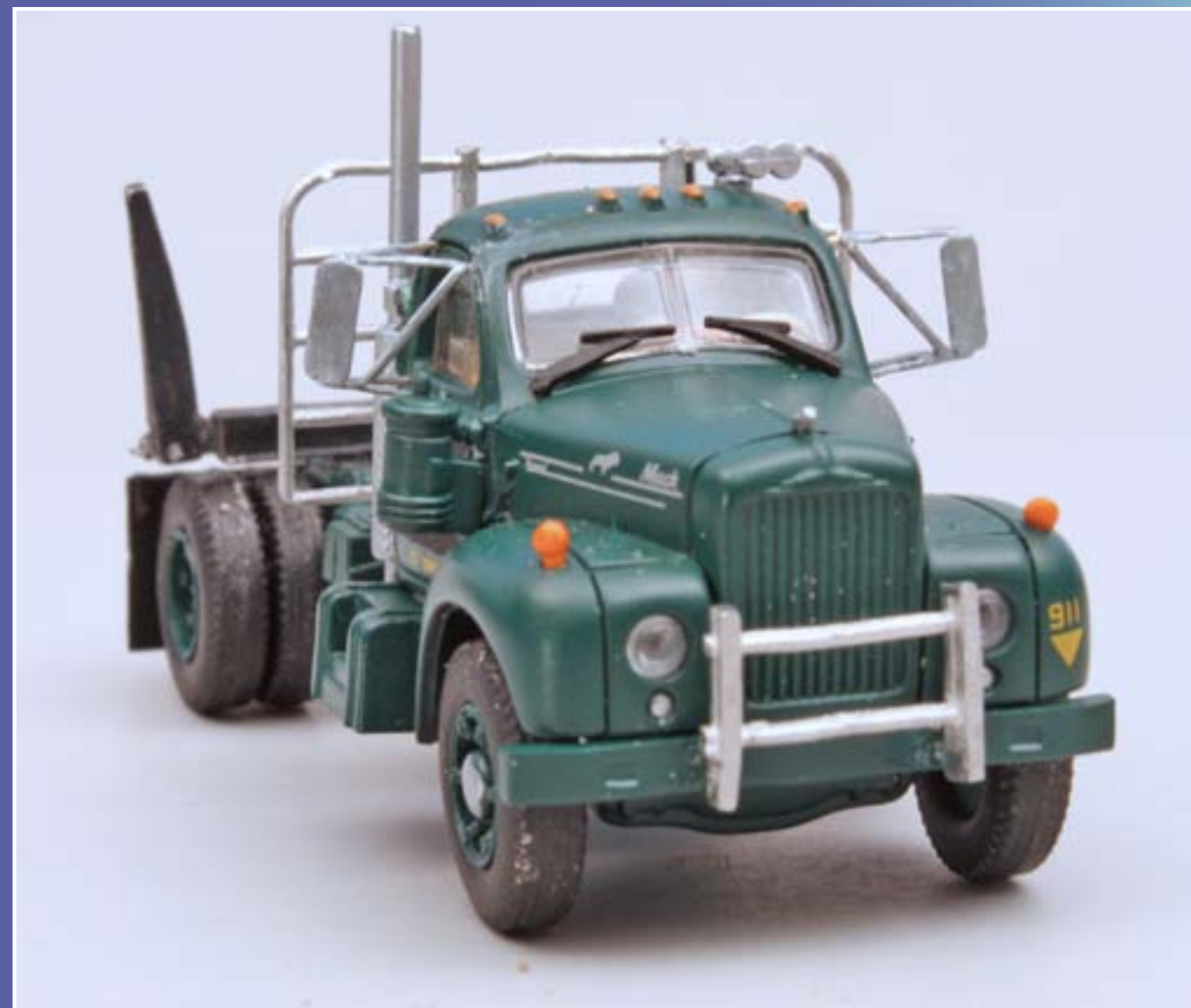
Figure 8: I added etched metal mirrors from Alloy Forms and painted them a light gray. I also decided that I needed a brush guard. This was fashioned from another headache rack I had broken, but it could easily be made from strip and rod styrene.
