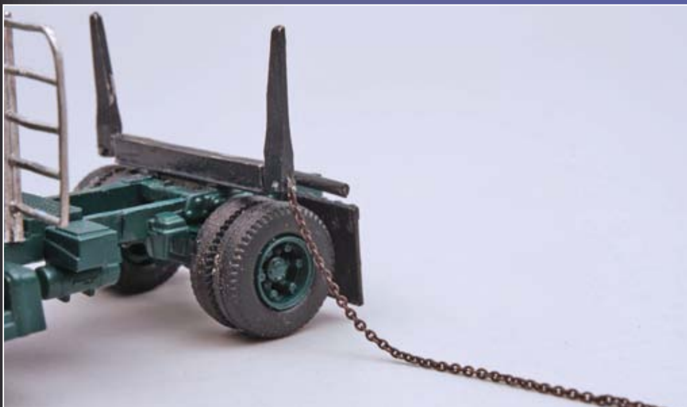
Figure 16: The next step was to add the details to the log bunks. I again used the .010" stainless wire and created small hooks to attach the chain. I used chain from A-Line, affixing one end to the hook with CA.
