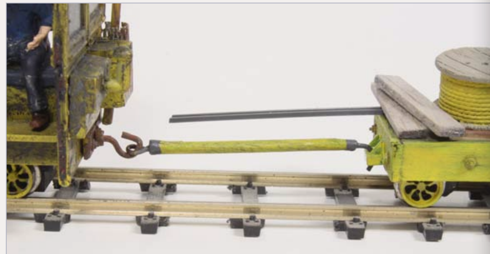
FIGURE 6: The drawbar is long enough to allow a piece of rail to balance on the trailer and not hit the speeder. The hook on the right end of the drawbar has a slight curve to keep it from popping up while being pulled.
