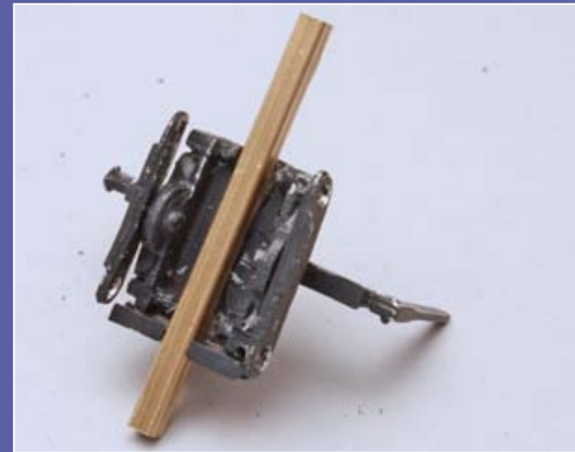
Figure 11: I cut a piece of 5/32" square brass tubing to 10' scale feet which would be used on the bogey. I then affixed the larger diameter piece to the underside of the bogey using CA.
