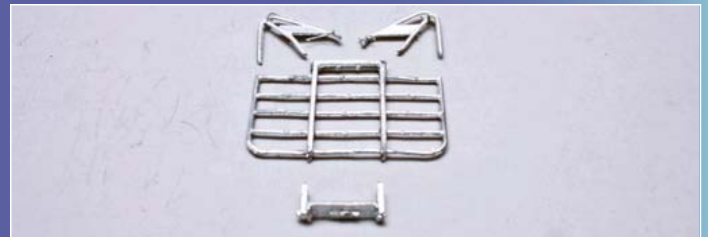
Figure 5: I then prepped the headache rack to be placed on the frame. The headache rack was too modern for the type of truck I was trying to model, so I made a few cuts and achieved a back-dated rack. Since these are cast metal parts, they will take a little time to clean up, I use a sharp knife and a set of small jeweler's files.
