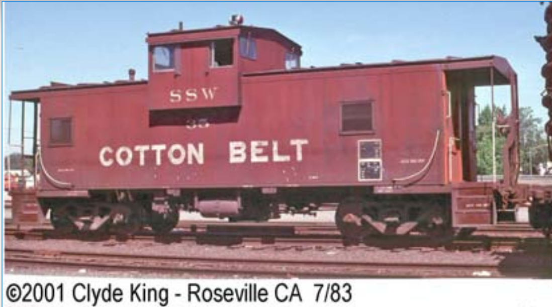
Figure 5: Here's a prototype photo of the C-40-9 series caboose. Photo by Clyde King, from Richard Percy's fabulous SP web site: http://espee.railfan.net/espee.html .
