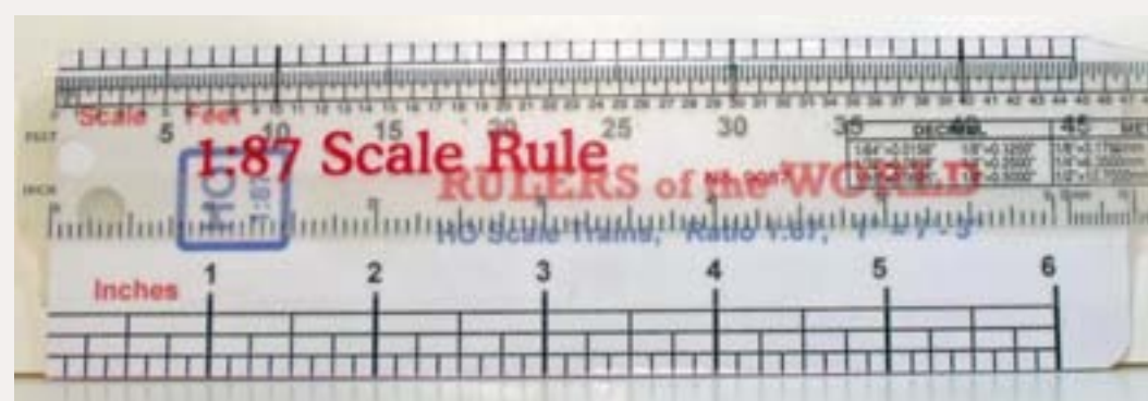
Figure 2: Comparison of a Rulers of the World ruler and another plastic 1:87 scale ruler. Their measurements match up to 15 feet, but then begin to diverge slightly until they disagree by about 1/4 of a scale foot at 45 scale feet.
