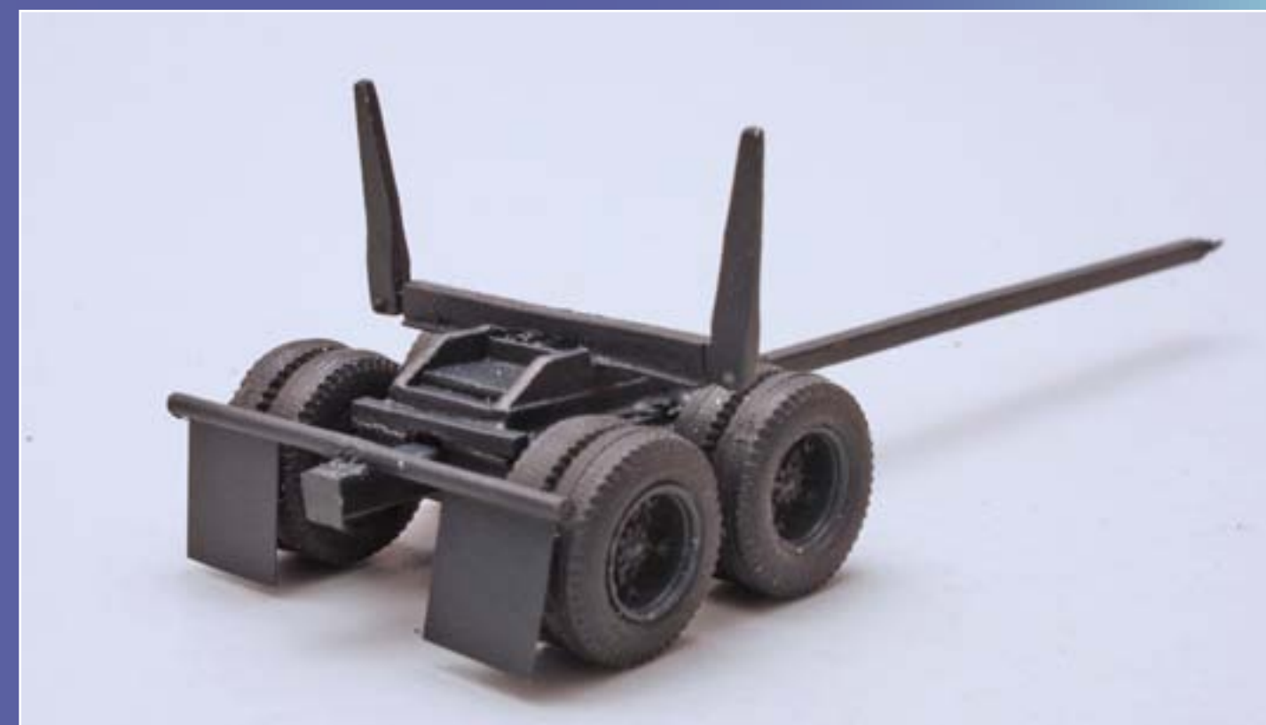
Figure 15: Here is the rear view of the bogey. You can see, I also added a piece of styrene on the rear of the bogey as a stop for the sliding beam.
