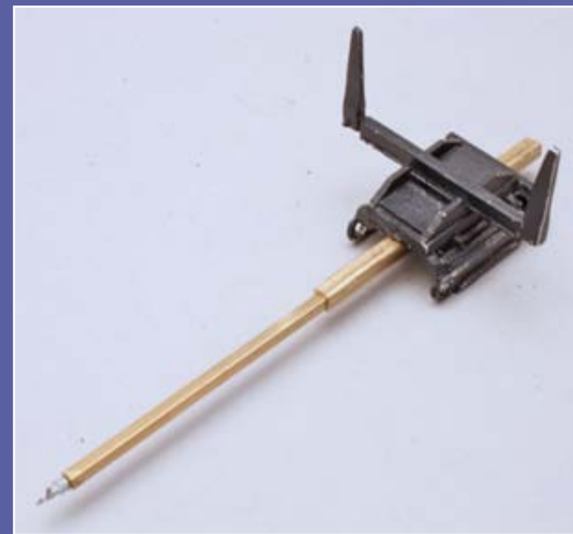
Figure 12: I cut a piece of 1/8" square brass tubing 20 scale feet long. To make a hitch, I took one of the levers from the tow truck sprue and placed it inside of the tube. I used some .010" stainless steel wire to make a loop. I secured this together with CA and placed it inside the other piece of brass to complete the beam.
