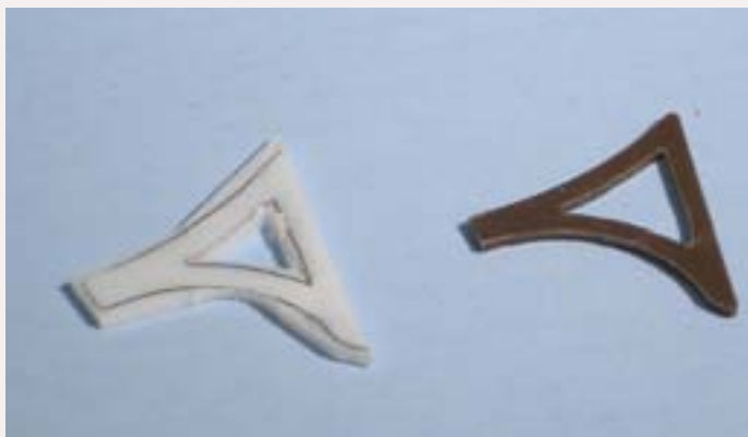
Figure 2: With the bracket traced on the bread clip and the excess plastic trimmed away, all that's left is to finish with a hobby knife and files.
