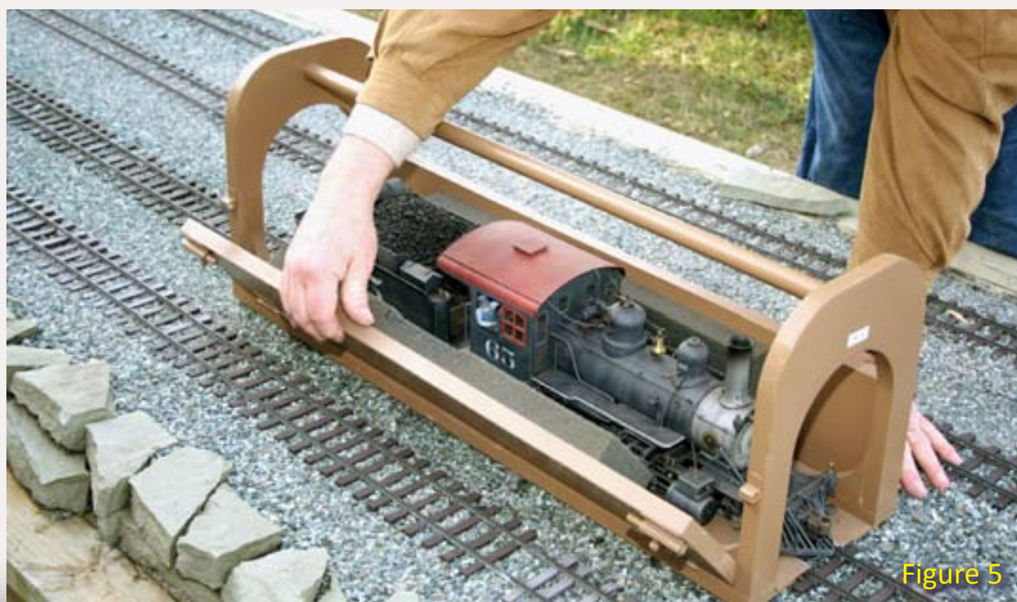
Figure 5: Note the soft, gray foam glued to the inside surface of the side panels. The foam is cut to length, width, and thickness for each loco and contoured to match any protruding details. Although the front and rear of the carrier are open, the foam grips the loco tightly and keeps the heavy engine from sliding forward or backward.
